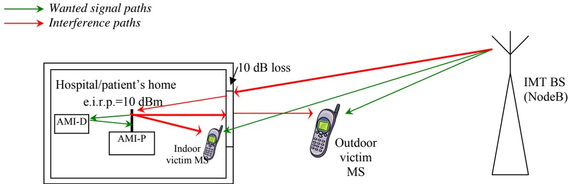
**Figure 4: Interference scenarios LP-AMI vs IMT-2000 Downlink**
