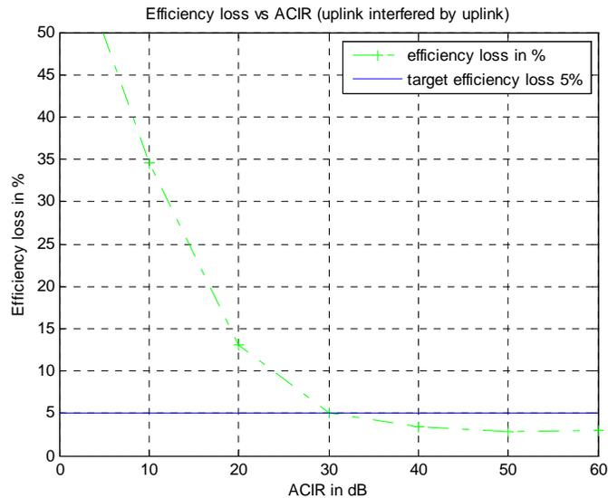
Figure 35: WiMAX UL modulation efficiency loss due to interference from WiMAX UL in urban area
