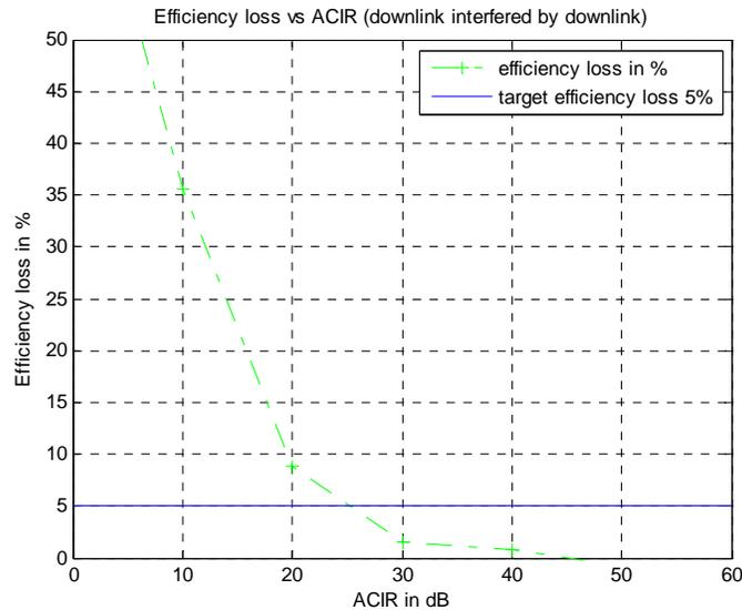
**Figure 26: WiMAX DL modulation efficiency loss due to interference from UMTS DL in rural area**
