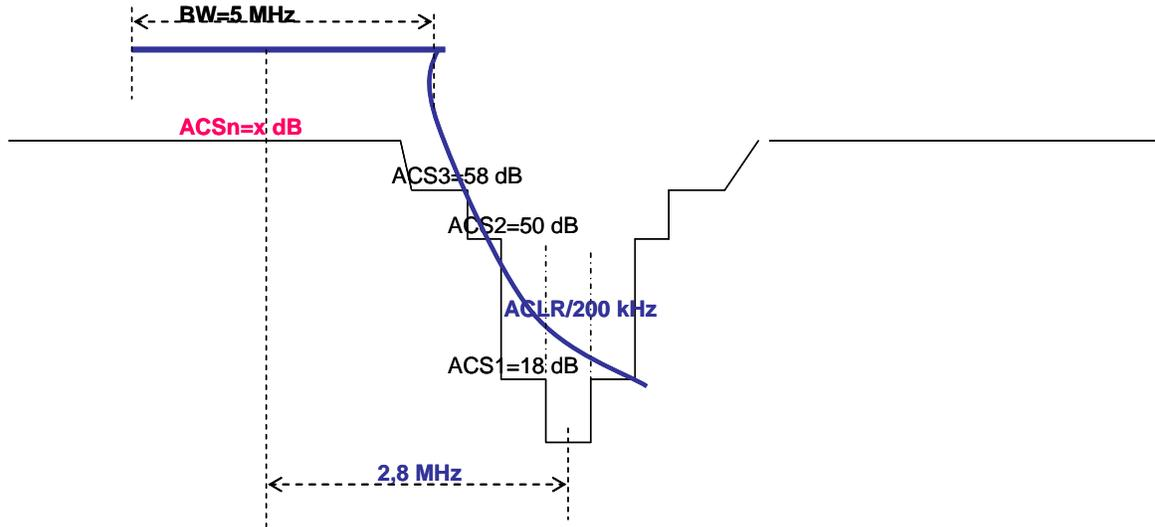
Figure 41: ACLR and ACS between LTE/WiMAX 5 MHz channel and GSM 200 kHz channel
