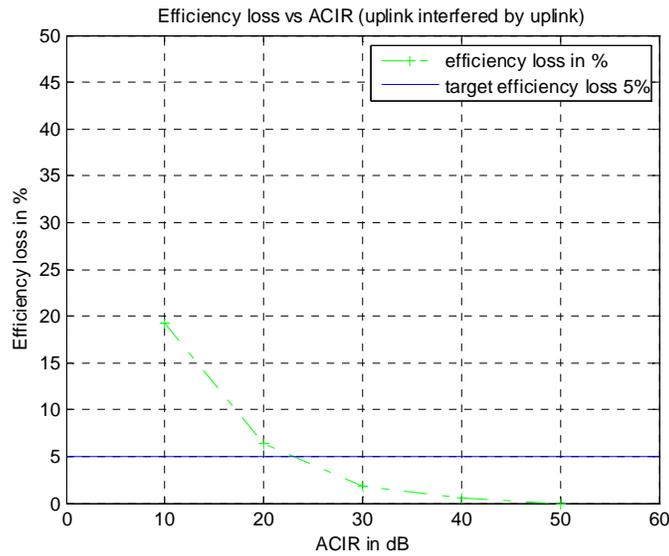
**Figure 27: WiMAX UL modulation efficiency loss due to interference from UMTS UL in urban area**
