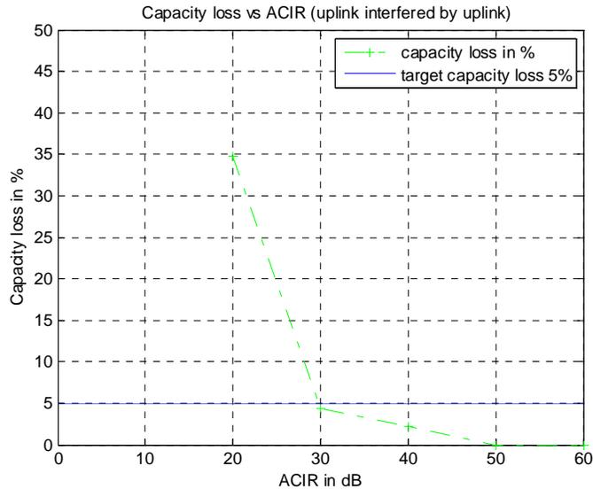
**Figure 23: UMTS UL capacity loss due to interference from WiMAX UL in urban area**
