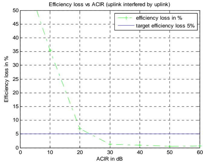
**Figure 36: WiMAX UL modulation efficiency loss due to interference from WiMAX UL in rural area**
