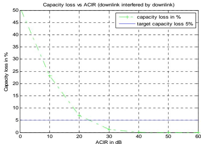
**Figure 21: UMTS DL capacity loss due to interference from WiMAX DL in urban area**
