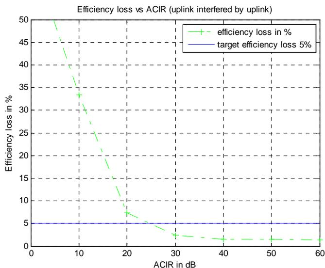
Figure 40: WiMAX UL modulation efficiency loss due to interference from WiMAX UL in rural area
