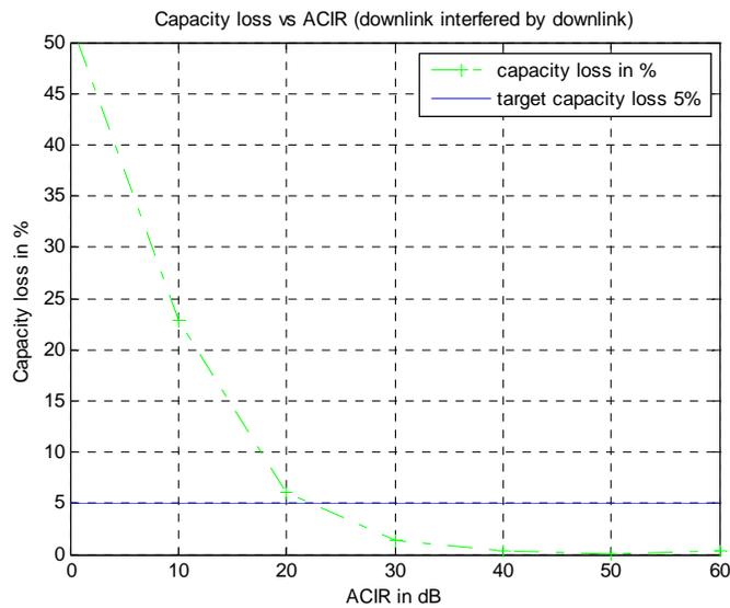
**Figure 17: UMTS DL capacity loss due to interference from WiMAX DL in urban area**
