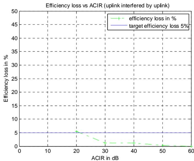
**Figure 28: WiMAX UL modulation efficiency loss due to interference from UMTS UL in rural area**
