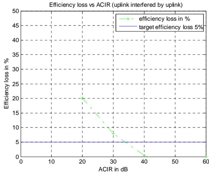
**Figure 31: WiMAX UL modulation efficiency loss due to interference from UMTS UL in urban area**
