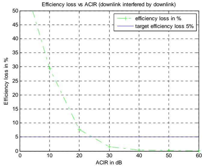
Figure 38: WiMAX DL modulation efficiency loss due to interference from WiMAX DL in rural area
