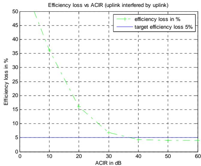
Figure 39: WiMAX UL modulation efficiency loss due to interference from WiMAX UL in urban area
