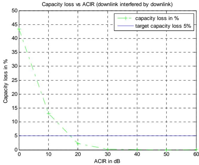
**Figure 22: UMTS DL capacity loss due to interference from WiMAX DL in rural area**
