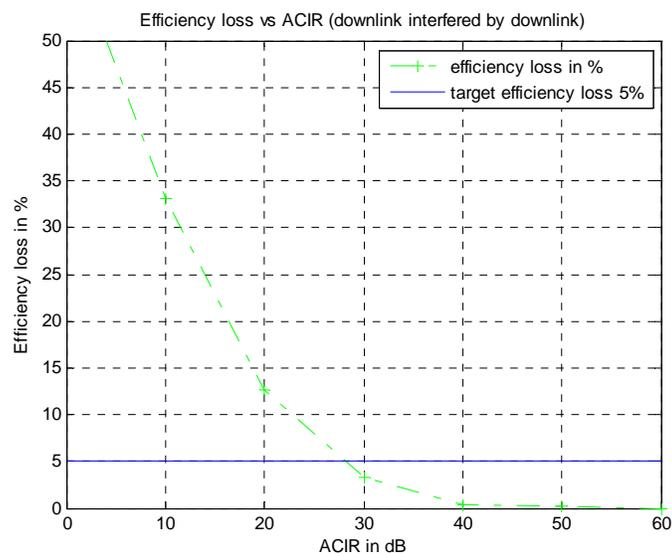
**Figure 37: WiMAX DL modulation efficiency loss due to interference from WiMAX DL in urban area**
