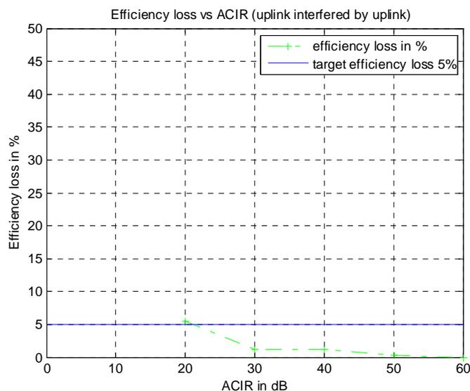
**Figure 32: WiMAX UL modulation efficiency loss due to interference from UMTS UL in rural area**
