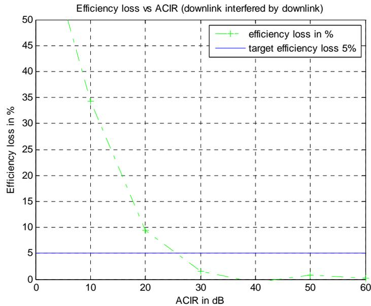
Figure 30: WiMAX DL modulation efficiency loss due to interference from UMTS DL in rural area
