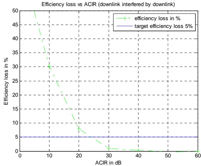
Figure 34: WiMAX DL modulation efficiency loss due to interference from WiMAX DL in rural area
