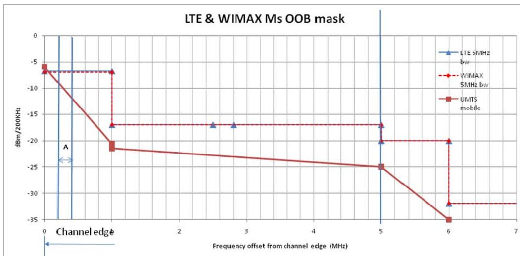
**Figure 4: Graphical comparison of LTE and WiMAX Mobile station SEMs (5MHz bandwidth)**
