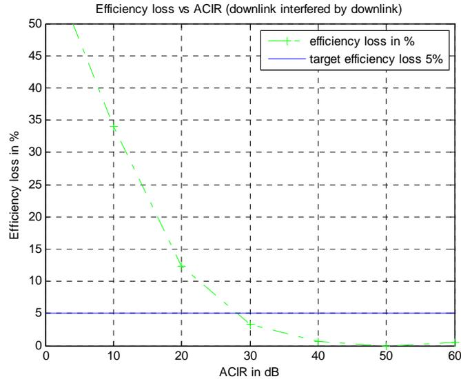
Figure 29: WiMAX DL modulation efficiency loss due to interference from UMTS DL in rural area
