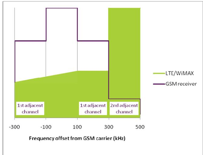
**Figure 6: GSM receiver adjacent channels (300 kHz separation)**
