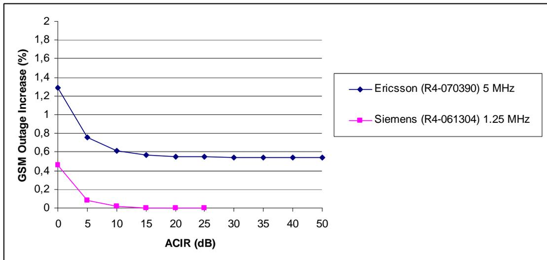
Figure 9: GSM uplink outage (3GPP TR36.942: Figure 7.19a)
