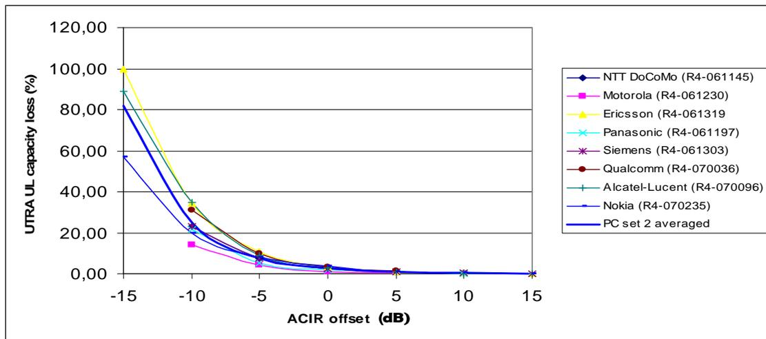
Figure 11: UTRA FDD uplink capacity loss due to interference from LTE
