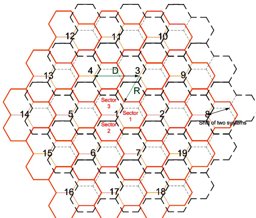
**Figure 16: Network layout of large area multiple systems deployment**
