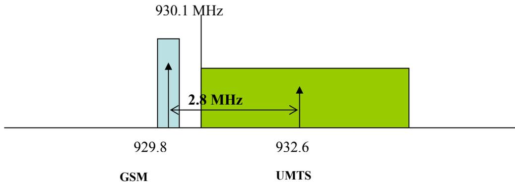
**Figure 5: Frequency arrangement of a GSM carrier and an UMTS carrier**
