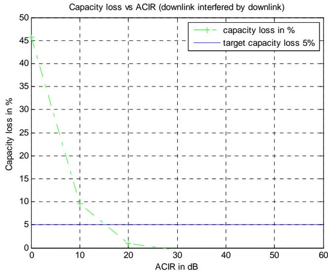
**Figure 18: UMTS DL capacity loss due to interference from WiMAX DL in urban area**
