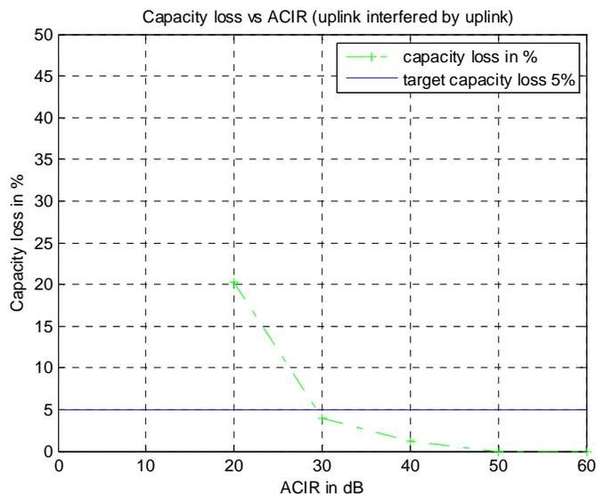
**Figure 24: UMTS DUL capacity loss due to interference from WiMAX DUL in rural area**
