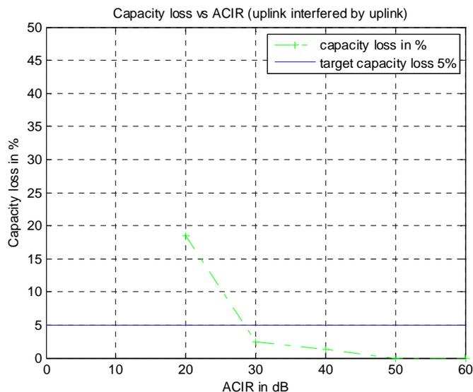
**Figure 20: UMTS UL capacity loss due to interference from WiMAX UL in rural area**
