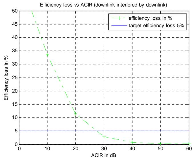
**Figure 33: WiMAX DL modulation efficiency loss due to interference from WiMAX DL in urban area**
