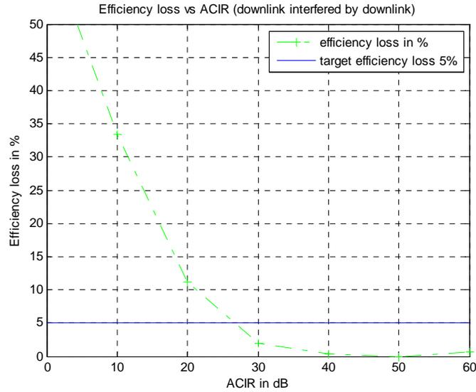
**Figure 25: WiMAX DL modulation efficiency loss due to interference from UMTS DL in urban area**
