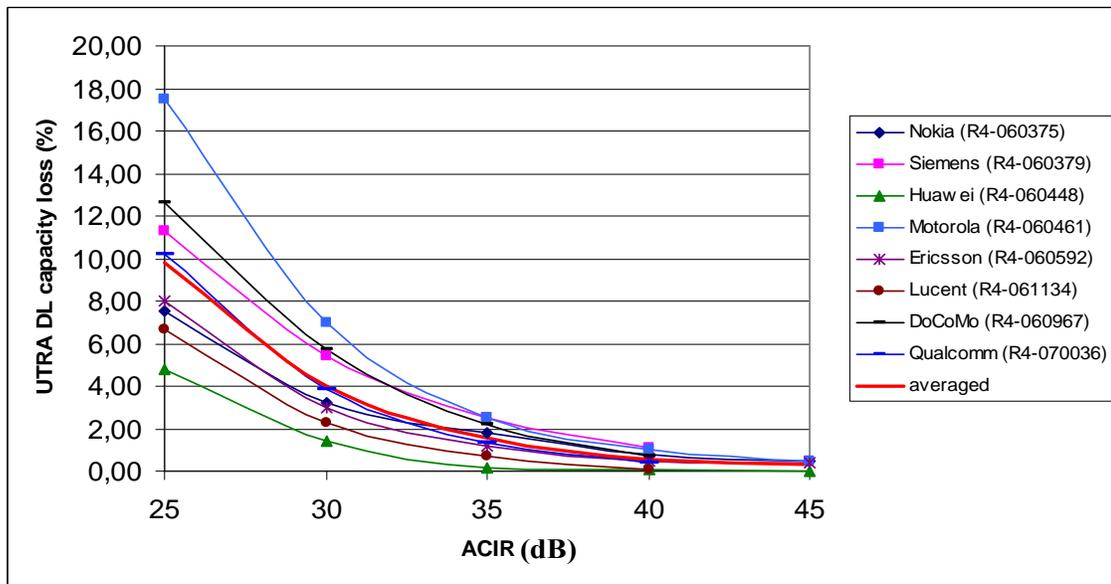
**Figure 10: UTRA FDD capacity loss due to interference from LTE**
