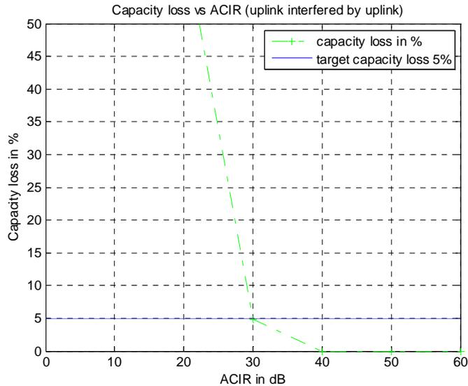
**Figure 19: UMTS UL capacity loss due to interference from WiMAX UL in urban area**
