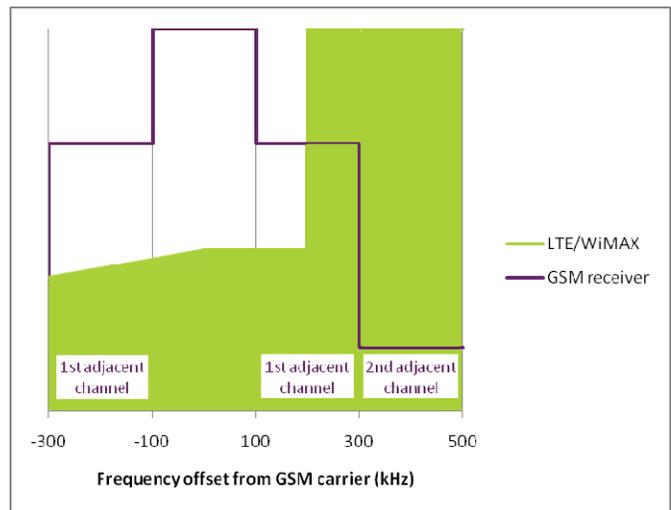
**Figure 7: GSM receiver adjacent channels (200 kHz separation)**
