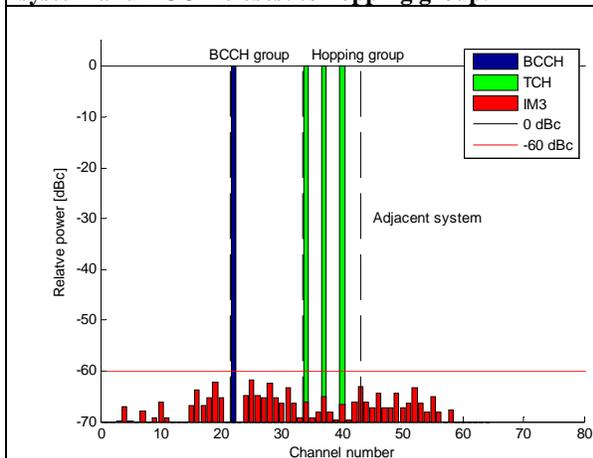
**Figure A3.3c: TCH hopping group close to band edge and BCCH furthest away from TCH group**
