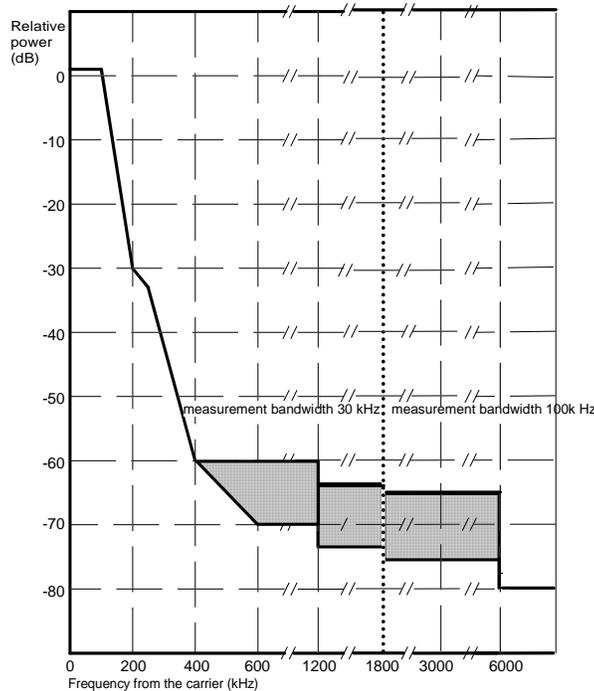
**Figure A1.1: Spectrum due to modulation and wideband noise for single GMSK carrier**
