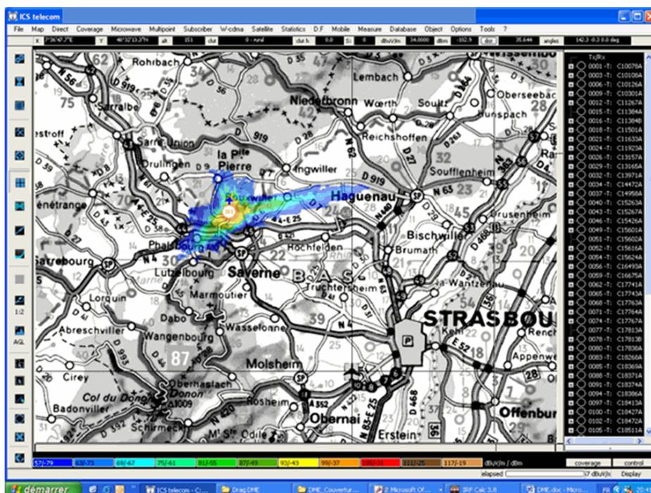
Figure A11.1: Coverage of the DME situated in Bouxwiller (67 330) at a 200 m altitude
