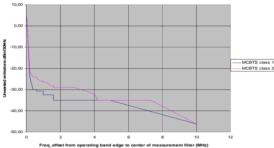
Figure A1.3: Out-of-band emission masks for MCBTS with 4 carriers at 600 kHz spacing (900 MHz)
