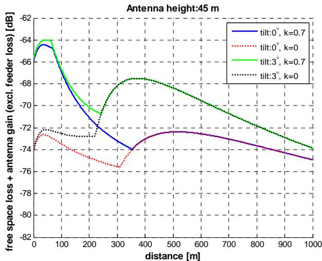
Figure 48: Free space path loss and public GSM BTS antenna gain as a function of distance between GSM-R terminal and public GSM BTS. Antenna height 45 m
