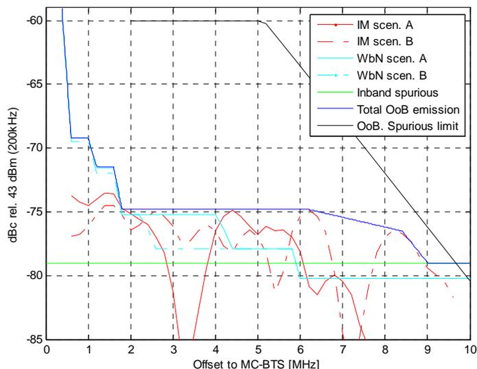
**Figure 41: GSM unwanted emissions with power control**
