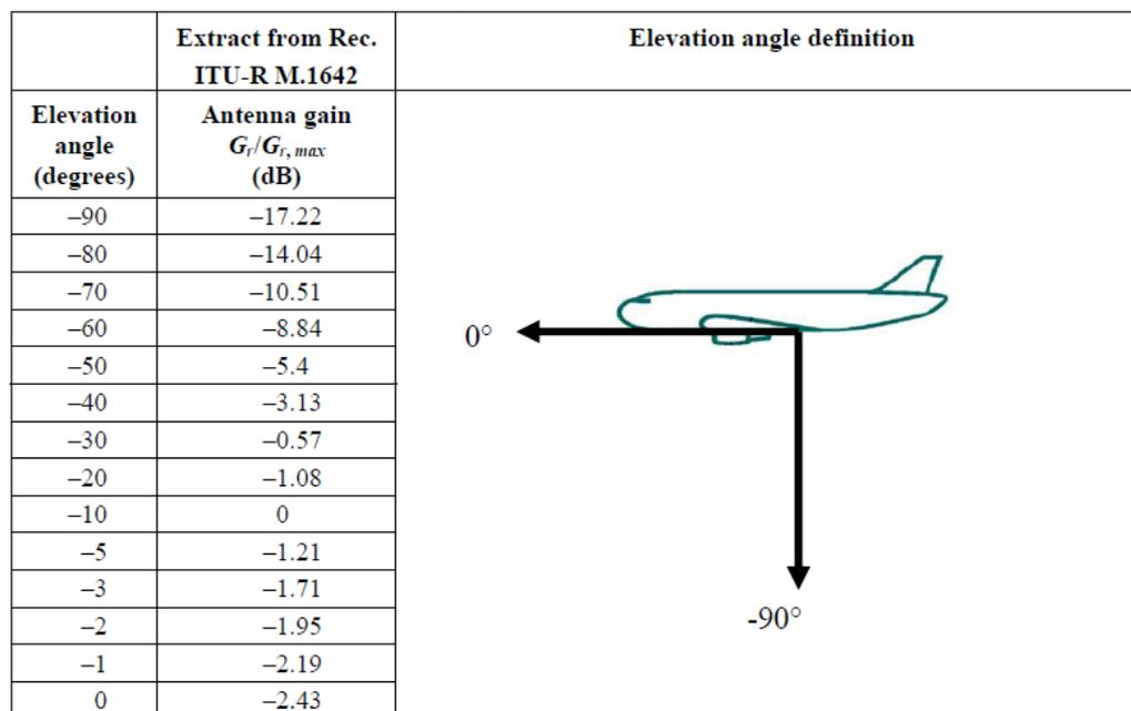
**Figure A8.2: DME antenna gain for elevation angles between 0°...-90°**
