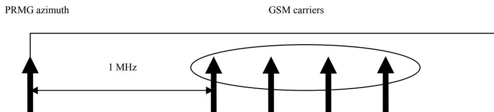
**Figure 13: Carrier separation between MCBTS and PRMG azimuth channel**
