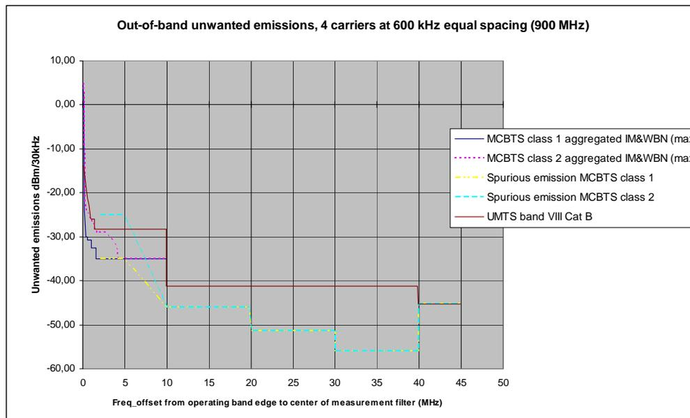
**Figure A3.9: Spectrum requirements GSM 900 MHz band**
