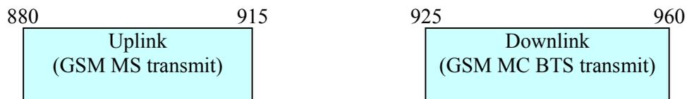
**Figure 8: The frequency plan of GSM in the 900 MHz band**
