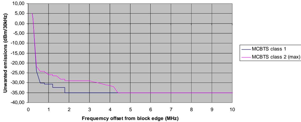
Figure A1.2: Inband unwanted emission masks for MCBTS with 4 carriers at 600 kHz spacing (900 MHz)
