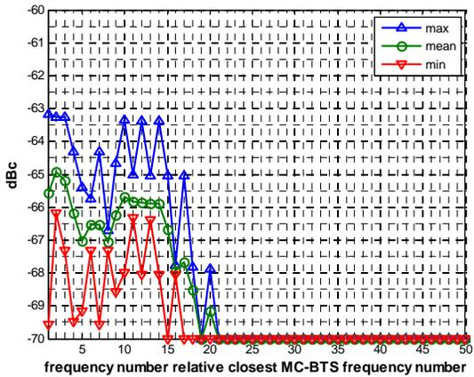
Figure A3.4c: TCH hopping group close to band edge and BCCH furthest away from TCH group
