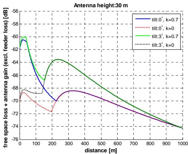
Figure 47: Free space path loss and public GSM BTS antenna gain as a function of distance between GSM-R terminal and public GSM BTS. Antenna height 30 m
