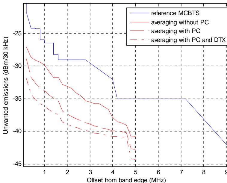
**Figure A10.1: Reference and average unwanted emissions from a Class 2 MCBTS**
