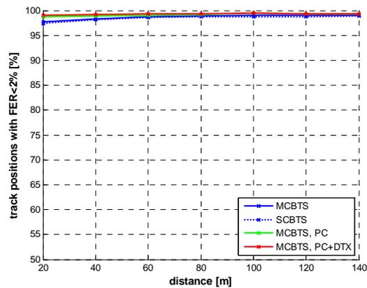
MC-BTS antenna height 30m, k=0.7, tilt 3°
