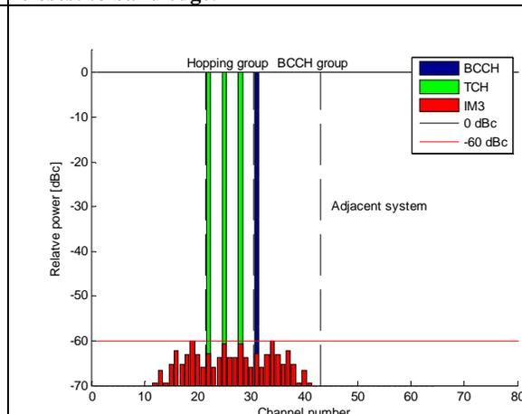
**Figure A3.3d: BCCH group at block edge and BCCH furthest away from band edge in that group.**
