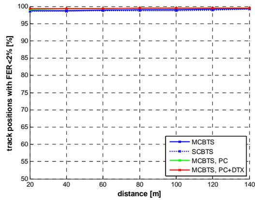
MC-BTS antenna height 45m, k=0.7, tilt 3°
