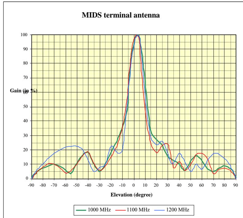
**Figure 42: MCBTS MIDS terminal vertical antenna diagram**
