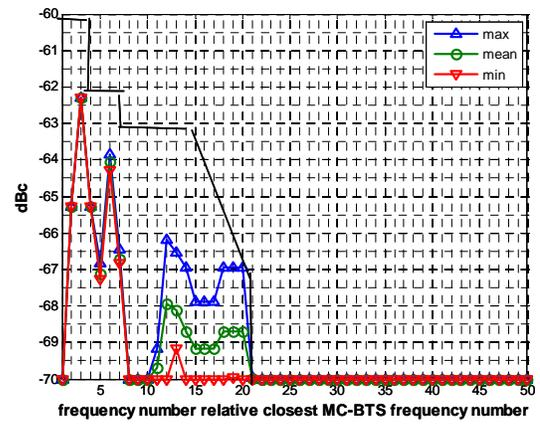
Figure A3.5b: BCCH group close to band edge, BCCH close to TCH group
