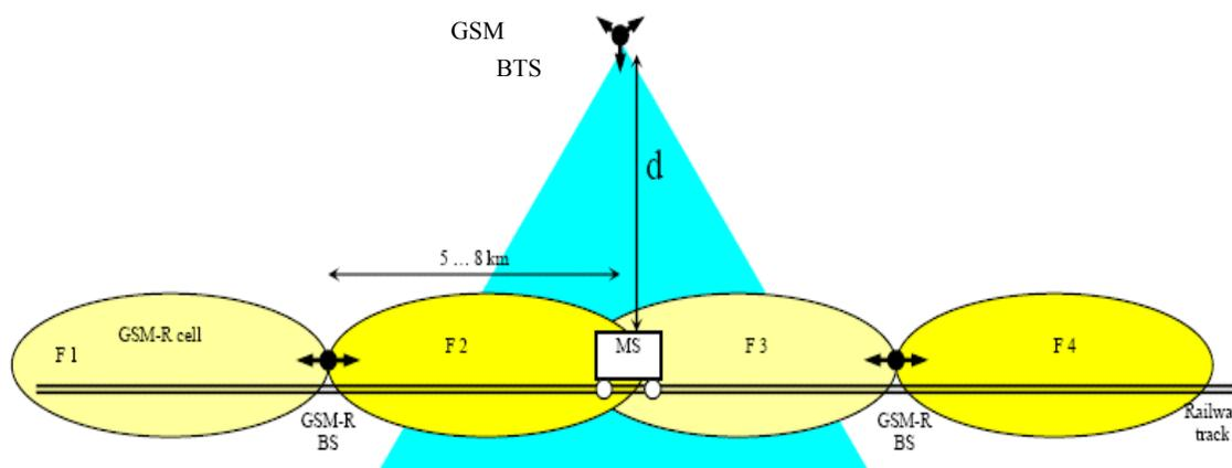
**Figure 26: Worst case scenario: E-GSM MCBTS interference to GSM-R MS**
