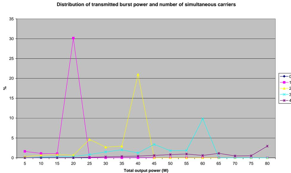
Figure A9.7: Distribution of used number of carriers and corresponding total carrier power
