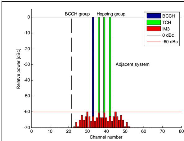
**Figure A3.3a: TCH hopping group close to adjacent system and BCCH closest to hopping group.**
