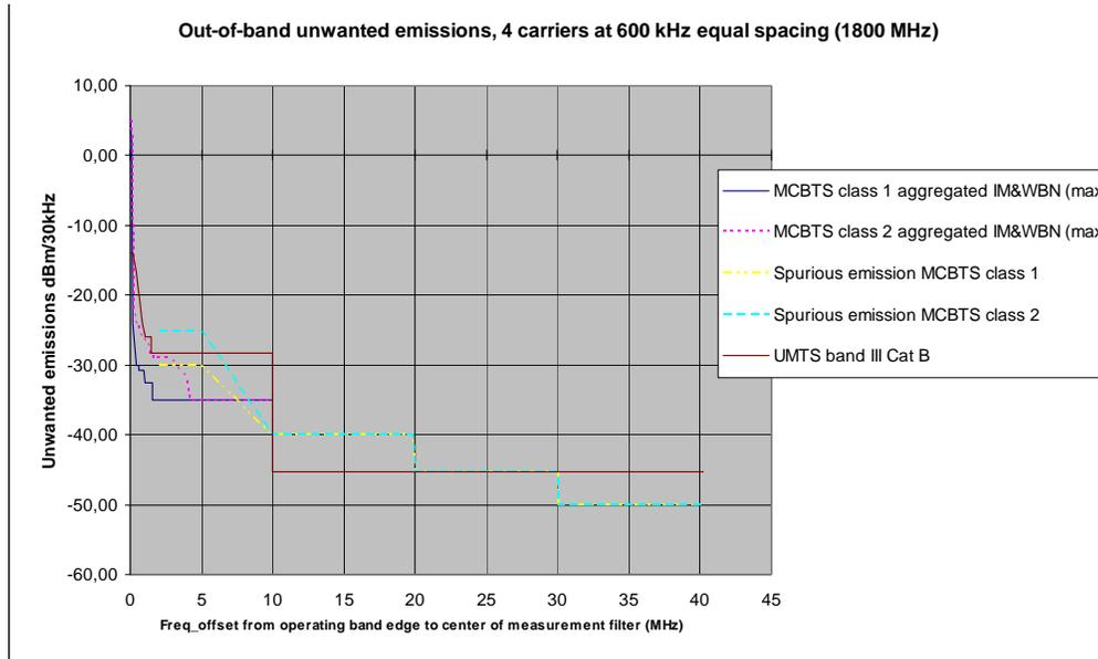
Figure A3.10: Spectrum requirements DCS 1800 MHz band
