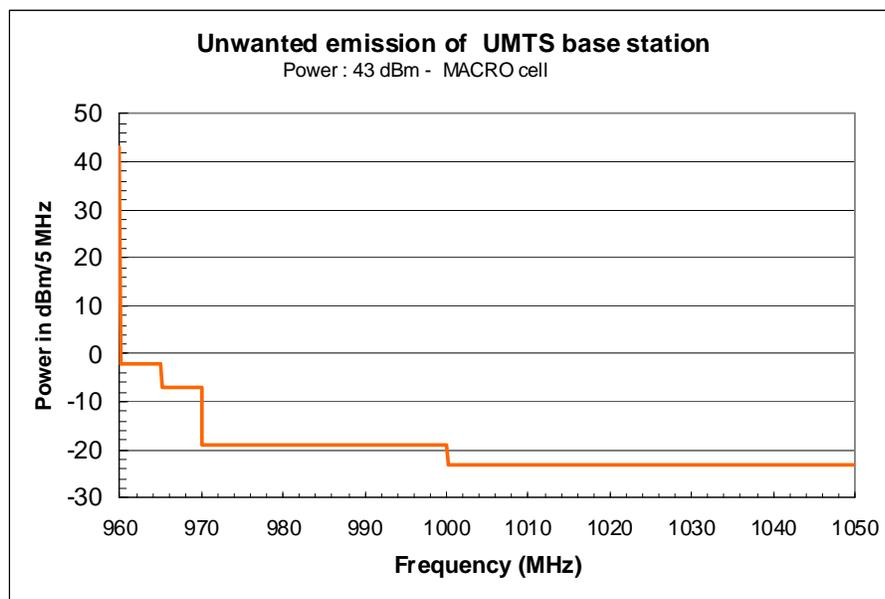
Figure 43: Unwanted emissions of UMTS Base Station at 960 MHz
