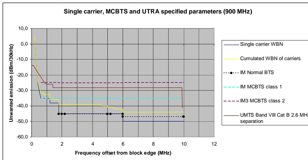
**Figure A3.2: In-band unwanted emissions for UTRA, GSM single carrier and multi-Carrier BTS in 900 MHz frequency band**
