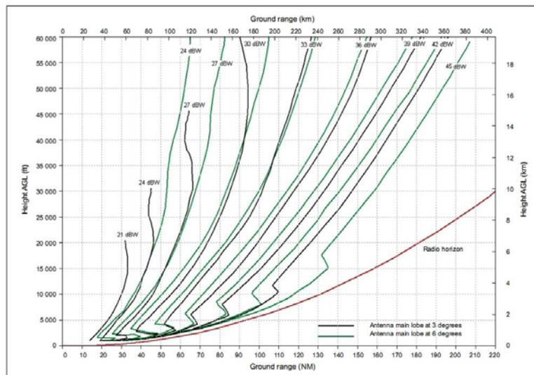
**Figure A8.1: Necessary EIRP to achieve a power density of -89 dBW/m<sup>2</sup> as a function of height above and distance from the DME**
