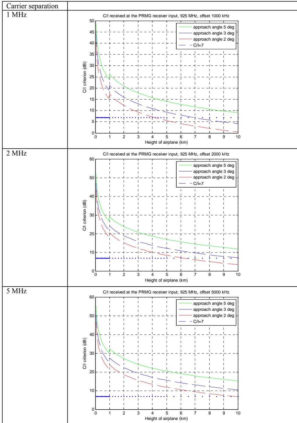
**Figure 17: RSN C/I with 1, 2 and 5 MHz carrier separation to MC BTS**
