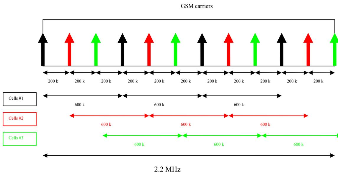
**Figure 6: MC BTS carrier distribution**
