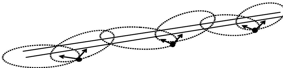
Figure 21: GSM-R deployment scenario
