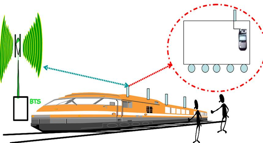
Figure 22: Connection between train mounted antenna and MS situated inside of the train
