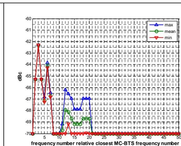
**Figure A3.4b: BCCH group at block edge and BCCH closest to band edge.**
