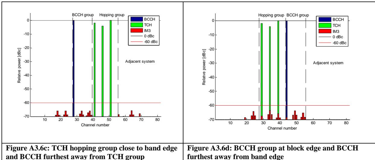
**Figure A3.6a-A3.6d: Frequency allocations according figure A3.3a-A3.3d with power control applied. Power control is 0 dBc, -2 dBc, and -4 dBc for the 3-TCHs**
