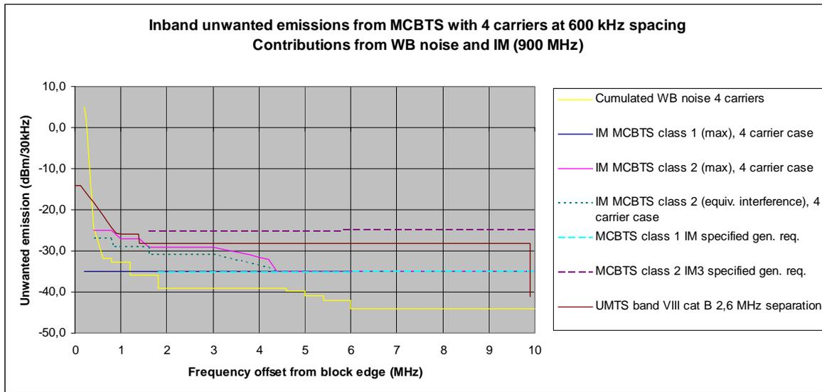
**Figure A3.7. Unwanted emission- contributions from IM and Wideband noise**
