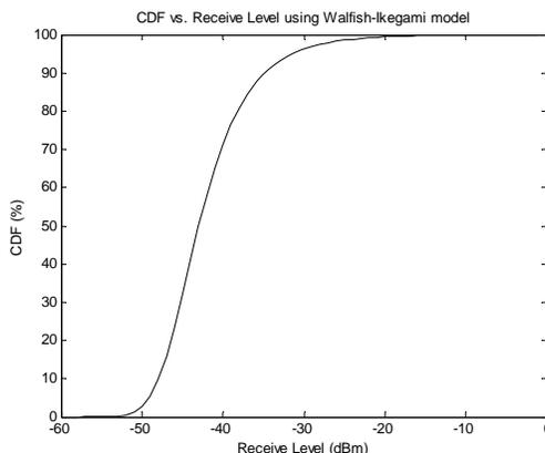
**Figure 49: Receive level in the case of 10 high power MSs, using Walfish-Ikegami propagation model**
