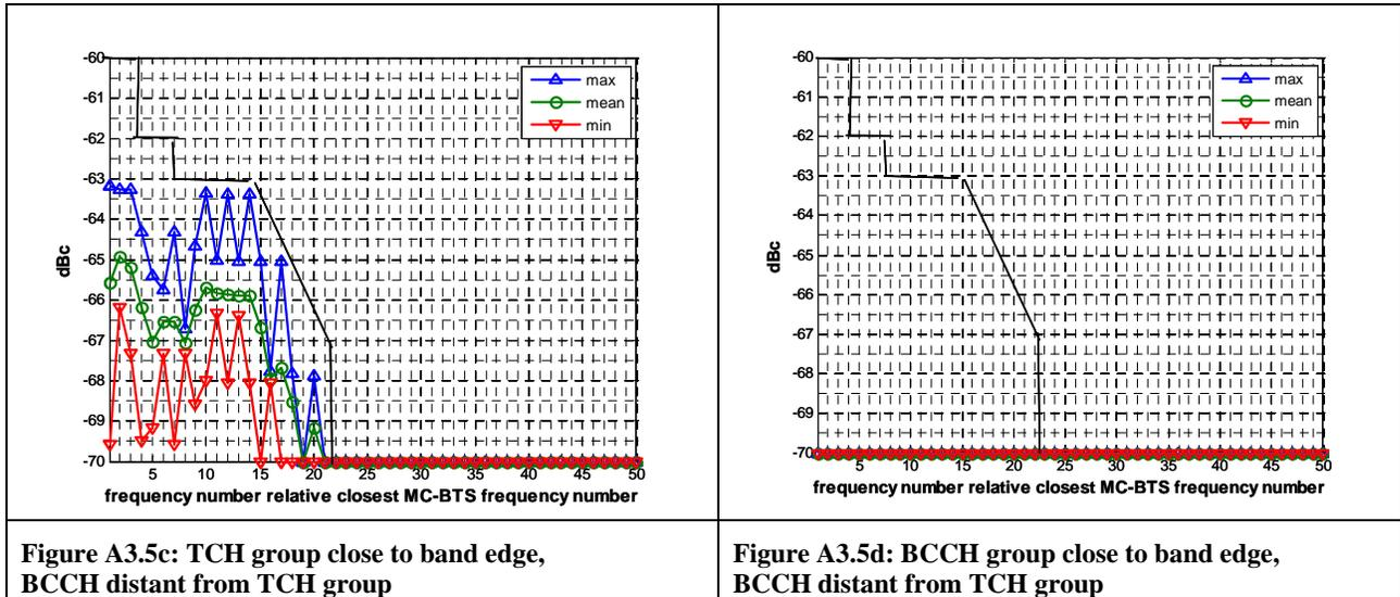
**Figure A3.5a-A3.5d: Creating a mask for Maximum emitted noise levels relative -70 dBc for the allocations in figure A3.3a-A3.3d**
