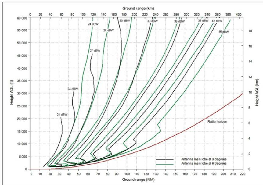
Figure 11: Necessary EIRP to achieve a power density of -89 dBW/m<sup>2</sup> as a function of height above and distance from the DME
