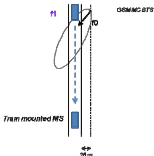
Figure 34: configuration for assessing the interference from GSM UL onto GSM MC BTS
