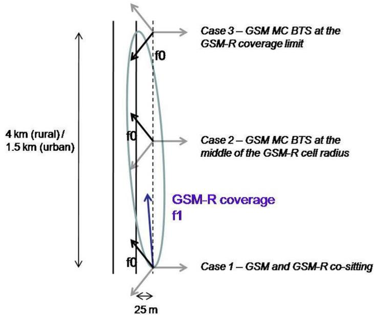
Figure 32: configuration for assessing the interference of GSM MC DL onto GSM-R DL (GSM MC tri-sector antenna)
