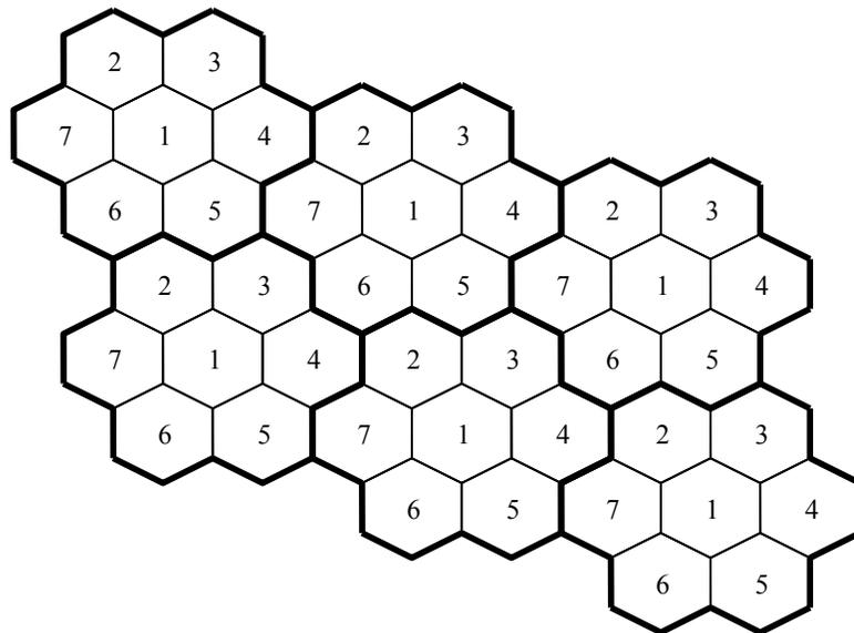
**Figure 35: GSM 7-reuse pattern**
