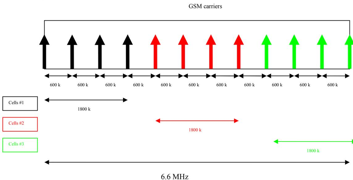
**Figure 14: Different carrier distribution**
