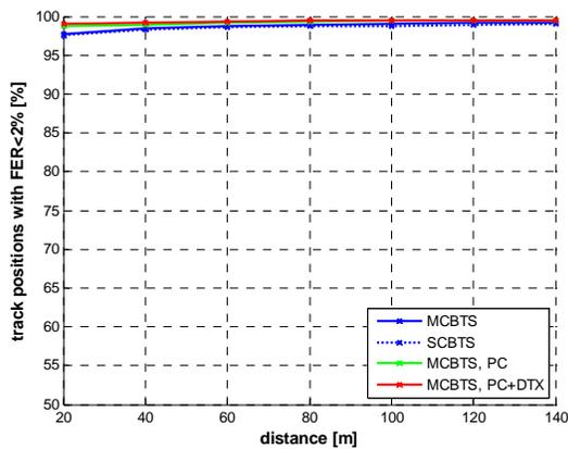
MC-BTS antenna height 30m, k=0.7, tilt 0°
