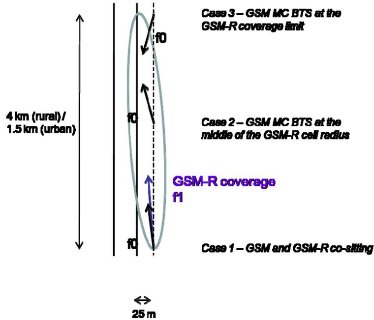
Figure 33: configuration for assessing the interference of GSM-R MC DL onto GSM-R DL (GSM MC bi-sector antenna)
