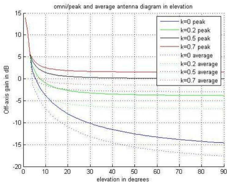
**Figure 7: Antenna diagram in elevation for MCBTS, omni case**
