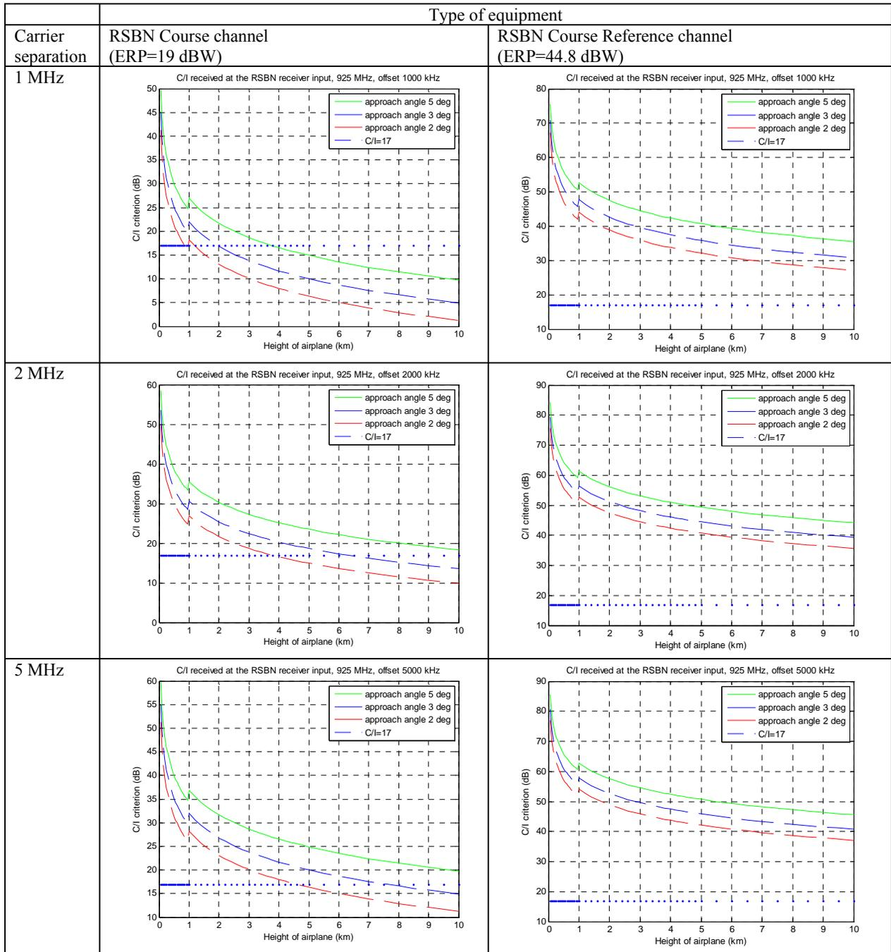
Figure 16: RSNB (ERP=44.8 dBW) C/I with 5 MHz carrier offset to MCBTS
