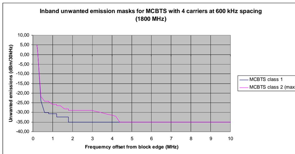
Figure A1.4: Inband unwanted emission masks for MCBTS with 4 carriers at 600 kHz spacing (1800 MHz)
