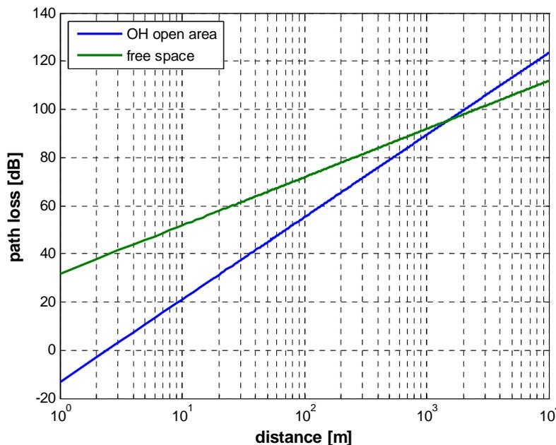
**Figure 23: A comparison of Okumura-Hata open area, BS antenna at 45 meters with free space propagation**
