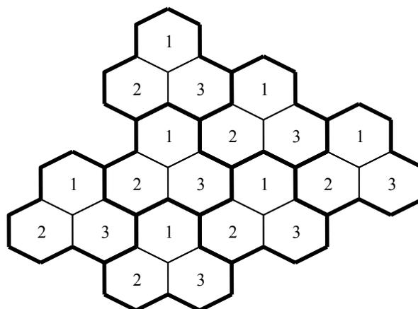
Figure 36: GSM 3-reuse pattern
