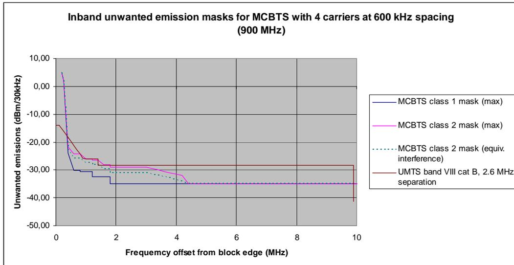
**Figure A3.8: Spectrum mask for max interference levels (class 1 and 2) and equivalent noise level to evaluate the effect of IM3 for MCBTS class 2**
