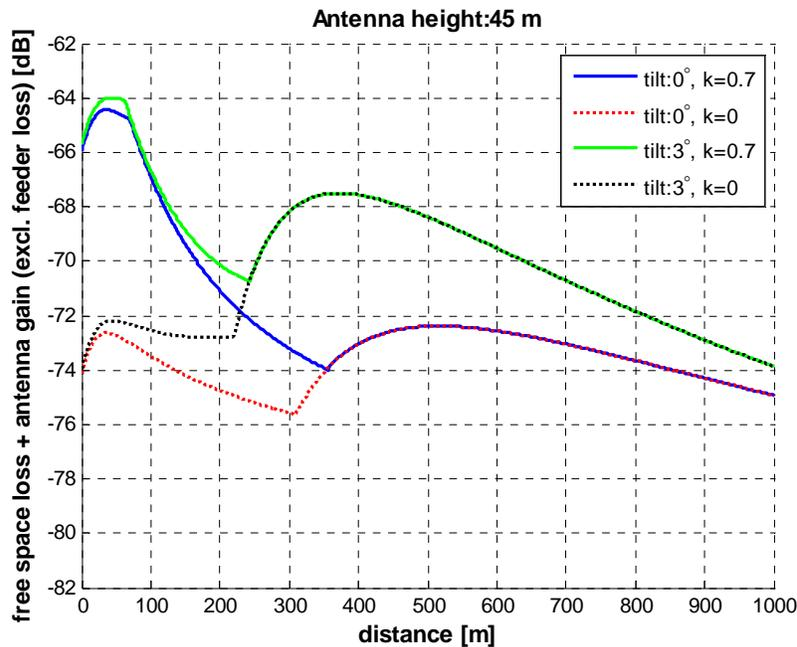
Figure 25: Free space path loss and public GSM BTS antenna gain as a function of distance between GSM-R terminal and public GSM BTS. Antenna height 45 m
