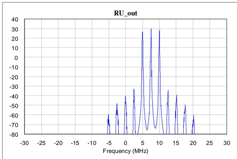
**Figure A3.1: Example of IM spectrum for 3 GSM carriers**
