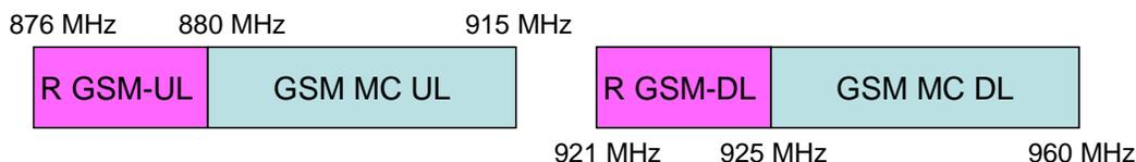
Figure 20: Frequency band plan for GSM-R and GSM in 900 MHz band
