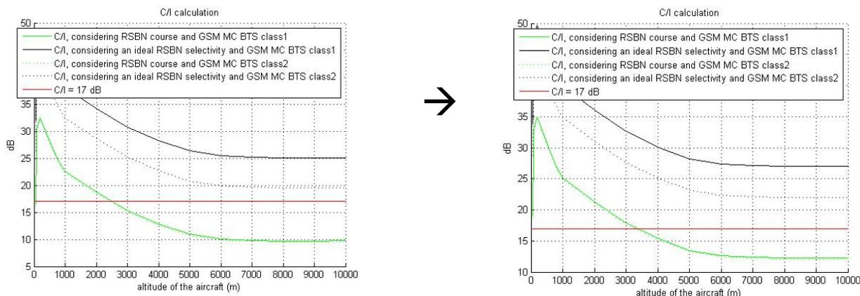
**Figure 15: Effect of different carrier distributions**
