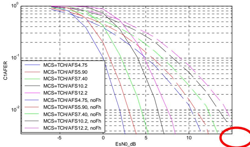
**Figure 27: Link-level performance of AMR speech codecs. Channel model is TU3. Single-antenna receiver.**
