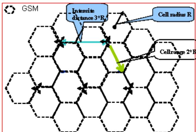
Figure A2.1: GSM network layout
