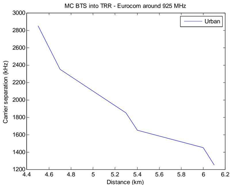
**Figure 12: Worst case MCL for MCBTS into Eurocom TRR depending on carrier separation**
