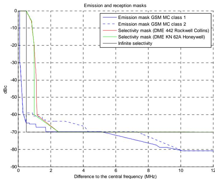
**Figure 39: DME receiver selectivity and GSM MMC emission mask**
