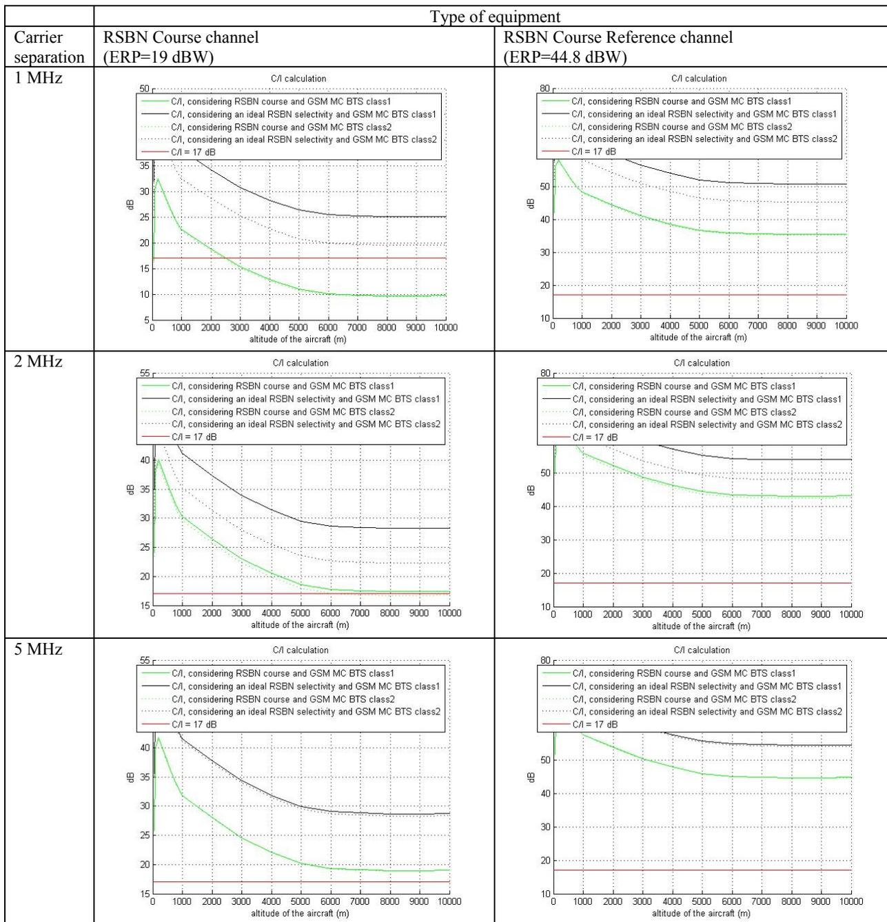
Figure 19: RSNB C/I with 1, 2 and 5 MHz carrier separation to MC BTS
