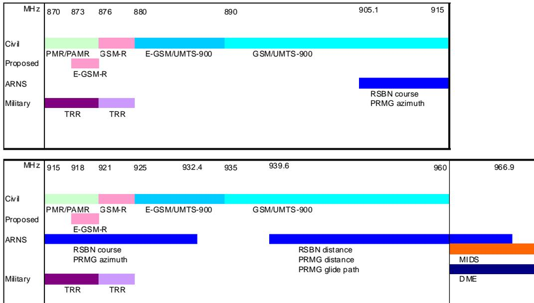
**Figure 2: Frequency usage at the 900 MHz range relevant for the studies in this Report**
