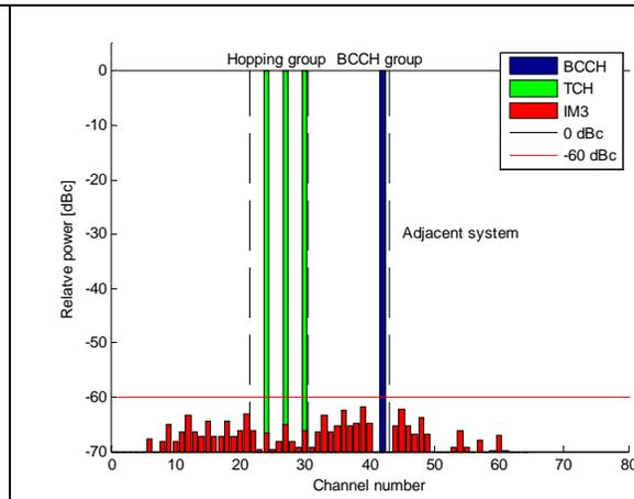
**Figure A3.3b: BCCH group at block edge and BCCH closest to band edge.**
