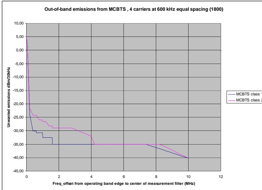
**Figure A1.5: Out-of-band emission masks for MCBTS with 4 carriers at 600 kHz spacing (1800 MHz)**
