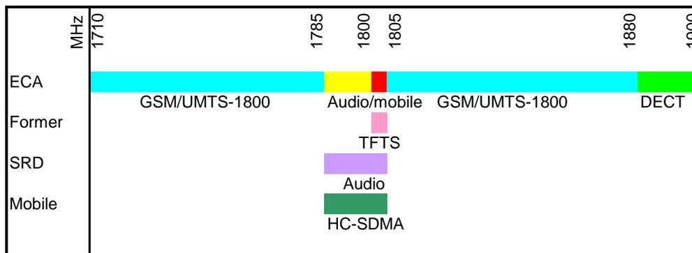
**Figure 3: Frequency usage at the 1800 MHz range relevant for the studies in this Report**
