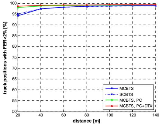
MC-BTS antenna height 30m, k=0.7, tilt 0°
