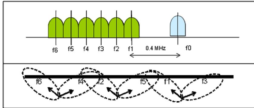
Figure 31: GSM-R frequency re-use
