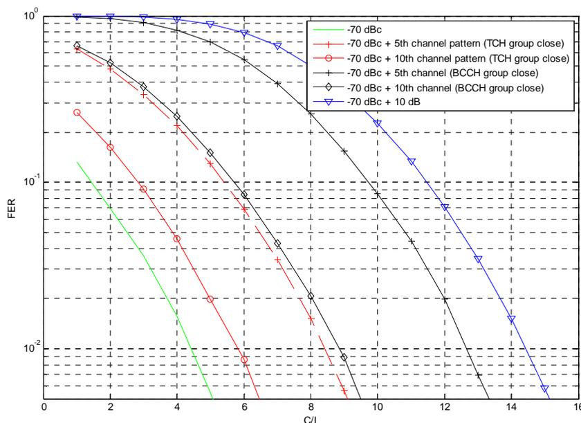
**Figure A3.12: AFS5.90 FER as a function of C/I, comparing the original -70 dBc noise level to noise with IM3 exceptions for MCBTS class 2 at channel nr 5 and 16 in figure 3**
