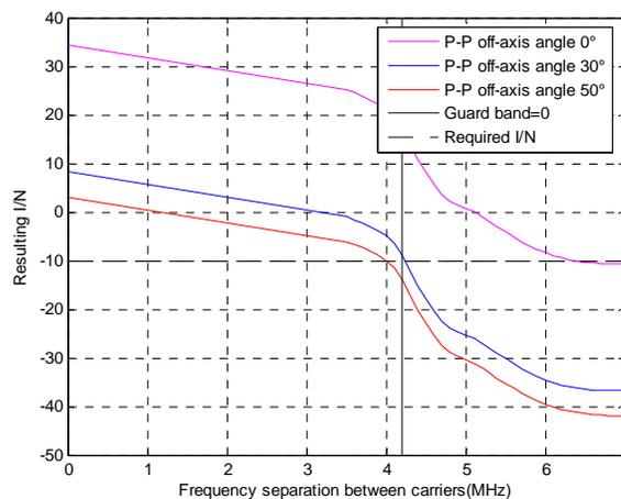
**Figure 5.2.10: Interference from a P-P system (1.4 MHz bandwidth, 1.75 MHz channelling) class 2 on an omnidirectional BWA CS at a 20 km distance**
