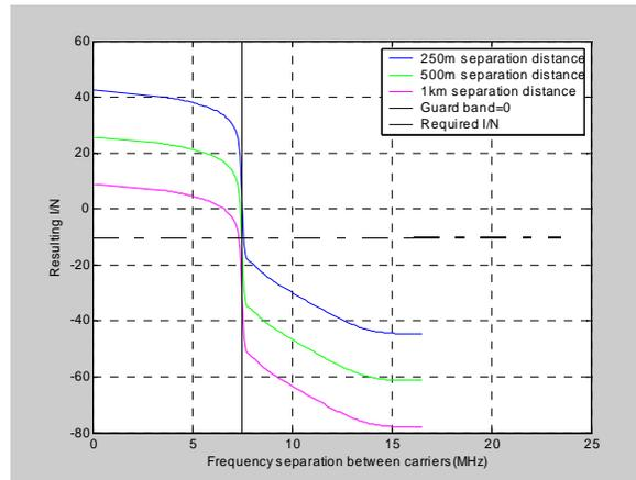
**Figure 5.3.11: Interference from an omni-directional ENG/OB into BWA TS located at distance of 250 m, 500 m and 1 km**
