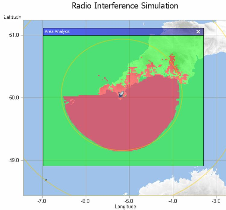
**Fig. 5.4.6(b): Mitigation area around Goonhilly ES for interference from CS-2 (Long Term Propagation; circle 100 km).**
