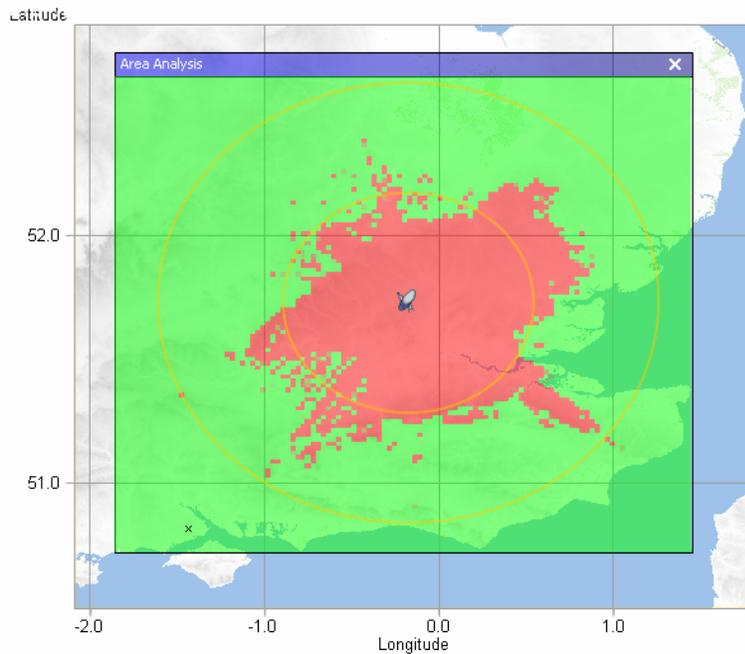
**Fig. 5.4.4(a): Mitigation area around Brookmans Park ES for interference from CS-1 (Long Term Propagation; circles 50 and 100 km)**
