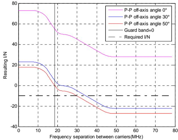
**Figure 5.2.11: Interference from a P-P system (30 MHz bandwidth) class 2 on an omni-directional BWA CS at a 2 km distance**
