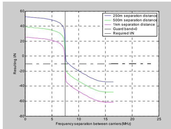
**Figure 5.3.9: Interference from an omni-directional ENG/OB into an omni-directional BWA CS located at distances of 250 m, 500 m and 1 km**
