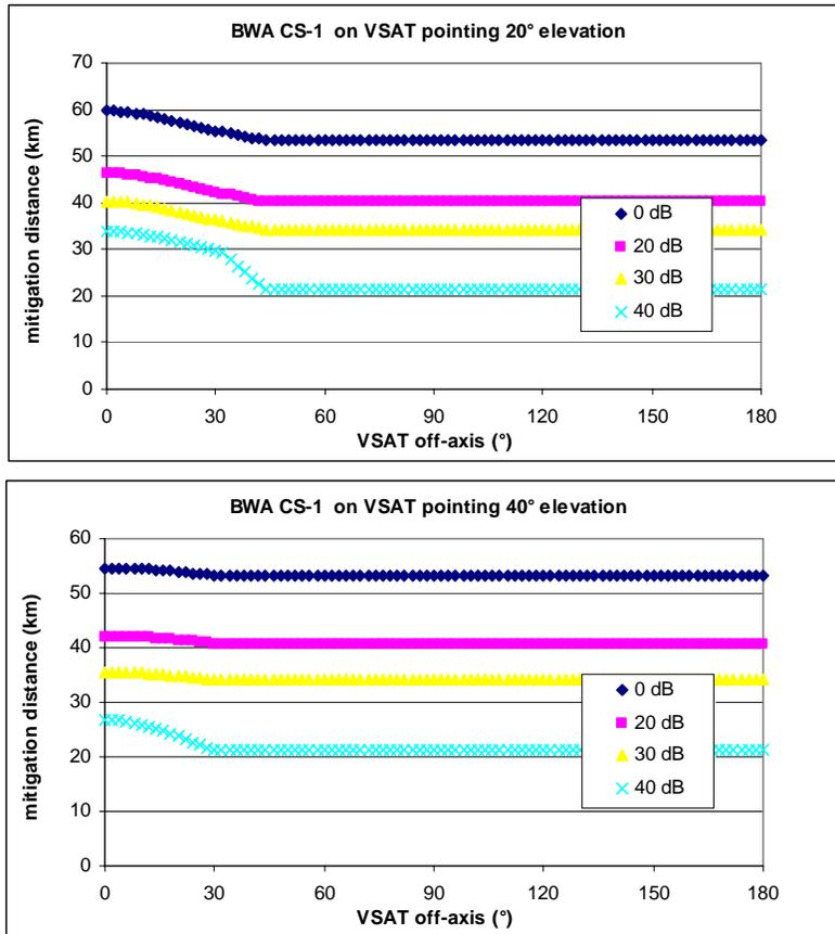
**Figure 5.4.18: Impact from BWA CS1 into VSAT**
