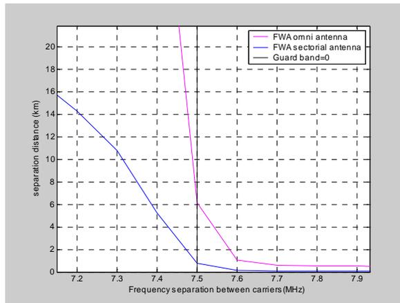
**Figure 5.3.14: Impact from an airborne ENG/OB on an omni-directional and sectorial BWA CS**
