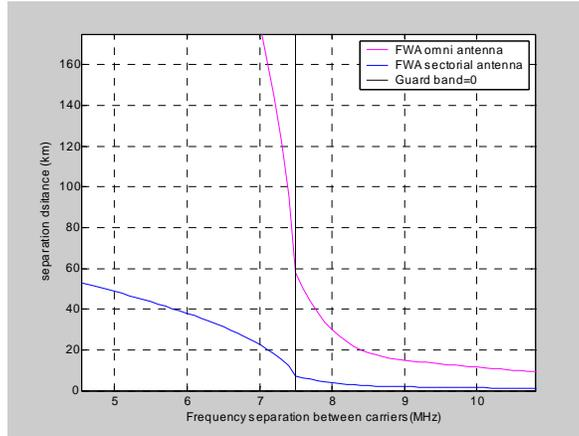
**Figure 5.3.13: Impact from an omni-directional and sectorial BWA CS to an airborne ENG/OB**
