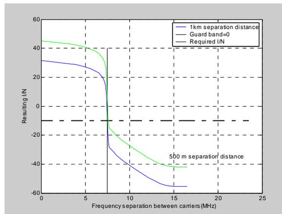
**Figure 5.3.10: Interference from a terrestrial ENG/OB into a sectorial BWA located at distance of 500 m and 1 km**
