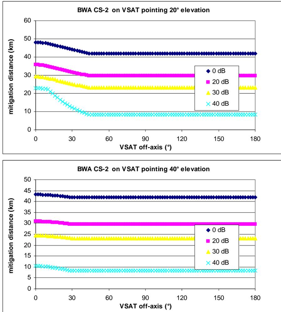
Figure 5.4.19: Impact from BWA CS2 into VSAT
