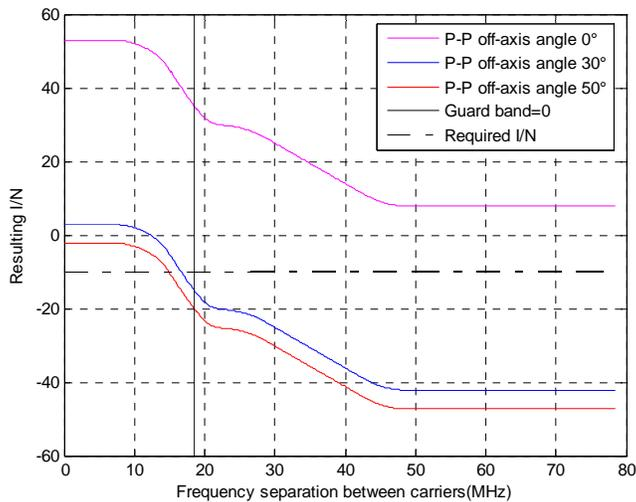
**Figure 5.2.12: Interference from a P-P system (30 MHz bandwidth) class 2 on an omni-directional BWA CS at a 20 km distance**
