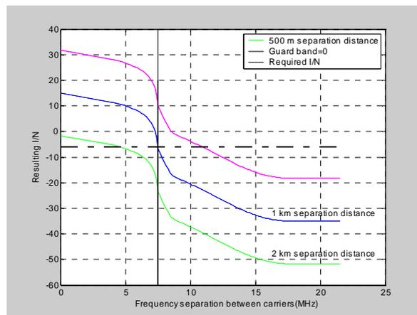
**Figure 5.3.6: Interference from BWA sectorial TS into an omni-directional ENG/OB located at distances of 500 m, 1 km and 2 km**
