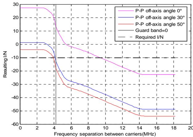
**Figure 5.2.6: Interference from an omni-directional BWA TS on a P-P type 1 (1.4 MHz) with a 18km separation distance**
