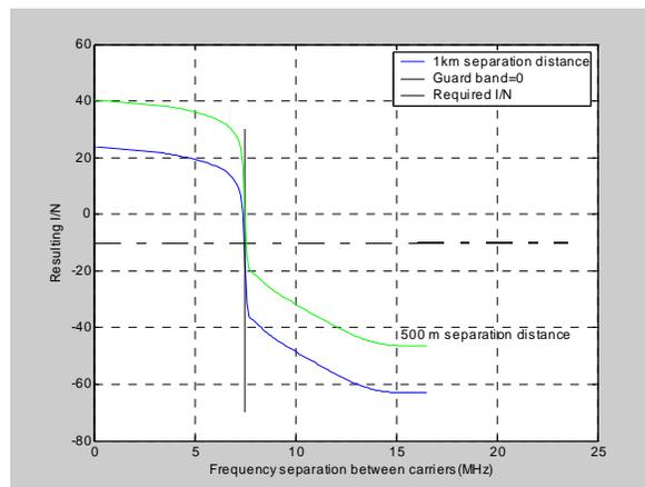
**Figure 5.3.12: Interference from an omni-directional ENG/OB into BWA TS located at distance of 500 m and 1 km**
