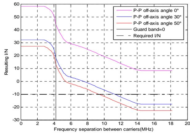
**Figure 5.2.5: Interference from an omni-directional BWA TS on a P-P type 1 (1.4 MHz) with a 500m separation distance**
