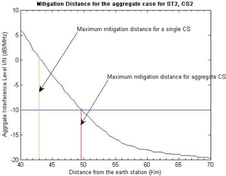
**Figure 5.4.13: Mitigation distance for the aggregate impact from BWA CS2 into FSS ES ST2 – Scenario 1**
