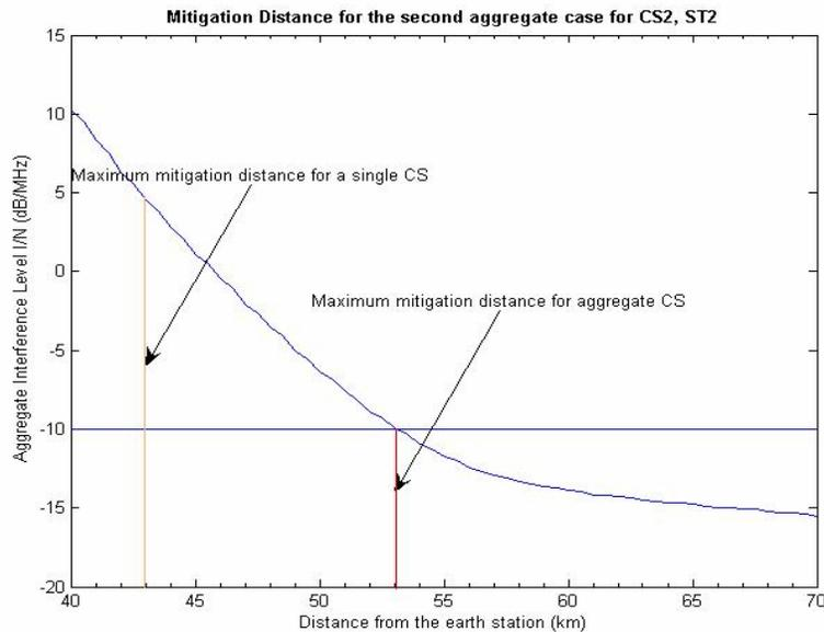
**Figure 5.4.14: Mitigation distance for the aggregate impact from BWA CS2 into FSS ES ST2 – Scenario 2**
