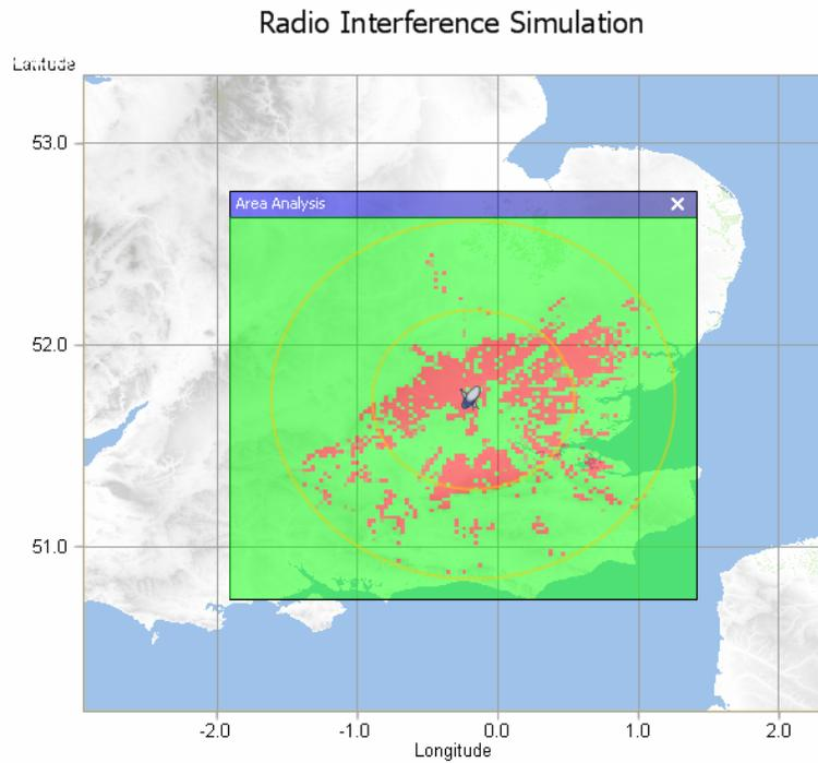
**Figure 5.4.17: Mitigation area around Brookmans Park ES for interference from TS-2 (Short Term Propagation; circles 50 and 100 km)**
