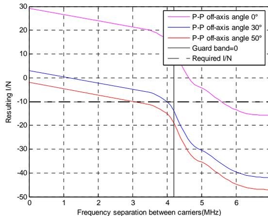
**Figure 5.2.14: Interference from a P-P system (1.4 MHz bandwidth, 1.75 MHz channelling) class 2 on an omni-directional BWA TS at a 18 km distance**
