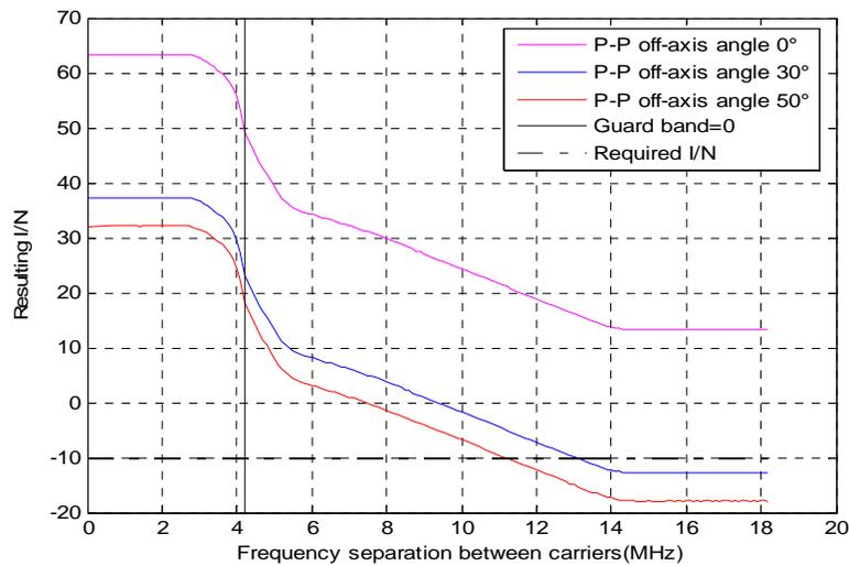
**Figure 5.2.1: Interference from an omni-directional BWA CS on a P-P type 1 (1.4 MHz) with a 2 km separation distance**
