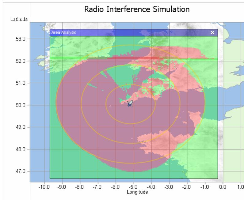
**Fig. 5.4.7(a): Mitigation area around Goonhilly ES for interference from CS-1 (Short Term Propagation; circles 100, 200, 300 km)**
