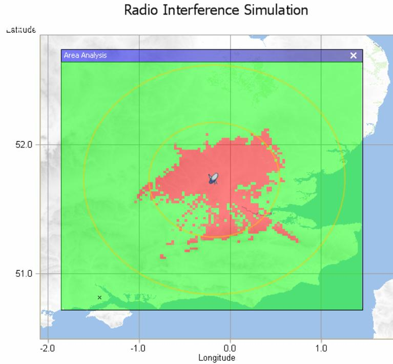
**Fig. 5.4.4 (b): Mitigation area around Brookmans Park ES for interference from CS-2 (Long Term Propagation; circles 50 and 100 km)**
