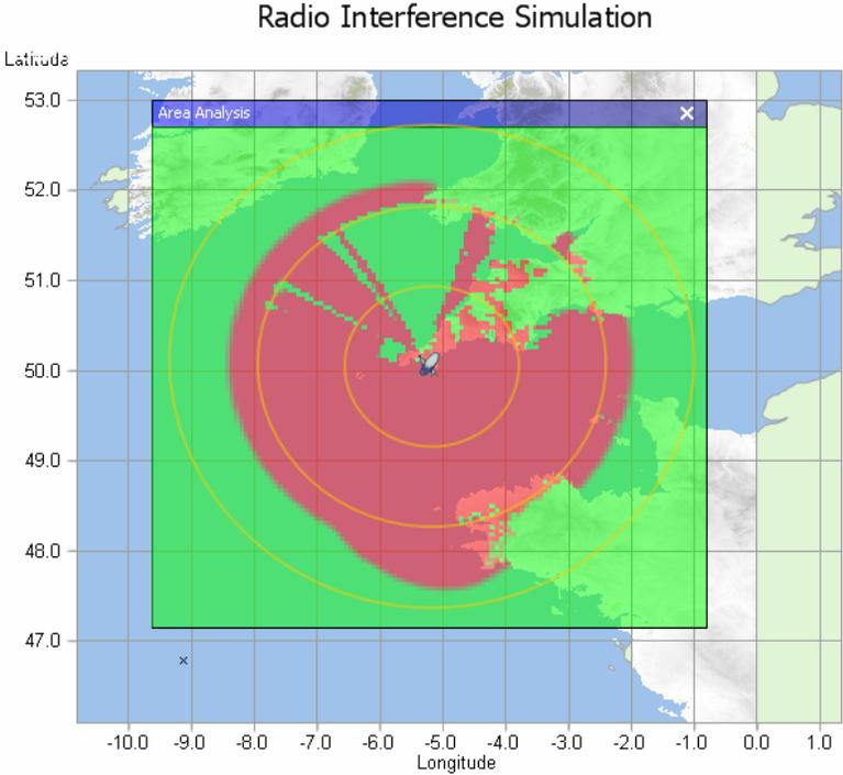
**Fig. 5.4.7(b): Mitigation area around Goonhilly ES for interference from CS-2 (Short Term Propagation; circles 100, 200, 300 km)**
