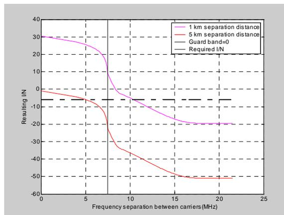
**Figure 5.3.3: Interference from an omni-directional BWA CS into an ENG/OB located at a distances of 1 km and 5 km**
