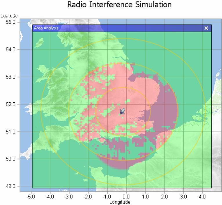
**Fig. 5.4.5(b): Mitigation area around Brookmans Park ES for interference from CS-2 (Short Term Propagation; circles 100, 200 and 300 km)**
