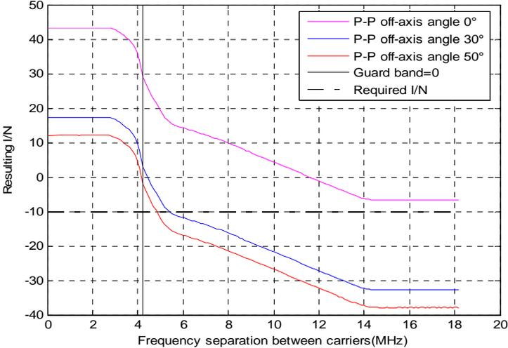
Figure 5.2.2: Interference from an omni-directional BWA CS on a P-P type 1 (1.4 MHz) with a 20 km separation distance
