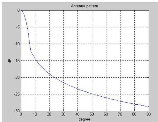
Figure 5.3.1: Diagram of sectorial antenna modelled with Rec. F.1336
