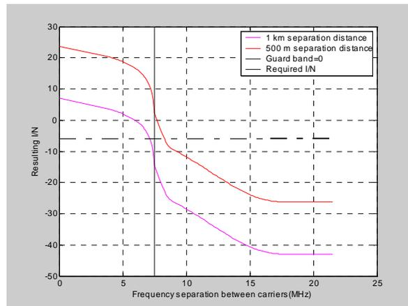
**Figure 5.3.5: Interference from a BWA omni-directional TS into an omni-directional ENG/OB located at distances of 500 m and 1 km**
