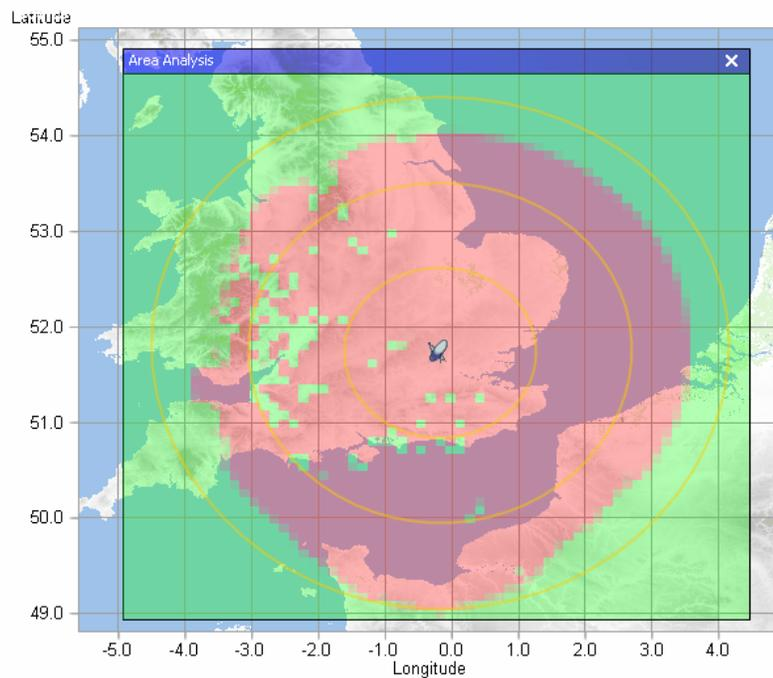
**Fig. 5.4.5(a): Mitigation area around Brookmans Park ES for interference from CS-1 (Short Term Propagation; circles 100, 200 and 300 km)**
