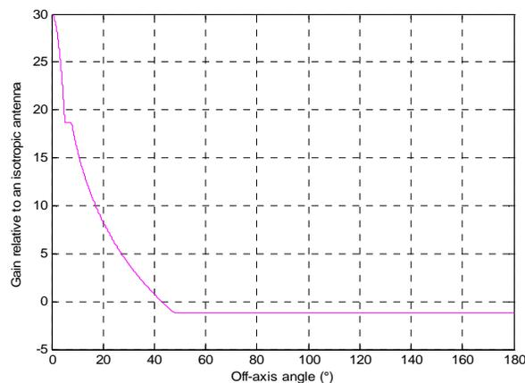
**Figure 4.1: P-P systems antenna diagram with 30 dBi antenna gain modelled with the ITU-R REC F.699-5**
