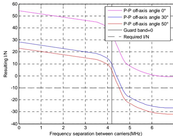
**Figure 5.2.7: Interference from a P-P system (1.4 MHz bandwidth, 1.75 MHz channelling) class 4 on an omni-directional BWA CS at a 2 km distance**
