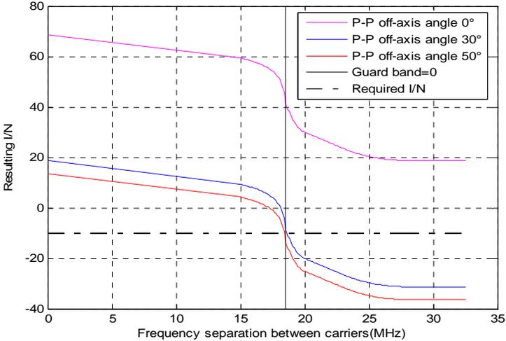
Figure 5.2.3: Interference from an omni-directional BWA CS on a P-P type 2 (30 MHz) with a 2 km separation distance
