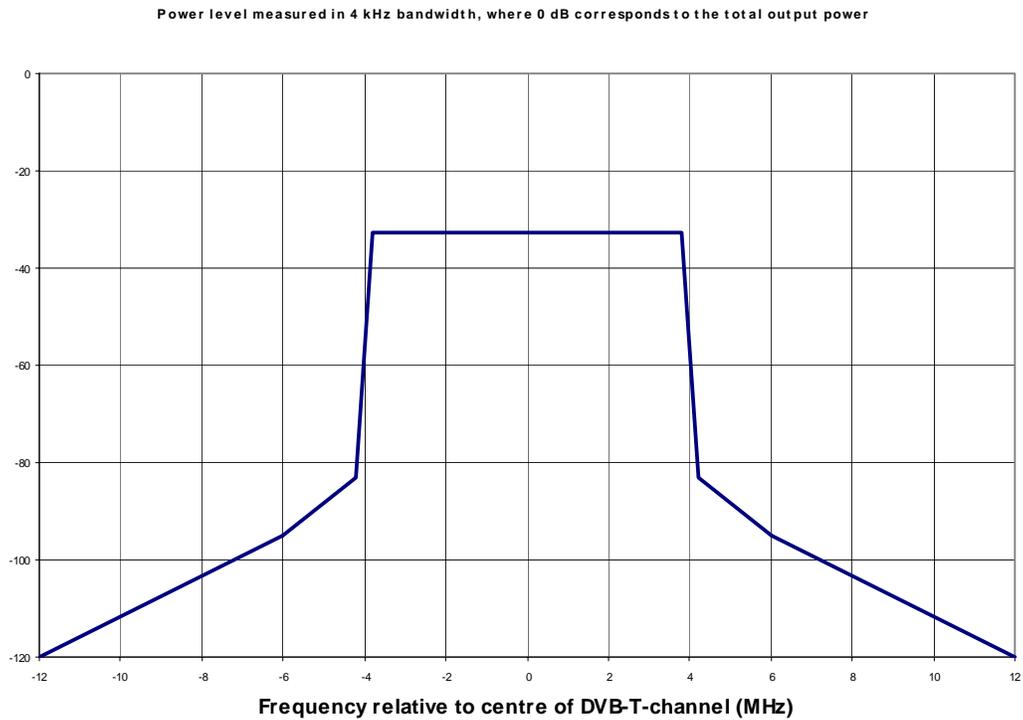
Figure: Spectral mask of a 8 MHz digital ENG/OB based on the DVB-T standard (EN 300 744)
