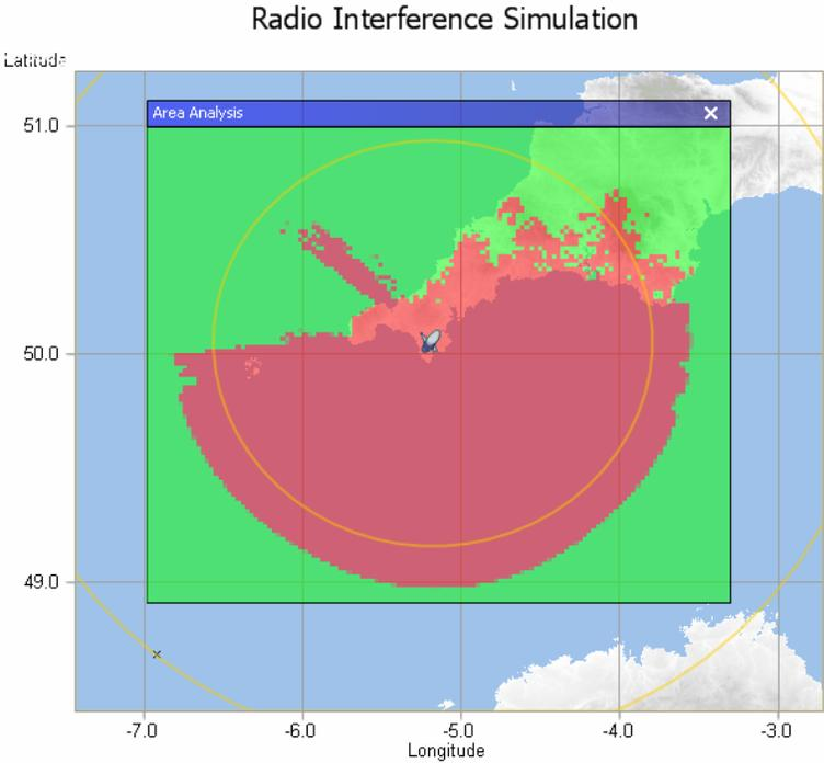
**Fig. 5.4.6(a): Mitigation area around Goonhilly ES for interference from CS-1 (Long Term Propagation; circle 100 km).**
