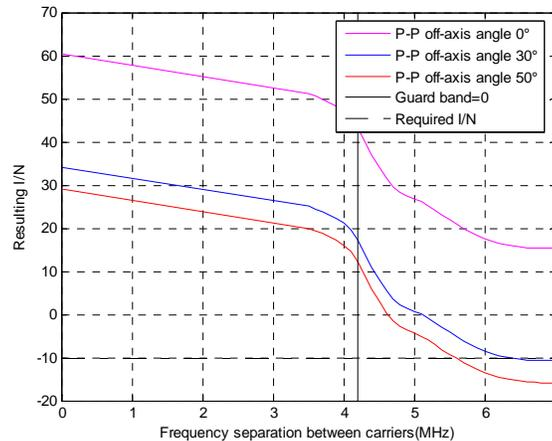
**Figure 5.2.13: Interference from a P-P system (1.4 MHz bandwidth, 1.75 MHz channelling) class 2 on an omni-directional BWA TS at a 500 m distance**
