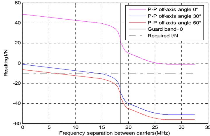
**Figure 5.2.4: Interference from an omni-directional BWA CS on a P-P type 2 (30 MHz) with a 20 km separation distance**
