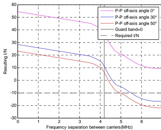
**Figure 5.2.9: Interference from a P-P system (1.4 MHz bandwidth, 1.75 MHz channelling) class 2 on an omnidirectional BWA CS at a 2 km distance**
