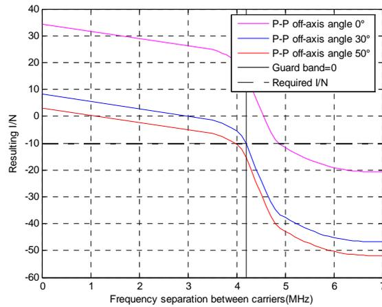
**Figure 5.2.8: Interference from a P-P system (1.4 MHz bandwidth, 1.75 MHz channelling) class 4 on an omnidirectional BWA CS at a 20 km distance**
