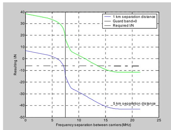
**Figure 5.3.4: Interference from a sectorial BWA CS into an ENG/OB located at distances of 1 km and 5 km**
