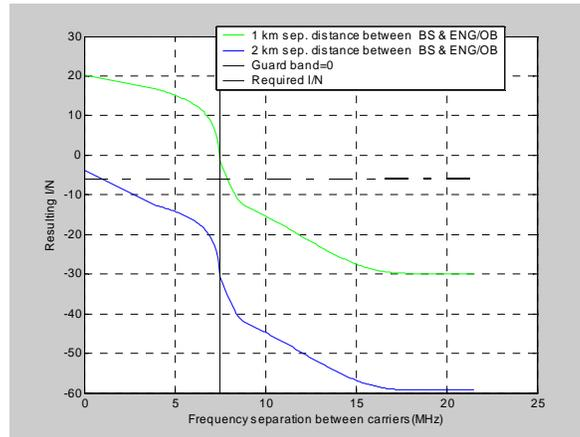
**Figure 5.3.7: Interference from 6 omni-directional BWA TS with 5 dBi gain into ENG/OB**
