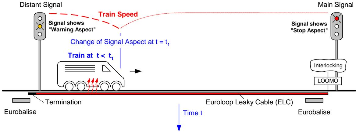
Figure A-4: Train performance along track *with Euroloop infill* function. Top: Situation *before* change of main signal aspect
