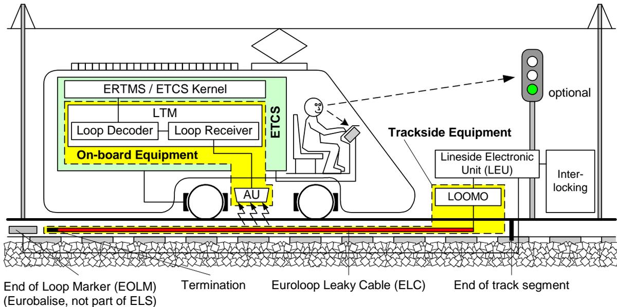
**Figure A-7: Trackside & On-board Equipment of Euroloop Sub-System (ELS)**
