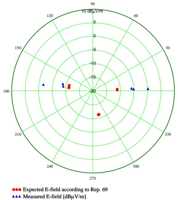
**Figure B-8: Expected field versus measured field at 14.9 MHz**
