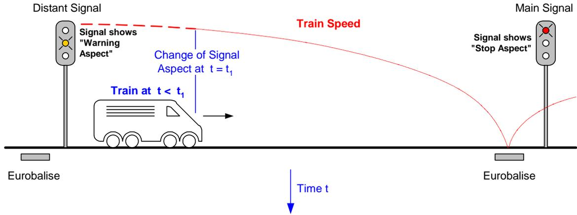
Figure A-2: Train performance along track *without Euroloop infill* function. Situation *before* change of main signal aspect
