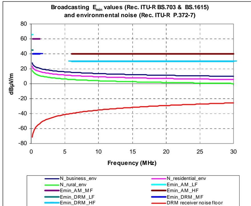
Figure E-1: AM and DRM minimum field strengths to be protected and environmental noise
