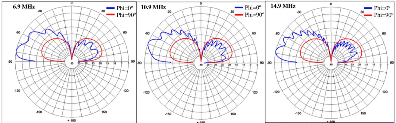
Figure C-2: Vertical diagrams at 6.9, 10.9 and 14.9 MHz  $\Phi = 0^\circ$  (blue)  $\Phi = 90^\circ$  (red)
