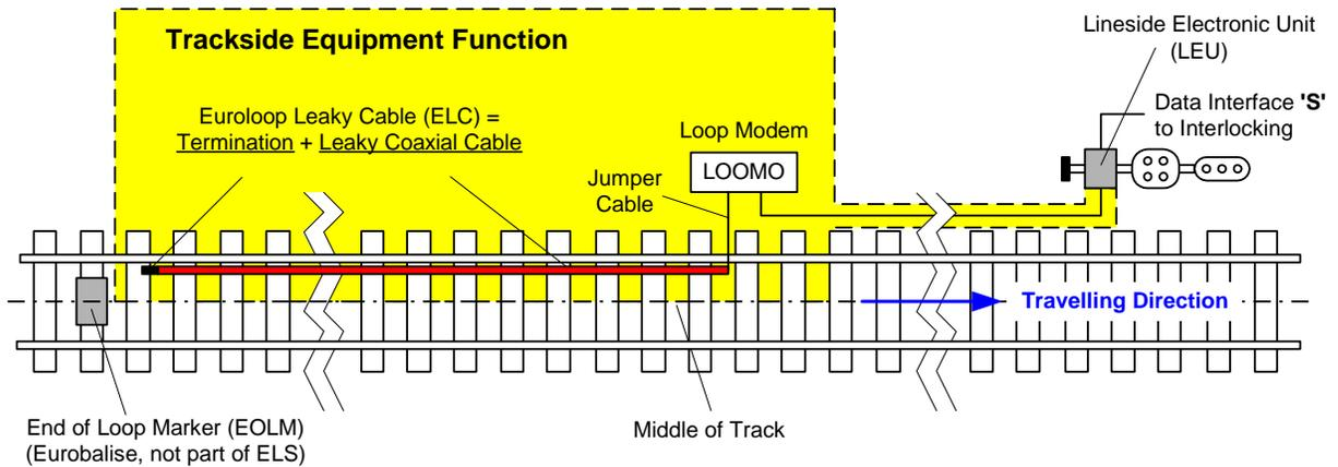
**Figure A-6: Typical Installation of Euroloop Trackside Equipment**
