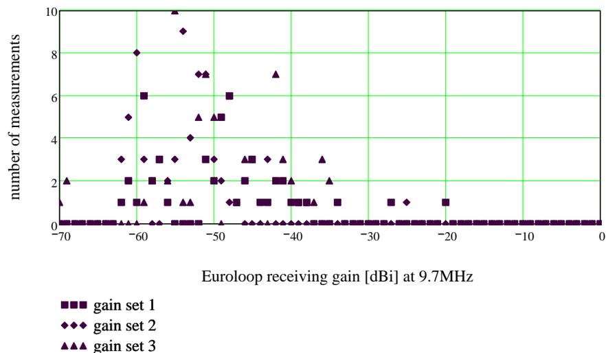
Figure B-3: Euroloop receiving gain histogram 9.2 – 10.2 MHz
