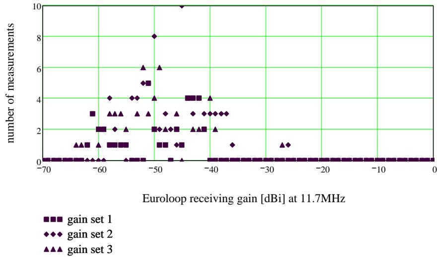
**Figure B-4: Euroloop receiving gain histogram 11.2 – 12.2 MHz**
