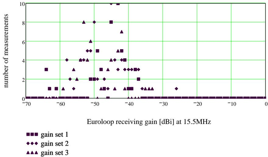
**Figure B-5: Euroloop receiving gain histogram 15 – 16 MHz**
