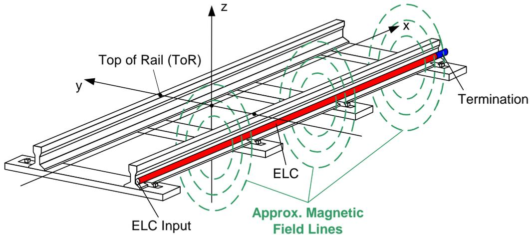
**Figure A-8: ELC Mounted on Outer Side of Rail's web with Indication of Magnetic Field Lines**
