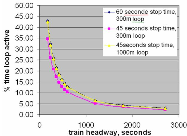
**Figure A-11: Loop Occupancy versus Train Headway for Different Station Stop Times**
