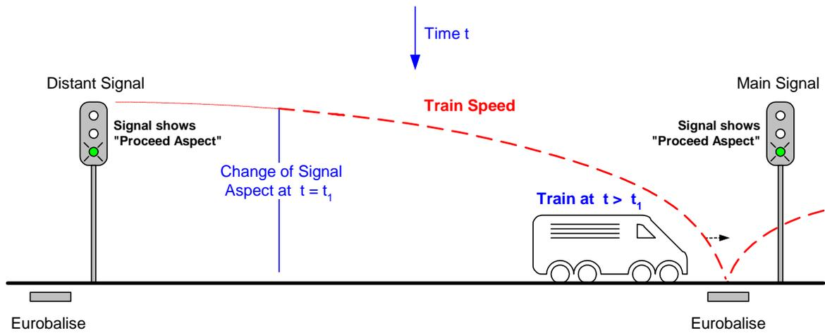
Figure A-3: Train performance along track *without Euroloop infill* function. Situation *after* change of main signal aspect
