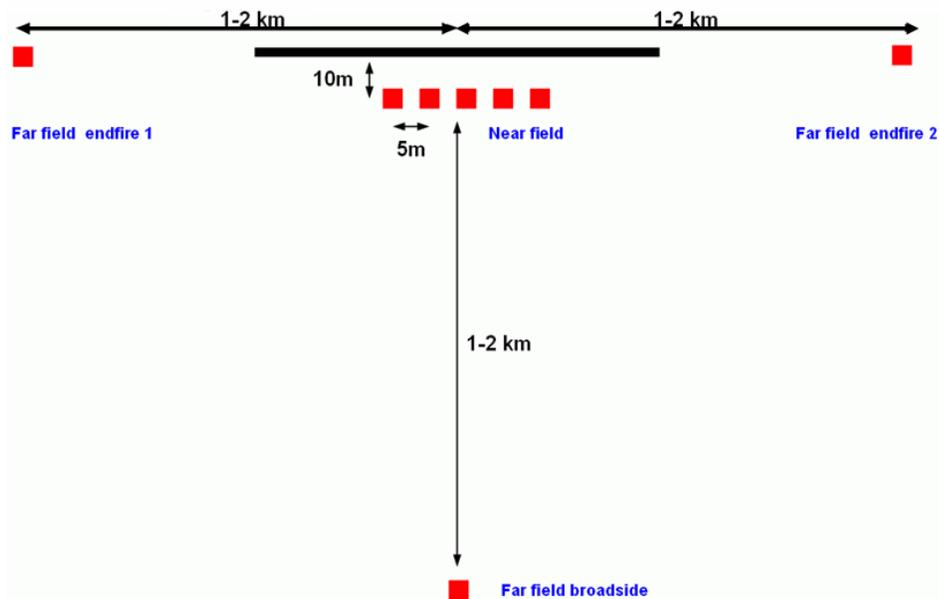
Figure B-1: Topology of Euroloop far field measurements
