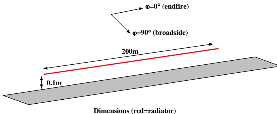
Figure C-1: Model for the Euroloop antenna
