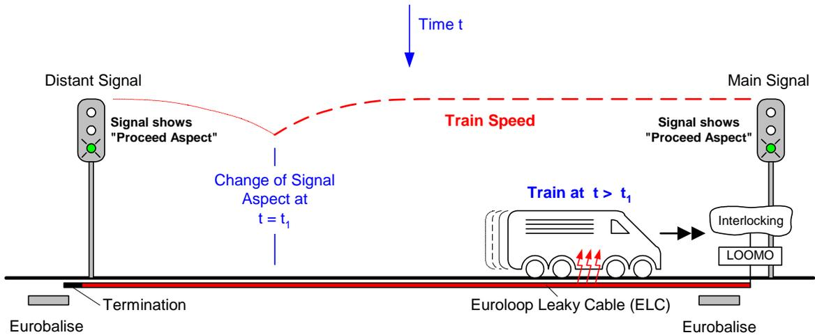
Figure A-5: Train performance along track *with Euroloop infill* function. Top: Situation *after* change of main signal aspect
