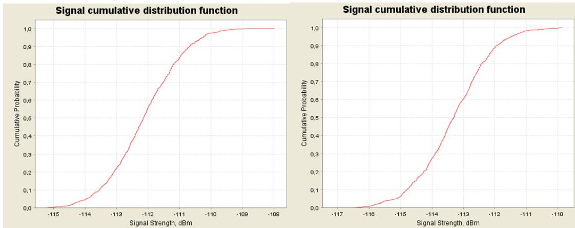
**Figure 35: CDF graphs for the ac-MS for 1800 MHz at 8000 m (left) and 10000 m (right) above ground**
