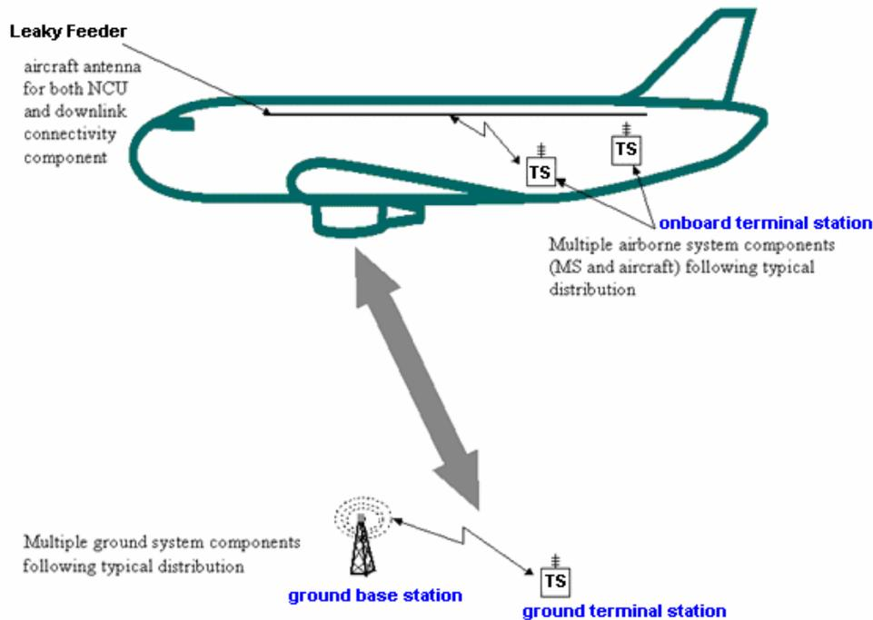
**Figure 4: GSMOB and terrestrial cellular system interference scenario**
