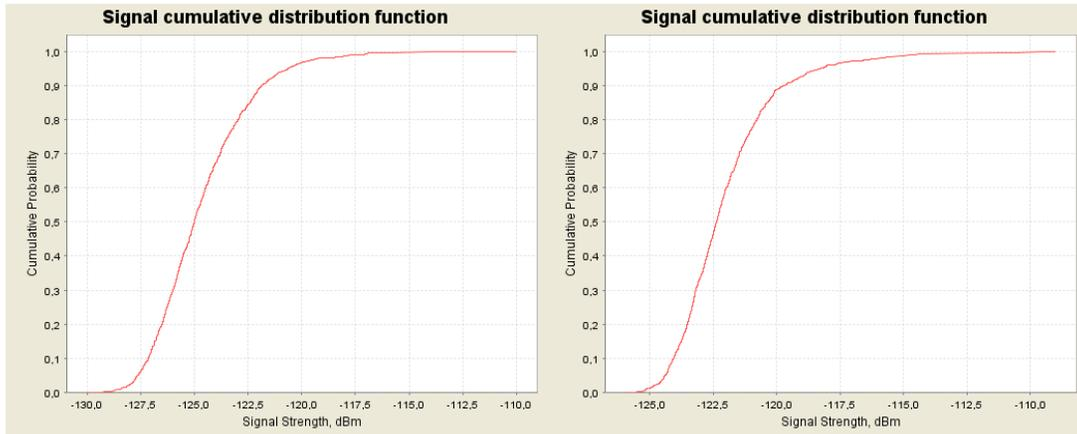
**Figure 59: CDF graphs for the multiple NCU (GSM) for 1800 MHz for normal busy (left) and extreme busy (right) cases**
