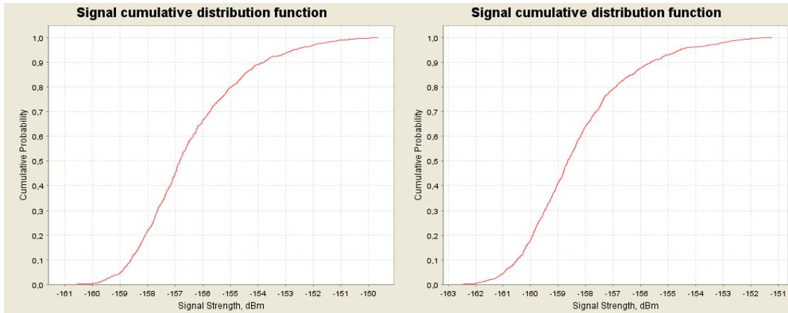
Figure 69: CDF graphs for the ac-MS for 1800 MHz at 8000 m (left) and 10000 m (right) above ground
