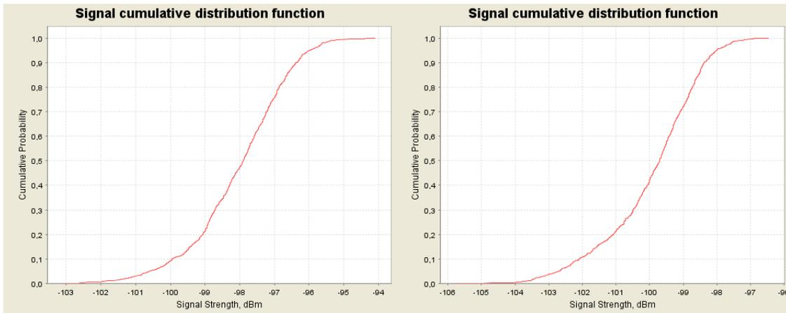
Figure 33: CDF graphs for the ac-MS for 900 MHz at 8000 m (left) and 10000 m (right) above ground
