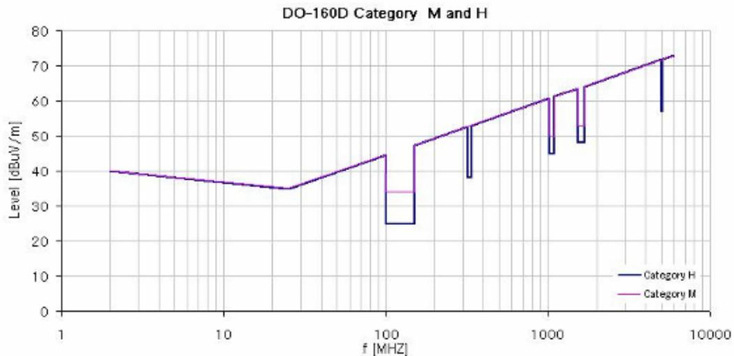
**92: Limit line for emission of radio frequency energy according to category M and H**
