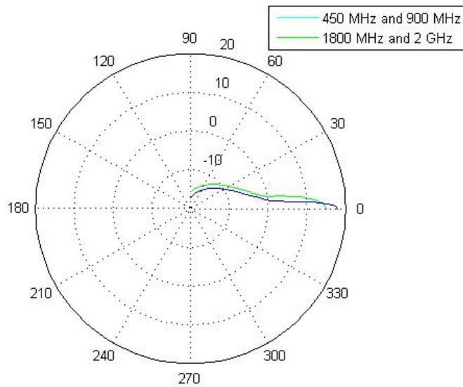
**Figure 105: Elevation patterns used for the SEAMCAT simulations**
