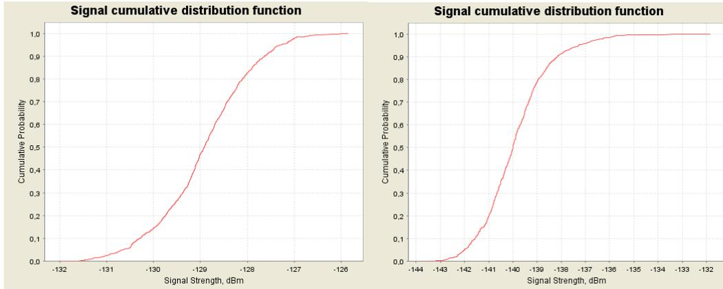
Figure 66: CDF graphs for the ac-MS for 1800 MHz at 3000 m (left) and 5000 m (right) above ground
