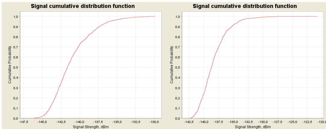
**Figure 64: CDF graphs for the multiple ac-BTS for 1800 MHz for normal busy (left) and extreme busy (right) cases for 50 GSM 1800 channels onboard**
