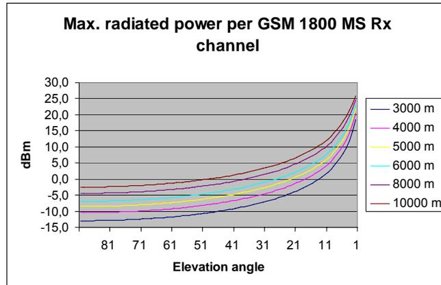
Figure 12: Maximum radiated power in GSM MS receive channels from different heights
