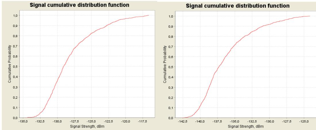
Figure 42: CDF graphs for the ac-BTS for 1800 MHz at 3000 m (left) and 5000 m (right) above ground
