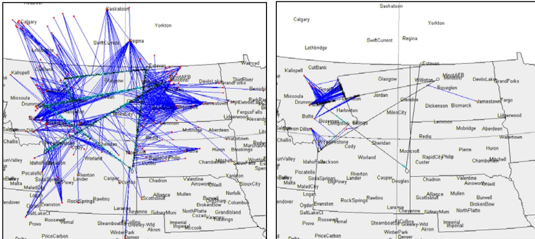
**Figure 112: Maps of terrestrial system acquisition during flight. Left: Unmodified aircraft; Right: RF shielded aircraft**
