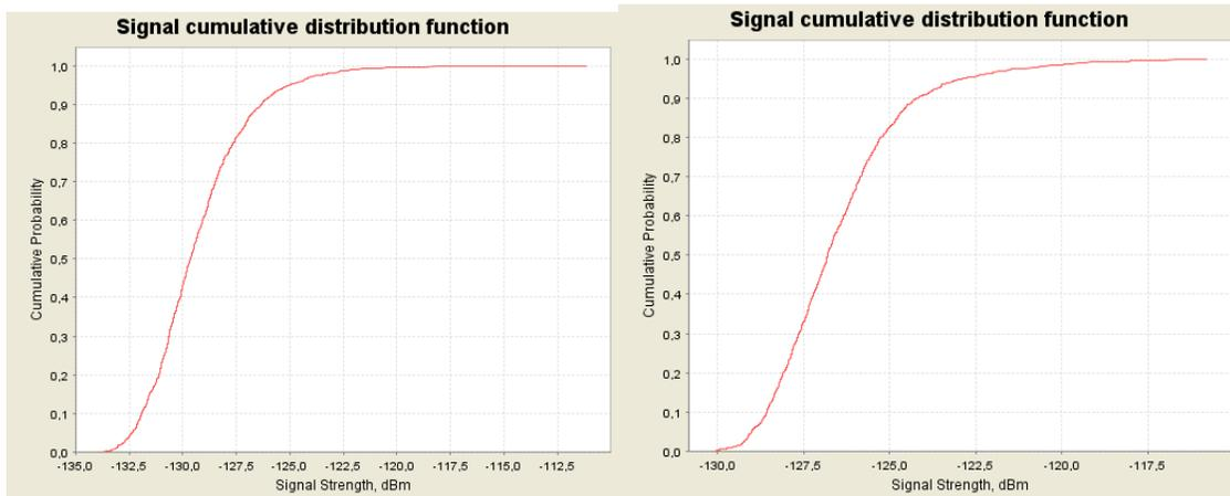
**Figure 56: CDF graphs for the multiple NCU (GSM) for 900 MHz for normal busy (left) and extreme busy (right) cases**
