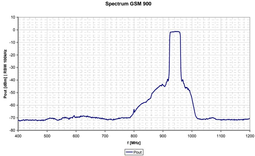
**Figure 95: GSM 900 output spectrum wideband**
