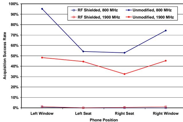
**Figure 113: Acquisition Statistics @ 9,000 m Altitude**
