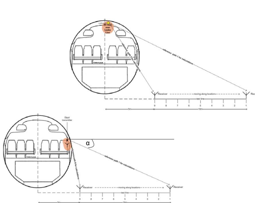
**Figure 89: Principle setup aircraft attenuation test**
