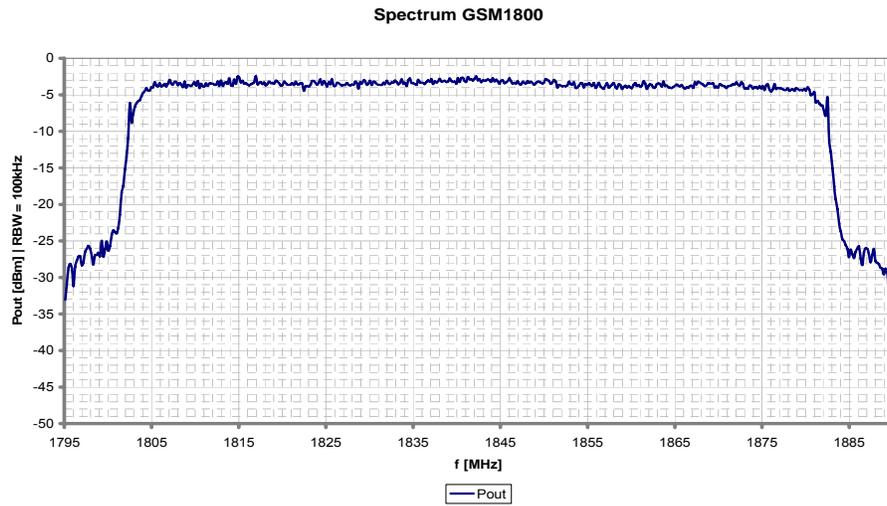
**Figure 96: GSM 1800 output spectrum narrow band**
