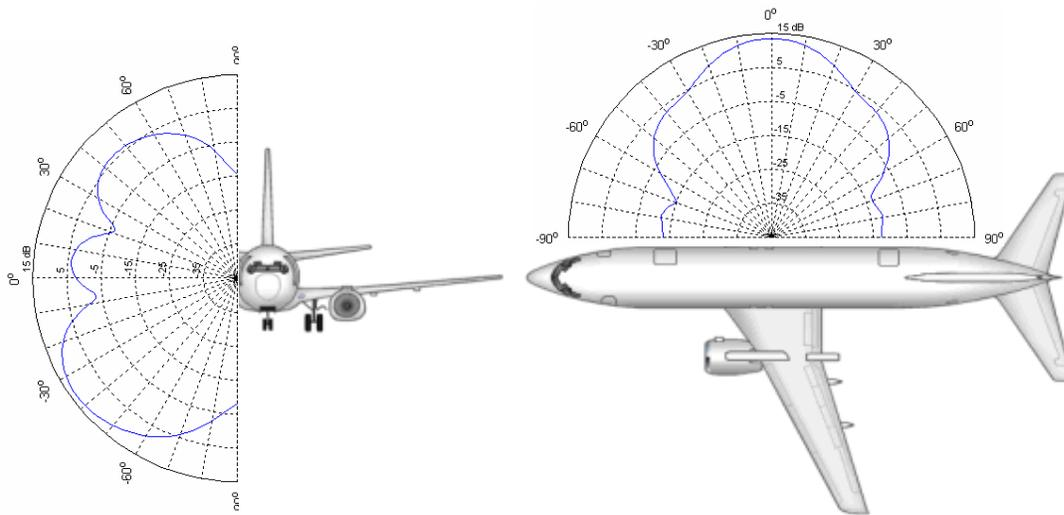
**Figure 77: Elevation and azimuth patterns for a single aircraft window coherently illuminated by an isotropic source**
