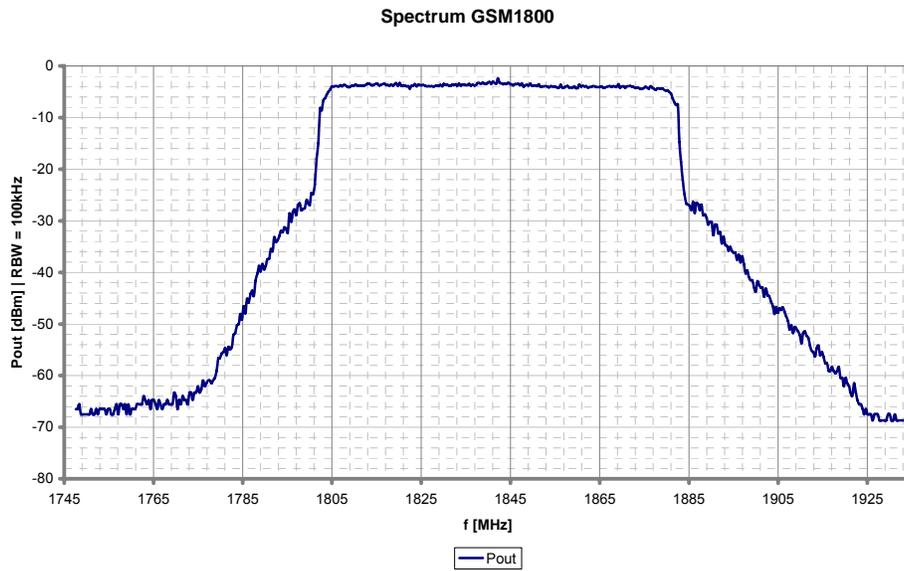
**Figure 97: GSM 1800 output spectrum**
