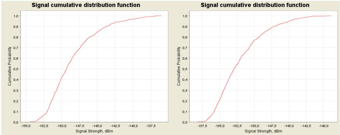
Figure 37: CDF graphs for the NCU (GSM) for 900 MHz at 8000 m (left) and 10000 m (right) above ground
