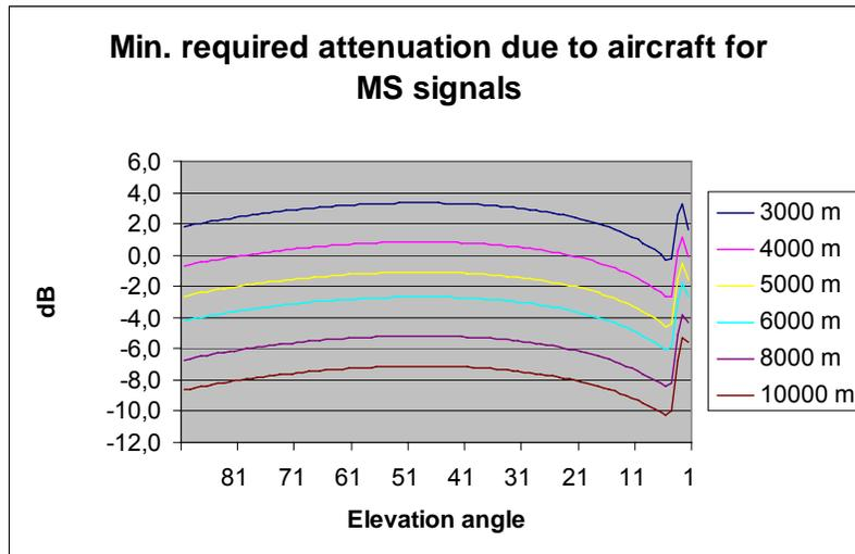
Figure 14: Attenuation requirements for signals to/from ac-MS
