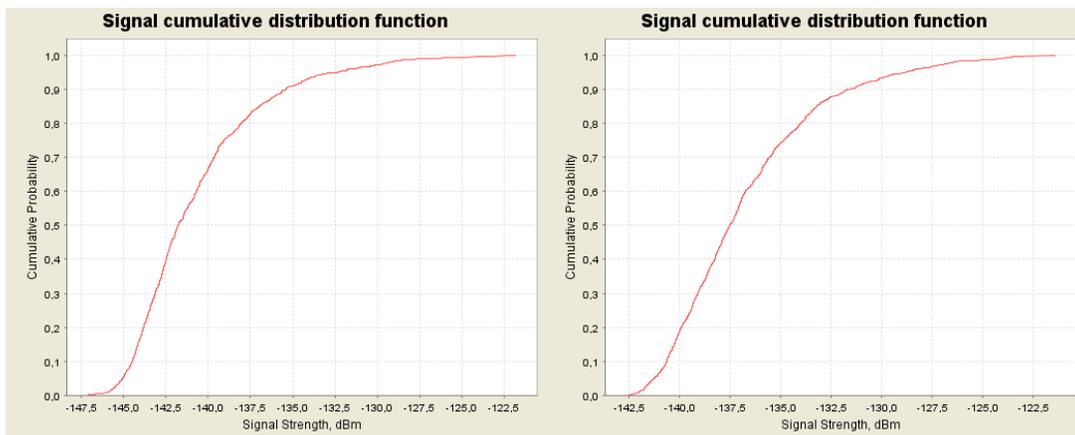
**Figure 55: CDF graphs for the multiple ac-BTS for 1800 MHz for 50 GSM 1800 channels onboard for the normal busy (left) and the extreme busy (right) cases**
