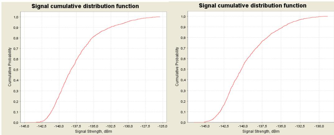
Figure 49: CDF graphs for the NCU (UMTS) for 900 MHz at 8000 m (left) and 10 000 m (right) above ground
