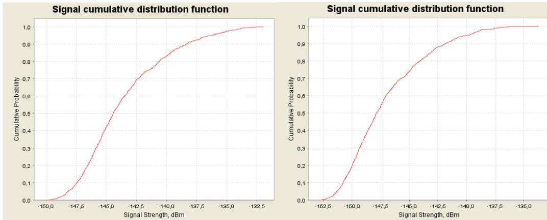
Figure 43: CDF graphs for the ac-BTS for 1800 MHz at 8000 m (left) and 10000 m (right) above ground
