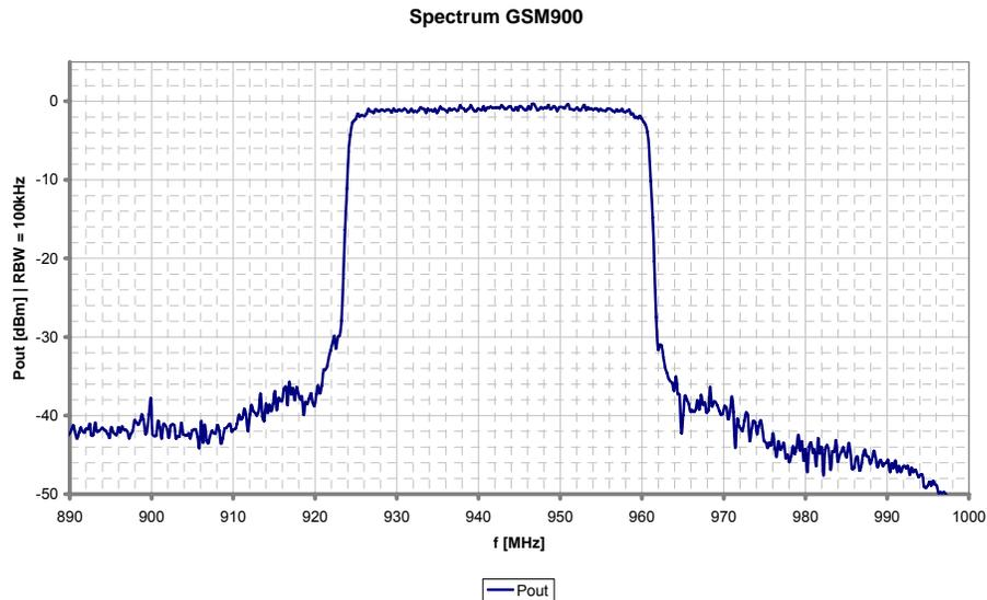
**Figure 94:GSM 900 output spectrum**
