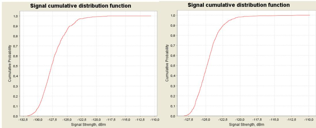
**Figure 62: CDF graphs for the multiple NCU (UMTS) for 2000 MHz for normal busy (left) and extreme busy (right) cases**
