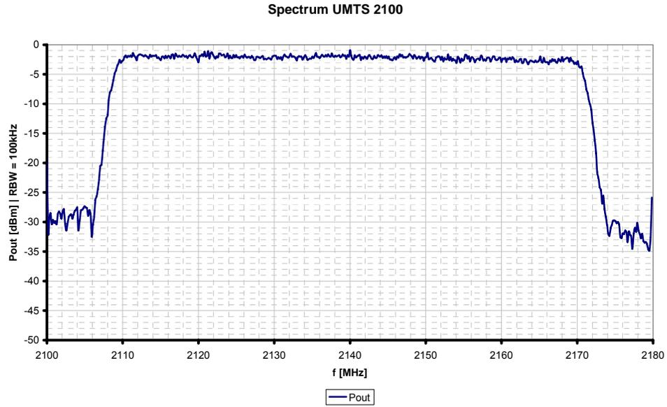
**Figure 99: UMTS output spectrum narrow band**
