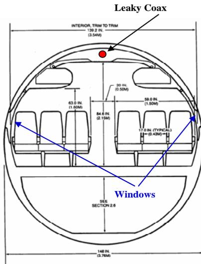
**Figure 74: Detail showing a typical leaky cable installation in a narrow body aircraft**
