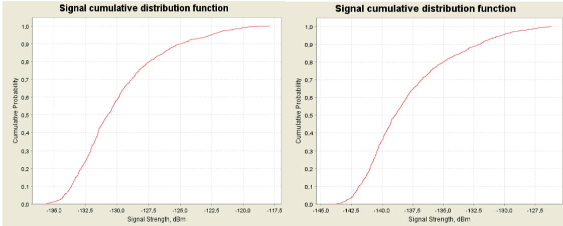
Figure 40: CDF graphs for the NCU (UMTS) for 2000 MHz at 3000 m (left) and 5000 m (right) above ground
