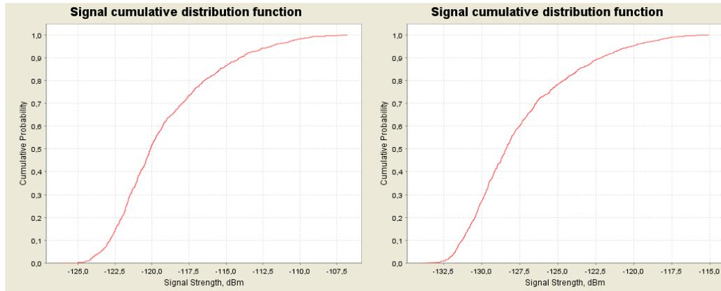
Figure 44: CDF graphs for the NCU (GSM) for 900 MHz at 3000 m (left) and 5000 m (right) above ground
