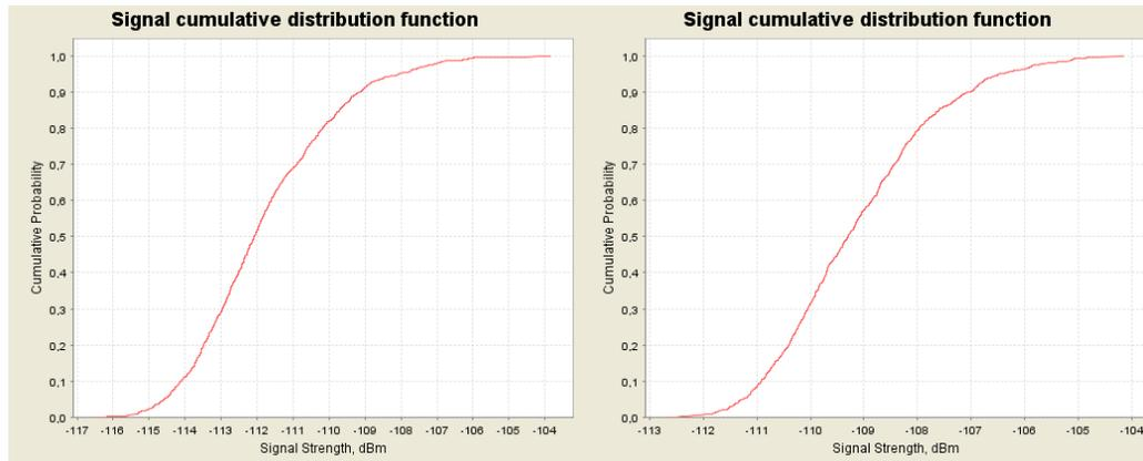
**Figure 65: CDF graphs for the multiple NCU (CDMA) for 450 MHz for normal busy (left) and extreme busy (right) cases**
