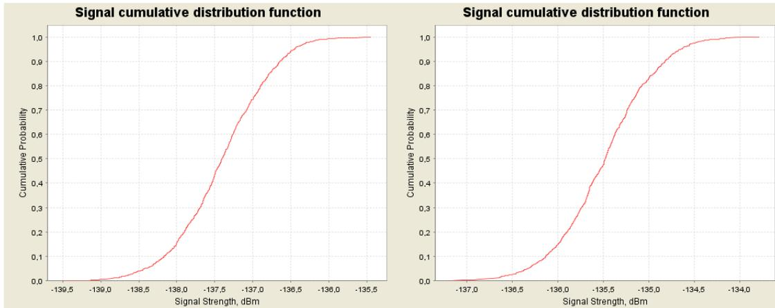
**Figure 73: CDF graphs for the multiple ac-MS for 1800 MHz for normal busy (left) and extreme busy (right) cases for 50 GSM 1800 channels onboard**
