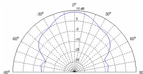
**Figure 79: Aircraft azimuth gain pattern for the 100% random array model. Azimuth slice is shown for peak gain elevation angle of 37.2° below horizontal**
