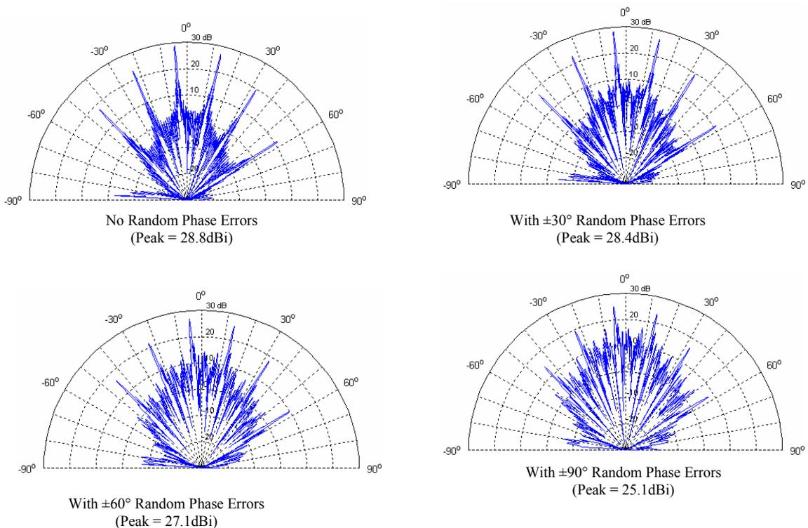
**Figure 80: Azimuth plots of aircraft aperture and array gain for varying amounts of phase noise. Azimuth slices are at the elevation angle of maximum gain,  $37.2^\circ$  below horizontal**
