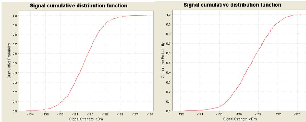
**Figure 70: CDF graphs for the multiple ac-MS for 1800 MHz for 10 GSM 1800 channels onboard for the normal busy day (left) and the extreme busy day (right) cases**
