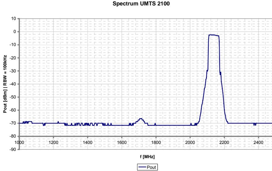
Figure 101: UMTS output spectrum wide band
