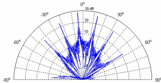
**Figure 78: Aircraft azimuth aperture and array gain pattern for the 100% coherent array model. Azimuth slice is shown for peak gain elevation angle of 37.2° below horizontal**
