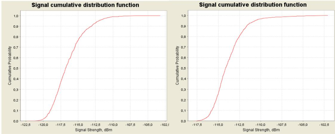
**Figure 58: CDF graphs for the multiple NCU (GSM) for 900 MHz for normal busy (left) and extreme busy (right) cases**
