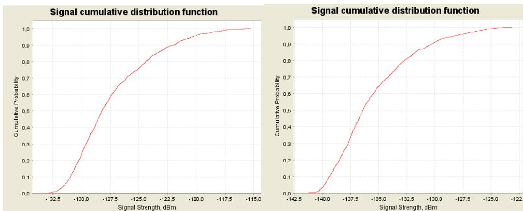
**Figure 46: CDF graphs for the NCU (GSM) for 1800 MHz at 3000 m (left) and 5000 m (right) above ground**
