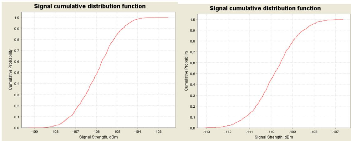
**Figure 34: CDF graphs for the ac-MS for 1800 MHz at 3000 m (left) and 5000 m (right) above ground**
