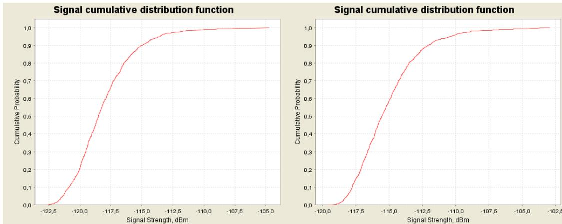
**Figure 60: CDF graphs for the multiple NCU (UMTS) for 900 MHz for normal busy (left) and extreme busy (right) cases**
