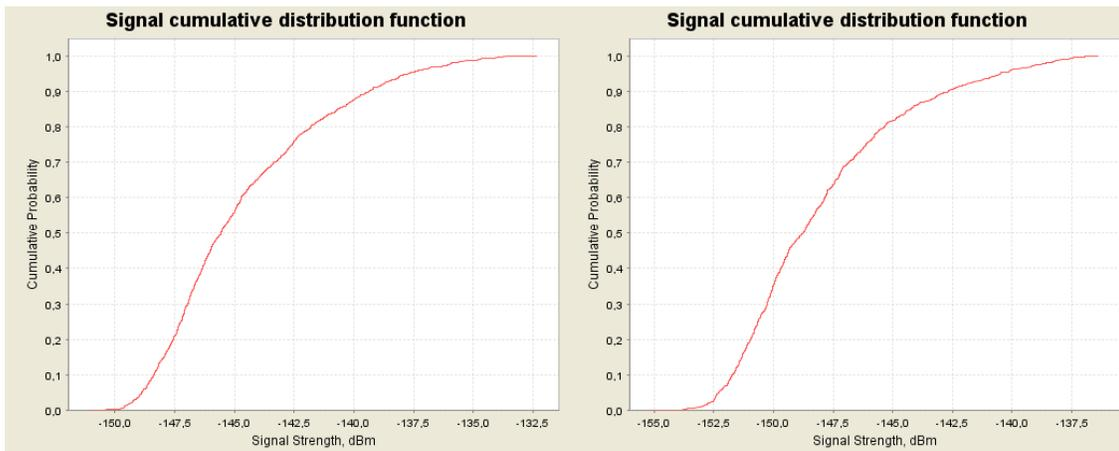
Figure 51: CDF graphs for the NCU (UMTS) for 1800 MHz at 8000 m (left) and 10000 m (right) above ground
