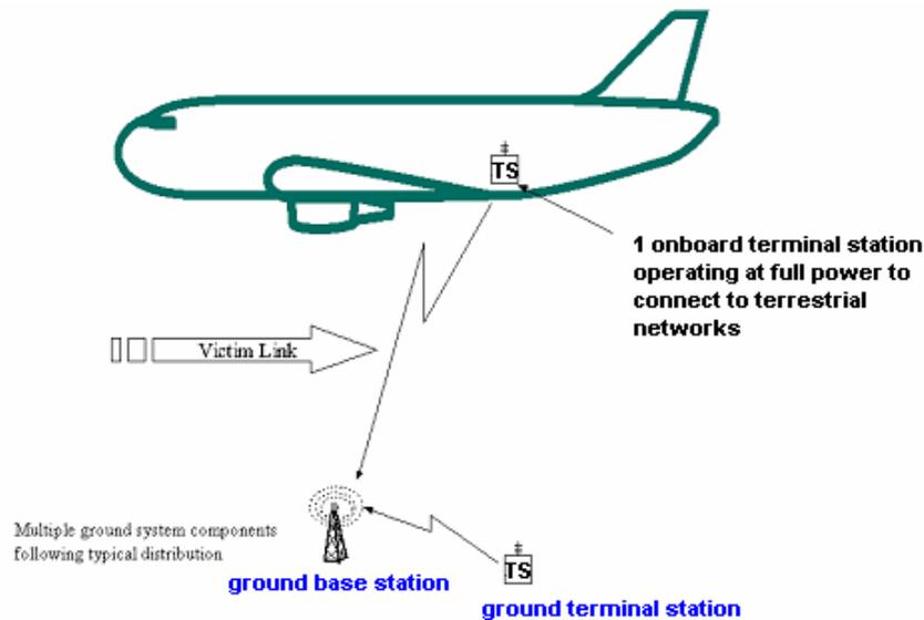
**Figure 7: Scenario 2 where ac-MS/UE signal is received by g-BTS/NodeB (no NCU)**
