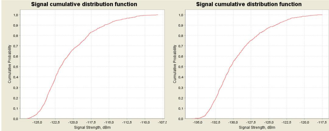
Figure 48: CDF graphs for the NCU (UMTS) for 900 MHz at 3000 m (left) and 5000 m (right) above ground
