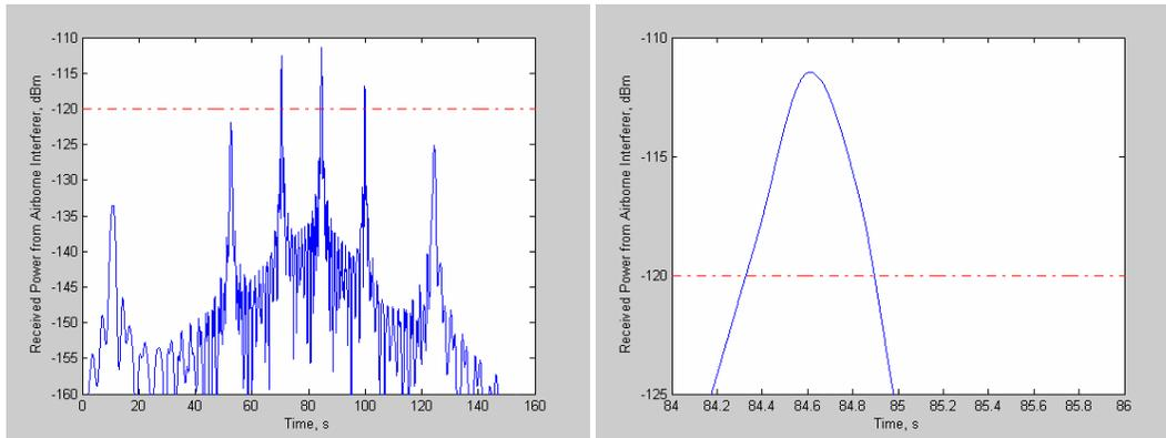
**Figure 83: Time history of interference power received by g-MS. 100% coherent array model. Dotted line denotes the  $(I/N = -6 \text{ dB})$  interference threshold for a GSM mobile. Plot on right is close-up view of the main gain peak**
