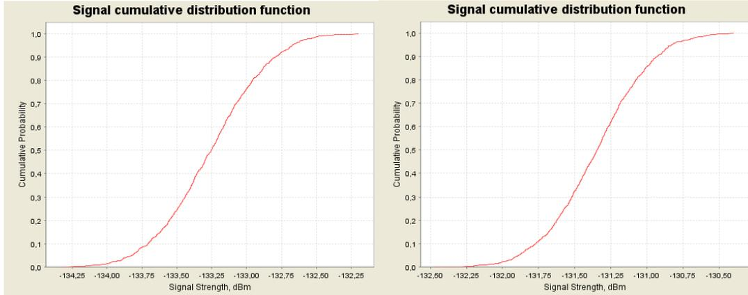
**Figure 72: CDF graphs for the multiple ac-MS for 1800 MHz for normal busy (left) and extreme busy (right) cases for 10 GSM 1800 channels onboard**
