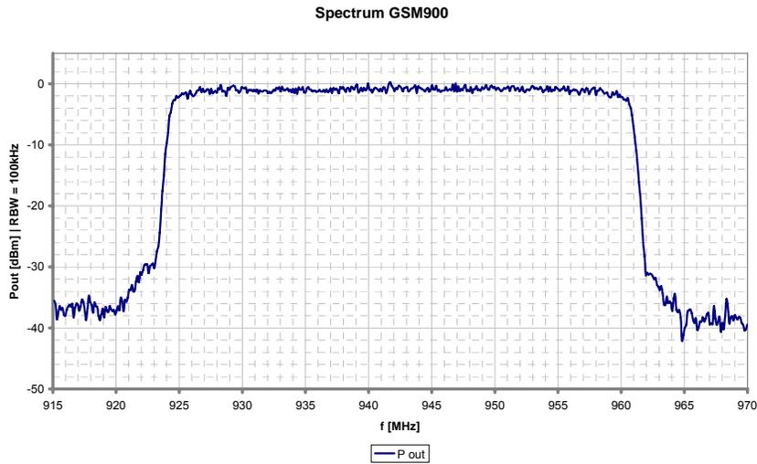
**Figure 93:GSM 900 output spectrum narrow band**
