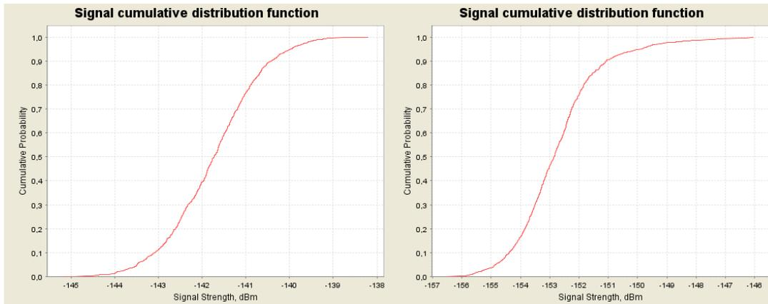
Figure 68: CDF graphs for the ac-MS for 1800 MHz at 3000 m (left) and 5000 m (right) above ground
