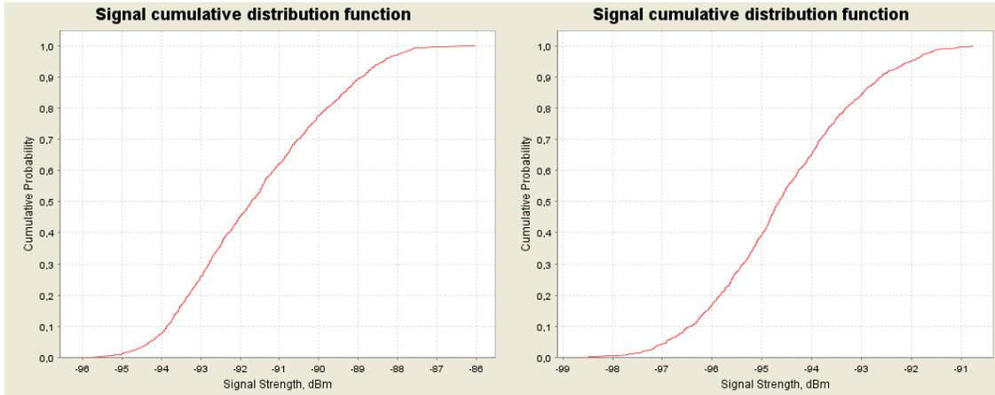
Figure 32: CDF graphs for the ac-MS for 900 MHz at 3000 m (left) and 5000 m (right) above ground
