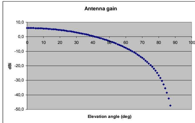
**Figure G-1 Typical vertical diagram for a 6 dBi patch antenna**
