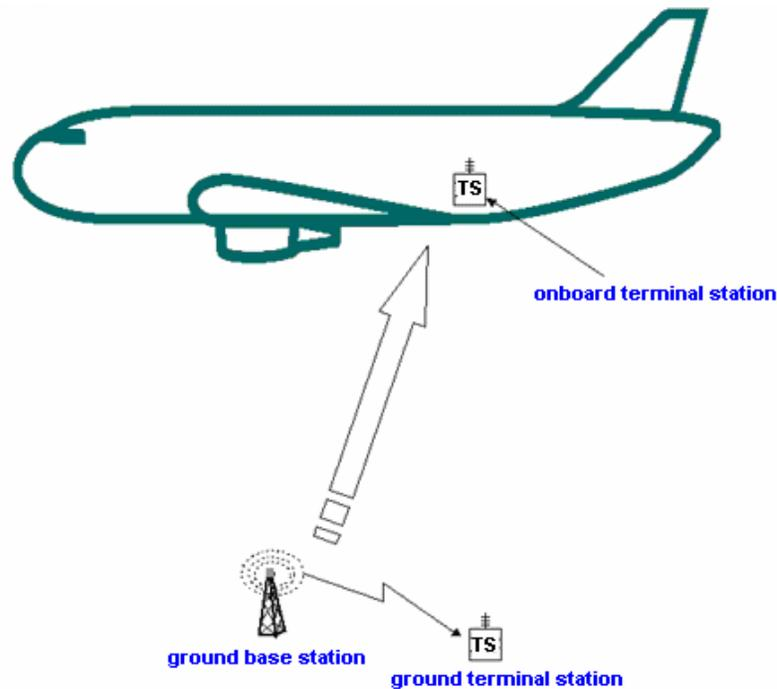
Figure 6: Scenario 1 where g-BTS signal is received by onboard mobile terminals
