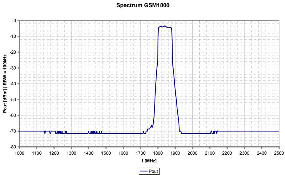
**Figure 98: GSM 1800 output spectrum wideband**
