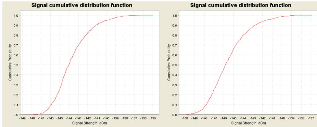
Figure 67: CDF graphs for the ac-MS for 1800 MHz at 8000 m (left) and 10000 m (right) above ground
