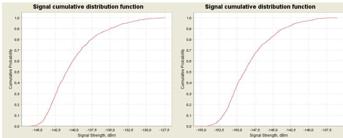
**Figure 38: CDF graphs for the NCU (GSM) for 1800 MHz at 3000 m (left) and 5000 m (right) above ground**
