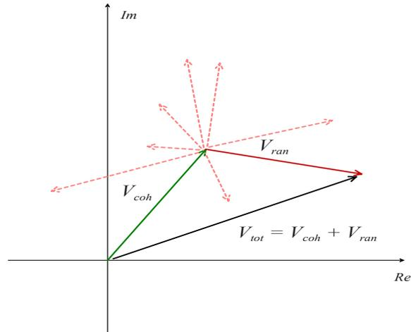
**Figure 81 Complex addition of the coherent and random field components. The dashed vectors indicate that the random component can take any direction and length**
