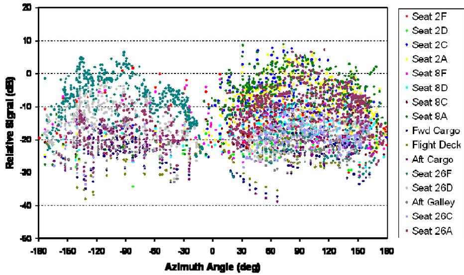
Figure 108: Unmodified aircraft received signals normalized to theoretical values
