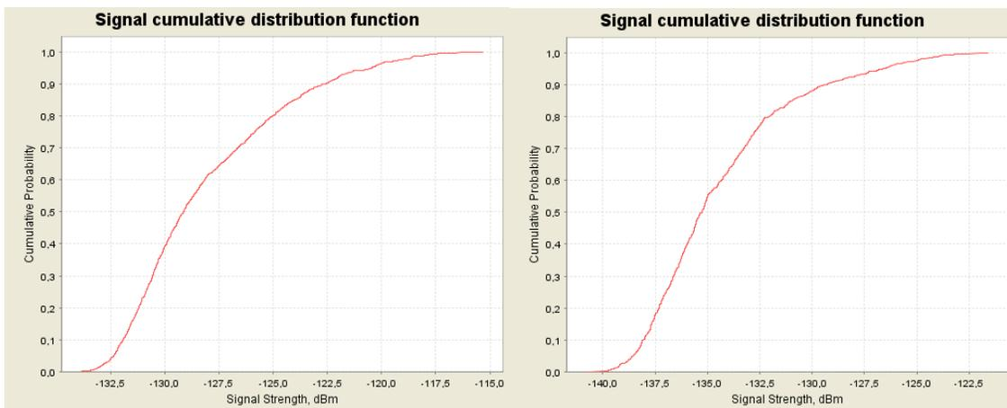
Figure 53: CDF graphs for the NCU (CDMA) for 450 MHz at 8000 m (left) and 10000 m (right) above ground
