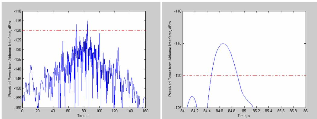
**Figure 84: Time history of interference power received by g-MS. Phased array with  $\pm 90^\circ$  random phase error**
