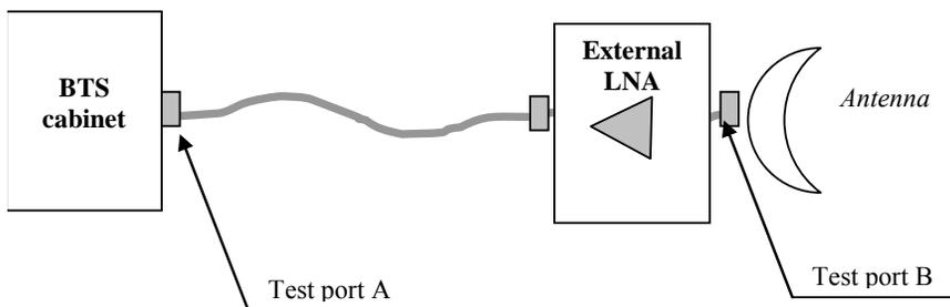
**Figure 103: BTS Reference Case 2 (LNA included)**
