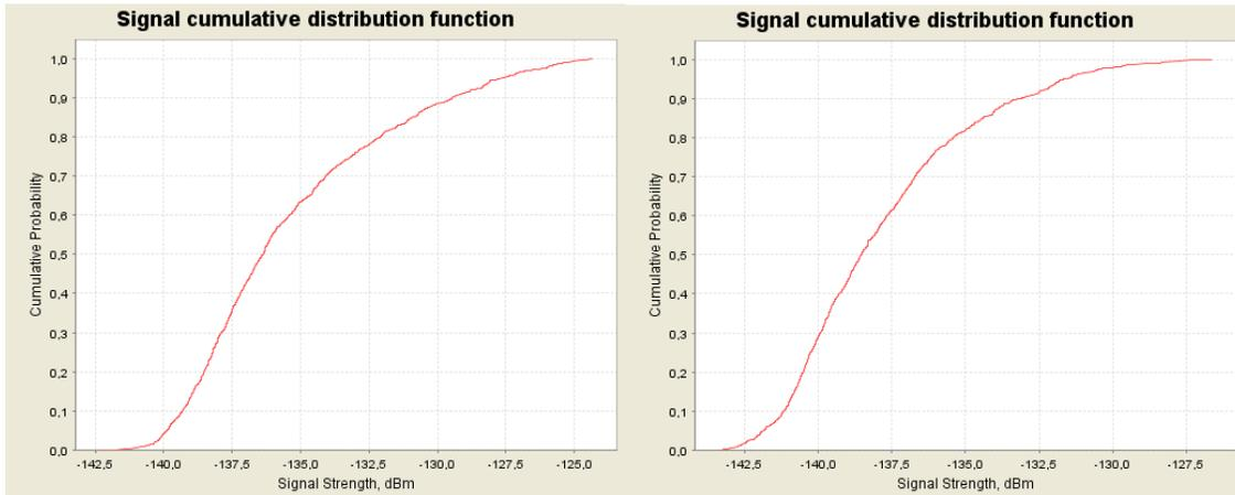
Figure 45: CDF graphs for the NCU (GSM) for 900 MHz at 8000 m (left) and 10000 m (right) above ground
