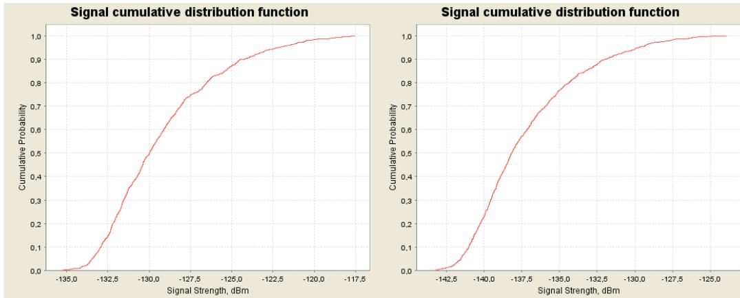
Figure 50: CDF graphs for the NCU (UMTS) for 1800 MHz at 3000 m (left) and 5000 m (right) above ground
