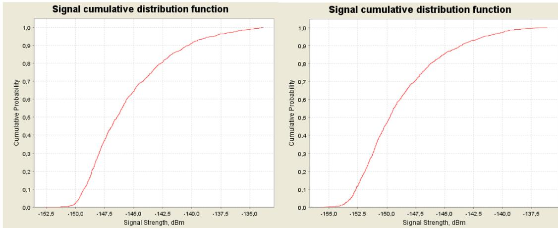
Figure 41: CDF graphs for the NCU (UMTS) for 2000 MHz at 8000 m (left) and 10000 m (right) above ground
