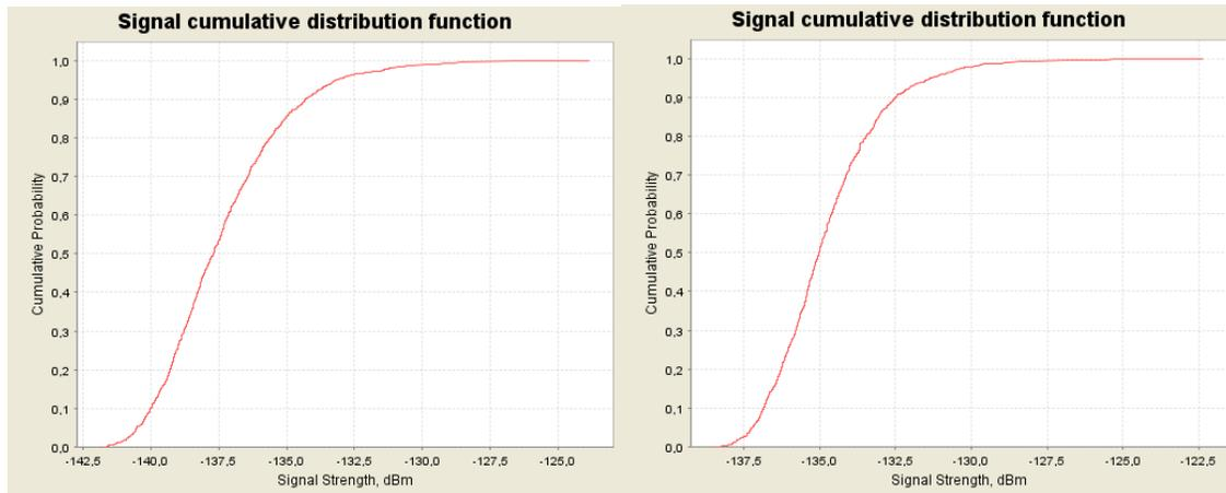
**Figure 57: CDF graphs for the multiple NCU (GSM) for 1800 MHz for normal busy (left) and extreme busy (right) cases**
