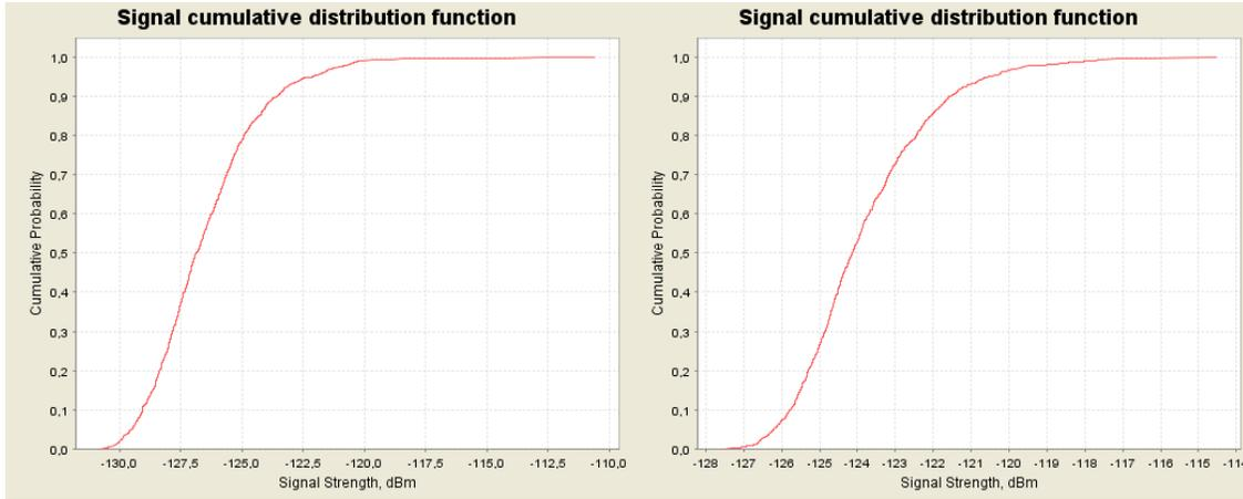
**Figure 61: CDF graphs for the multiple NCU (UMTS) for 1800 MHz for normal busy (left) and extreme busy (right) cases**
