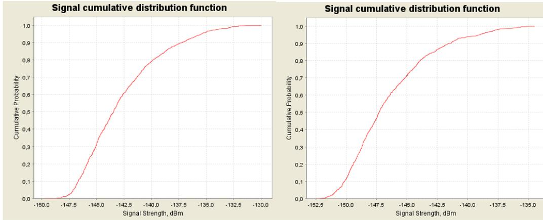
Figure 47: CDF graphs for the NCU (GSM) for 1800 MHz at 8000 m (left) and 10000 m (right) above ground
