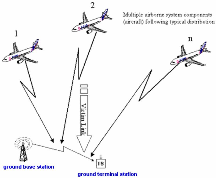
Figure 9: Scenario 4: GSMOB interfering terrestrial victim Downlink (g-BTS/NodeB to g-MS/UE) from multiple aircraft
