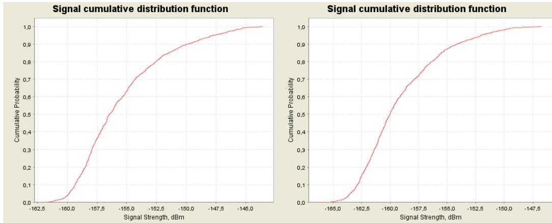
Figure 39: CDF graphs for the NCU (GSM) for 1800 MHz at 8000 m (left) and 10000 m (right) above ground
