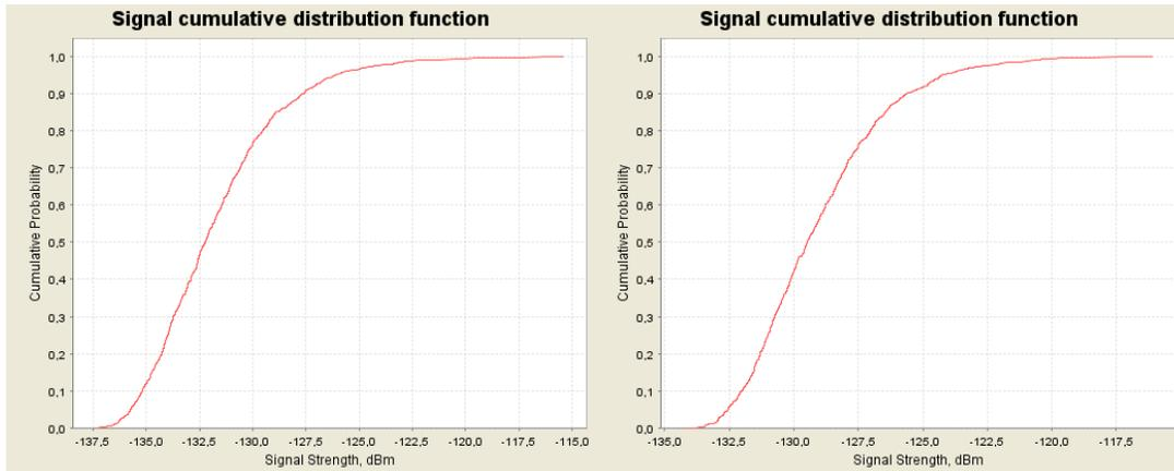
**Figure 54: CDF graphs for the multiple ac-BTS for 1800 MHz for 10 GSM 1800 channels onboard for the normal busy (left) and the extreme busy (right) cases**
