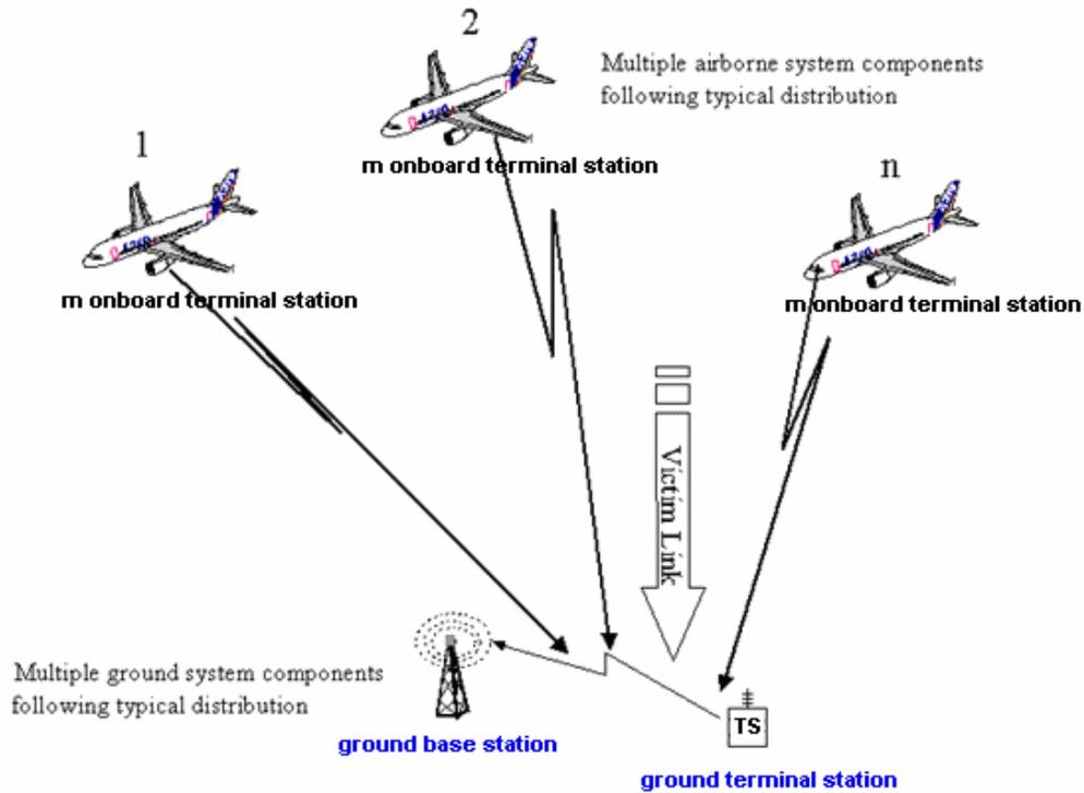
Figure 11: Scenario 6: GSMOB interfering terrestrial uplink (g-MS/UE to g-BTS/NodeB) from multiple aircraft
