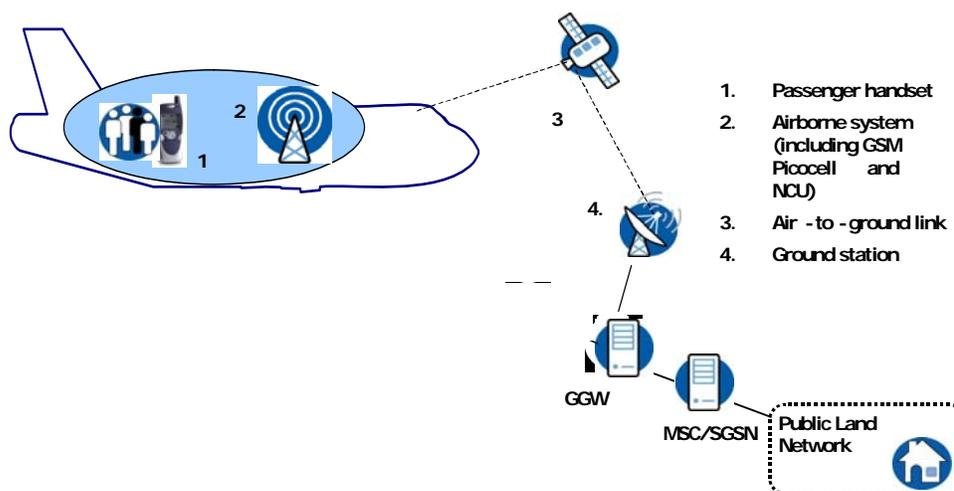
Figure 1: Overview of the GSMOB system and associated terrestrial components
