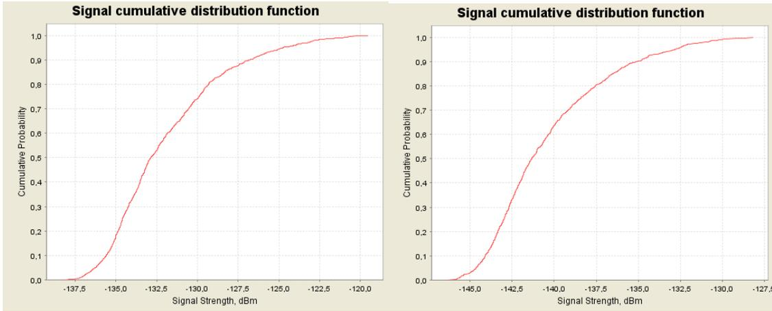
Figure 36: CDF graphs for the NCU (GSM) for 900 MHz at 3000 m (left) and 5000 m (right) above ground
