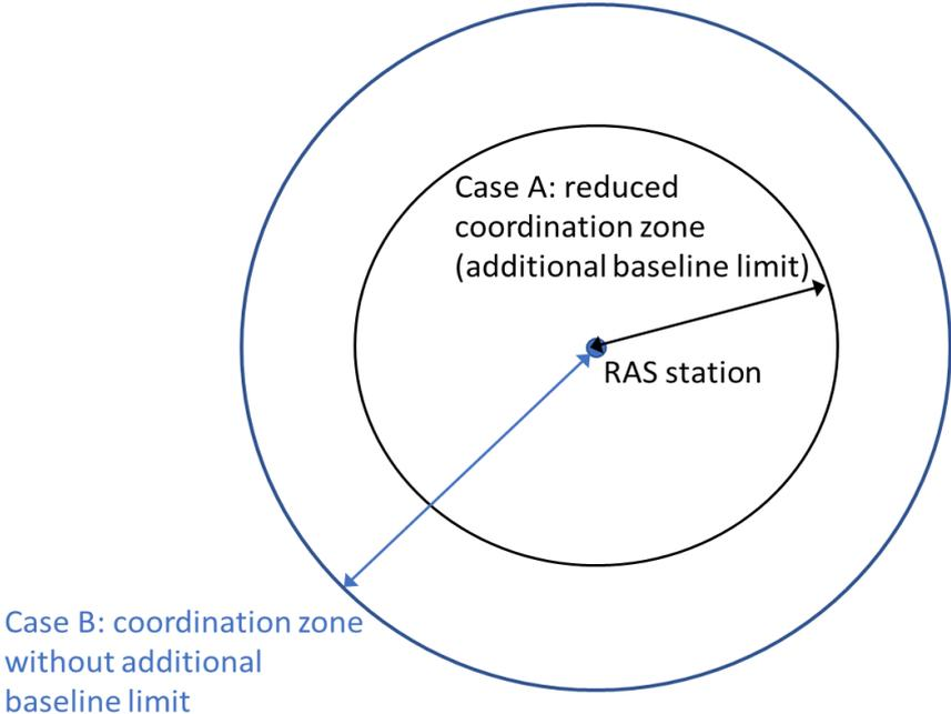
**Figure 12: Simplified example of coordination zones around RAS station for AAS base stations**
