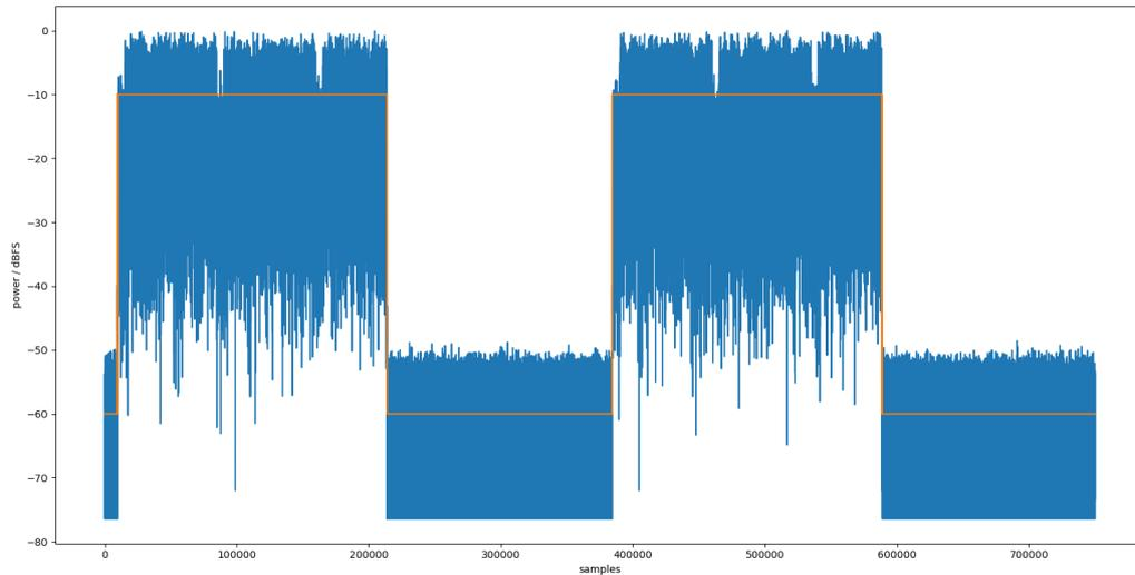
**Figure 71: Signal power vs. time and burst discriminator output**
