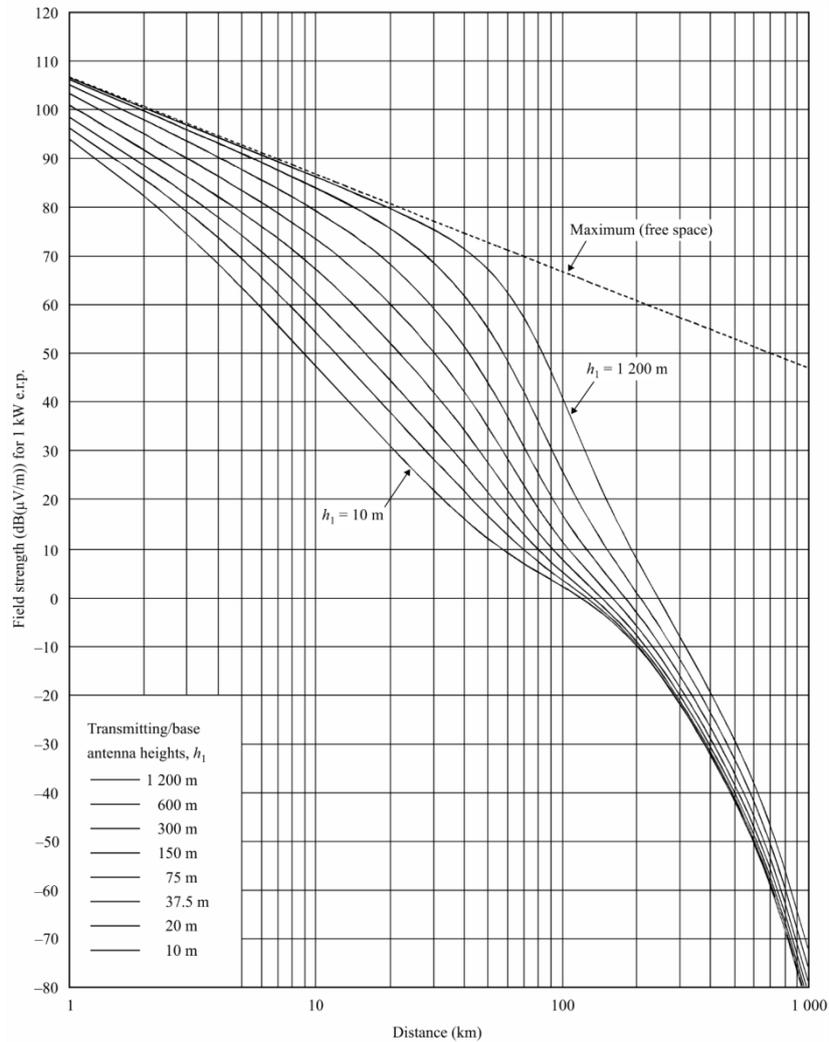
**Figure 39: Recommendation ITU-R P.1546 Field Strength for Various Antenna Heights**
