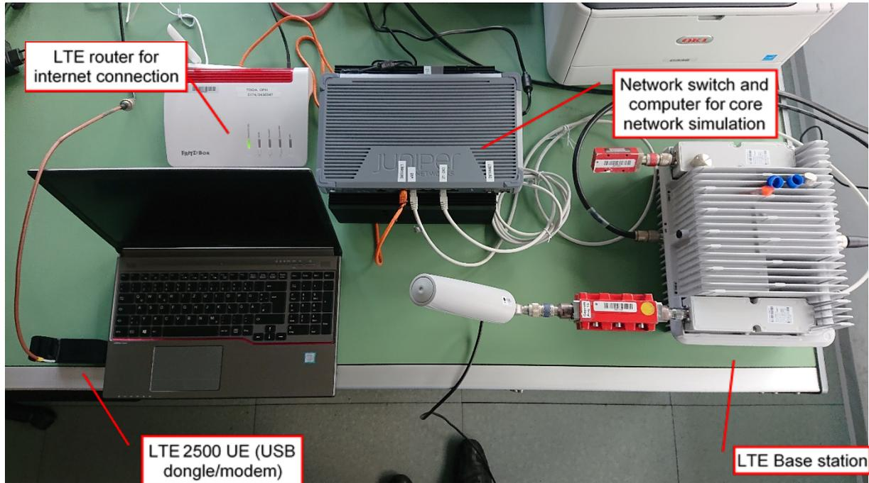
**Figure 46: Illustration of the LTE BS and UE**
