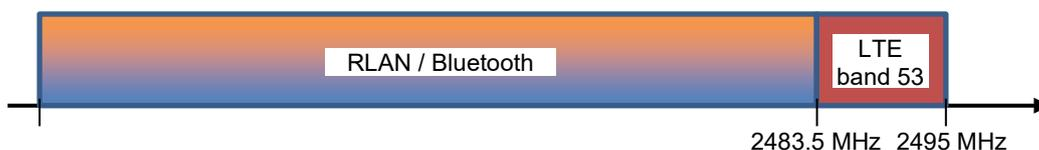
**Figure 44: Frequency band allocations**
