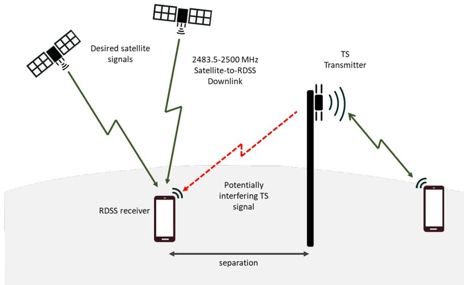
**Figure 6: Outdoor TS Base Station and UE device to RDSS receiver**
