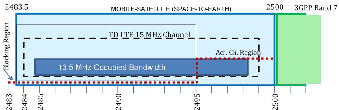
**Figure 41: The blocking response of E-UTRA 5 MHz channel in the TS 15 MHz channel**
