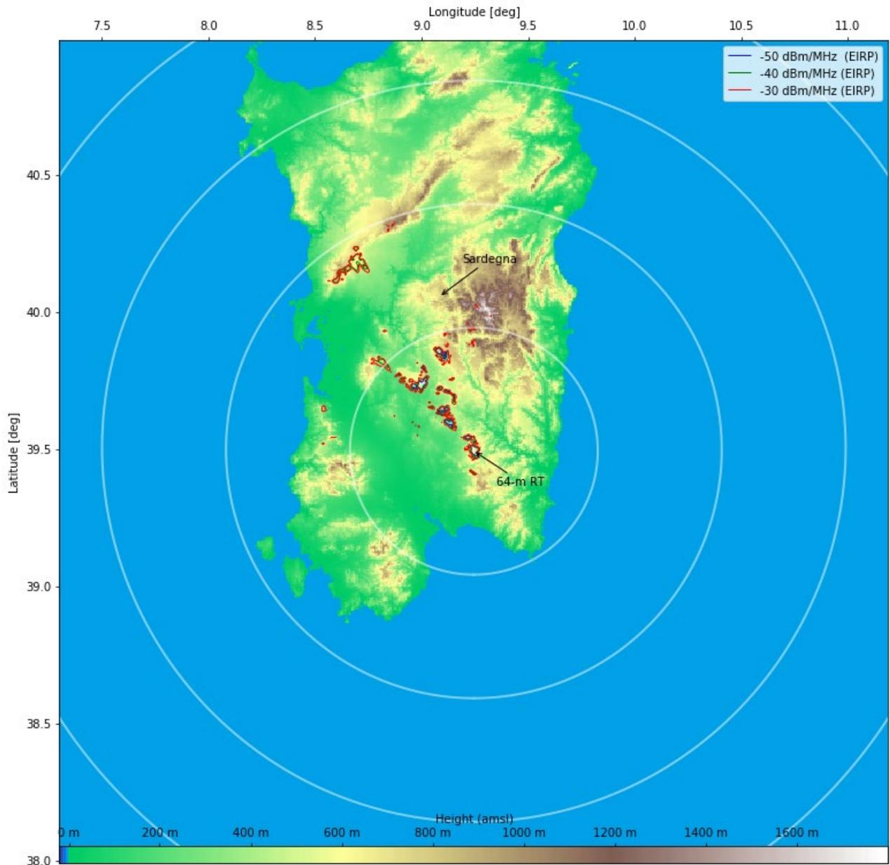
**Figure 36: Coordination zones for the single-interferer Sardegna case (4990-5000 MHz, continuum mode, UE at 1.5-m height) for various levels of spurious emission (-30/-40/-50 dBm/MHz)**
