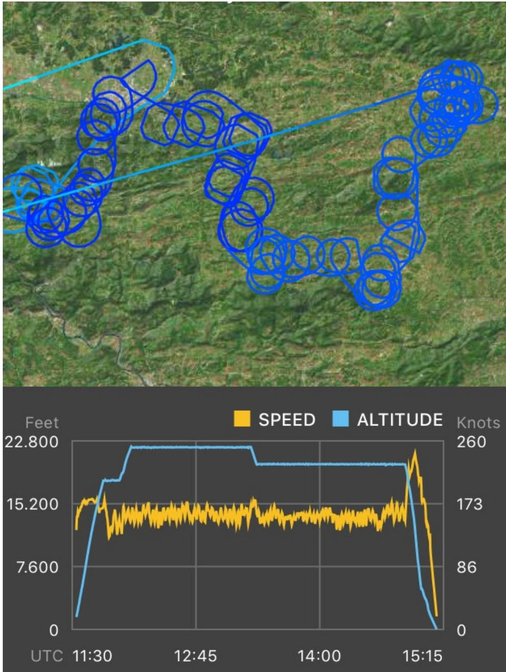
**Figure 16: Flight pattern copied from flight radar 24 showing the flightpath at 7km. of a relay airplane during the live coverage of a cycling race)**
