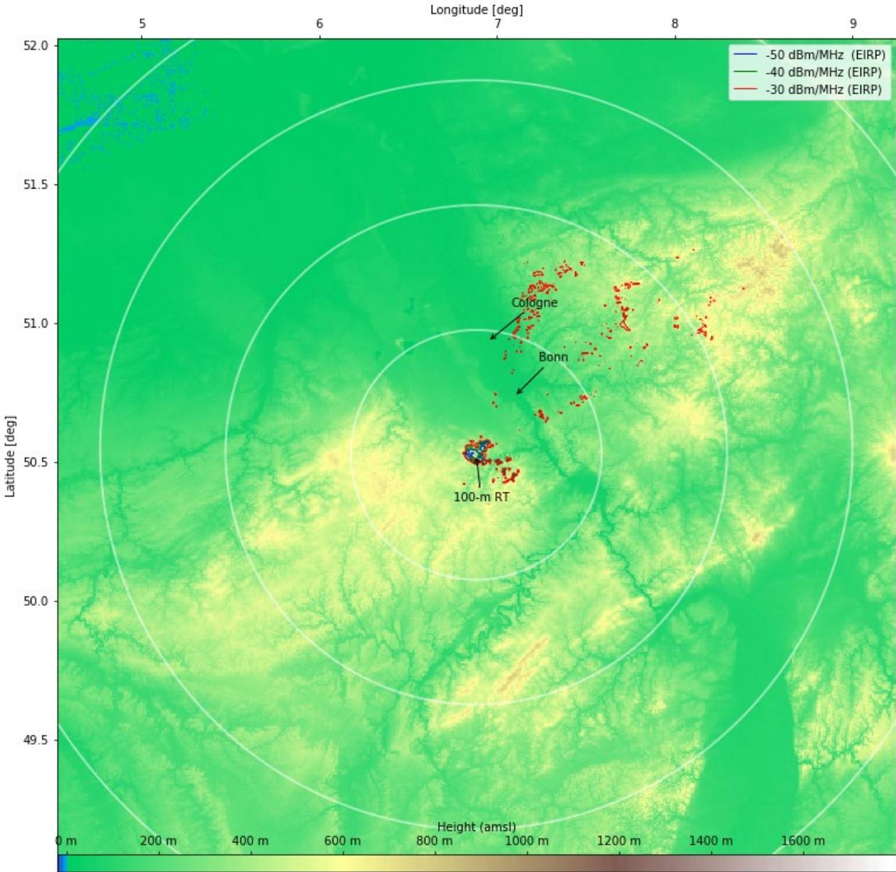
**Figure 34: Coordination zones for the single-interferer Effelsberg case (4990-5000 MHz, continuum mode, UE at 1.5-m height) for various levels of spurious emission (-30/-40/-50 dBm/MHz)**
