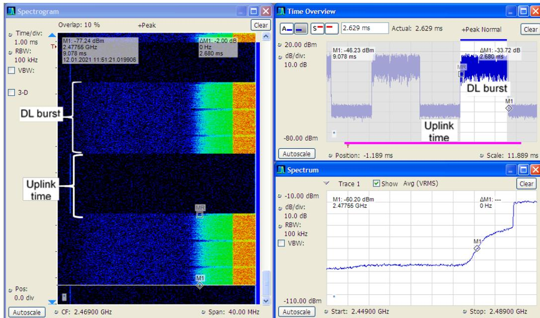
**Figure 48: Sample real time analyser display in the sideband measurements<sup>17</sup>**
