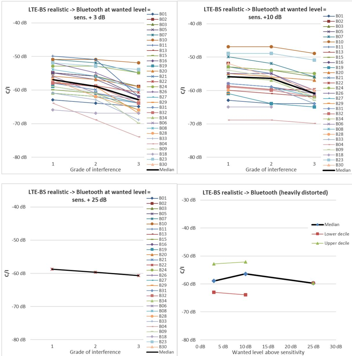
Figure 62: C/I for BLE devices exposed to LTE BS realistic interferer
