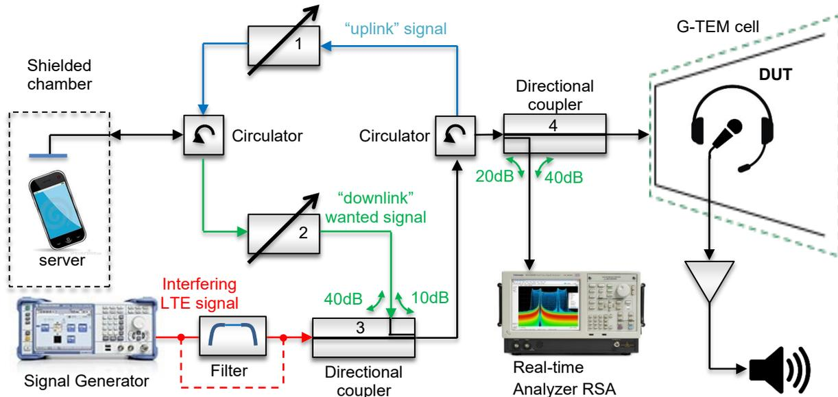
**Figure 58: Block diagram of the setup used for C/I measurements of devices with built-in antennas**
