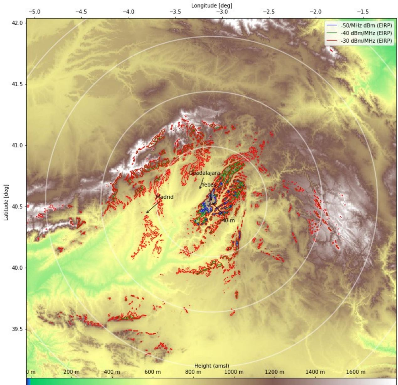
**Figure 35: Coordination zones for the single-interferer Yebes case (4990-5000 MHz, continuum mode, UE at 1.5-m height) for various levels of spurious emission (-30/-40/-50 dBm/MHz)**
