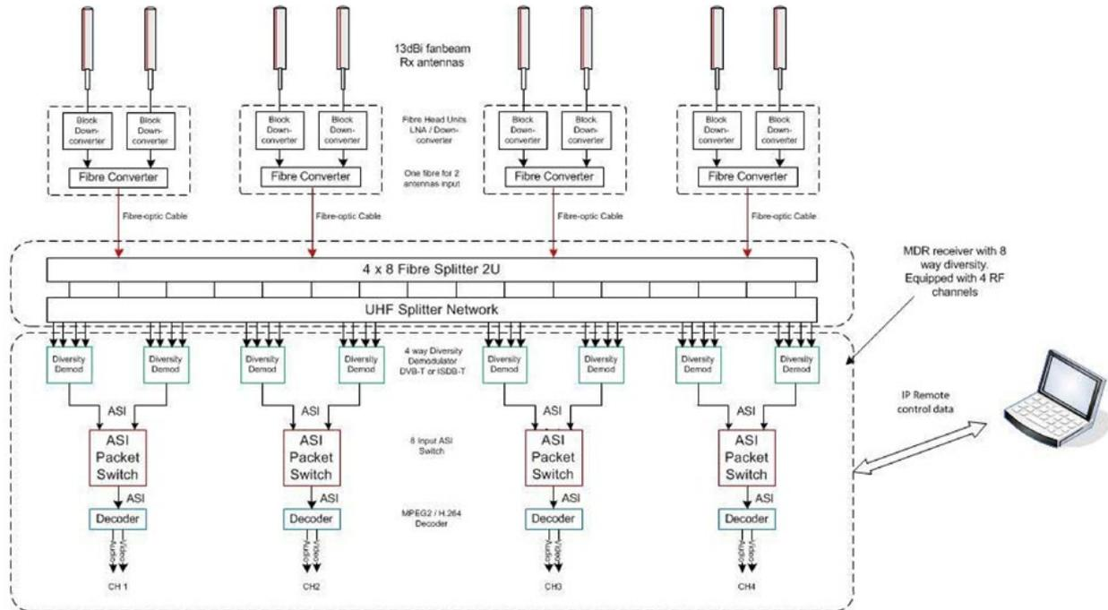
**Figure 18: Vislink 8-way diversity PMSE reception system**
