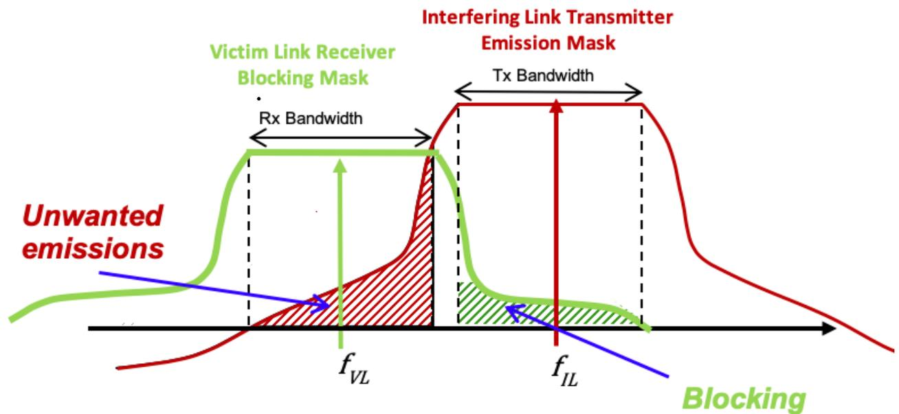
Figure 28: Blocking and Unwanted Emissions
