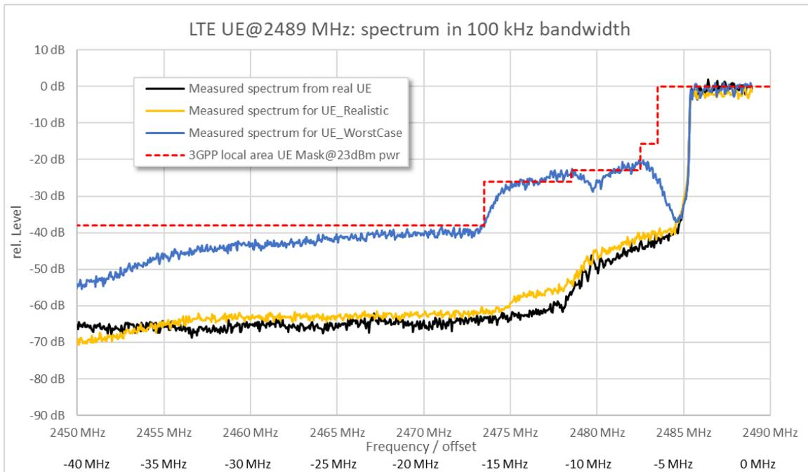
**Figure 53: Sideband emissions of LTE UE signals**
