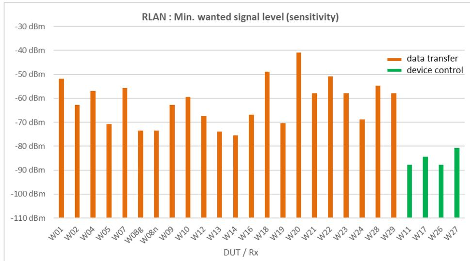
**Figure 57: Measured sensitivity of the selected RLAN devices**
