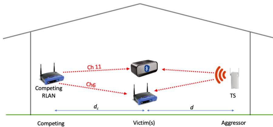
**Figure 31: Indoor TS to Indoor ISM devices**
