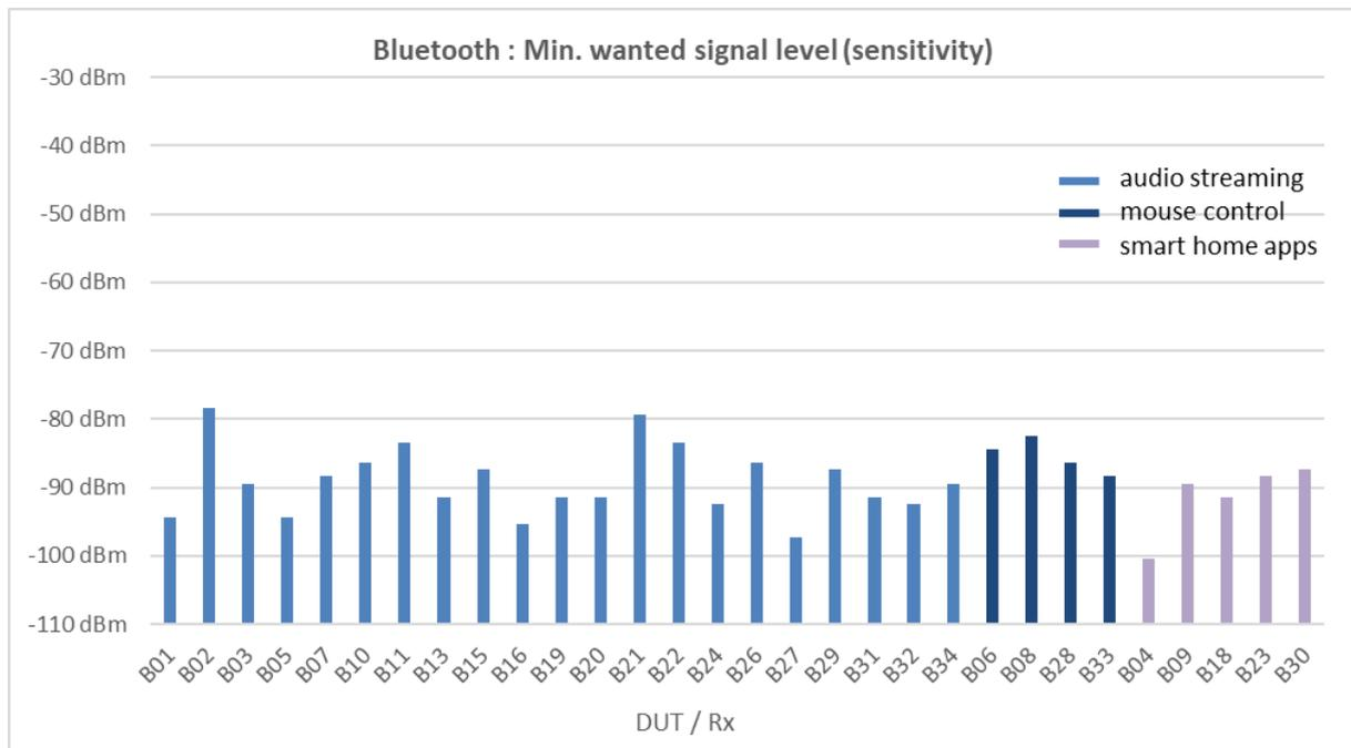
**Figure 56: Measured sensitivity of the selected Bluetooth devices**
