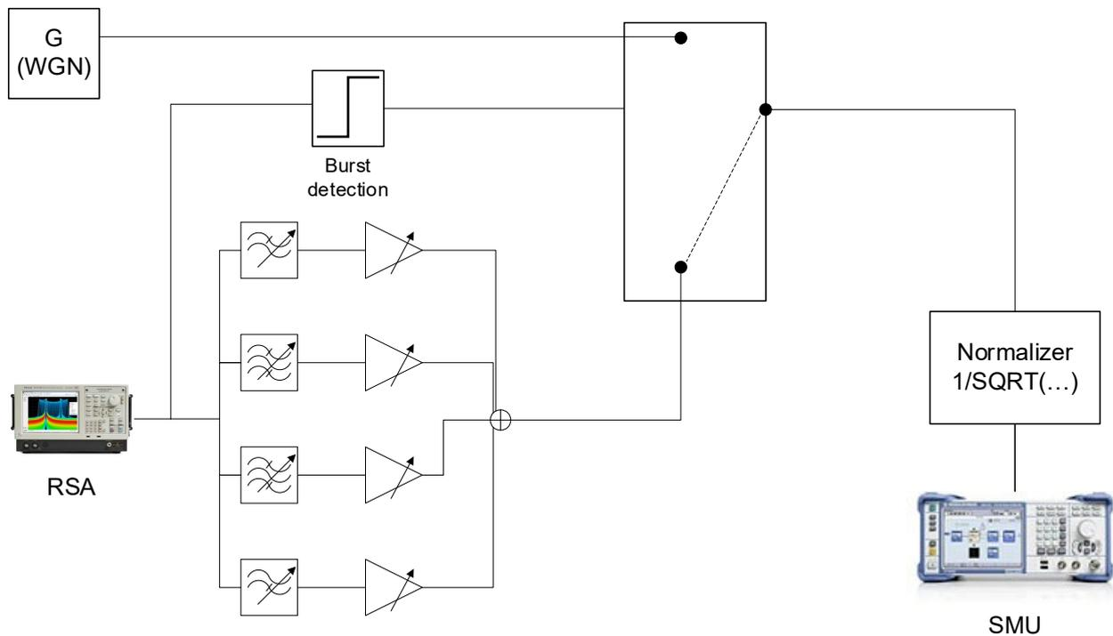
**Figure 70 -: signal conditioner schematic**
