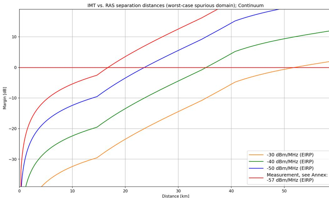
**Figure 32: Margin vs. distance for the single-interferer generic case (4990-5000 MHz, continuum mode)**
