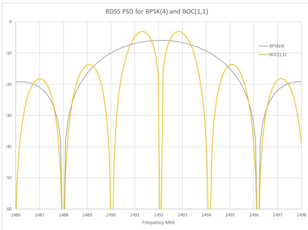
**Figure 5: RDSS Example Power Spectral Densities**
