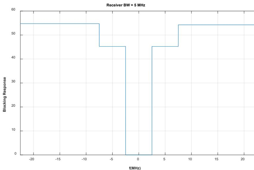
**Figure 40: Blocking response of E-UTRA BS receiver with 5 MHz channel BW**
