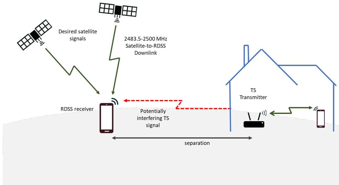
**Figure 7: Indoor TS Base Station and UE device to RDSS receiver**
