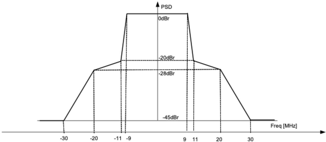
**Figure 24: IEEE 802.11 Transmission Spectral Mask**
