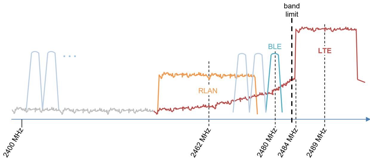
**Figure 45: Frequency arrangement**
