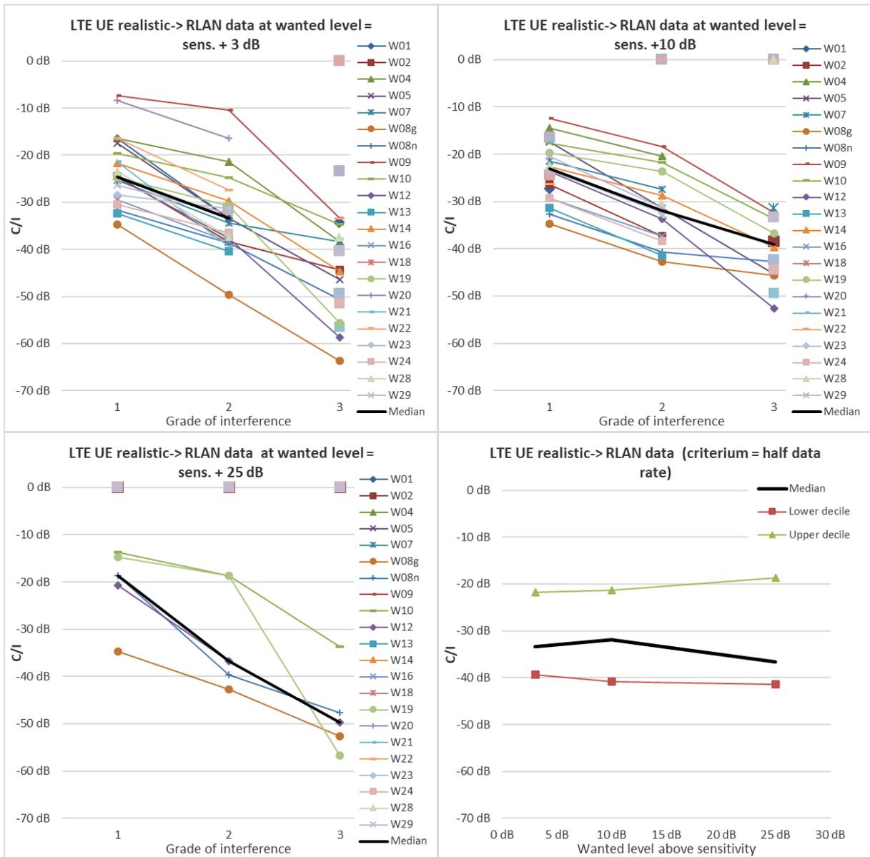
Figure 68: C/I for RLAN data transfer devices exposed to LTE UE realistic interferer
