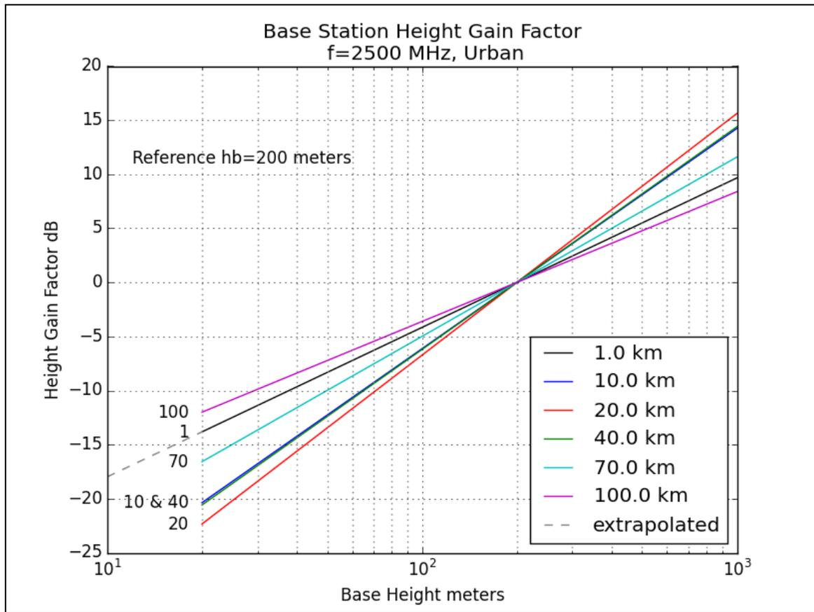
**Figure 38: Hata Base Height Gain Factor**
