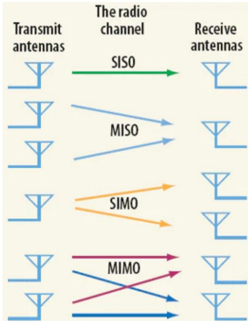
Figure 17: The radio link channel models
