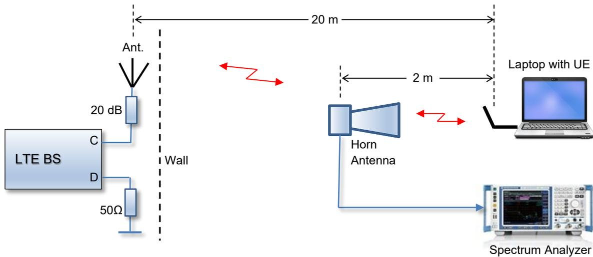
**Figure 74: Block diagram of the setup to measure the UE harmonics**
