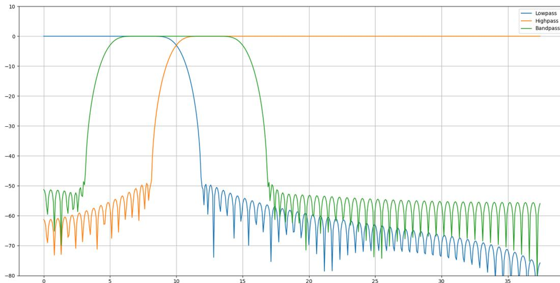
**Figure 72: frequency response of the 3 basic filter types used in the equalizer (x-axis: frequency in MHz; y-axis: attenuation in dB)**
