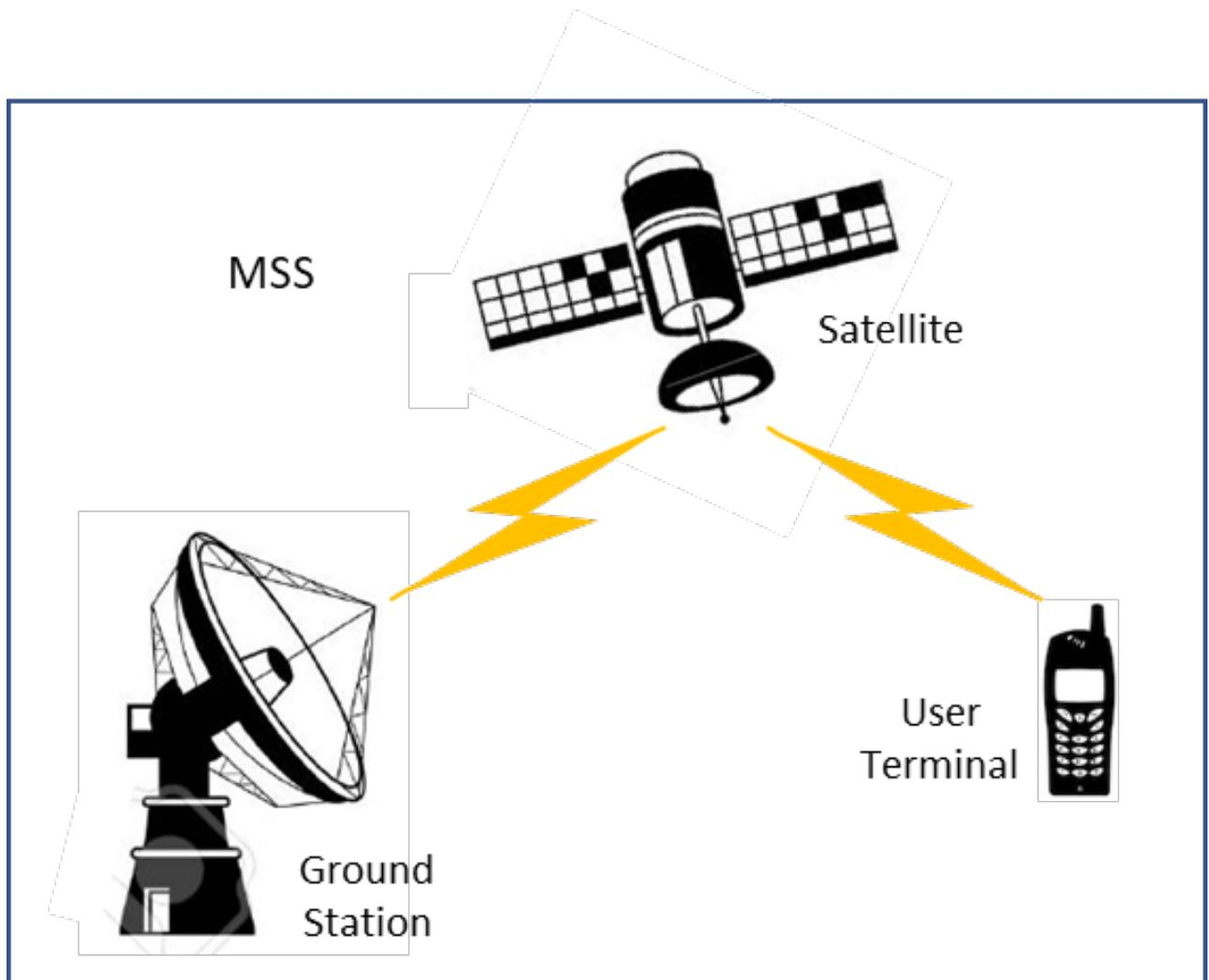
**Figure 3: MSS example system components**
