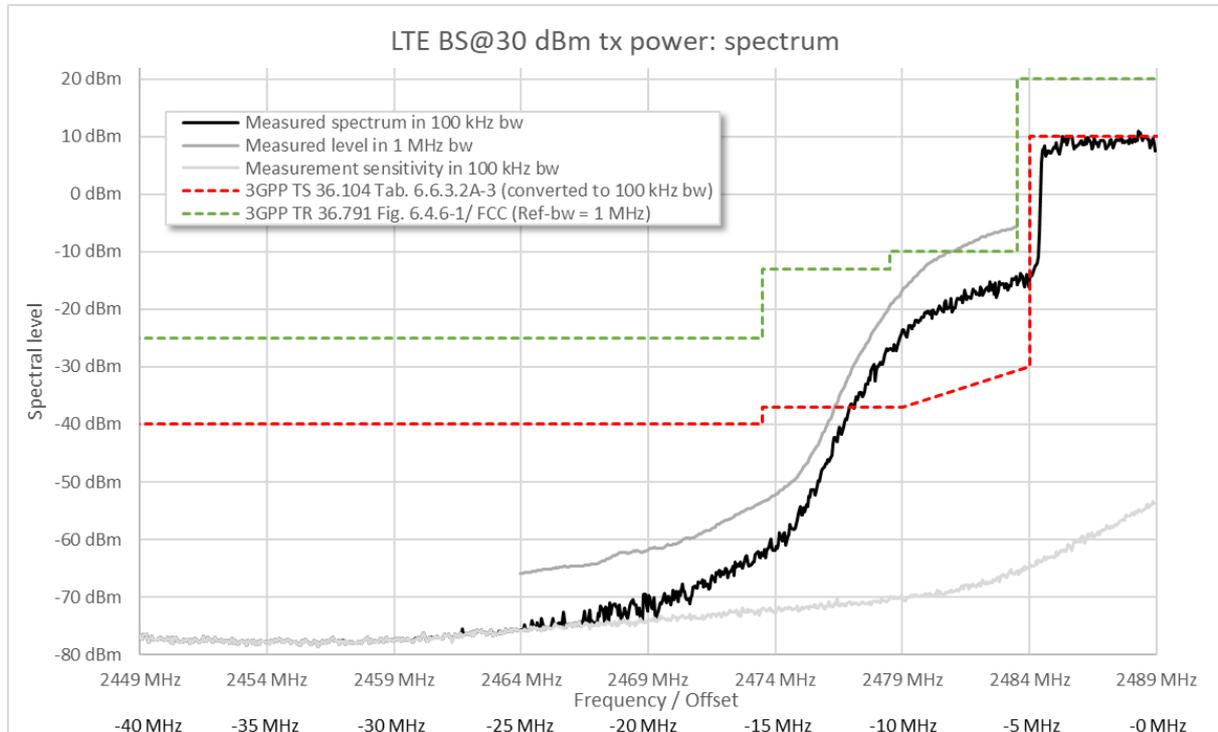
**Figure 49: Measured BS sideband spectrum and limit lines**
