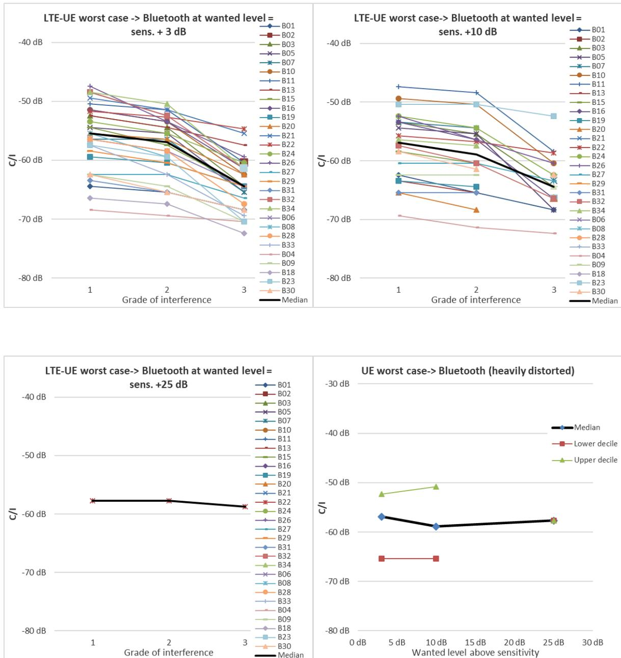
**Figure 65: C/I for BLE devices exposed to LTE UE worst case interferer**
