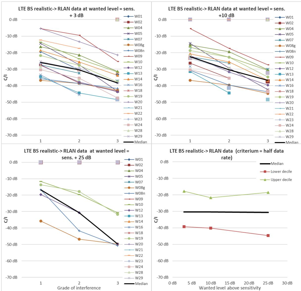
Figure 66: C/I for RLAN data transfer devices exposed to LTE BS realistic interferer
