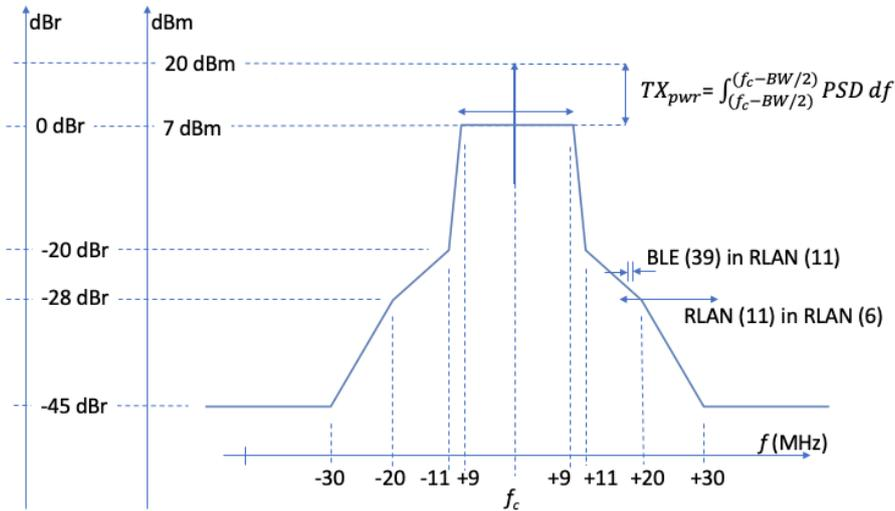
Figure 29: RLAN Transmission Mask with Unwanted Regions
