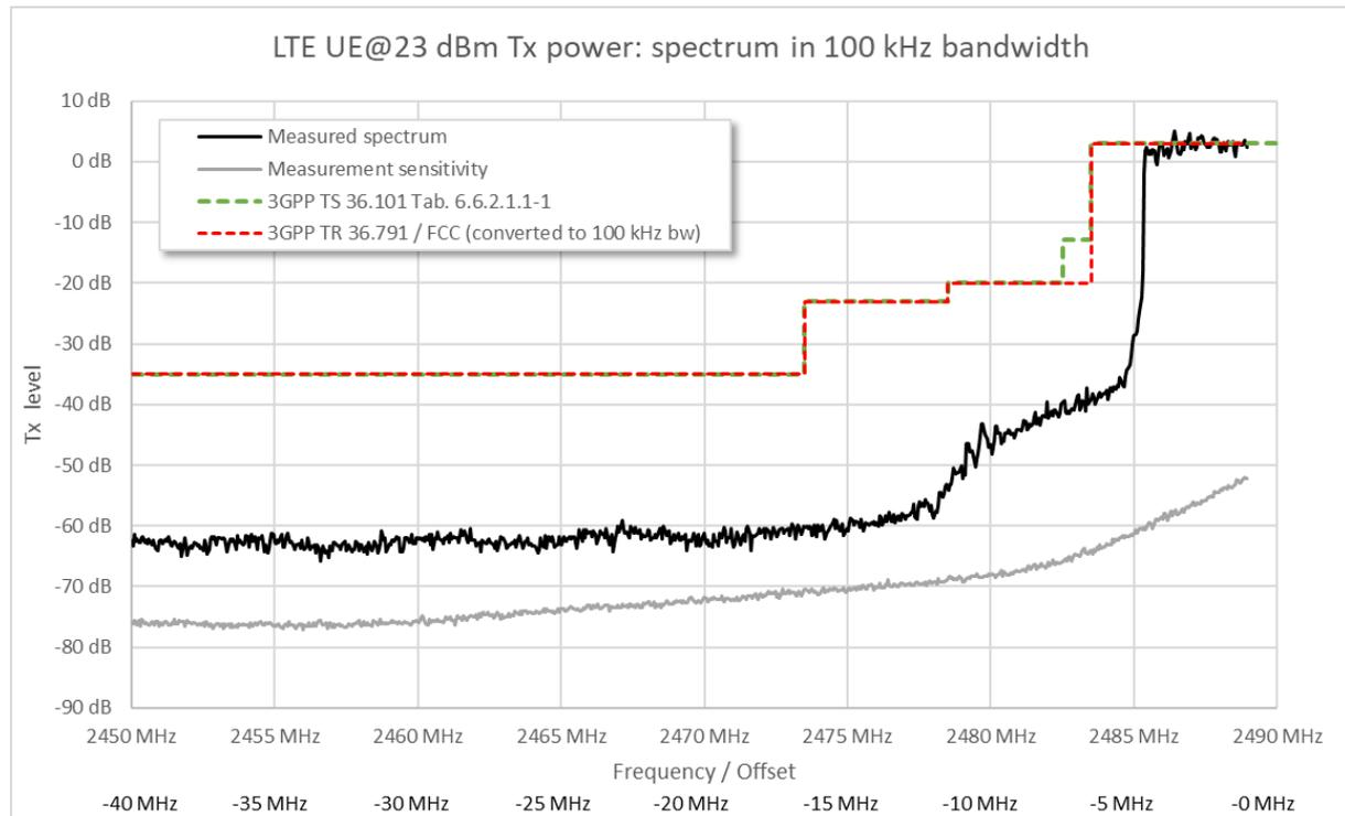
**Figure 51: Measured UE sideband spectrum and limit lines**
