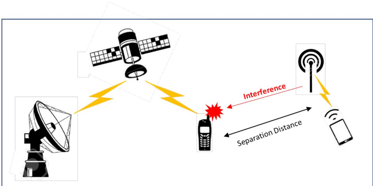
**Figure 4: Interference case considered**
