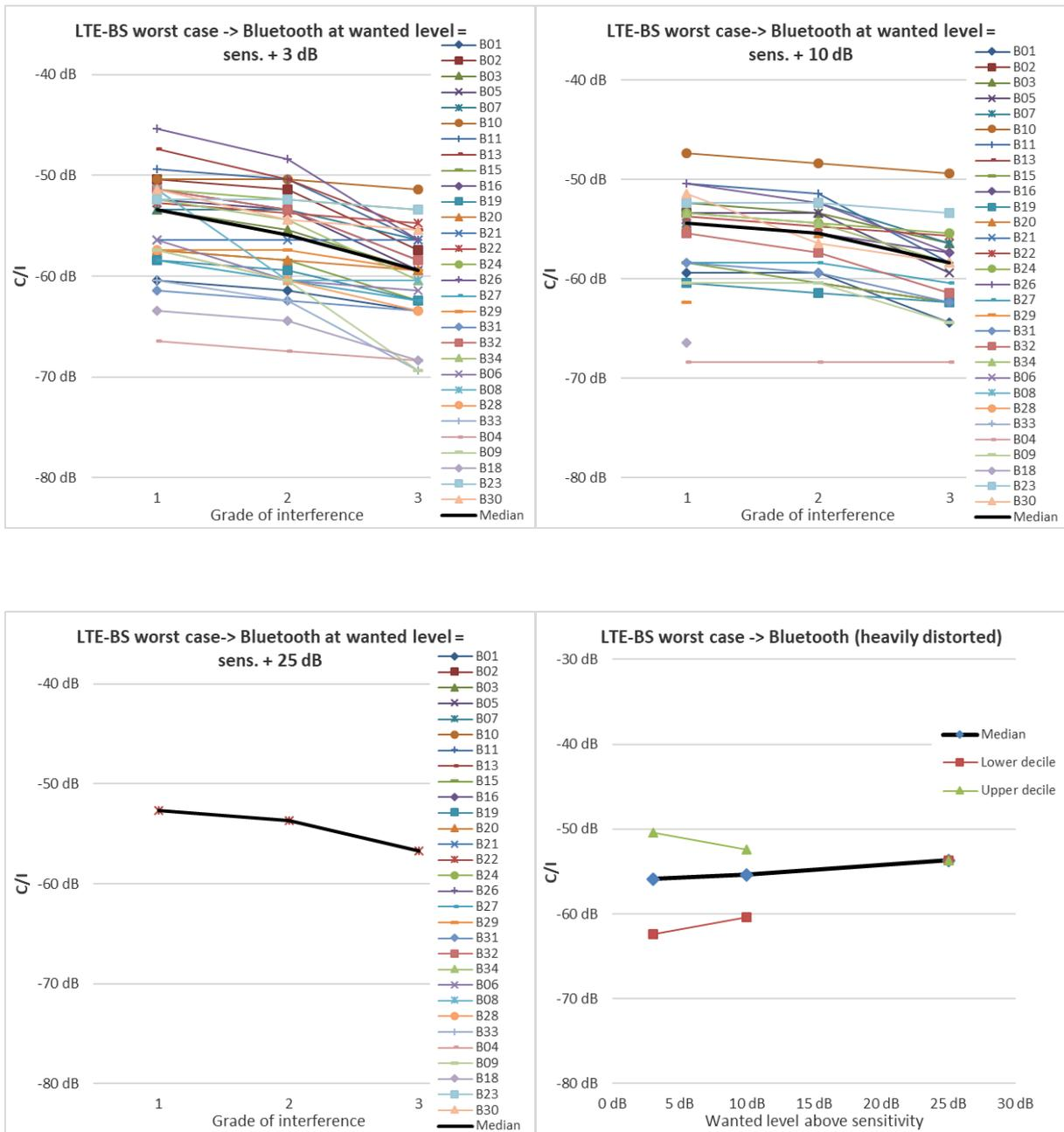
Figure 63: C/I for BLE devices exposed to LTE BS worst case interferer
