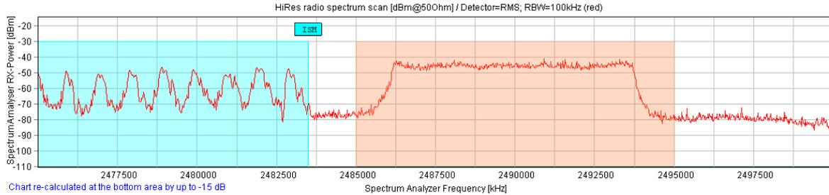
**Figure 42: Aggregated spectrum usage in the frequency domain of a video camera**
