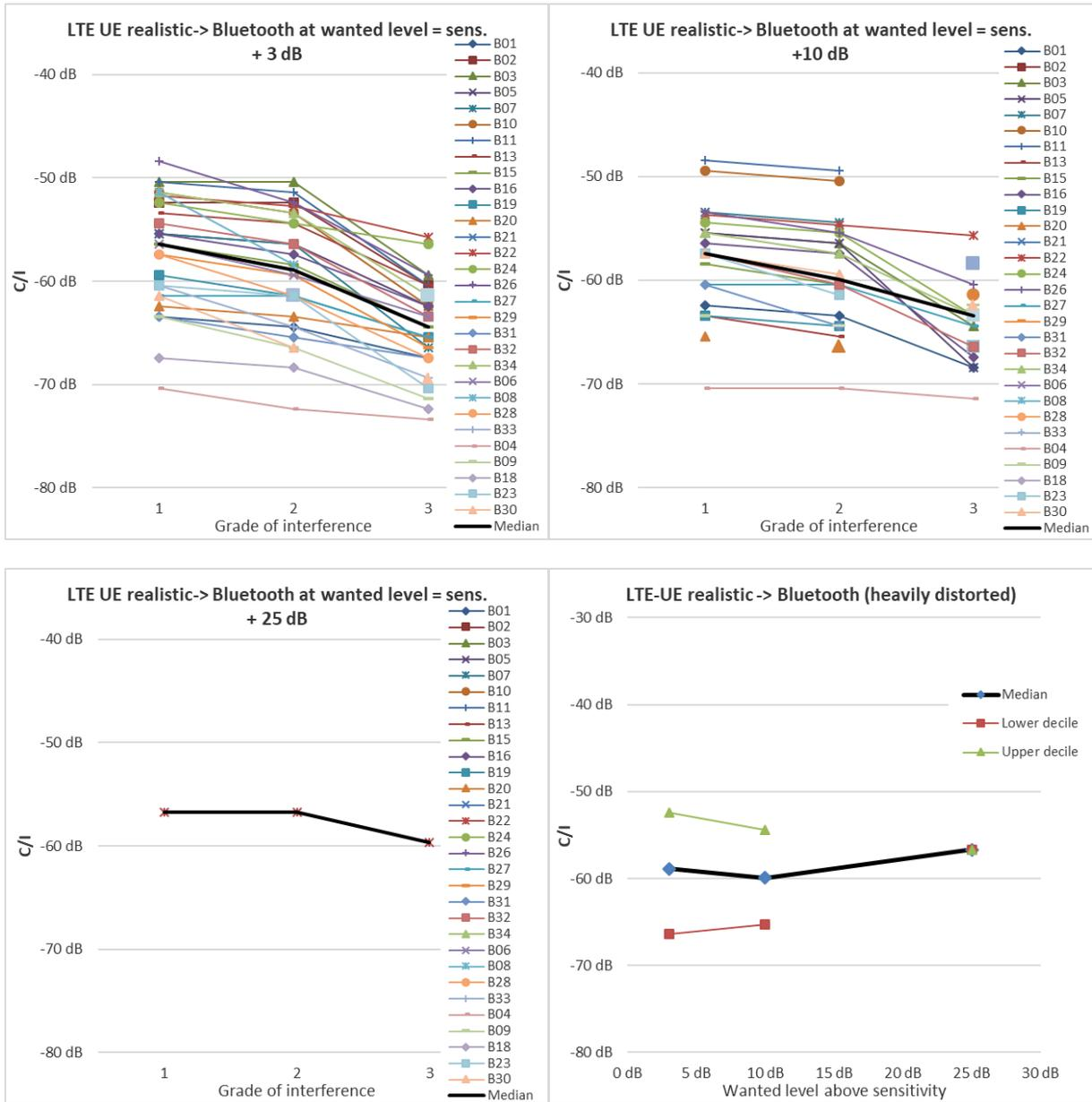
Figure 64: C/I for BLE devices exposed to LTE UE realistic interferer
