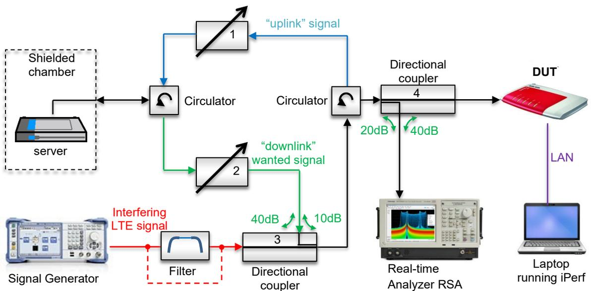
**Figure 60: Block diagram of the setup used for C/I measurements of devices with external antenna connectors**
