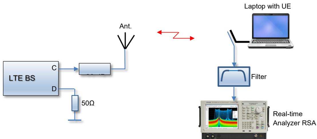
**Figure 50: Block diagram of the setup to record the LTE UE spectrum**
