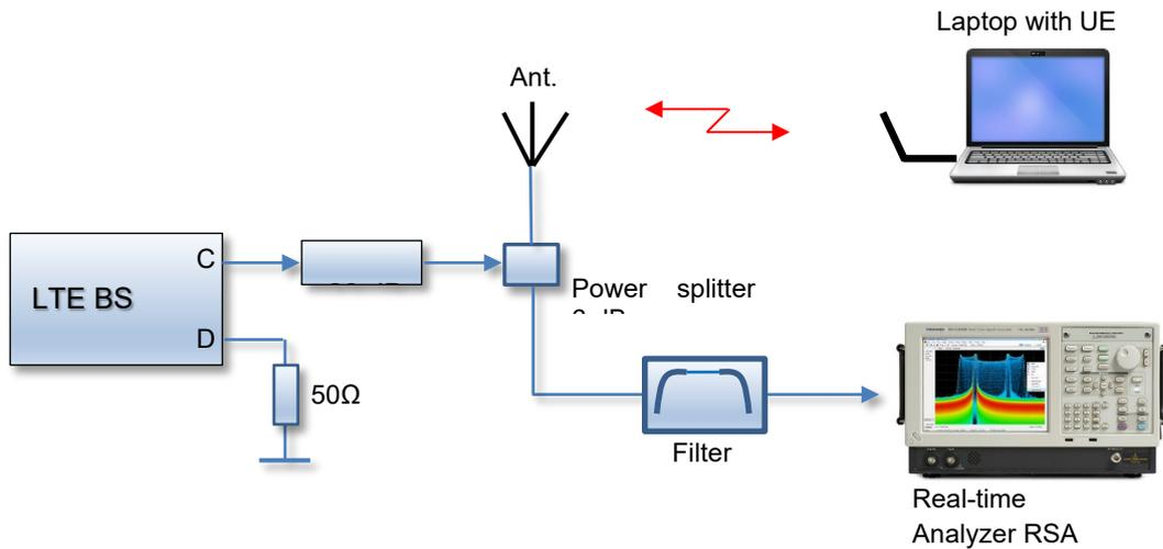
**Figure 47: Block diagram of the setup to record the LTE BS spectrum**
