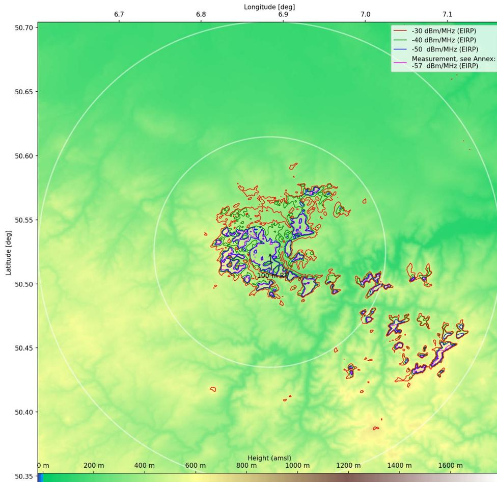
**Figure 33: Coordination zones for the single-interferer Effelsberg case (4990-5000 MHz, continuum mode, UE at 1.5-m height) based on measurement results**
