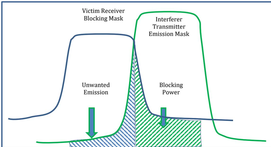
**Figure 21: Blocking and unwanted emissions diagram**
