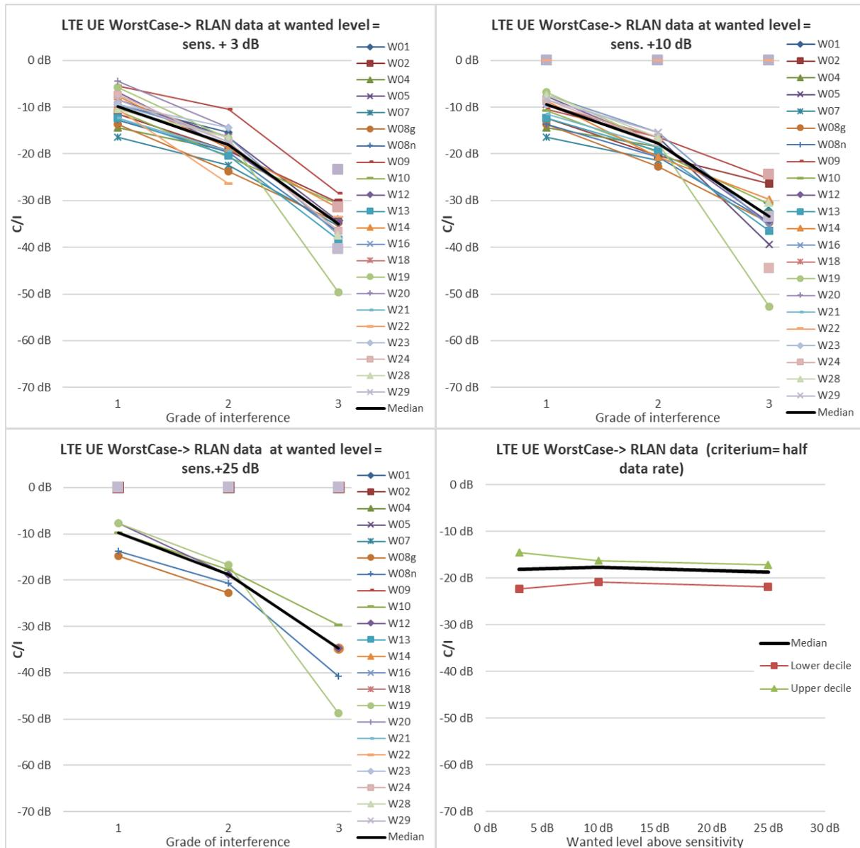
**Figure 69: C/I for RLAN data transfer devices exposed to LTE UE worst case interferer**
