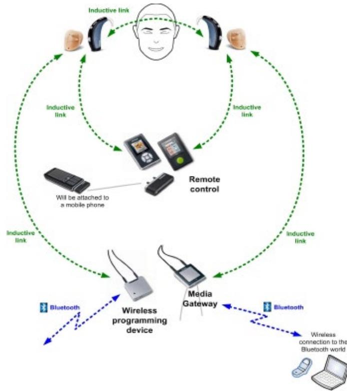
**Figure 26: ALD using inductive neck loop**
