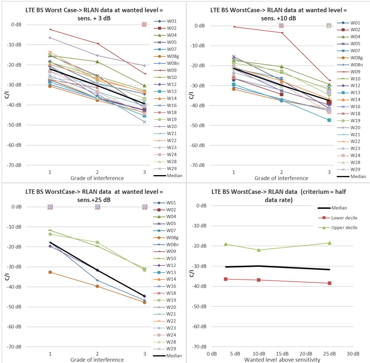
Figure 67: C/I for RLAN data transfer devices exposed to LTE BS worst case interferer
