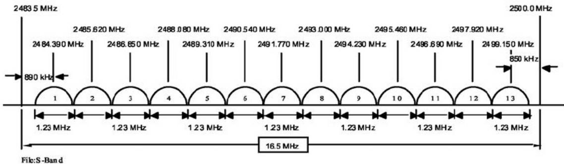
**Figure 2: CDMA channels within the downlink satellite-to-user device band**
