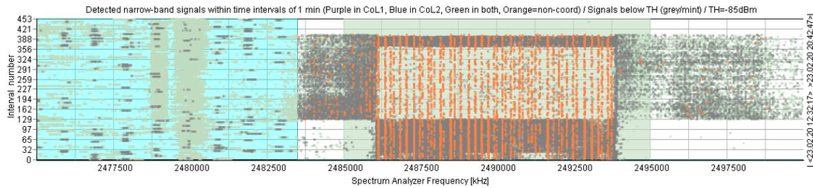
**Figure 43: Frequency usage of a video camera in time domain, 5-minute time blocks**
