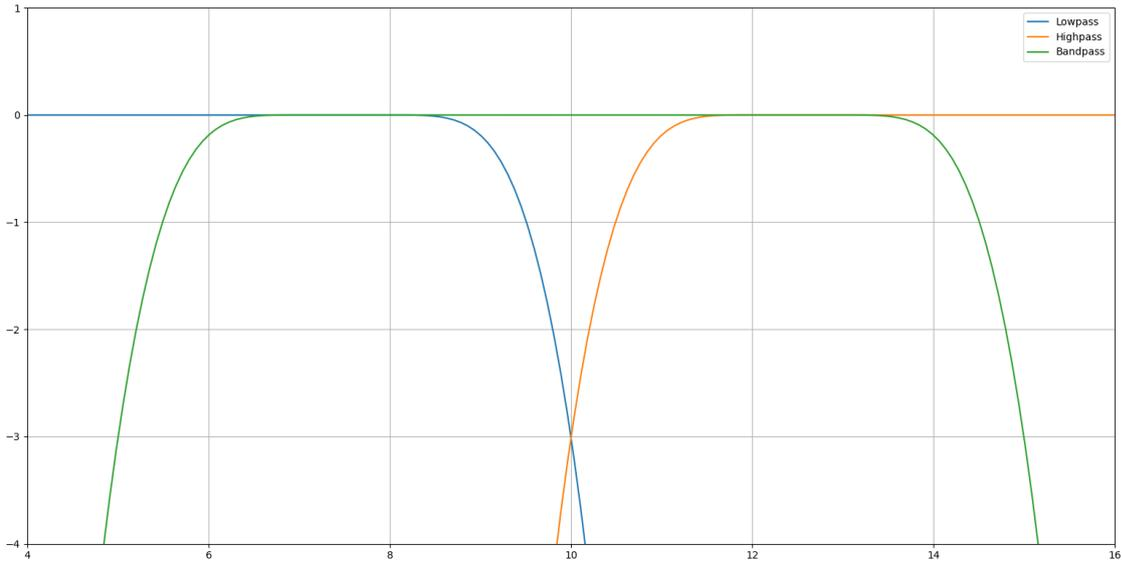
**Figure 73: frequency response of the 3 basic filter types used in the equalizer (x-axis: frequency in MHz; y-axis: attenuation in dB); zoomed**
