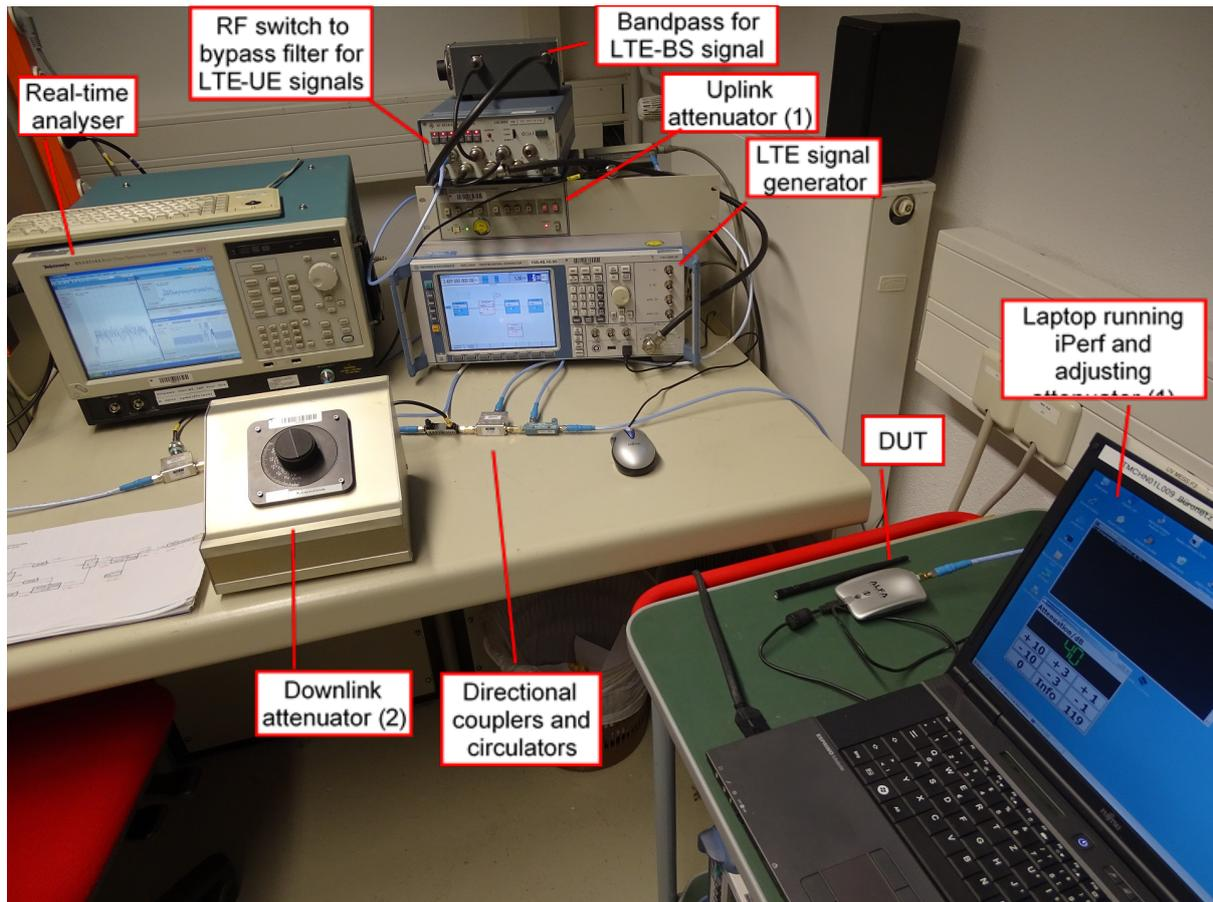
**Figure 61: Illustration of the measurement setup for devices with external antennas (example: USB Wi-Fi Adaptor)**
