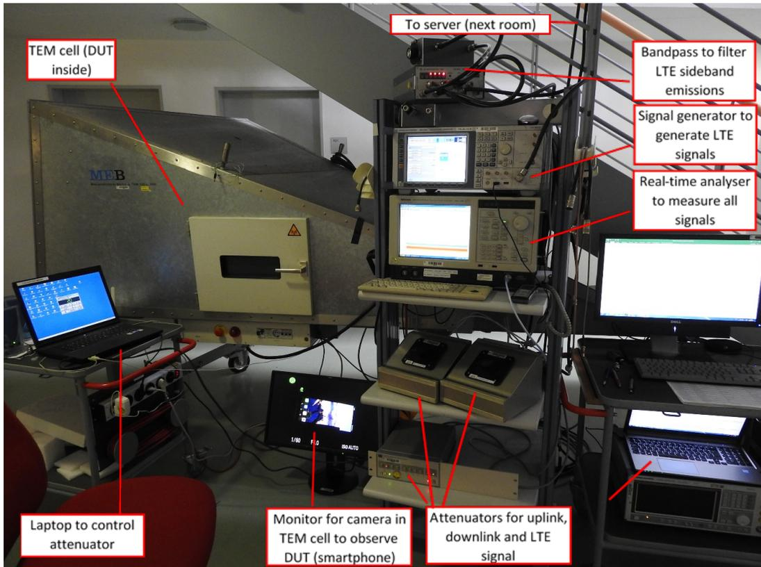
**Figure 59: Illustration of the measurement setup for devices with built-in antennas (example: BLE mouse control)**
