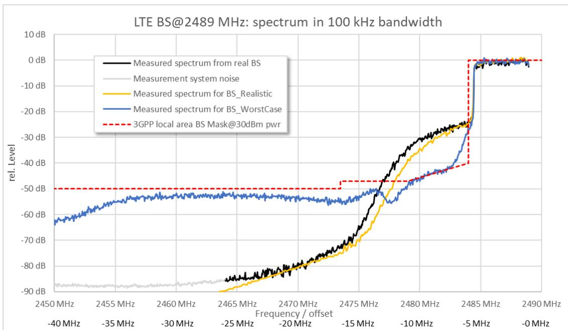
**Figure 52: Sideband emissions of LTE BS signals**
