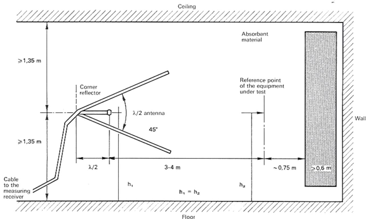
Figure I-1 (T/R 24-03). Indoor site arrangement (shown for horizontal polarisation).
