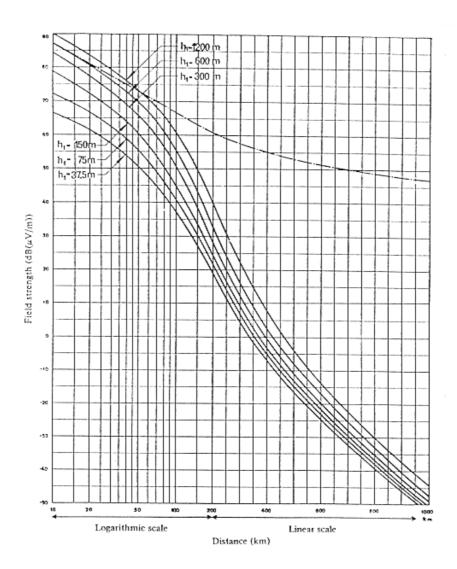
Field strength (dB ( $\mu$ V/m)) for 1 kW e.r.p. Frequency: 450 to 1000 MHz (Bands IV and V) - Cold sca = 10% of the time - 50% of the locations -  $h_2$  = 10 m --- - Free space
