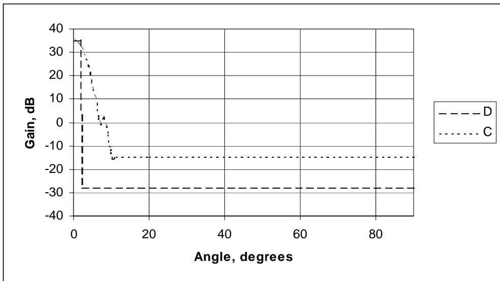
Figure 9: TM04069 antenna (C), and "perfect" equivalent (D)
