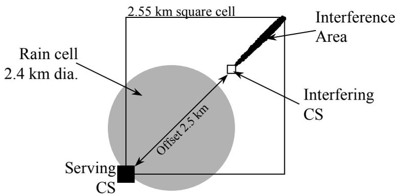
Figure 7: Geometry for IA computation
