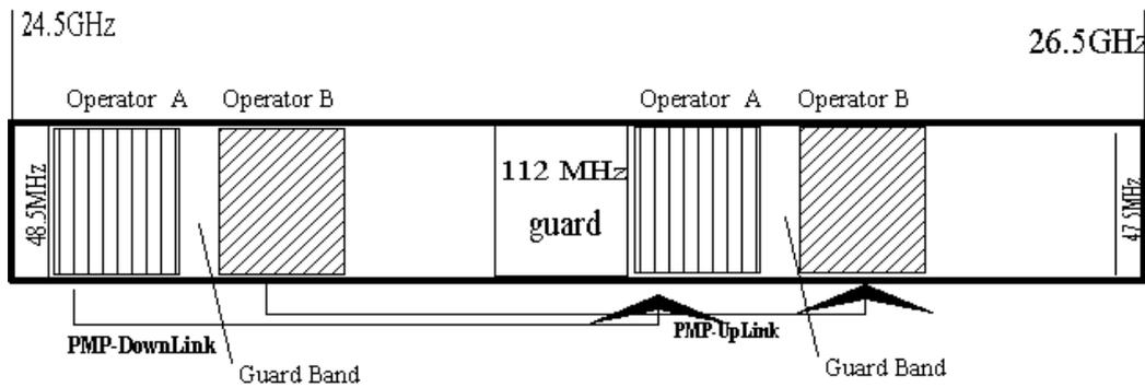
We also assume to state that one of the sub-bands ( lower) is for downlink purposes only, while the other sub-band (upper) is for uplink purposes only. This is needed in order to assume that, in the FDD case, the hub to hub and terminal to terminal interference scenarios can never happen.
