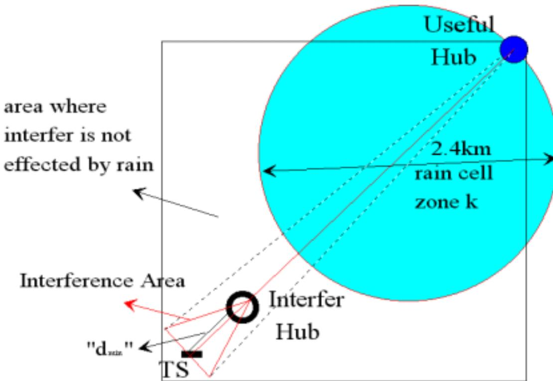
Figure 4: Interference scenario reference model
