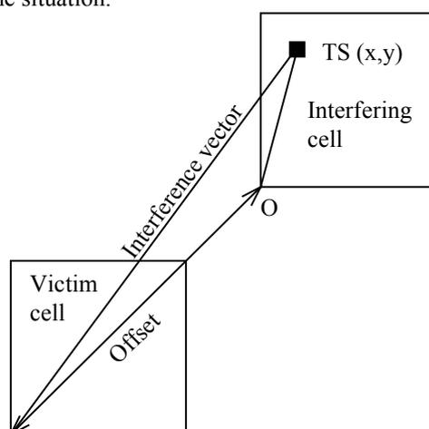
Figure 26: MC Interference geometry for co-channel uplink
