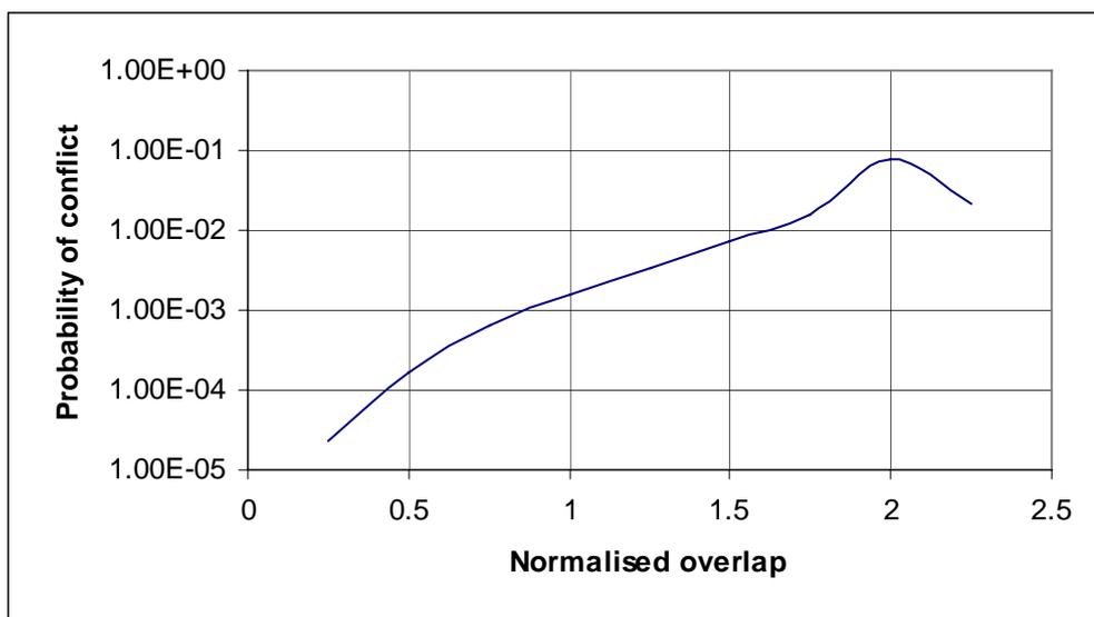
Figure 15: Interference probability as function of cell overlap
