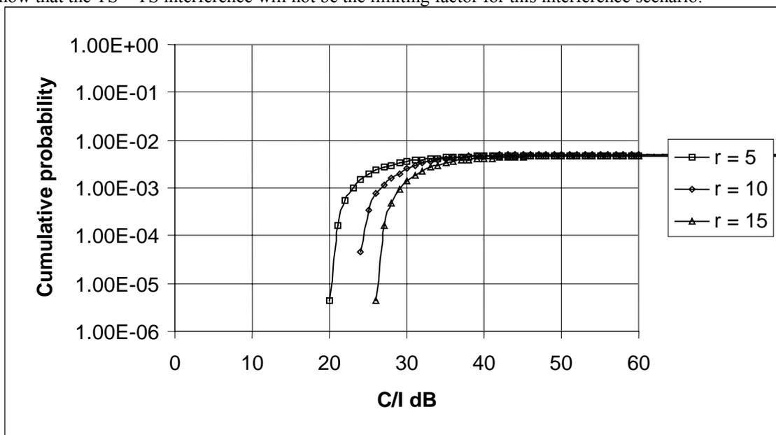
Figure 30: C/I distribution for same frequency adjacent area case
