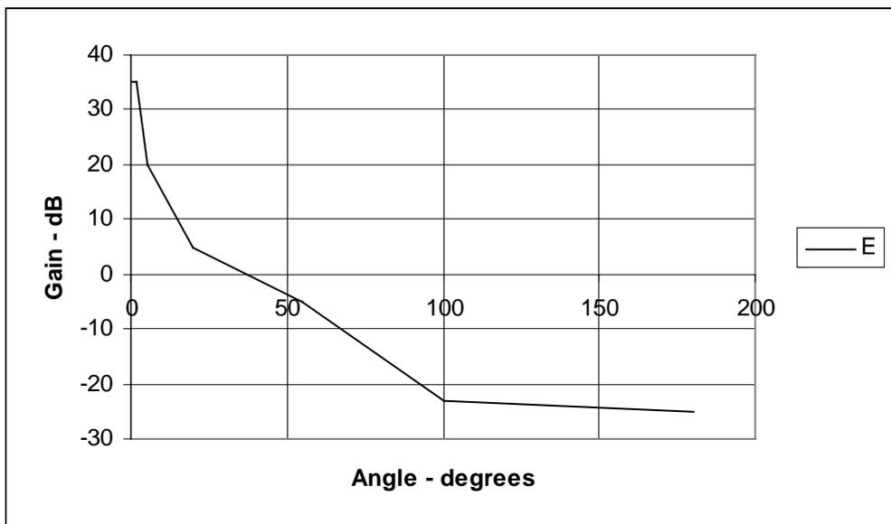
Figure 10: IEEE 802.16 26 GHz Type 2 antenna RPE
