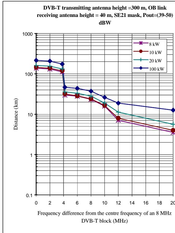
**Necessary separation distances in km between DVB-T and OB links in bands IV and V**
