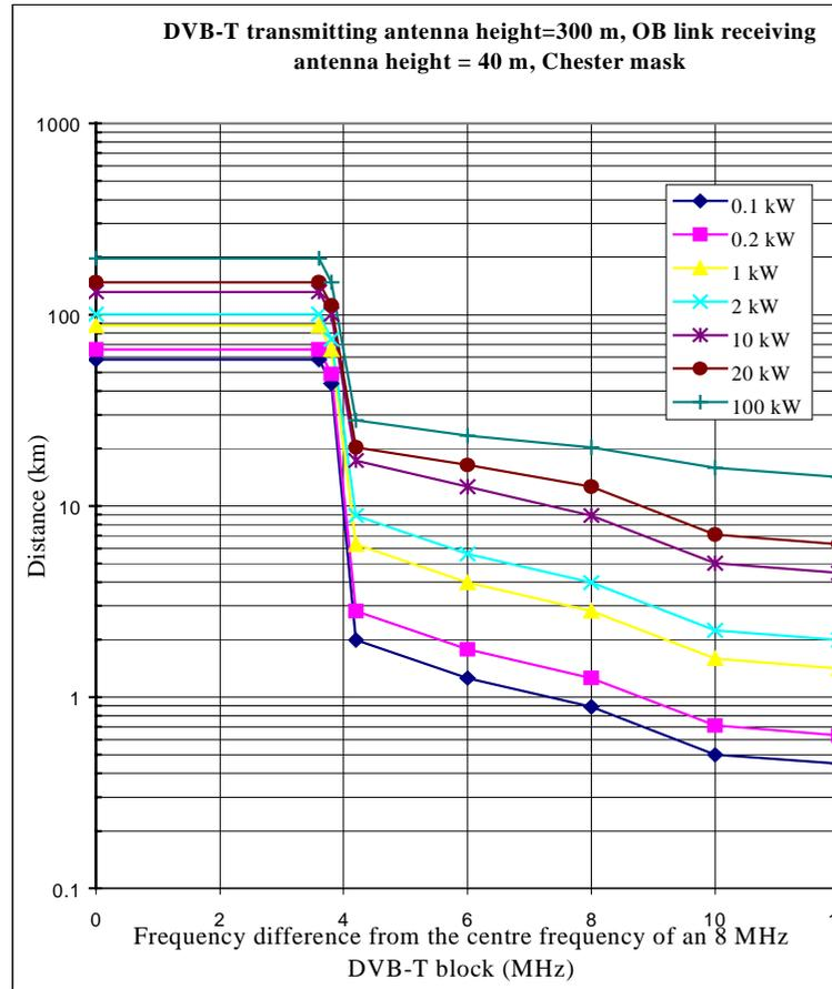
**Necessary separation distances in km between DVB-T and OB links in bands IV and V**
