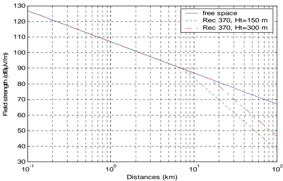
Figure A1.2: Extrapolation between the free space model and the Rec ITU-R P.370-7 model (figure 11) for a reception antenna height of 40 m
