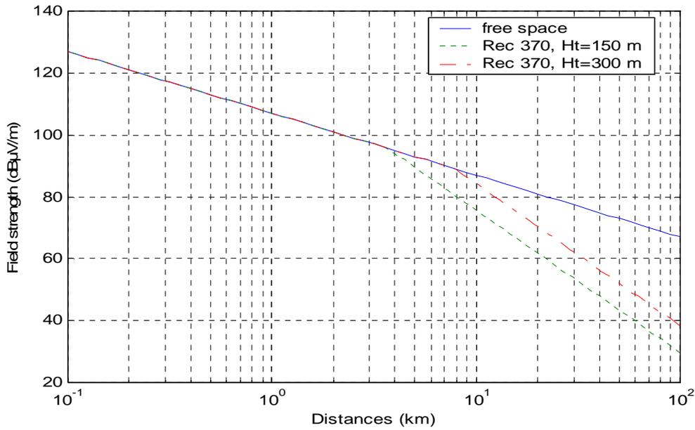
Figure A1.1: Extrapolation between the free space model and the Rec ITU-R P.370-7 model (figure 11) for a reception antenna height of 10 m
