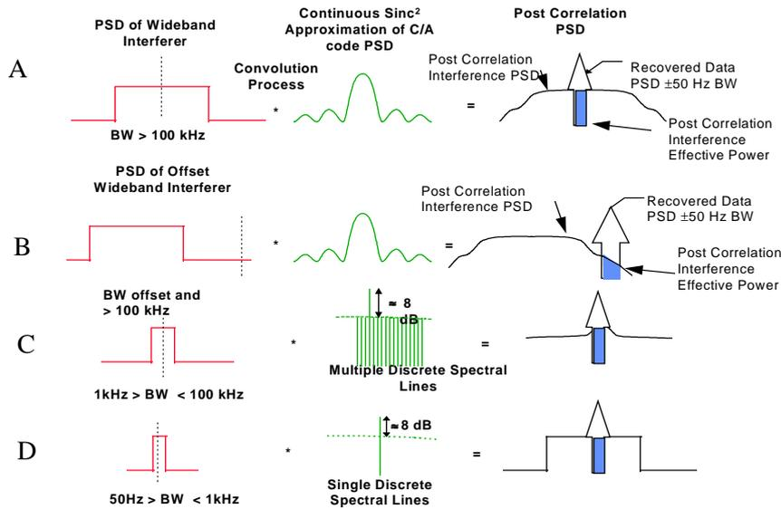
Figure A 1.2: Model of Correlation for varying Interfering Bandwidth
