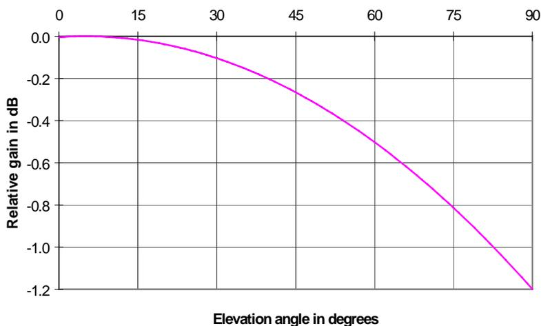
**Figure A 4.1: E-NSS-1 satellite antenna pattern**
