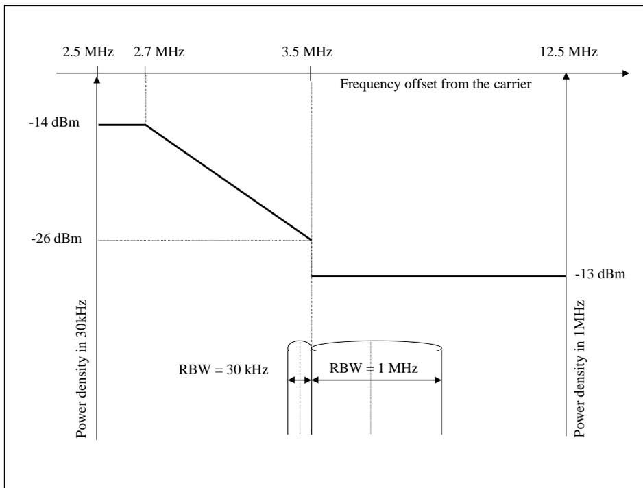
**Figure A2 – BS Spectrum emission mask measured in 30 kHz bandwidth**
