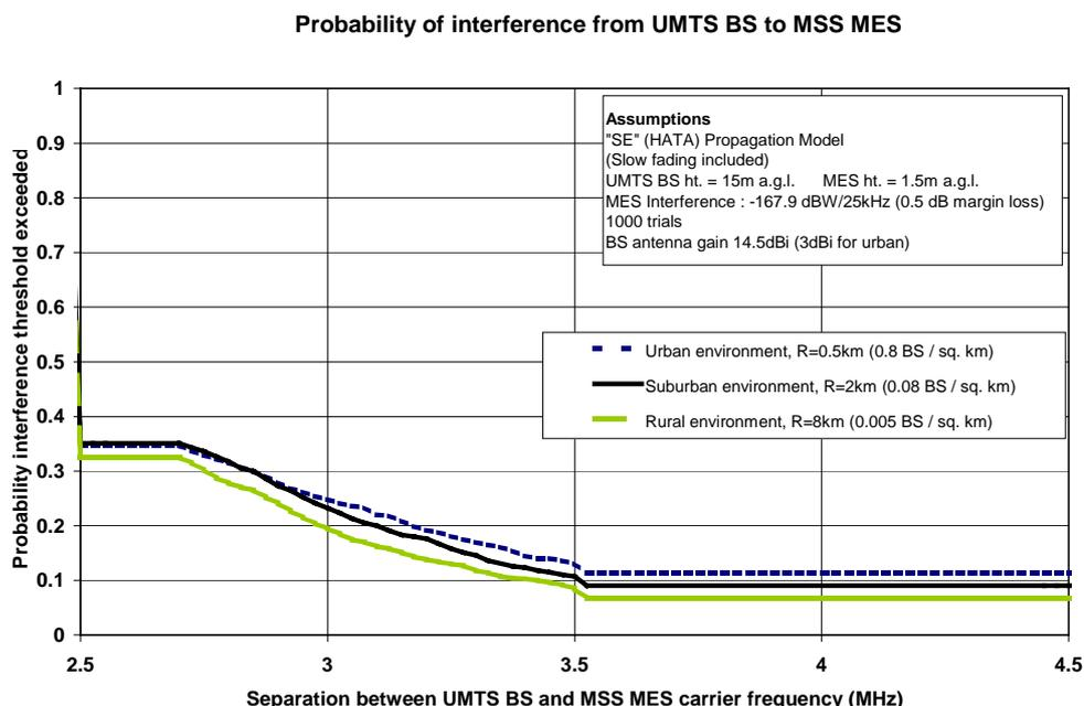
**Figure 6 – Probability of MES receiver interference as a function of carrier frequency separation**
