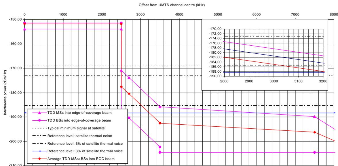
**Figure 3 - Interference power at a satellite receiver from the TDD mode of terrestrial UMTS used to provide limited area indoor coverage**
