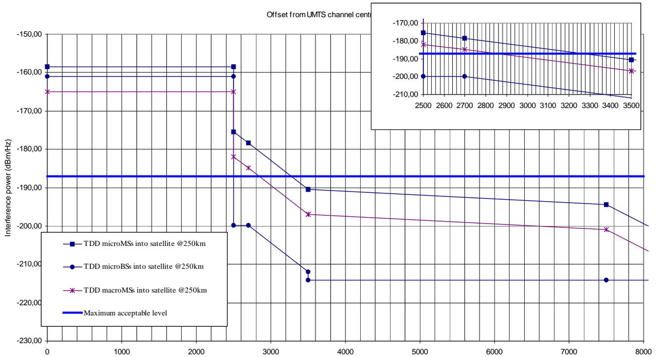
Figure 8 – Aggregated interference power at a spacecraft coming from the TDD mode of terrestrial UMTS
