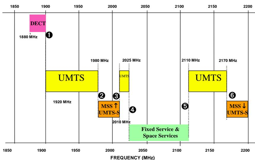
Figure 1 - European frequency plan for the 2 GHz band
