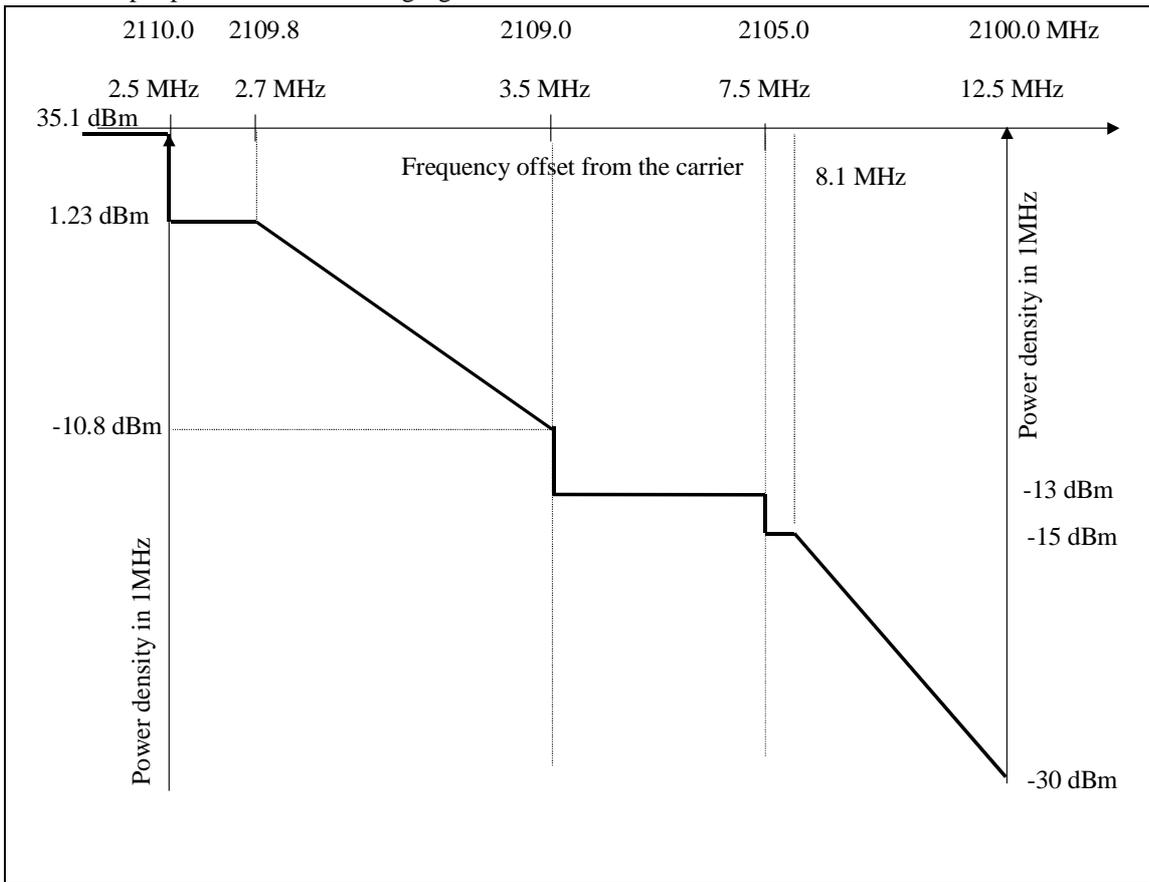
Figure A3 - Equivalent BS emission mask for a BS with 41 dBm output used in the compatibility studies at 2110 MHz.
