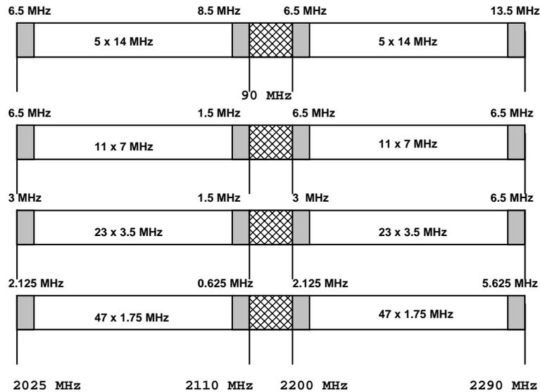
**Figure D3 - Channel arrangement for the Fixed service in the band 2025-2110 MHz paired with 2200-2290 MHz**
