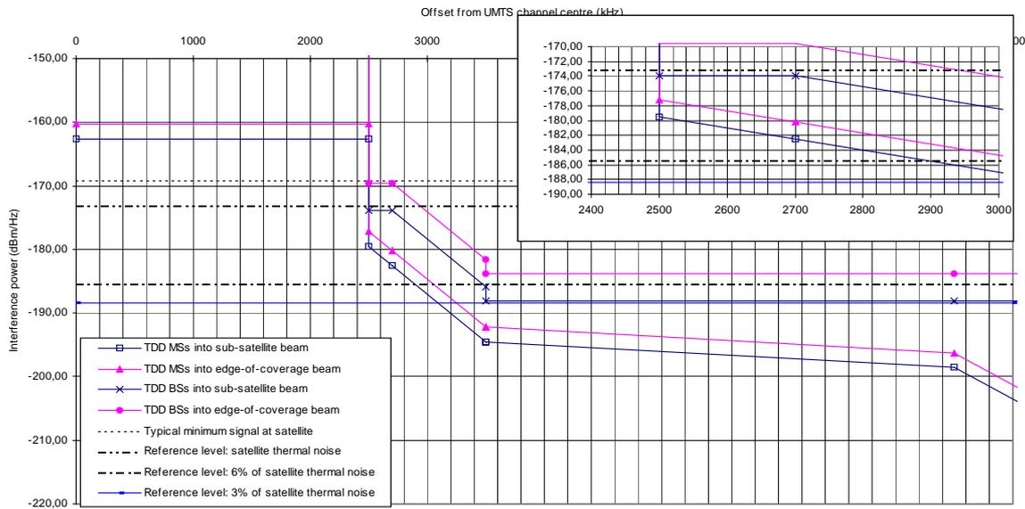
**Figure 4 - Interference power at a satellite receiver from the TDD mode of terrestrial UMTS used to provide outdoor coverage**
