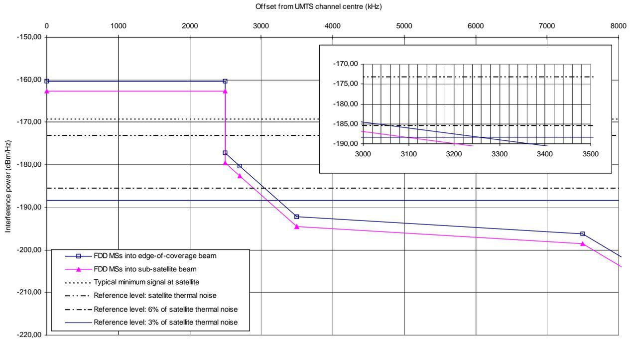
Figure 2 – Calculation of aggregate interference at satellite receiver from the FDD mode MSs of terrestrial UMTS
