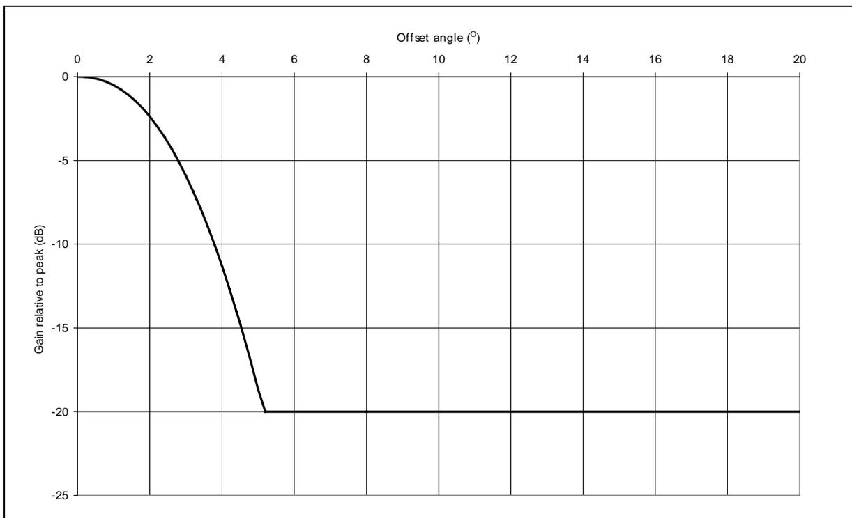
**Figure A6 - Satellite Beam Antenna Gain**
