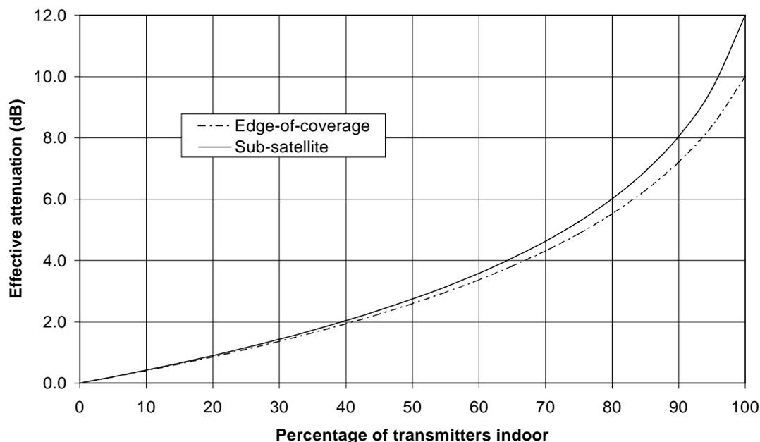
**Figure 5 - Variation of effective attenuation with percentage of transmitters indoor**
