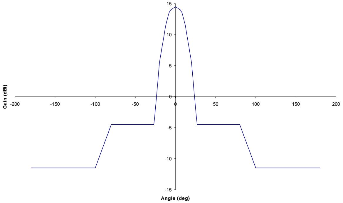
**Figure A4 – Base Station antenna pattern**
