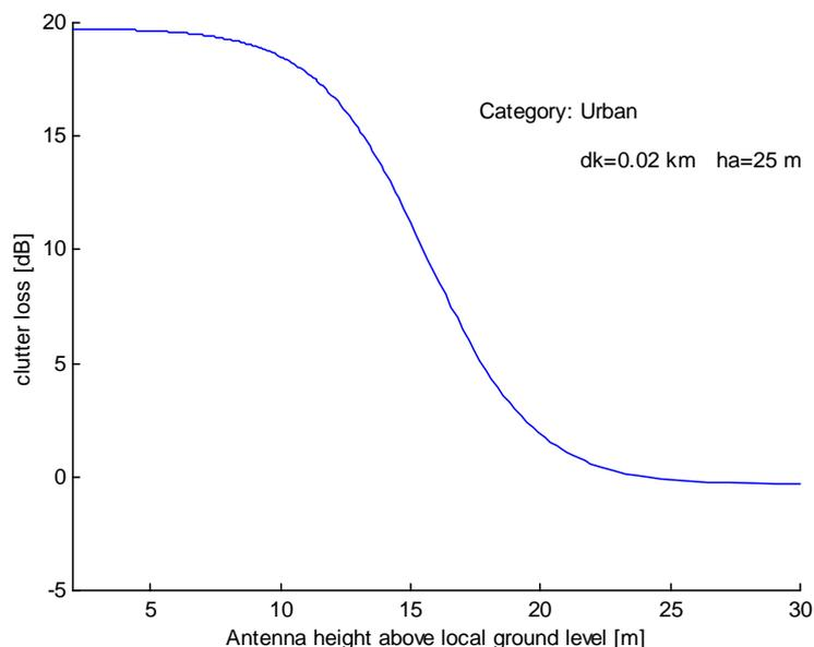
Figure D2 – Average loss due to clutter loss vs antenna height
