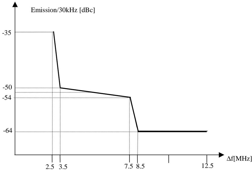
**Figure A1 - UMTS Mobile Station (or UE : User Equipment) spectrum mask**
