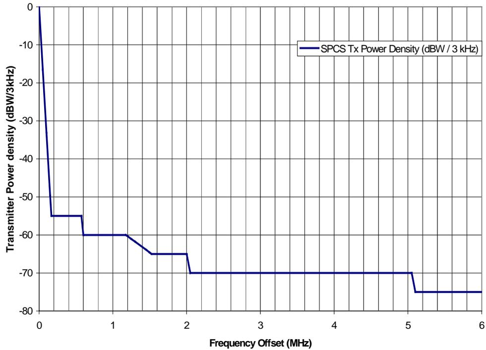
**Figure A5 - 2 GHz S-PCN out-of-band mask**
