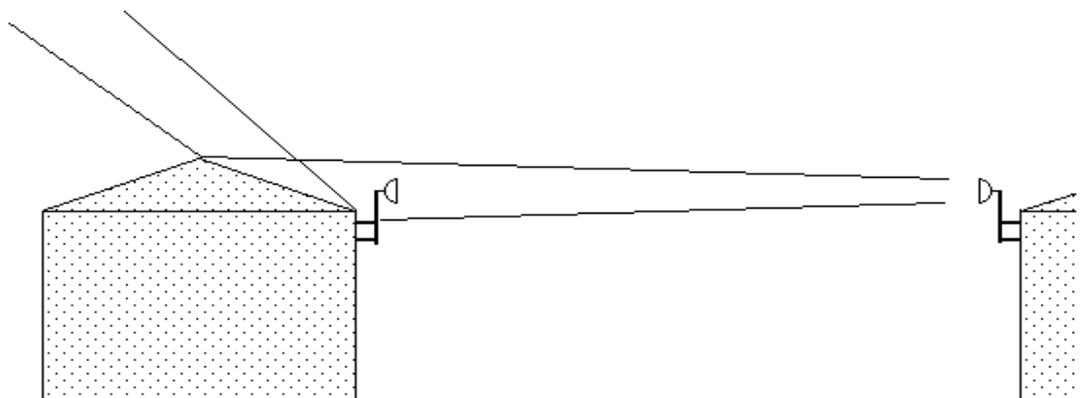
**Figure 1: Reflections of fixed link transmissions from a pitched roof**
