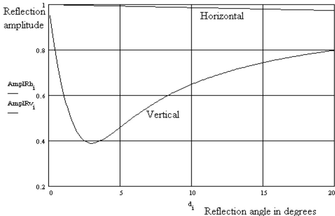
**Figure 2: Reflection amplitudes for vertical and horizontally polarised signals**
