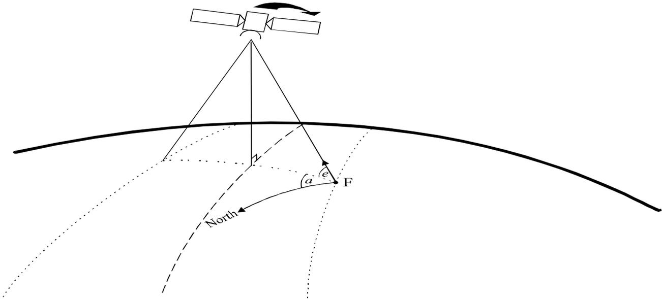
**Figure 2: Relationship between satellite sensor and Fixed Service transmitter**
