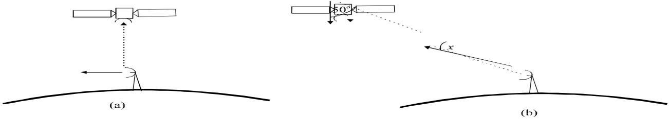
**Figure 4: Interference paths between a fixed link and a satellite**
