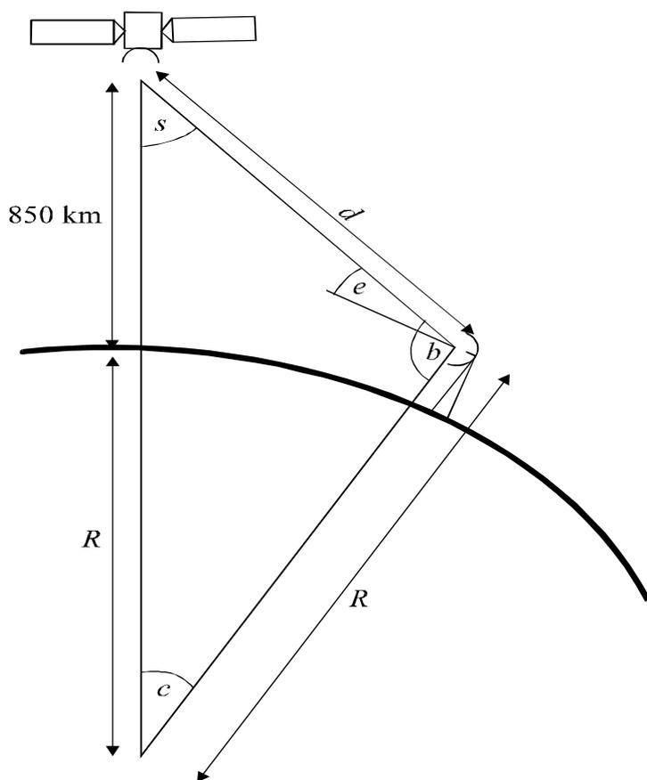
**Figure 3: Geometrical relationship between satellite and Fixed Service transmitter**
