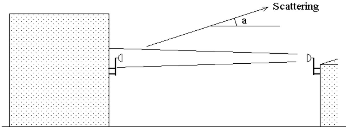
**Figure 3: Scattering from vertical surfaces**
