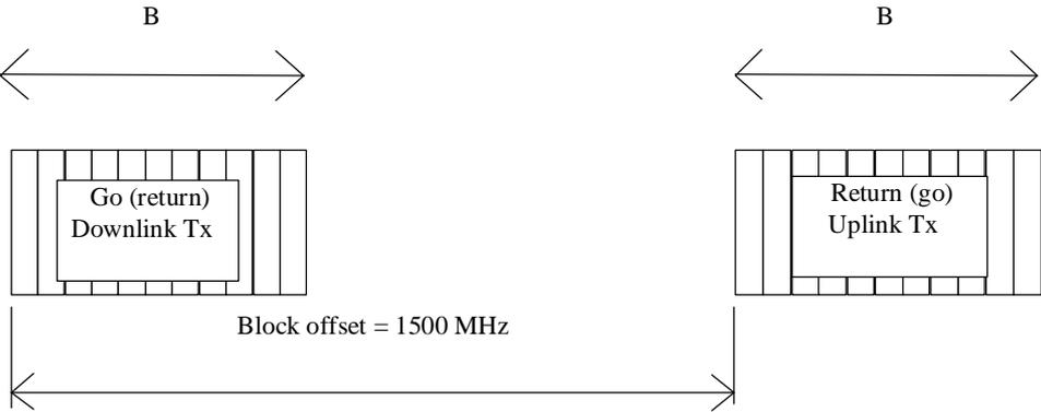
Figure 3: Application with FDD P-P and P-MP symmetric systems (for one operator)
