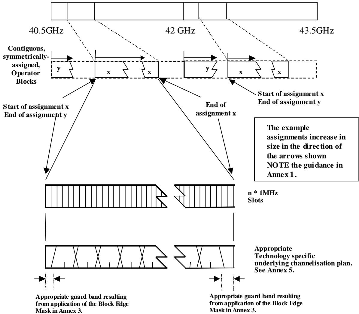
**Figure 8: Frequency plan elements**
