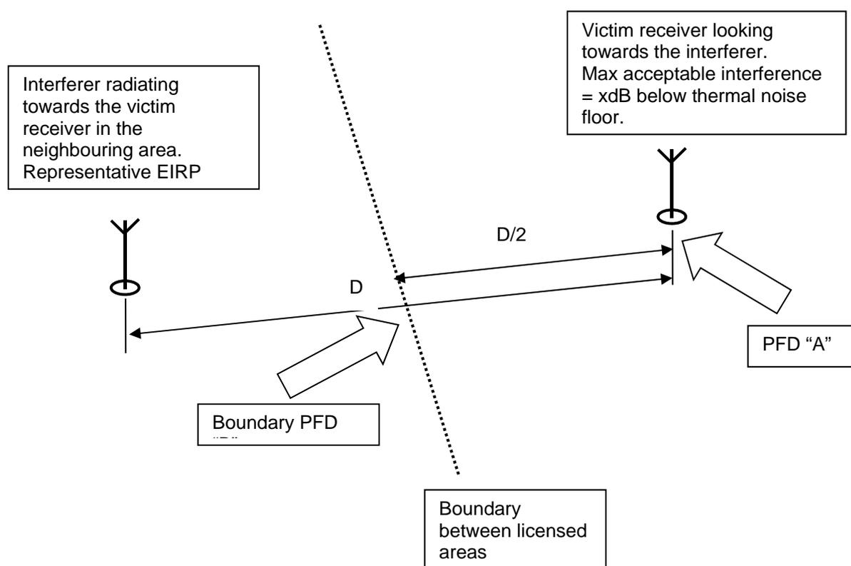
**Figure 10: Example of PFD boundary limit**
