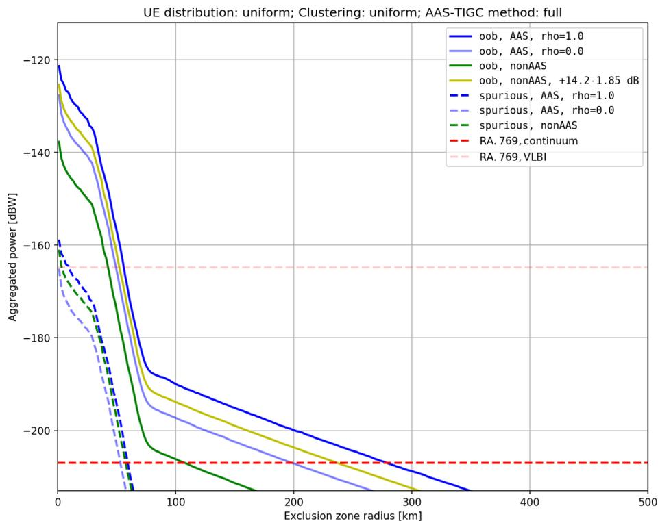
**Figure 76: Aggregated power vs. coordination zone radii, deployment: uniform, UE dist.: uniform,  $p=50\%$**
