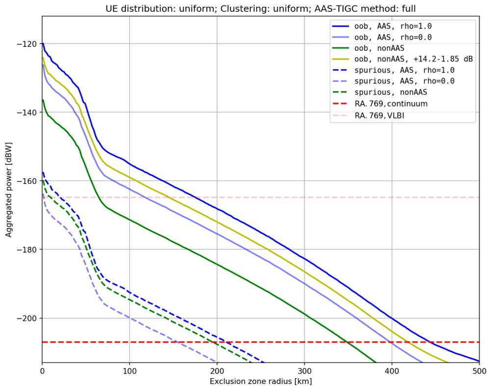
**Figure 73: Aggregated power vs. coordination zone radii, deployment: uniform, UE dist.: uniform,  $p = 2\%$**
