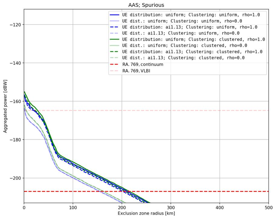
Figure 72: Aggregated power vs. coordination zone radii, AAS, spurious,  $p = 2\%$
