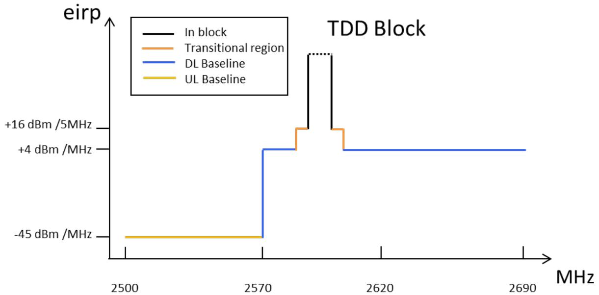
**Figure 8: Combined BEM elements for synchronised TDD blocks / downlink only blocks for non-AAS**
