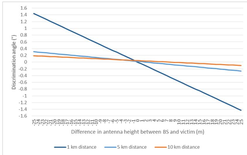
**Figure 25: Discrimination angles between BS and victim for difference in antenna height between BS and victim**
