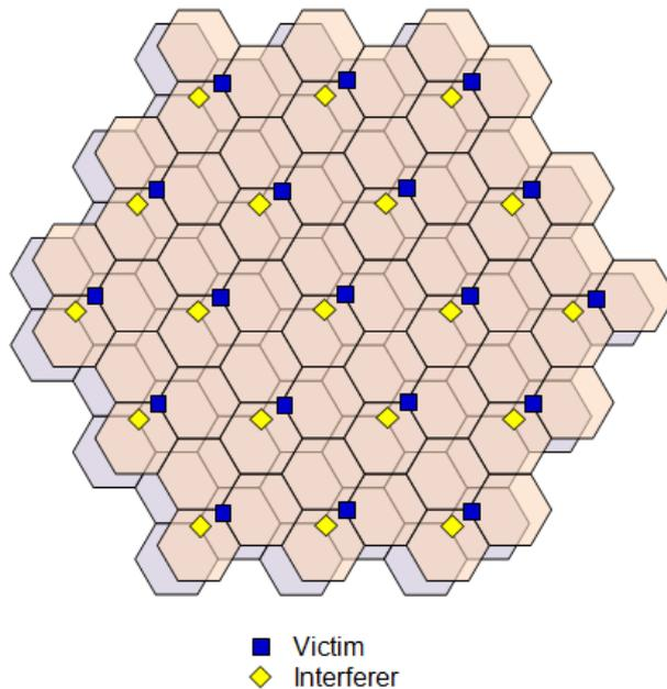
**Figure 17: Interferer-victim separation of 70 metres**
