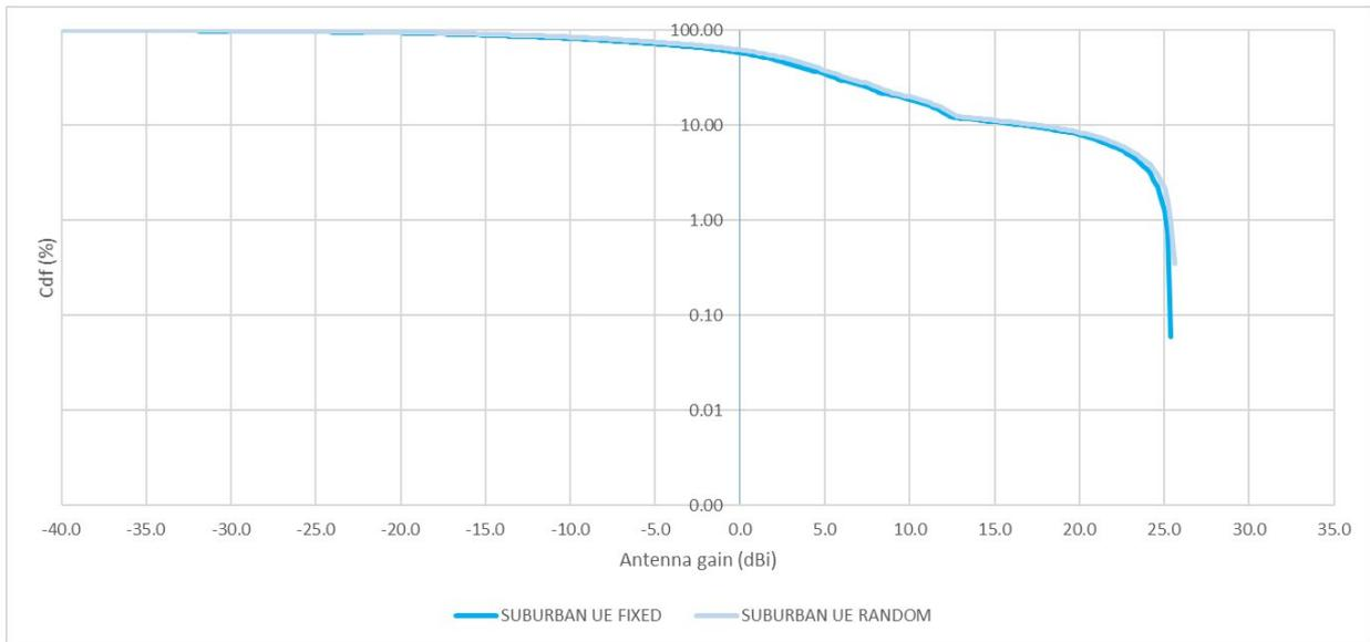
**Figure 42: AAS antenna gain towards radar for fixed UE height and random height distribution for suburban case**
