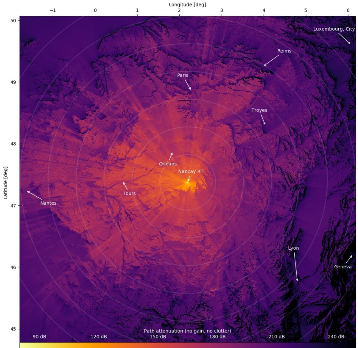
**Figure 83: Attenuation map around Nançay radio telescope in France**
