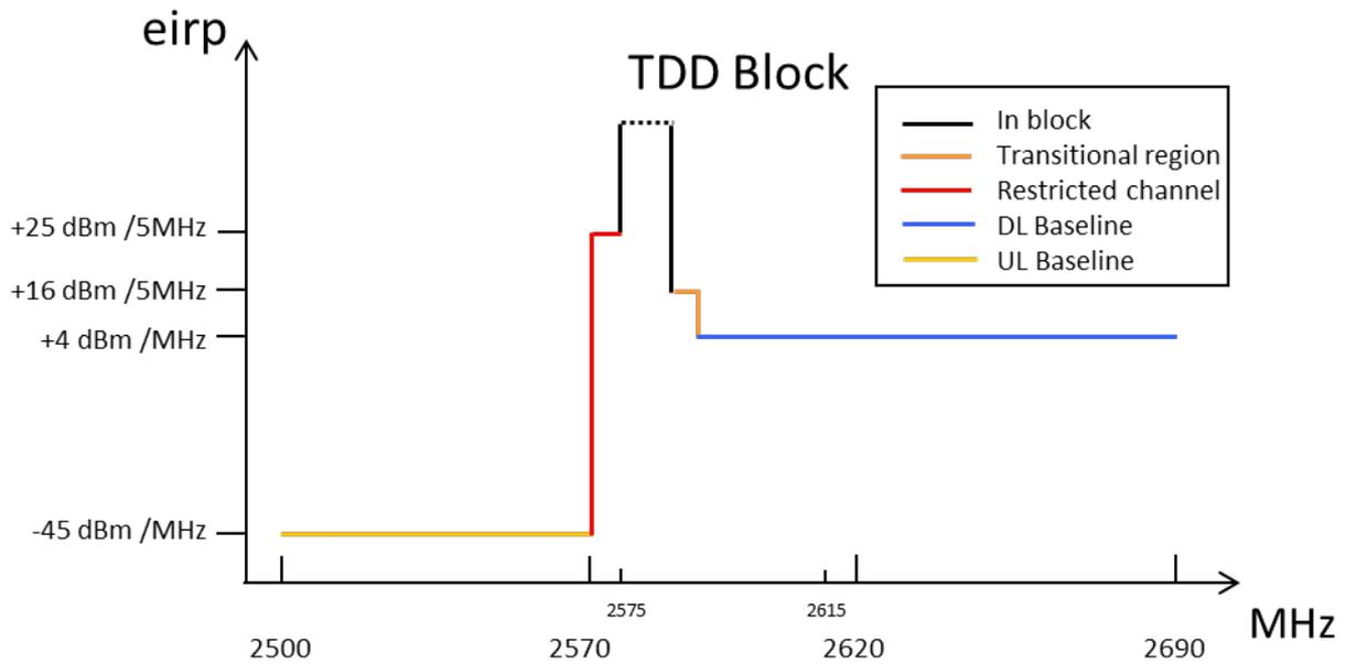
**Figure 10: Combined BEM elements for synchronised TDD/downlink only blocks and a restricted spectrum block in 2570-2575 MHz for non-AAS**
