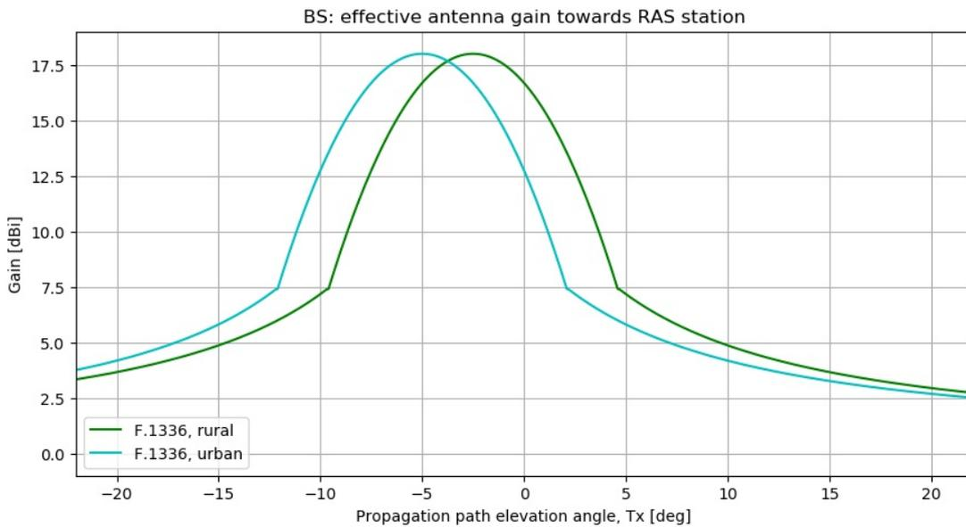
**Figure 80: Effective 4G non-AAS antenna gain as a function of propagation path elevation angle**
