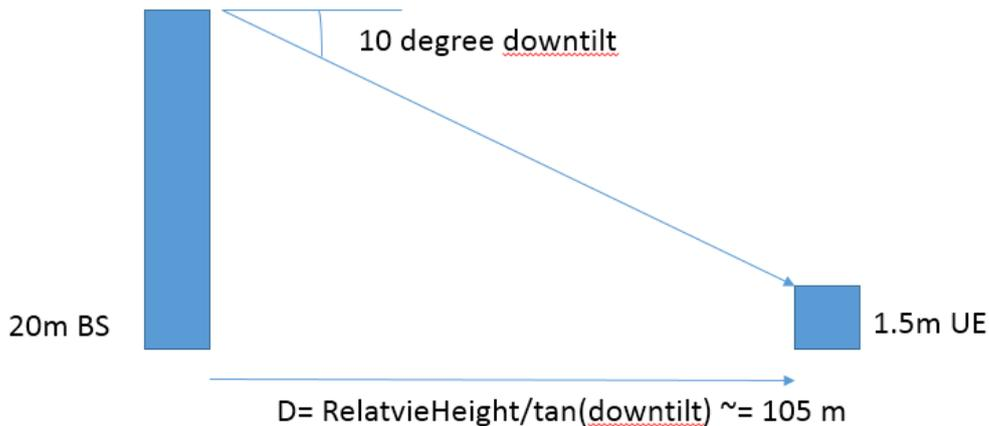
**Figure 59: Cell center for antenna with 10 degree downtilt and BS height of 20 m**
