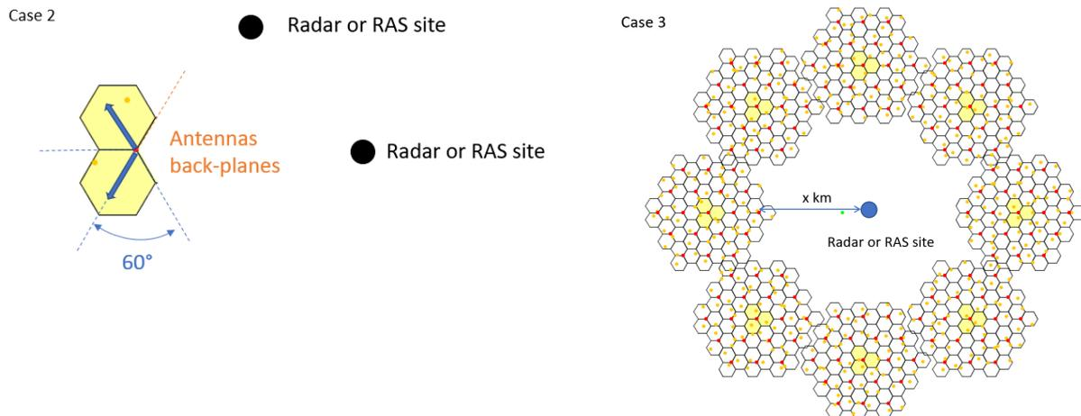
**Figure 4: Case 2 with cellular BS sectors not towards radar within  $\pm 60$  degree of boresight. Case 3 with cellular ring/grids around radar/RAS sites**
