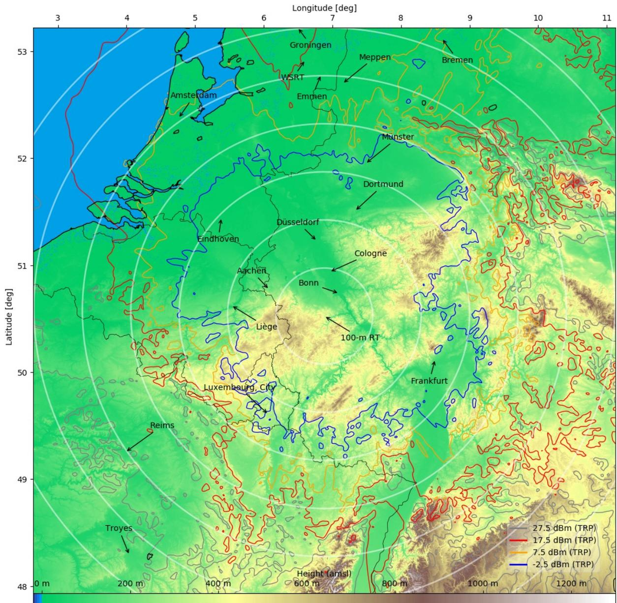
**Figure 88: Proposed coordination zones (OOB, 5G AAS) around 100 m telescope in Effelsberg, Germany**
