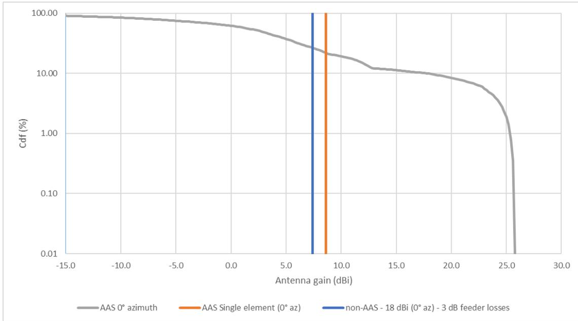
Figure 30: Antenna gain comparison (suburban case at 0° azimuth)
