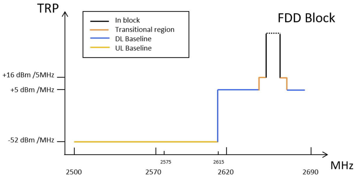
**Figure 12: Combined BEM elements for an FDD block with TDD (synchronised/unsynchronised) networks within 2570-2620 MHz for AAS**
