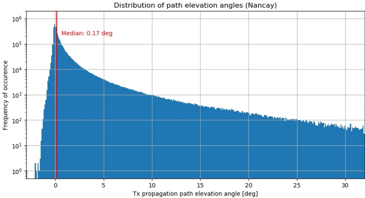
**Figure 95: Histogram of propagation path elevation angles (Tx) around Nançay observatory**
