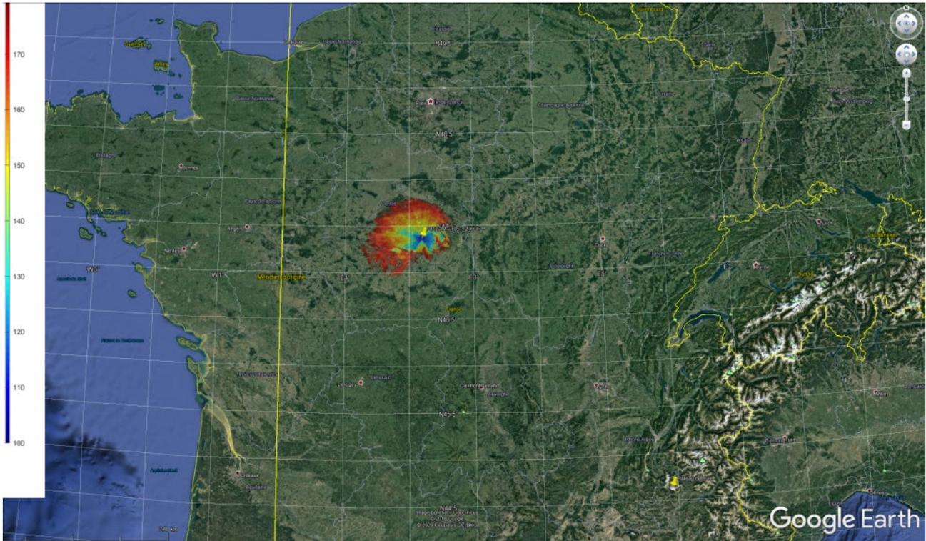
**Figure 104: Propagation Losses at 50% around the radio astronomy site of Nançay. Limited to 180 dB of losses (180 dB is exceeded outside of red colour – No colour)**
