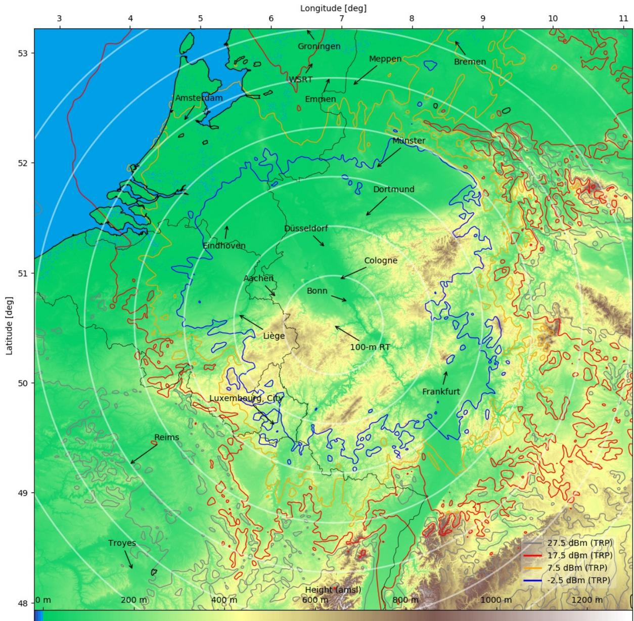
**Figure 92: Proposed coordination zones (OOB, 4G non-AAS) around 100 m telescope in Effelsberg, Germany**
