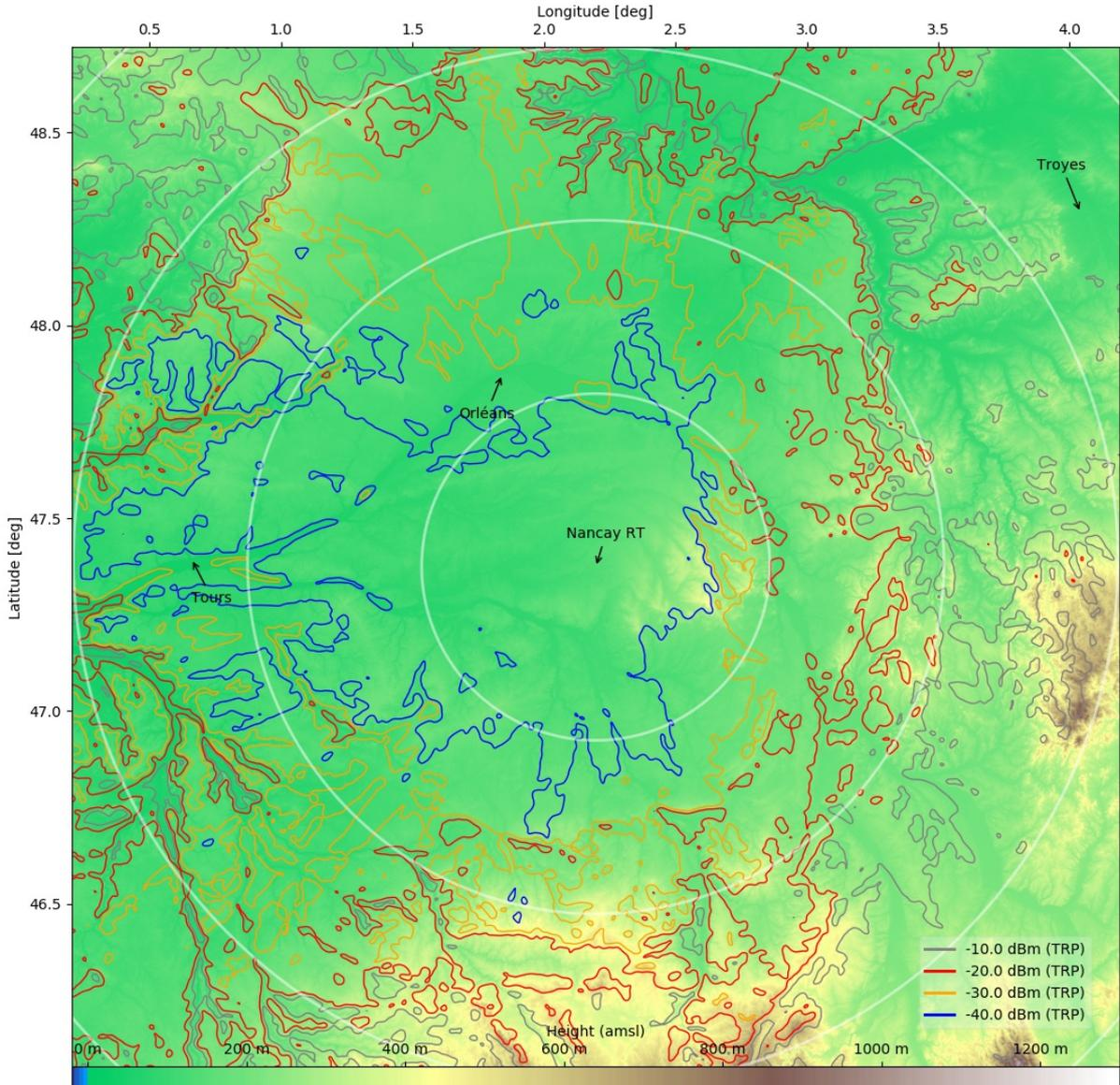
**Figure 87: Proposed coordination zones (spurious, 5G AAS) around Nancay radio telescope in France**
