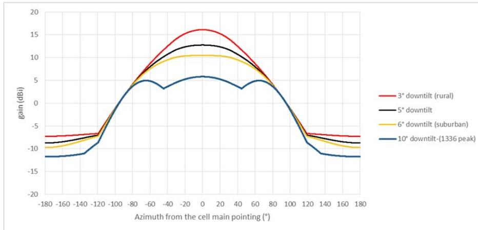
**Figure 27: Antenna gain for non-AAS in horizon as a function of azimuth and different antenna downtilts**
