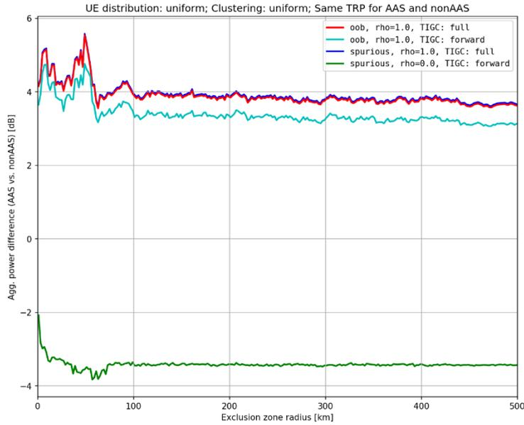
**Figure 74: Difference in aggregated power between AAS and non-AAS as a function of distance for various scenarios**
