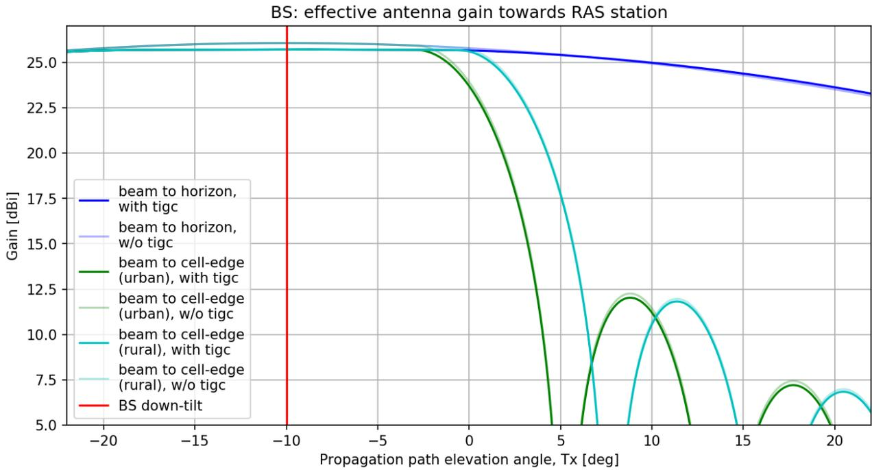
**Figure 94: Effective antenna gain change due to limiting the max. beam elevation to cell edge**
