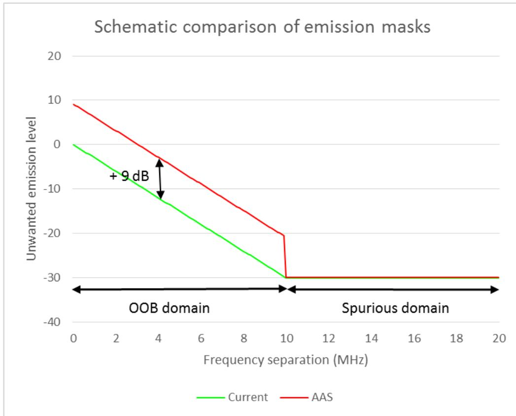
**Figure 34: Schematic comparison of unwanted emission masks for the current non-AAS case with proposed AAS case**
