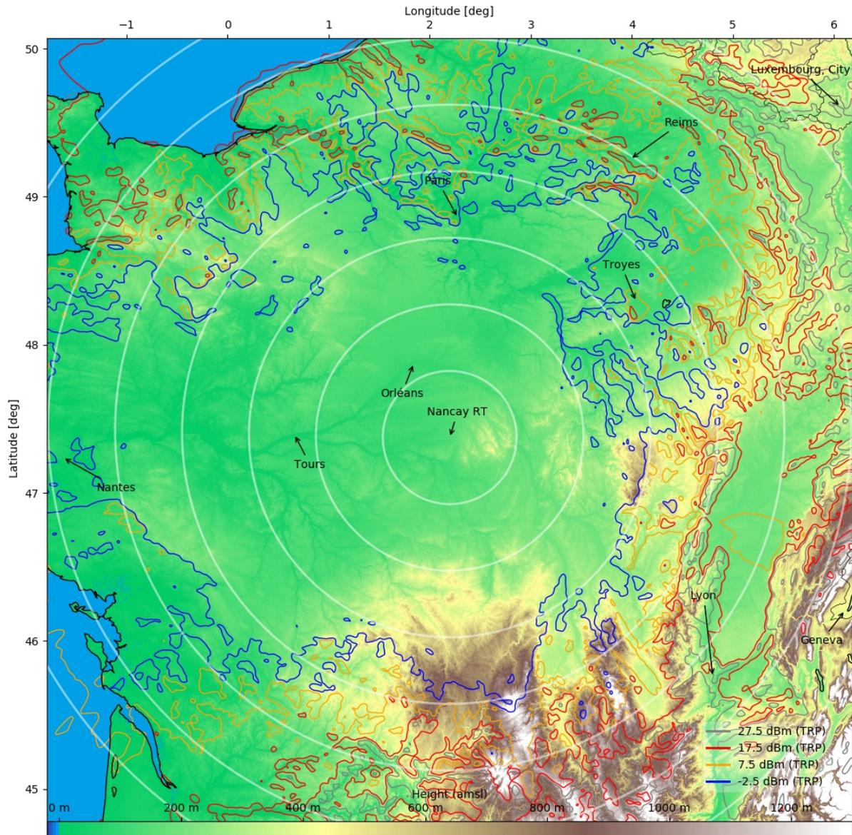
Figure 86: Proposed coordination zones (OOB, 5G AAS) around Nançay radio telescope in France
