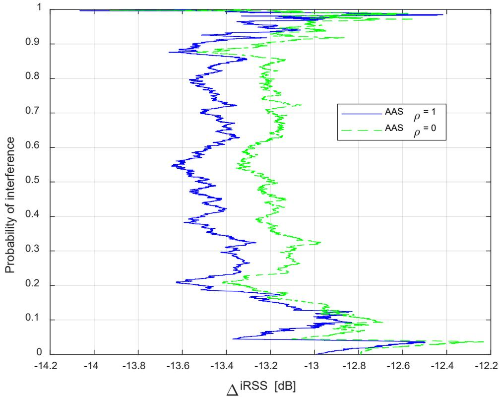
**Figure 51: Probability of interference for  $\Delta iRSS$  for realistic case of ring/grid around radar station with distance separation  $\sim 5$  km. Macro rural case single UE per snapshot and full RB allocation for  $\rho = 1$  and  $\rho = 0$ . The fluctuation of about  $\pm 0.5$  dB is within the accuracy in the simulation with the chosen #of of snapshots**
