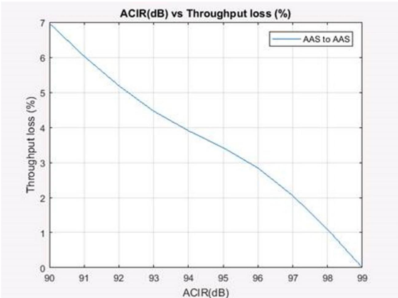
**Figure 19: Impact of AAS base station to AAS base station interference**
