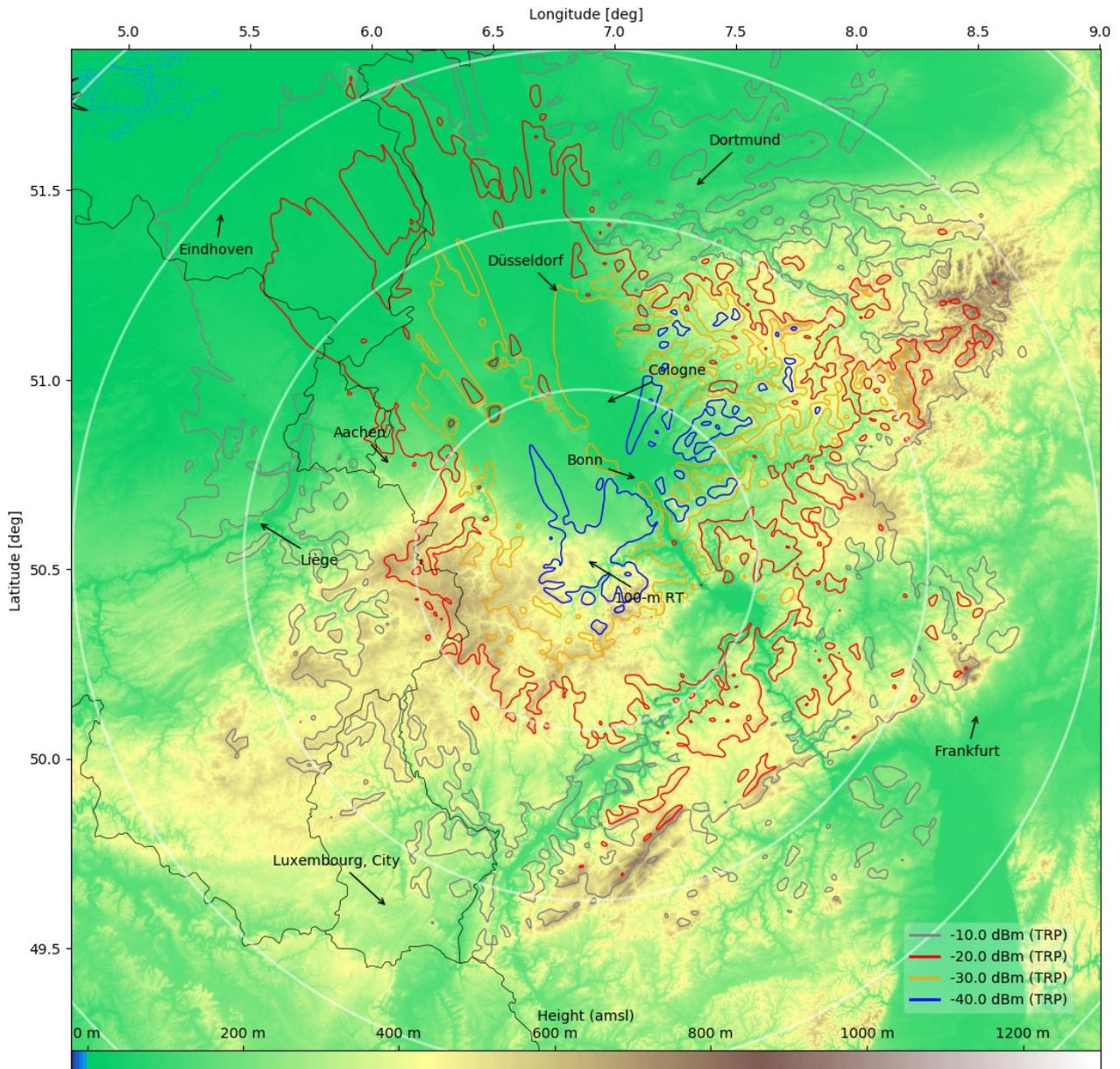
**Figure 89: Proposed coordination zones (spurious, 5G AAS) around 100 m telescope in Effelsberg, Germany**
