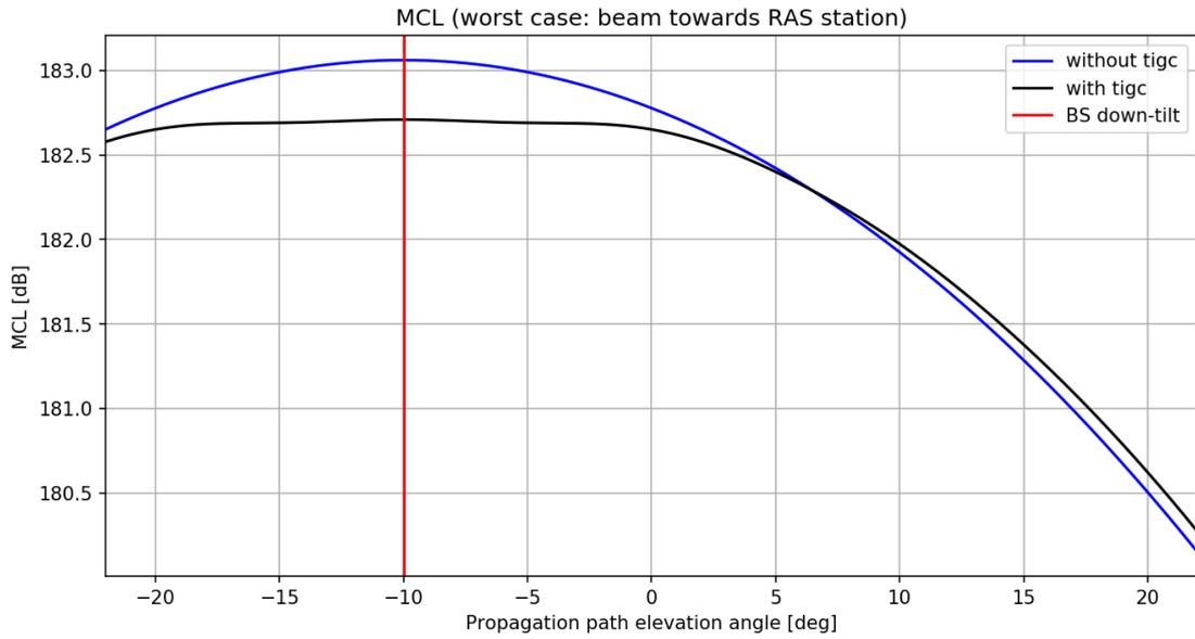
**Figure 79: MCL (spurious, 5G AAS) as a function of propagation path elevation angle**
