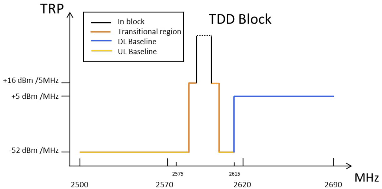
Figure 14: Combined BEM elements for unsynchronised TDD blocks for AAS
