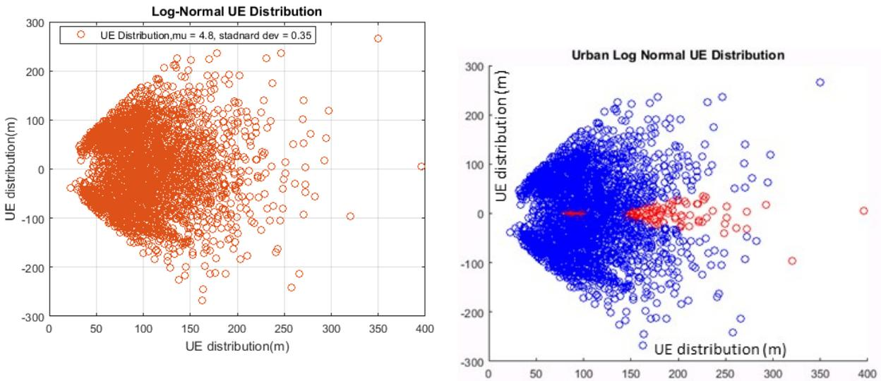
**Figure 61: (left) Urban scenario log-normal UE distribution; (right) Location of the 5% top AAS antenna gains for the Urban scenario log-normal UE distribution**
