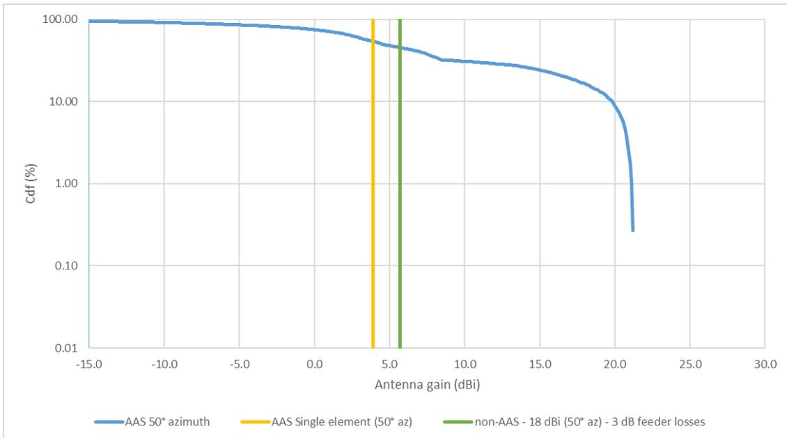
Figure 31: Antenna gain comparison (suburban case at 50° azimuth)
