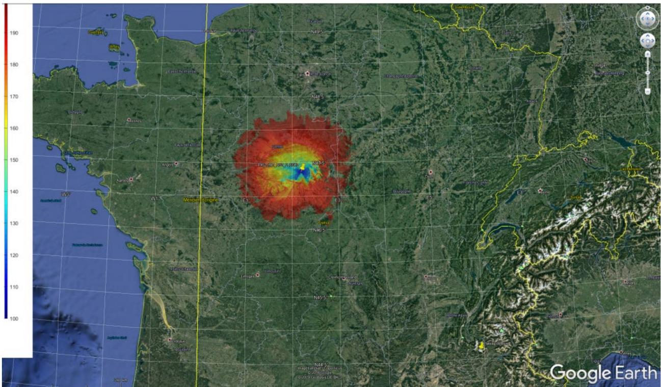
Figure 103: Propagation Losses at 50% around the radio astronomy site of Nançay. Limited to 200 dB of losses (200 dB is exceeded outside of red colour – No colour)
