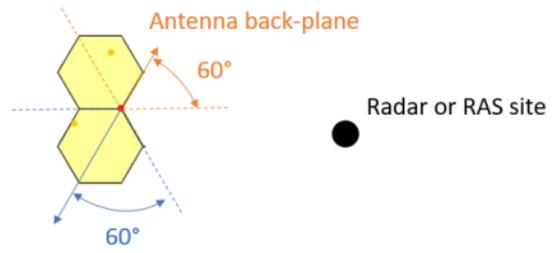
Figure 48: Case 1 with sector towards radar within  $\pm 60$  degree of boresight. Case 2 sectors not towards radar within the  $\pm 60$  degree of boresight
