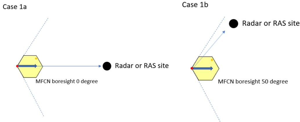
**Figure 3: Case 1 with cellular BS sector ( $\pm 60$  degree) towards radar. In (a) with BS antenna boresight 0 degree towards radar and (b) boresight 50 degrees towards radar**
