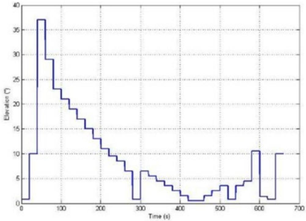
Figure 20: From ECC Report 174 "Meteorological radars, typical elevation variation over time"
