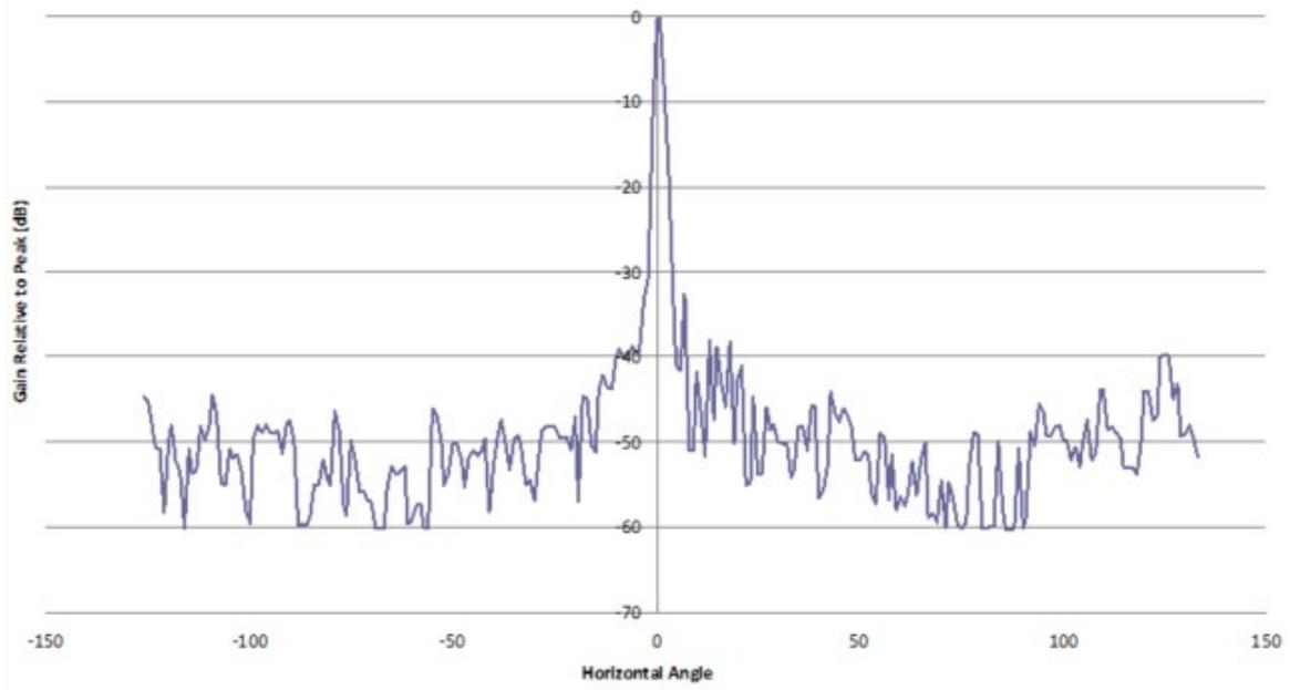
Figure 22: From ECC Report 174 "ATC radar antenna pattern in azimuth"
