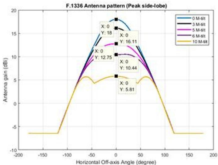
**Figure 65: Antenna pattern for non-AAS: based on F.1336-4 [22]**
