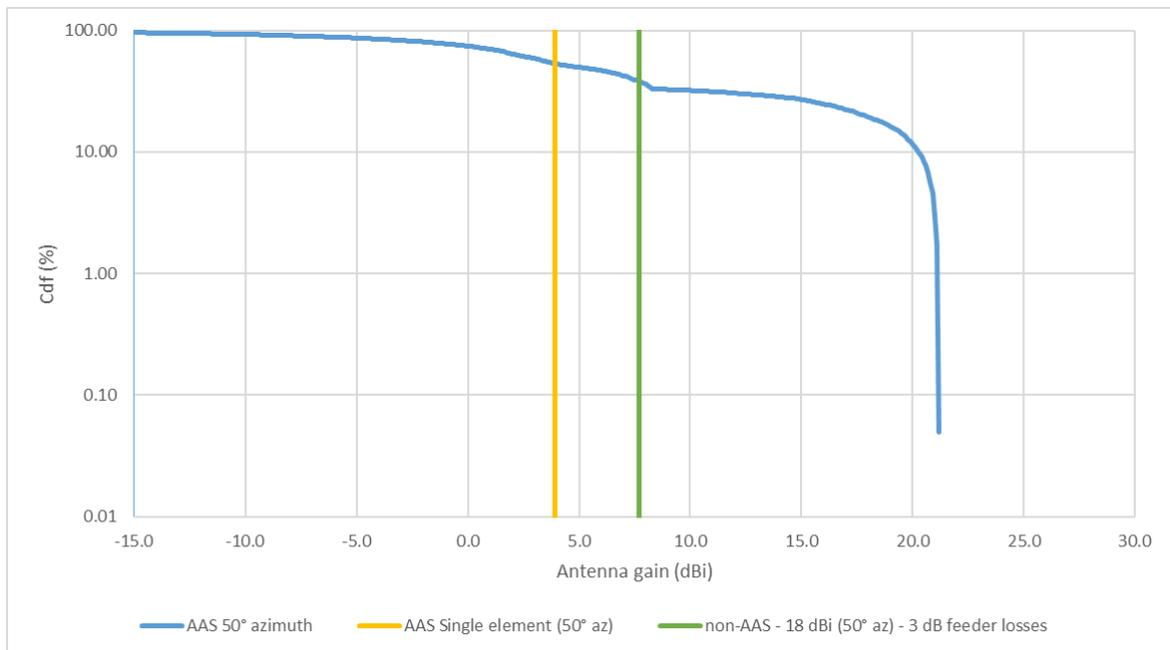
Figure 33: Antenna gain comparison (rural case at 50° azimuth)
