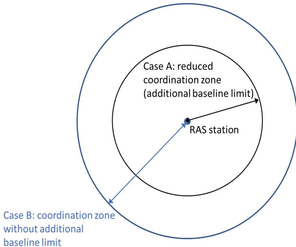
**Figure 16: Simplified example of coordination zones around RAS station for AAS base stations**
