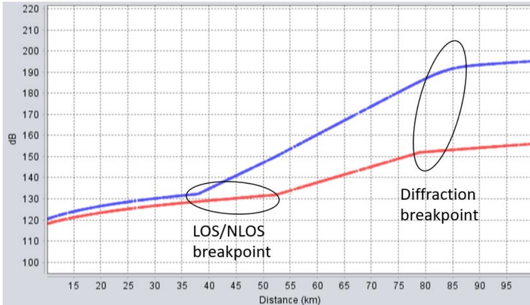
**Figure 47: Path loss versus distance for Recommendation ITU-R P.452 [24] model. For  $p_{P.452} = 2\%$  (red) and  $50\%$  (blue) with BS antenna height 30 m and RAS antenna height 50 m above ground**
