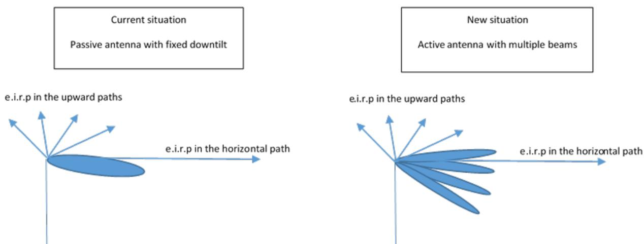
**Figure 24: Passive antenna with fixed downtilt and active antenna with multiple beams**
