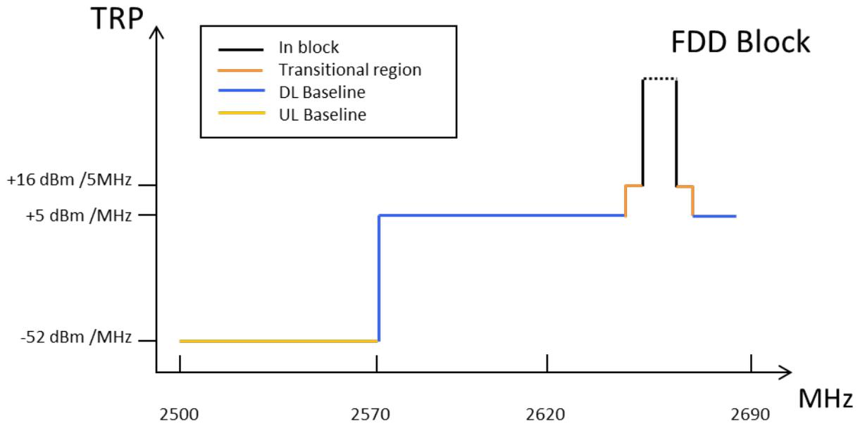
**Figure 11: Combined BEM elements for an FDD block above 2620 MHz with downlink only operation within 2570-2620 MHz for AAS**
