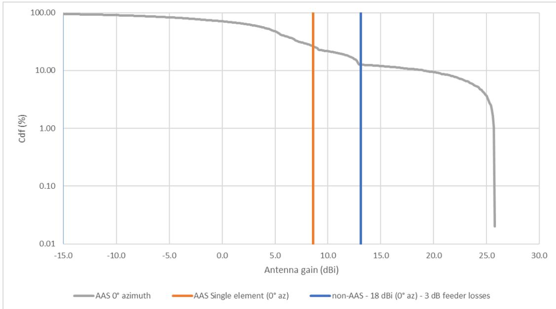
Figure 32: Antenna gain comparison (Rural case at 0° azimuth)
