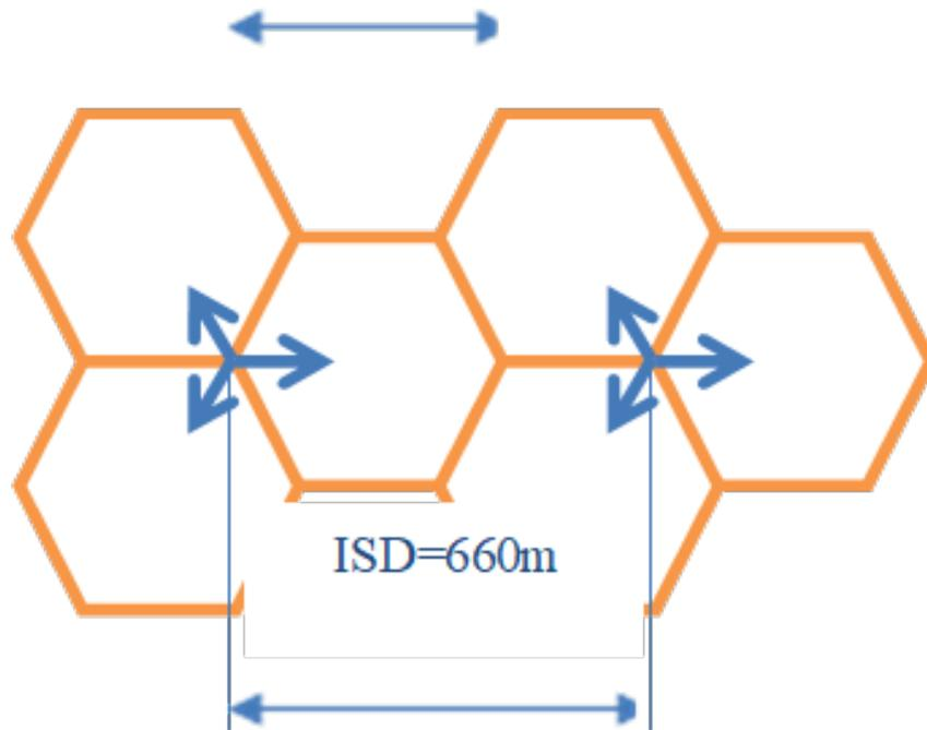
**Figure 53: Illustration of the geometry for a 3-sector deployment and defines the parameters cell**
