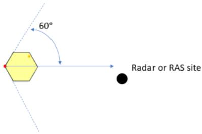
Case 2: with sectors not towards radar within  $\pm 60$  degree of boresight
