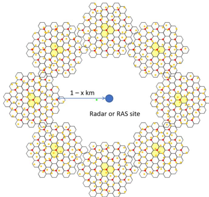
Figure 49: Case 3 Realistic case of cellular ring/grids around radar station with 8 two-tiers tri-sectors
