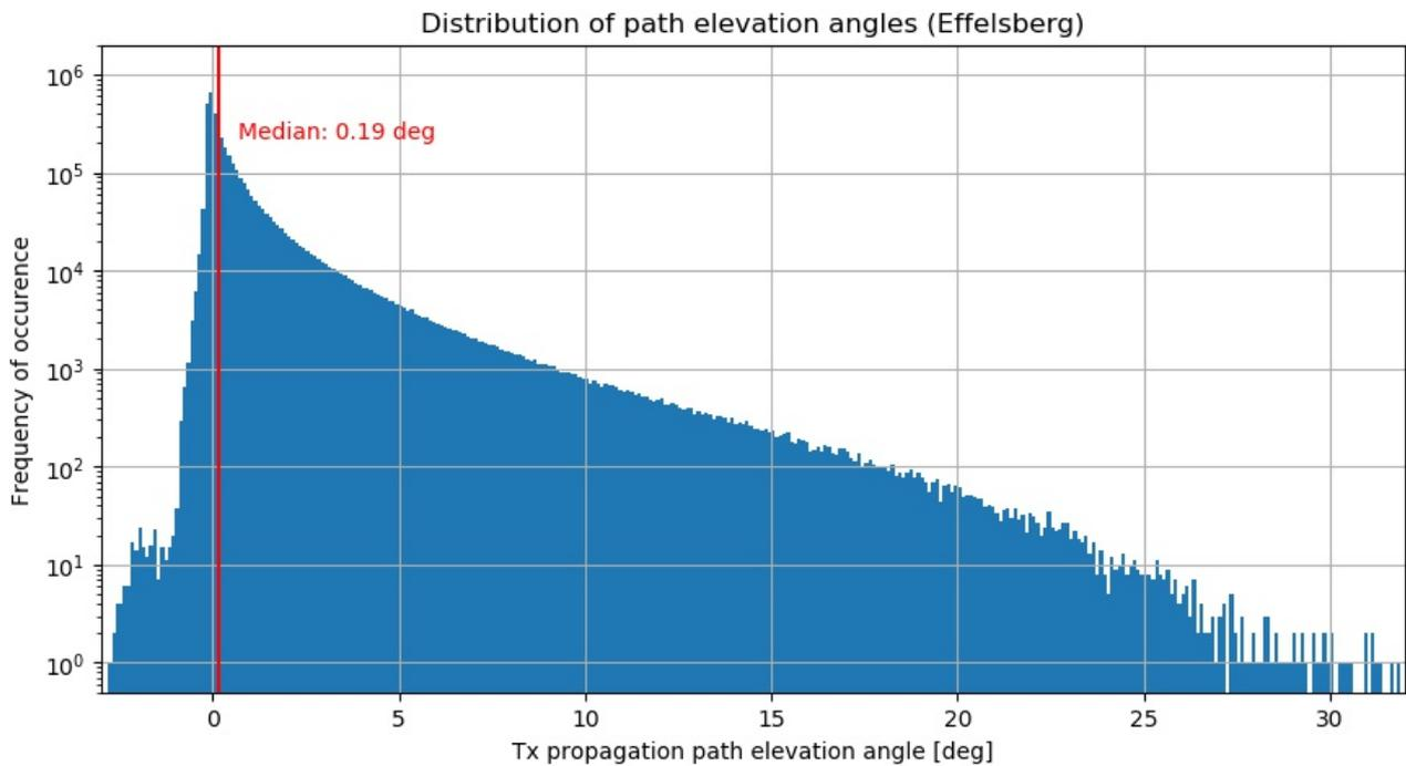
**Figure 96: Histogram of propagation path elevation angles (Tx) around Effelsberg observatory**
