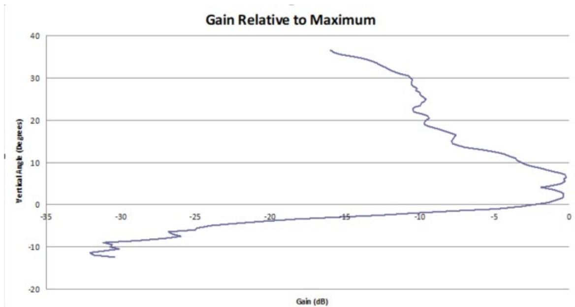
Figure 21: From ECC Report 174 "ATC radar antenna pattern in elevation"
