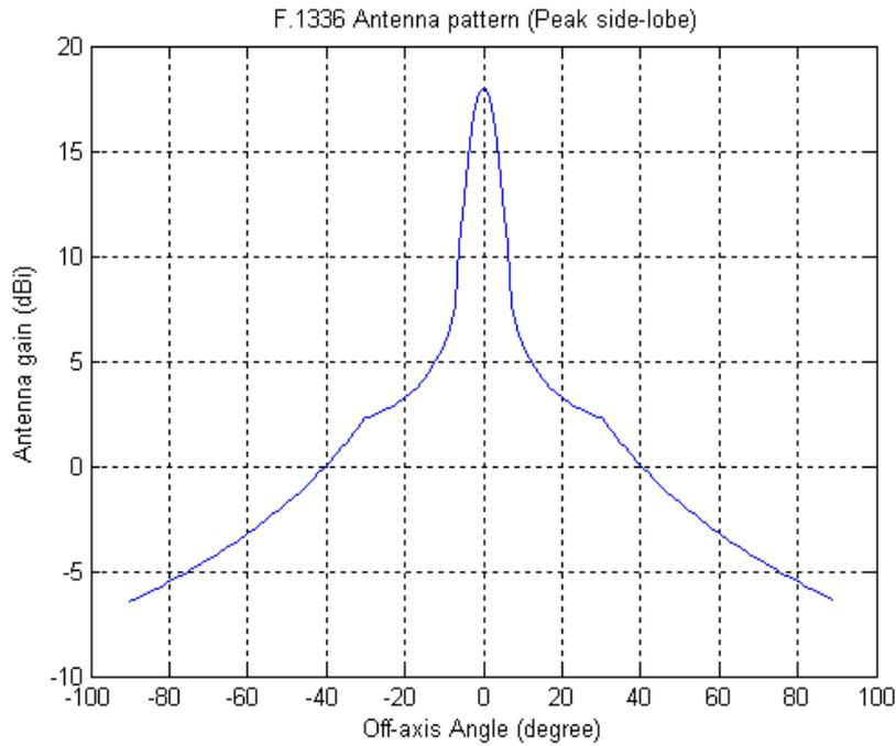
**Figure 52: Non-AAS antenna pattern based on Recommendation ITU-R F.1336-3**
