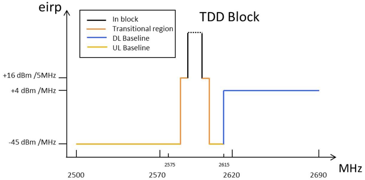
**Figure 9: Combined BEM elements for unsynchronised TDD blocks for non-AAS**
