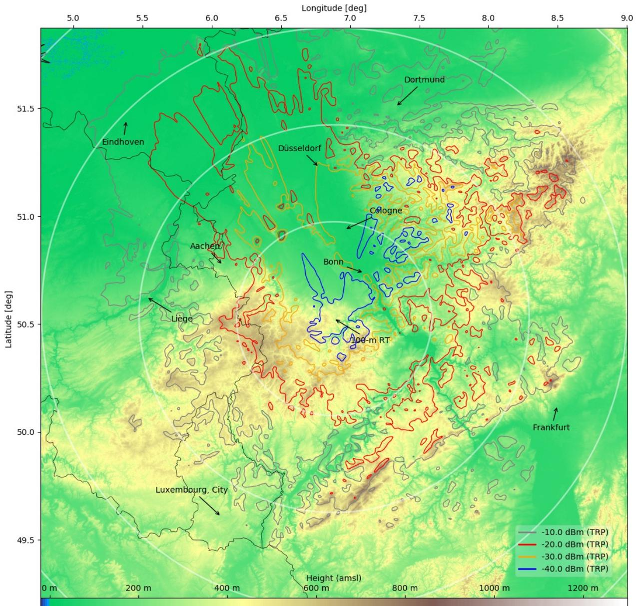
**Figure 93: Proposed coordination zones (spurious, 4G non-AAS) around 100 m telescope in Effelsberg, Germany**
