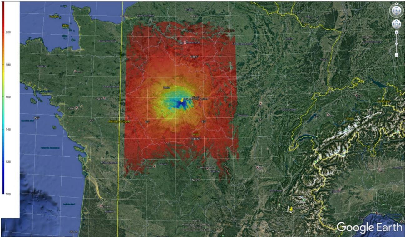
Figure 102: Propagation Losses at 50% around the radio astronomy site of Nançay. Limited to 220 dB of losses (220 dB is exceeded outside of red colour – No colour)
