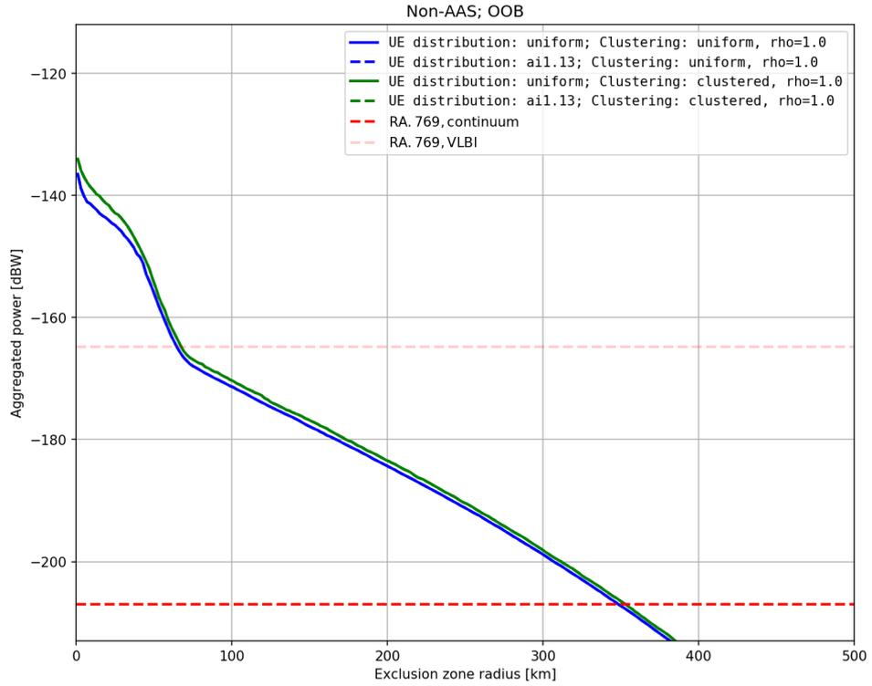
Figure 69: Aggregated power vs. coordination zone radii, non-AAS, OOB,  $p = 2\%$
