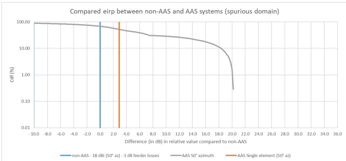
**Figure 36: Compared e.i.r.p. between non-AAS and AAS systems for urban case and 50° azimuth**
