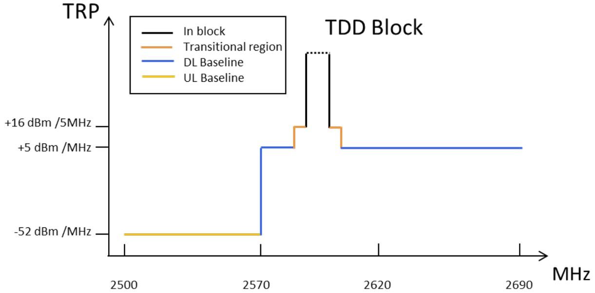
Figure 13: Combined BEM elements for synchronised TDD blocks/downlink only blocks for AAS
