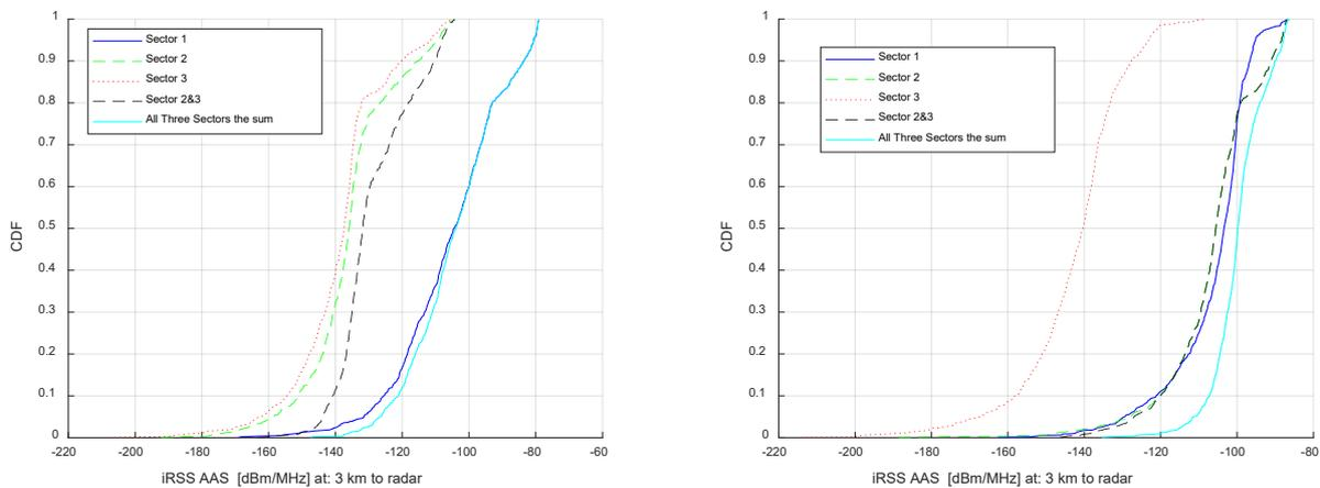
**Figure 43: Probability of  $iRSS$  for tri-sector macro urban and fully correlated case ( $\rho = 1$ ) and single UE with full bandwidth per snapshot (a) Boresight towards radar from sector 1 (b) Boresight 50 degree offset to radar from sector 1**
