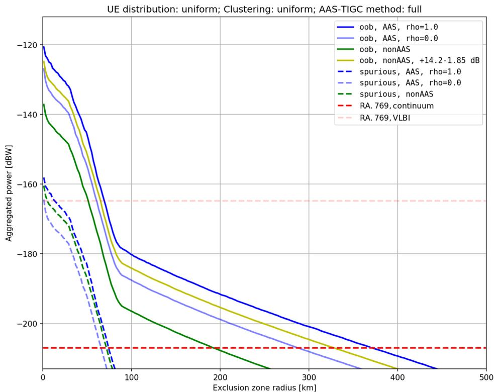
**Figure 75: Aggregated power vs. coordination zone radii, deployment: uniform, UE dist.: uniform,  $p = 10\%$**
