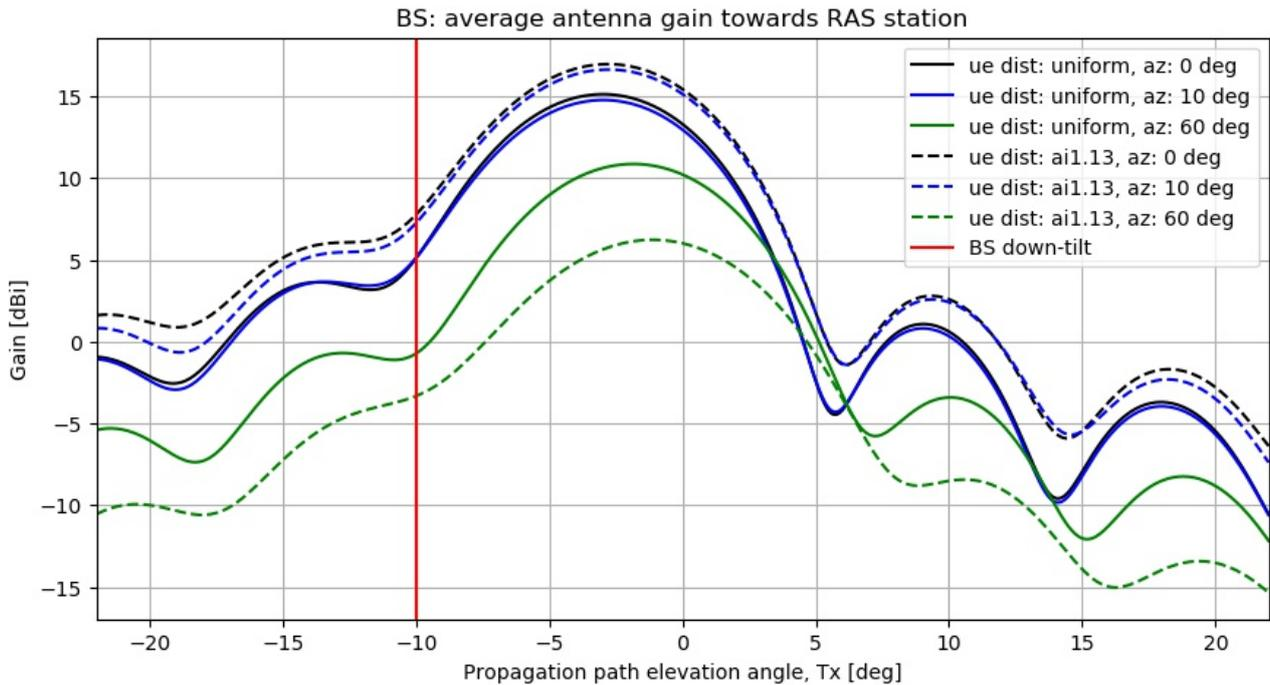
**Figure 99: Average antenna gain for three different azimuthal separation angles**
