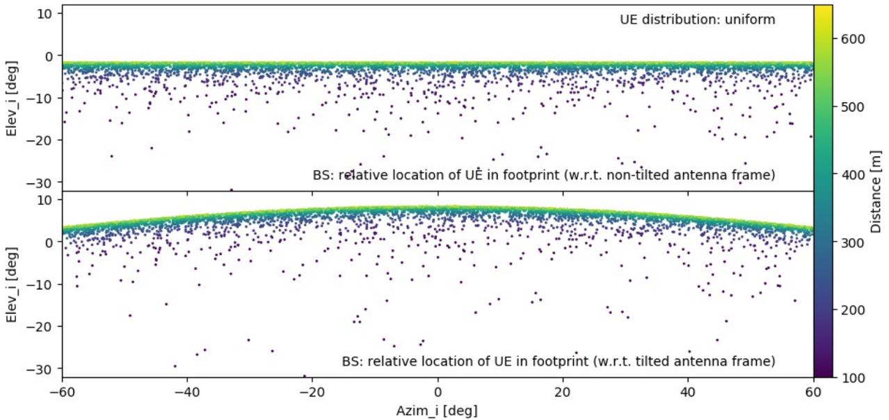
**Figure 97: UE position relative to BS antenna frame for uniform UE distribution**
