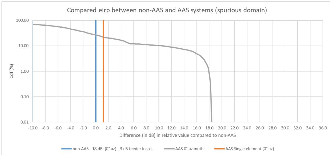
**Figure 37: Compared e.i.r.p. between non-AAS and AAS systems for suburban case and 0° azimuth**
