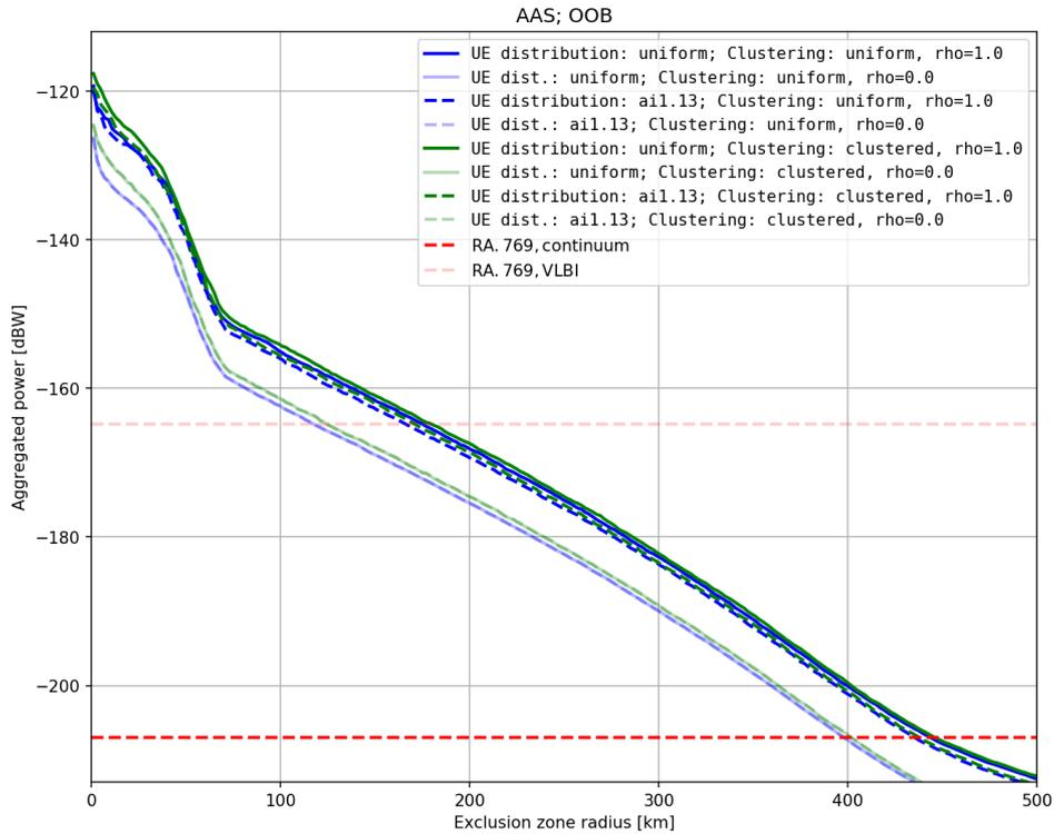
Figure 71: Aggregated power vs. coordination zone radii, AAS, OOB,  $p = 2\%$
