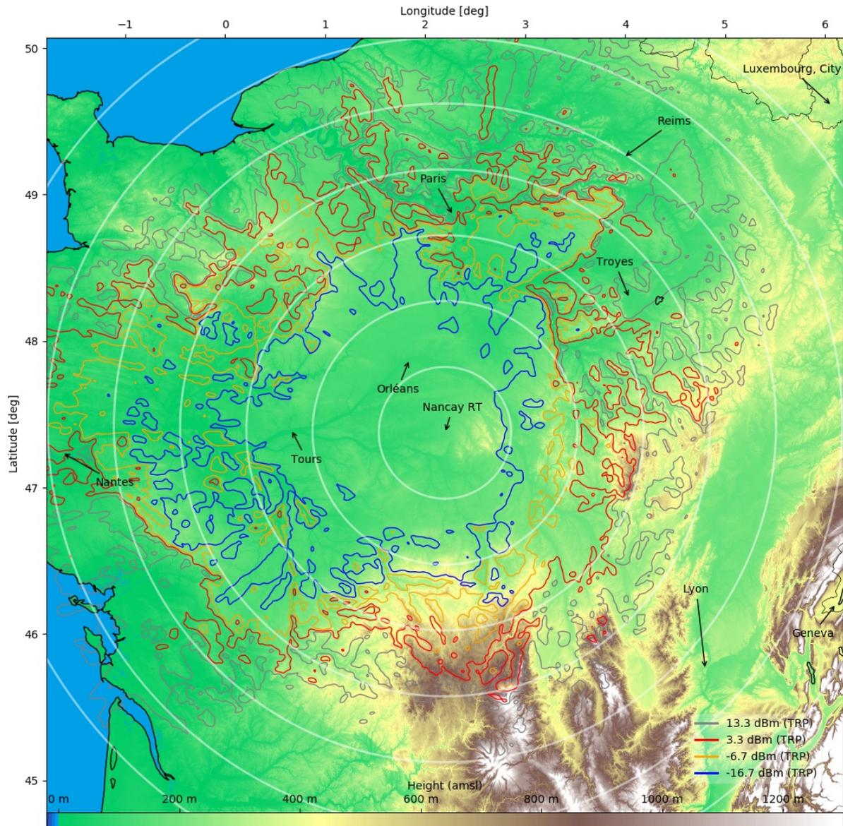
**Figure 90: Proposed coordination zones (OOB, 4G non-AAS) around Nançay radio telescope in France**
