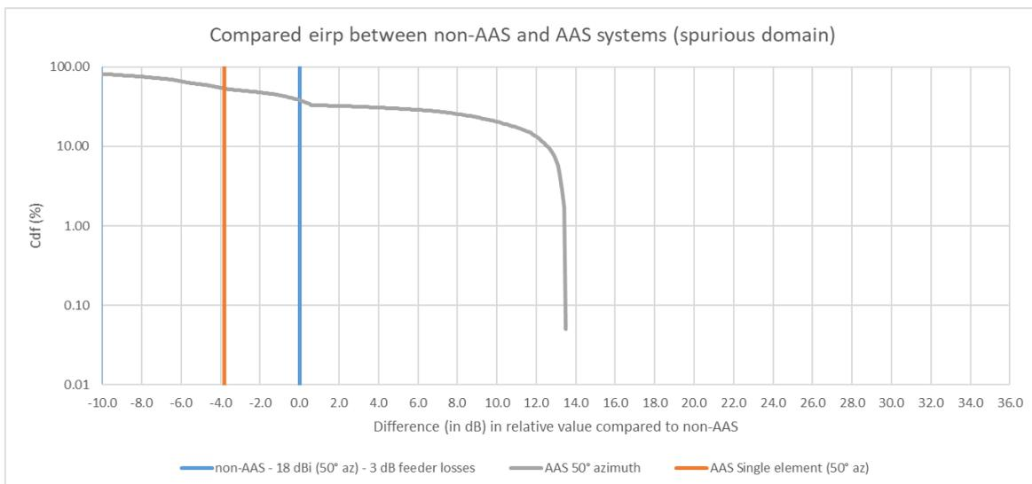
**Figure 40: Compared e.i.r.p. between non-AAS and AAS systems for urban case and 50° azimuth**
