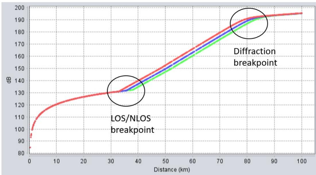
Figure 46: Path loss versus distance for Recommendation ITU-R P.452 [24]. For different BS antenna heights above ground with 20 m (red), 25 m (blue) and 30 m (green) and RAS with fixed 50 m height above ground. Showing LOS/NLOS breakpoint between 30 and 40 km and diffraction breakpoint around 75 to 85 km for these cases
