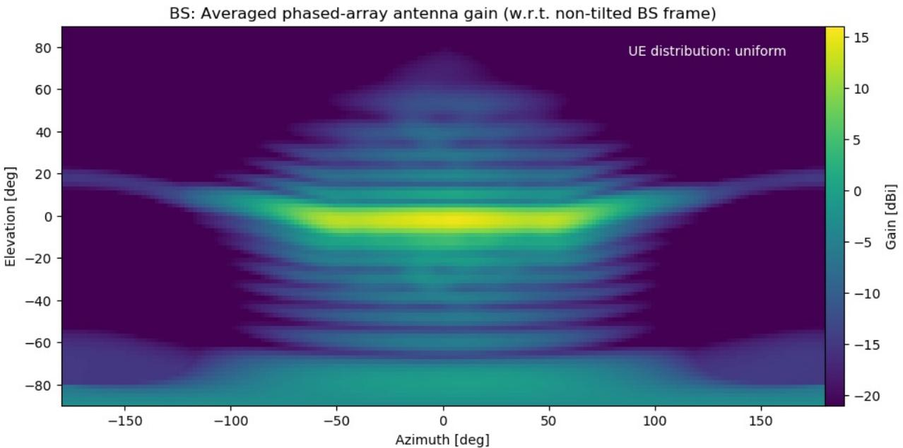
**Figure 98: Average antenna gain of AAS for the uniform UE distribution shown in Figure 97**
