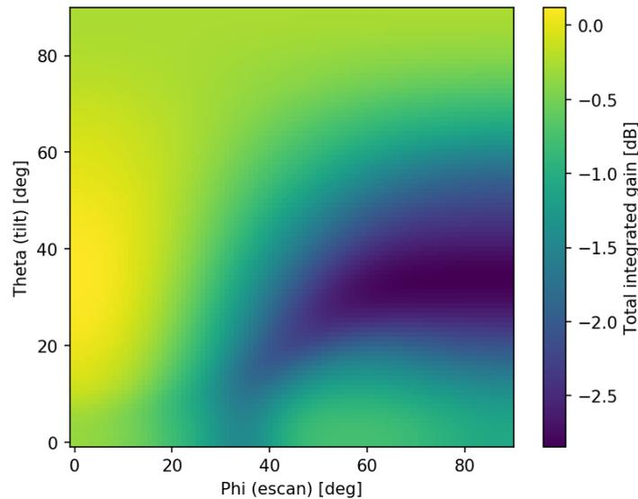
**Figure 66: Total integrated gain correction for AAS**
