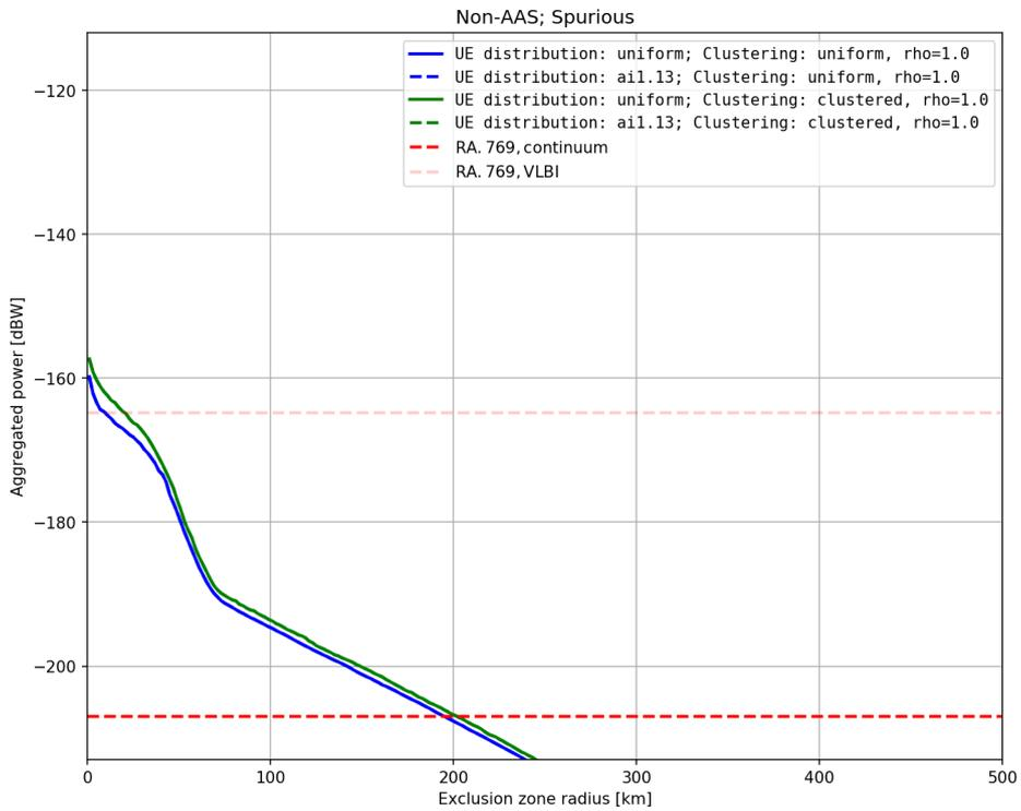
Figure 70: Aggregated power vs. coordination zone radii, non-AAS, spurious,  $p = 2\%$
