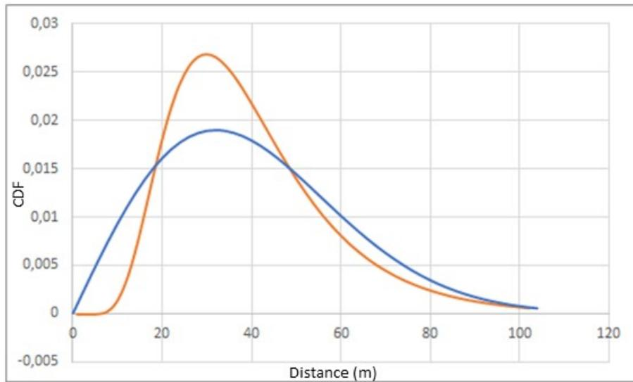
**Figure 57: TG5/1: Comparison between Rayleigh (Red curve) and Log-Normal distributions**
