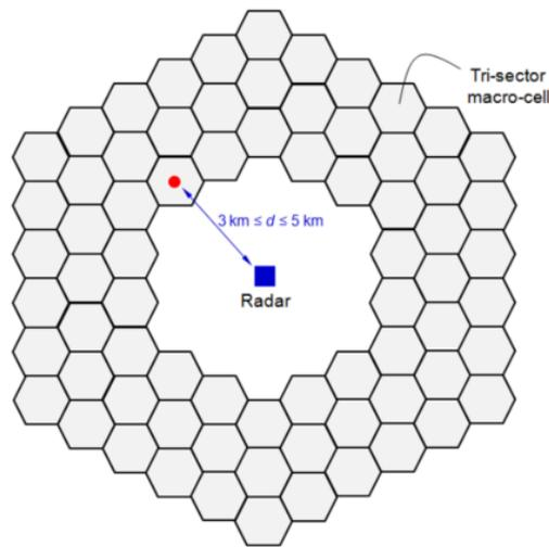
**Figure 23: From ECC Report 281 "A radar receiver is surrounded by 5 rings of 272 tri-sectored MFCN macro base stations (only three rings are shown)"**
