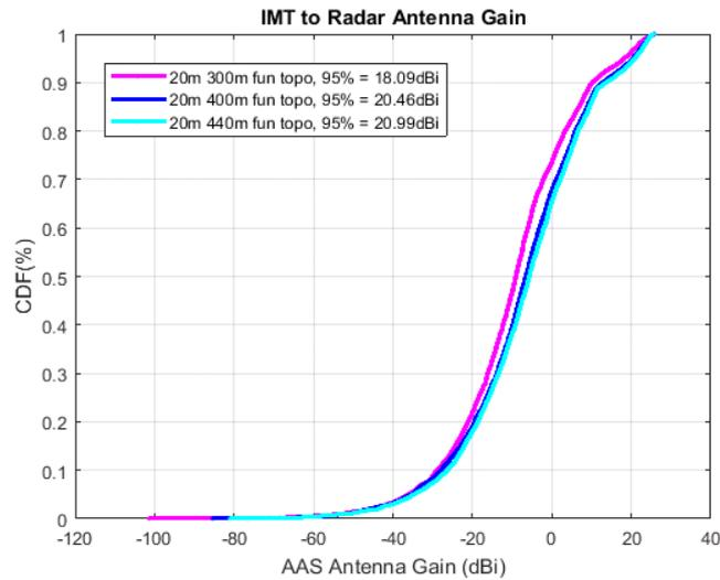
**Figure 63: IMT to radar AAS antenna gain for urban scenario for urban scenario and 20 m BS antenna height**
