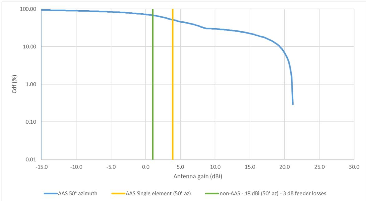
Figure 29: Antenna gain comparison (urban case at 50° azimuth)
