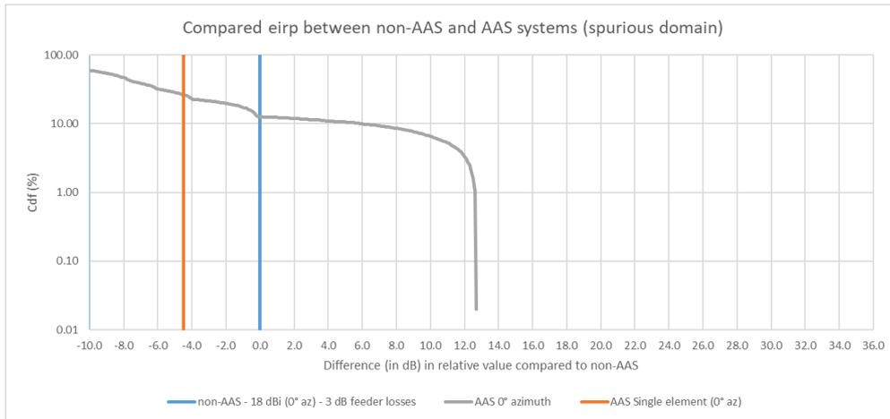
**Figure 39: Compared e.i.r.p. between non-AAS and AAS systems for rural case and 0° azimuth**
