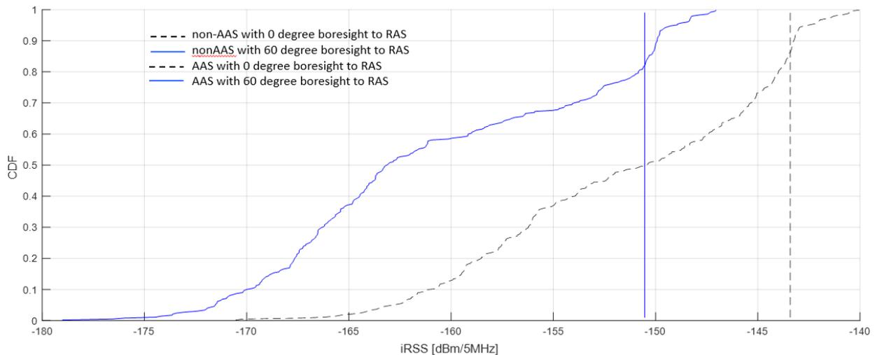
**Figure 44: iRSS for RAS at 60 km distance with boresight BS antenna to RAS 0 and 60 degree for single sector,  $p_{P.452} = 2\%$  and three UEs sharing bandwidth per snapshot (Table 72)**
