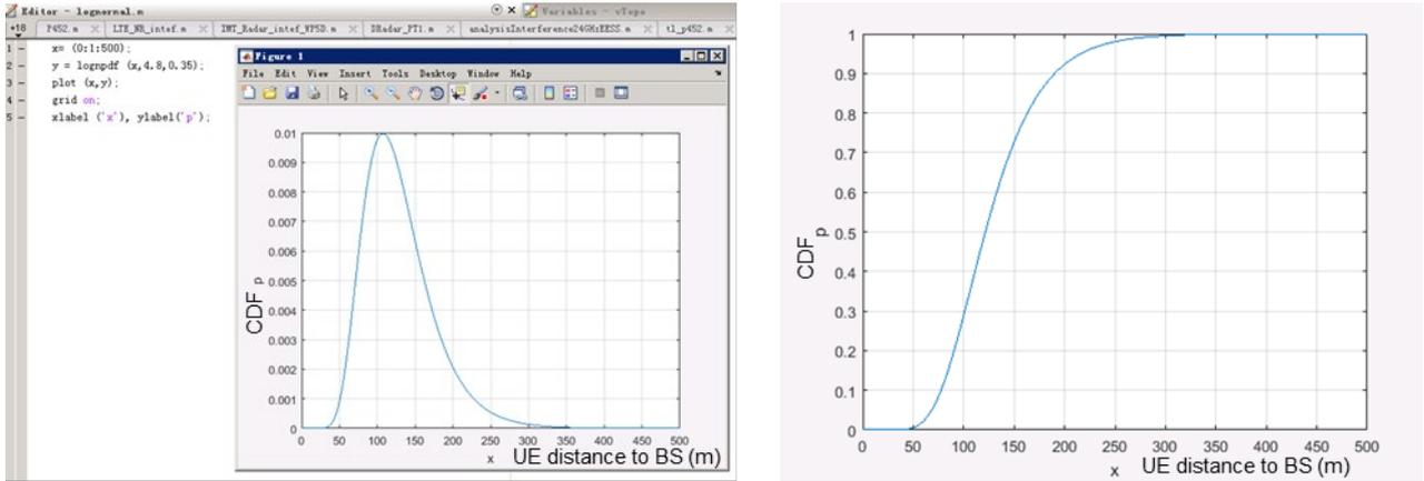
**Figure 60: (left) PDF of proposed log-normal distribution; (right) CDF of proposed log-normal distribution**
