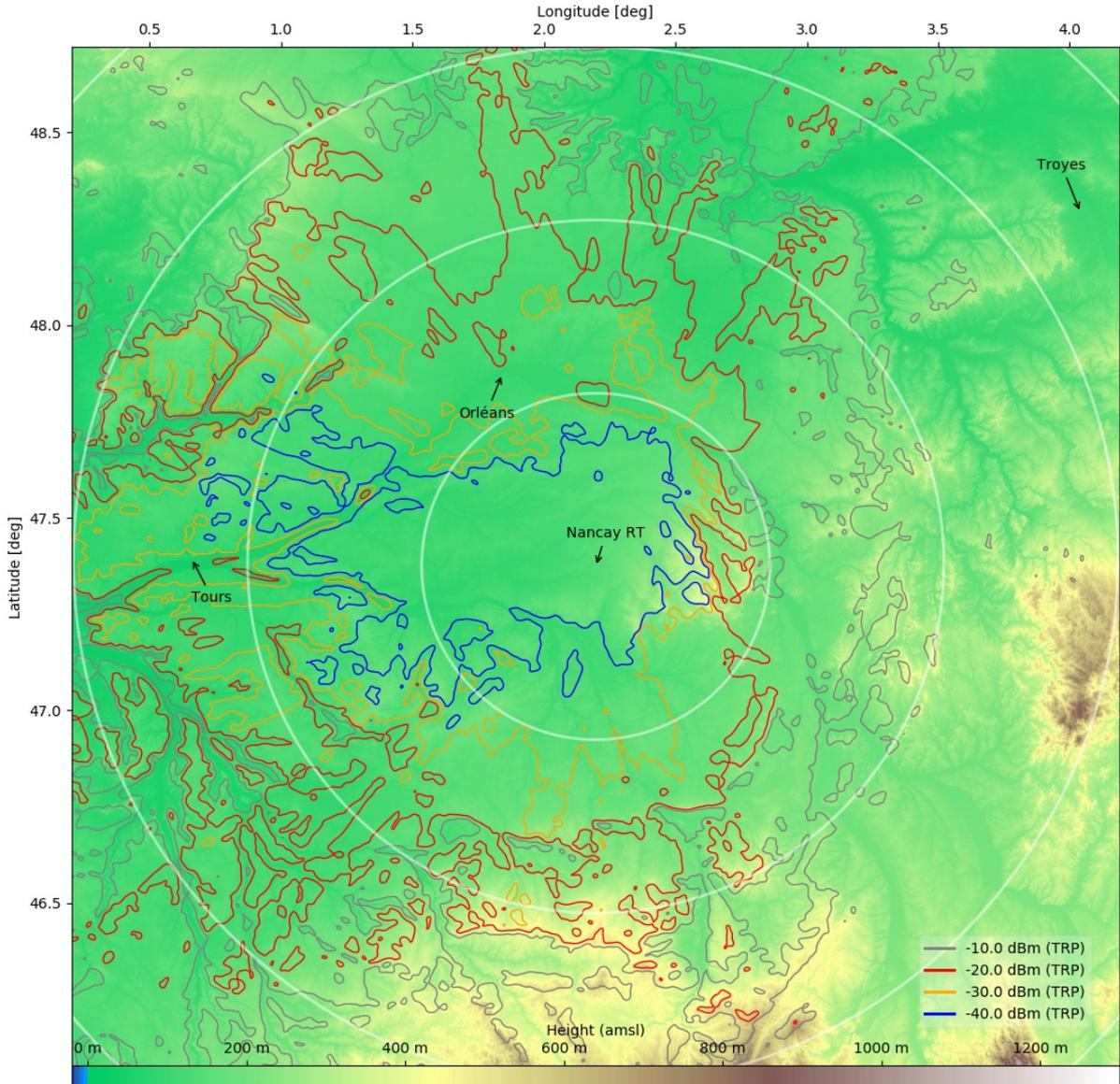
**Figure 91: Proposed coordination zones (spurious, 4G non-AAS) around Nancay radio telescope in France**
