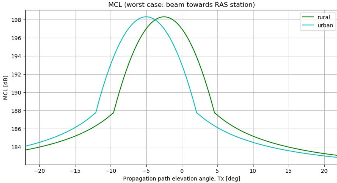
**Figure 81: MCL (OOB, 4G non-AAS) as a function of propagation path elevation angle**
