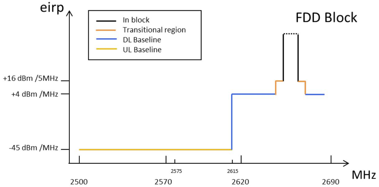
**Figure 7: Combined BEM elements for an FDD block with TDD (synchronised/unsynchronised) networks within 2570-2620 MHz for non-AAS**
