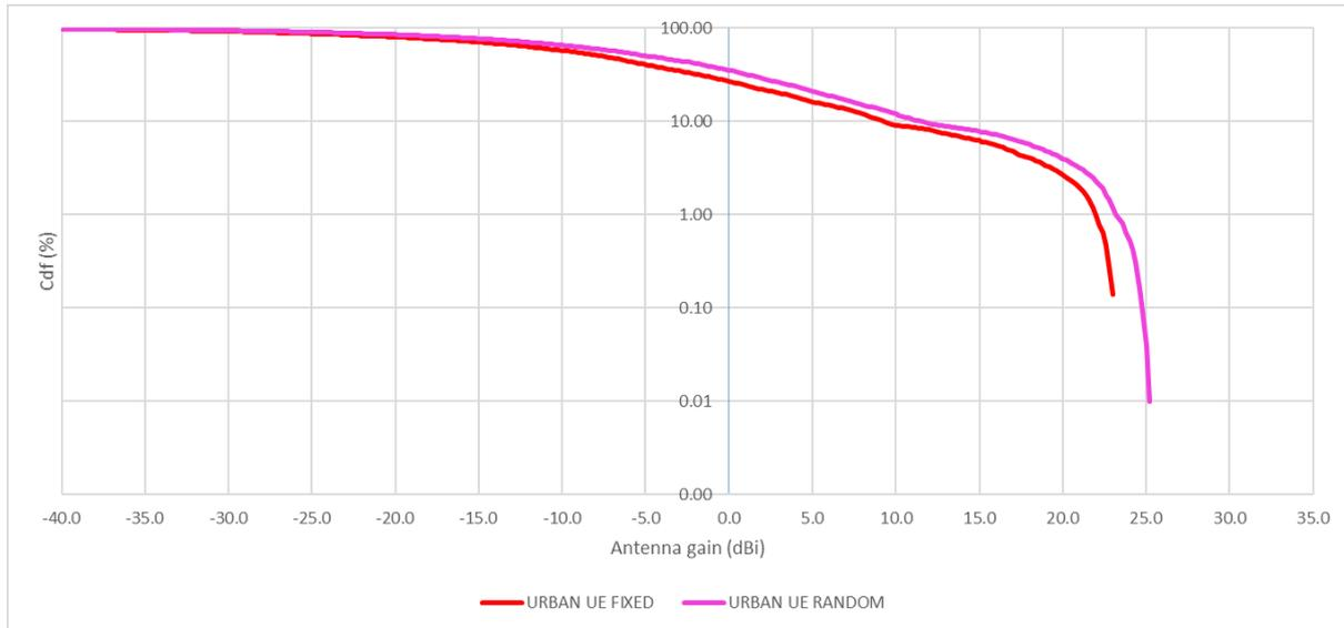
**Figure 41: AAS antenna gain towards radar for fixed UE height and random height distribution for urban case**
