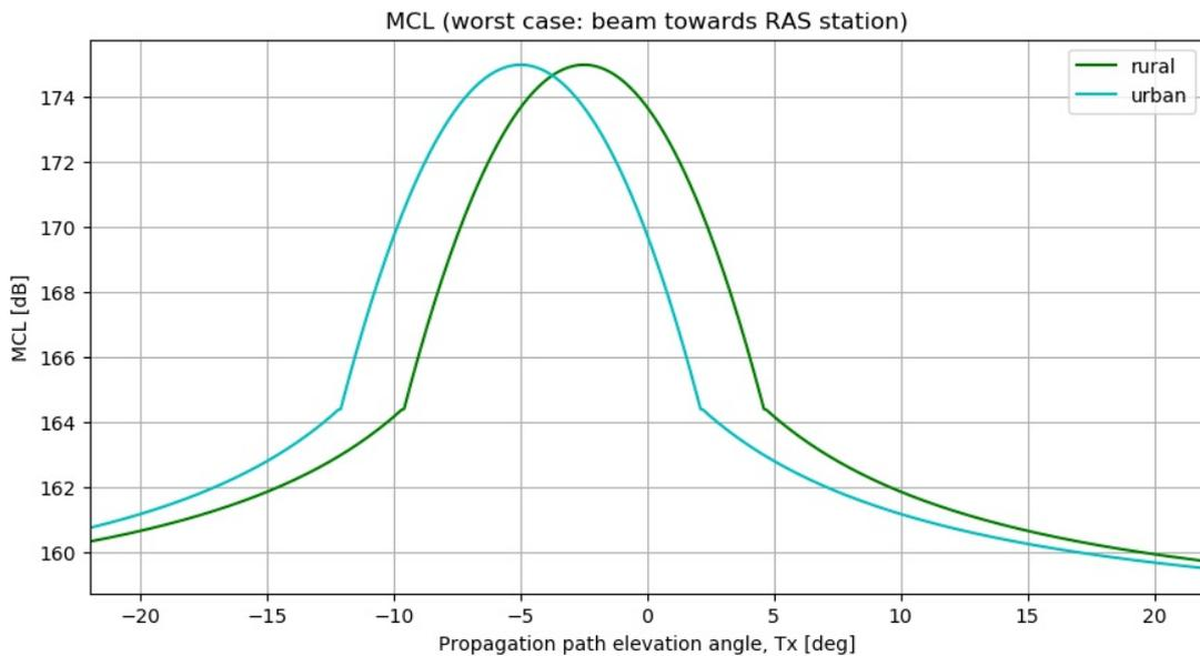
**Figure 82: MCL (spurious, 4G non-AAS) as a function of propagation path elevation angle**
