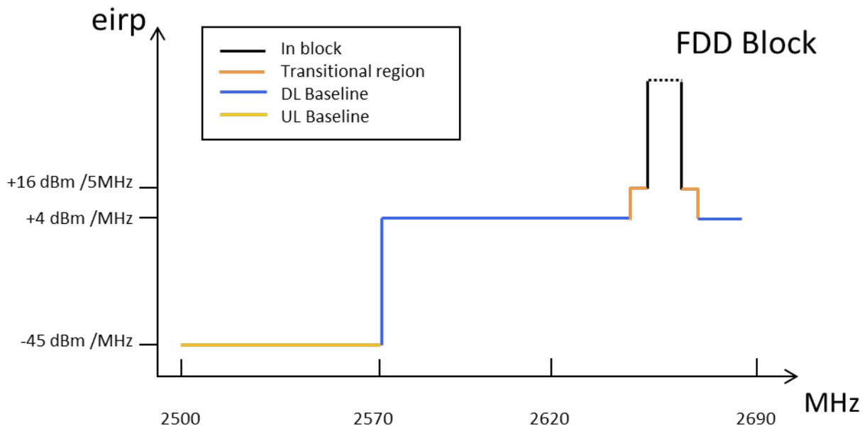
**Figure 6: Combined BEM elements for an FDD block above 2620 MHz with downlink only operation within 2570-2620 MHz for non-AAS**
