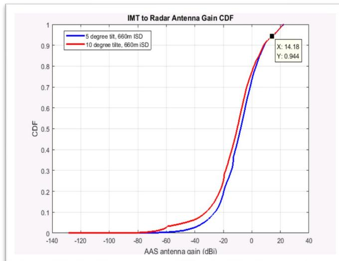
**Figure 64: Down tilt effect on AAS Antenna gain (hexagonal topology from ECC Report 174)**
