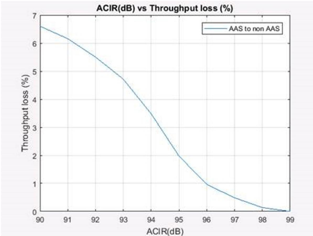
**Figure 18: Impact of AAS base station to non-AAS base station interference**
