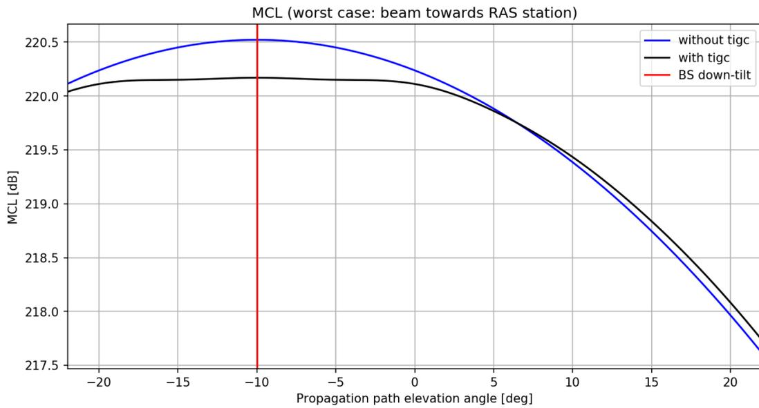
Figure 78: MCL (OOB, 5G AAS) as a function of propagation path elevation angle
