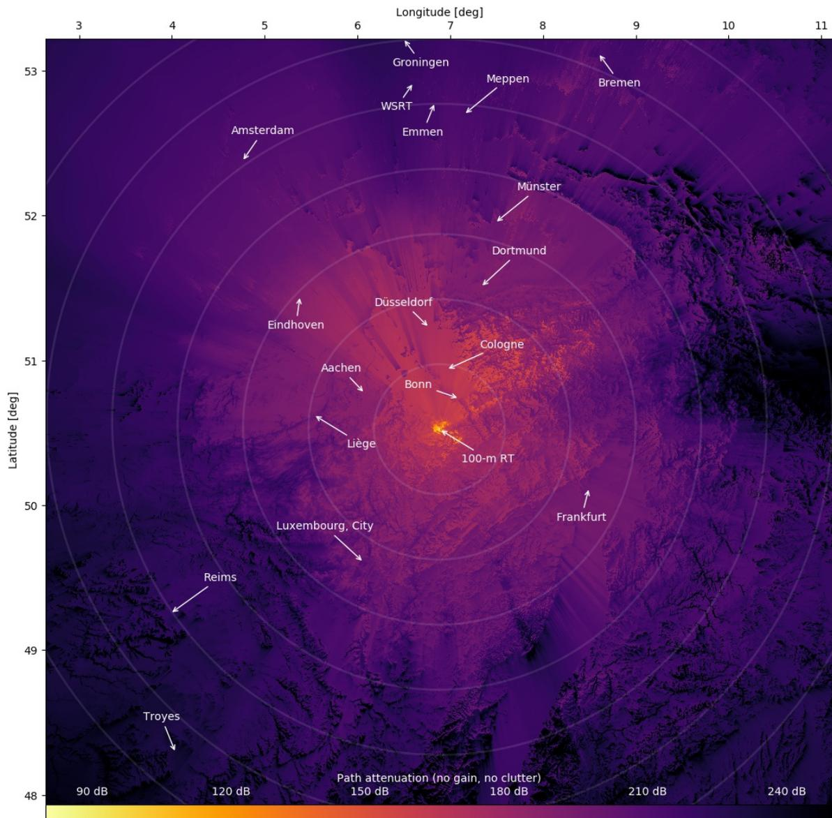
**Figure 84: Attenuation map around 100 m telescope in Effelsberg, Germany**
