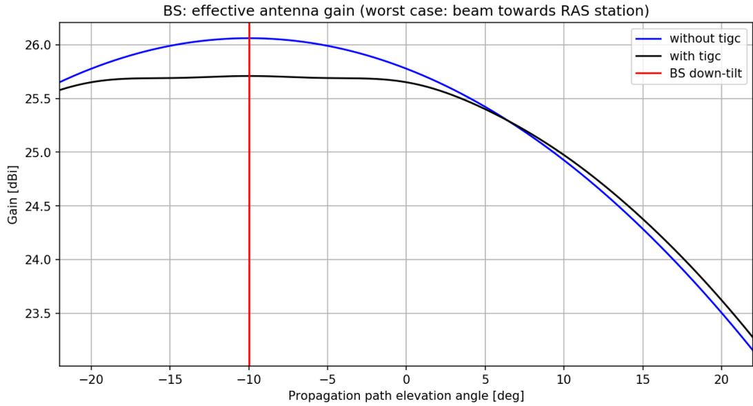
Figure 77: Effective 5G AAS antenna gain as a function of propagation path elevation angle
