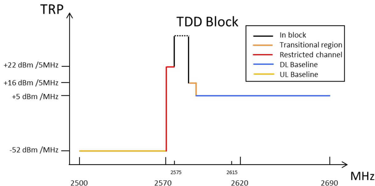
**Figure 15: Combined BEM elements for synchronised TDD/downlink only blocks and a restricted spectrum block in 2570-2575 MHz for AAS**
