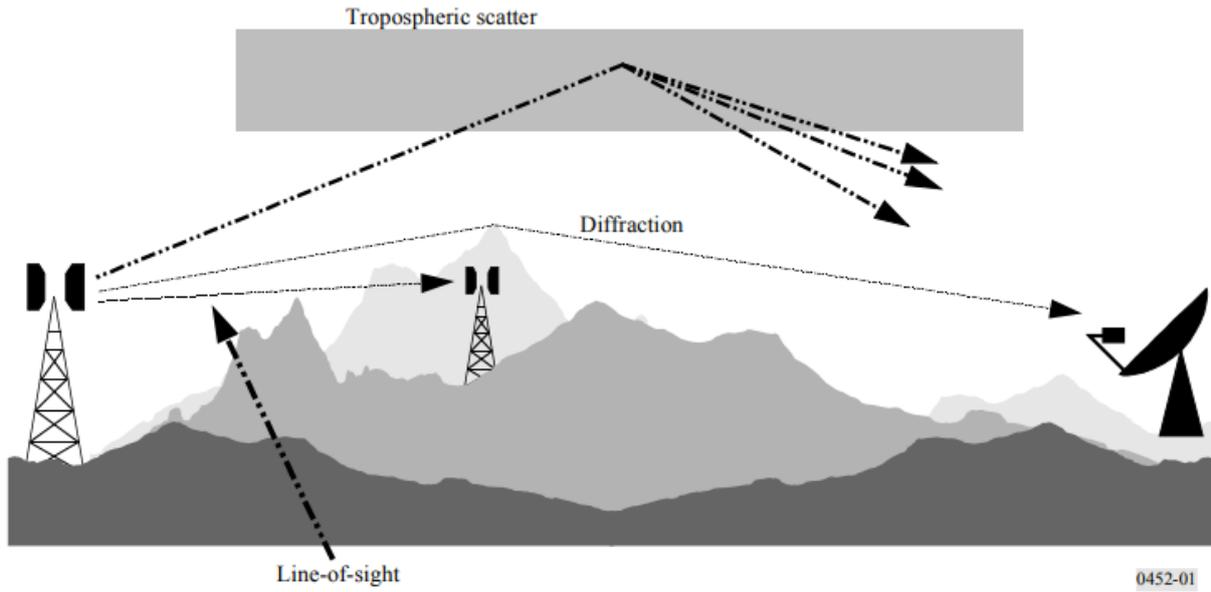
Figure 45: Long-term interference propagation mechanisms from Recommendation ITU-R P.452 [24]
