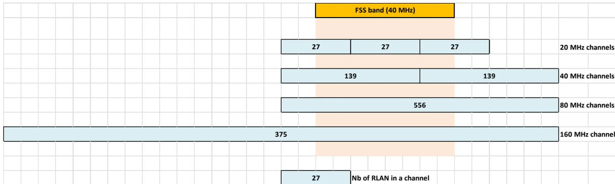
**Figure 59: RLAN channels incident to a 40 MHz FSS receiver bandwidth**
