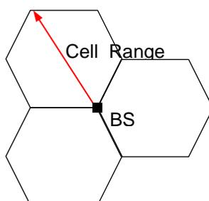
**Figure 2: Hexagonal three-sector cell layout**
