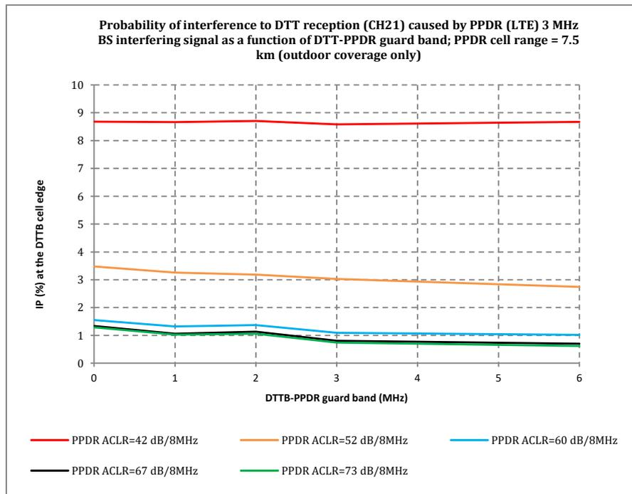
**Figure 12: LTE400 BS (e.i.r.p. 60 dBm/3MHz, cell range 7.5 km) impact on DTT reception at DTT cell edge**
