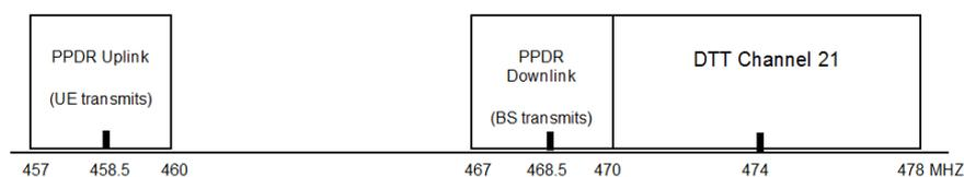
**Figure 8: PPDR (LTE) 400 MHz operating in an adjacent band to DTT channel 21 (GB=0 MHz)**
