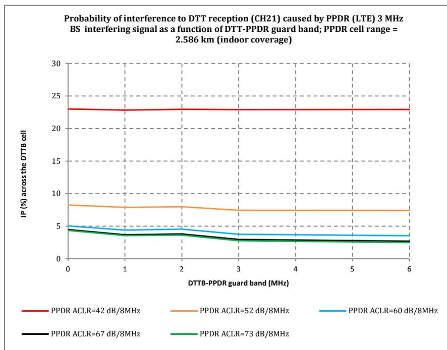
Figure 10: LTE400 BS (e.i.r.p.60 dBm/3MHz, cell range 2.568 km) impact on DTT reception
