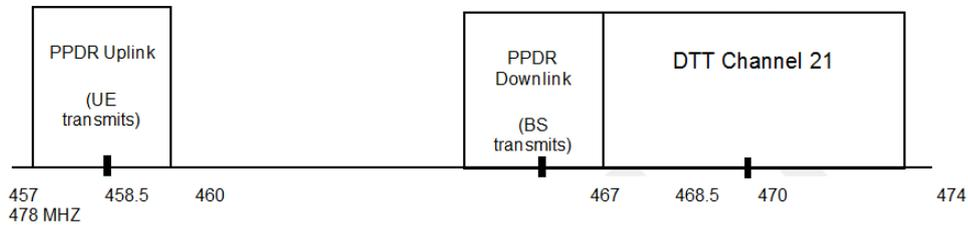
**Figure 85: Possible operation of PPDR (LTE) 400 MHz adjacent to DTT channel 21 without guard band.**
