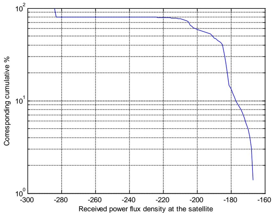
**Figure 27: Cumulative density function of power flux density**
