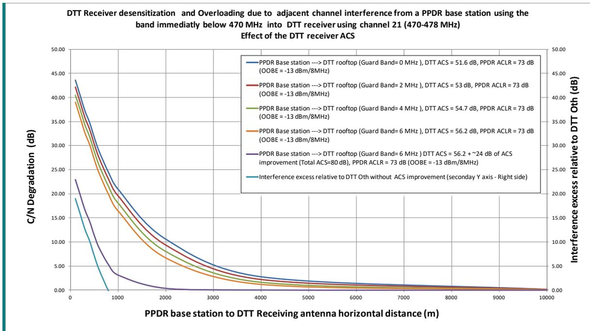
**Figure 17: Effect of the DTT receiver ACS on the risk of interference with the considered criteria, OOBE are in terms of e.i.r.p.**
