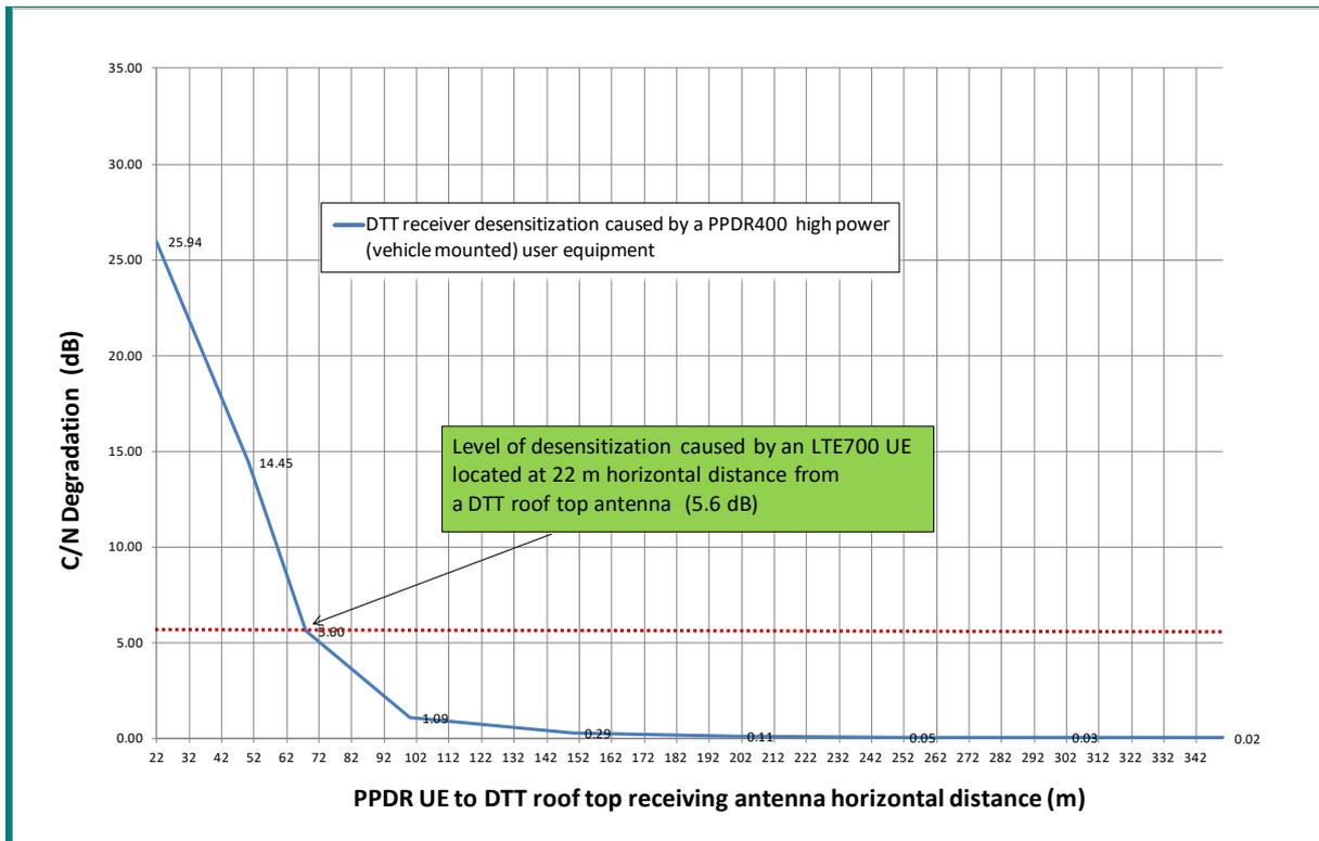
**Figure 15: C/N degradation vs horizontal separation distance between LTE UE and DTT reception**
