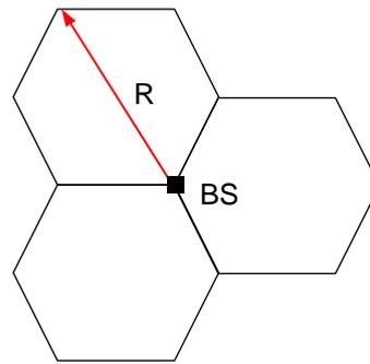
**Figure 49: Hexagonal three-sector cell layout (R: cell range)**
