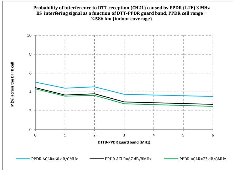
**Figure 11: LTE400 BS (e.i.r.p. 60 dBm/3MHz, cell range 2.568 km) impact on DTT reception**
