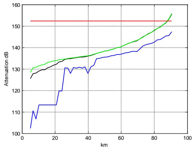
**Figure 31: Attenuation plots showing the required radii for exclusion zones around Effelsberg including terrain profile analysis for LTE400 base stations (left) and the user equipment (right). The green curves show the attenuation based on mean aggregate emission levels. The blue curves show the attenuation when the power levels exceed the mean level by no more than 2% of the time**
