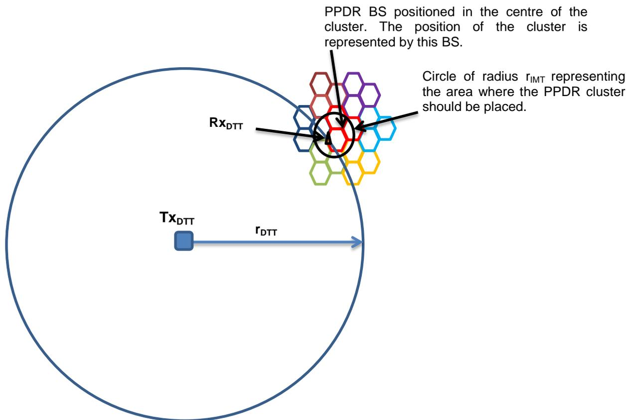
**Figure 52: Position of PPDR cluster around DTT receiver**
