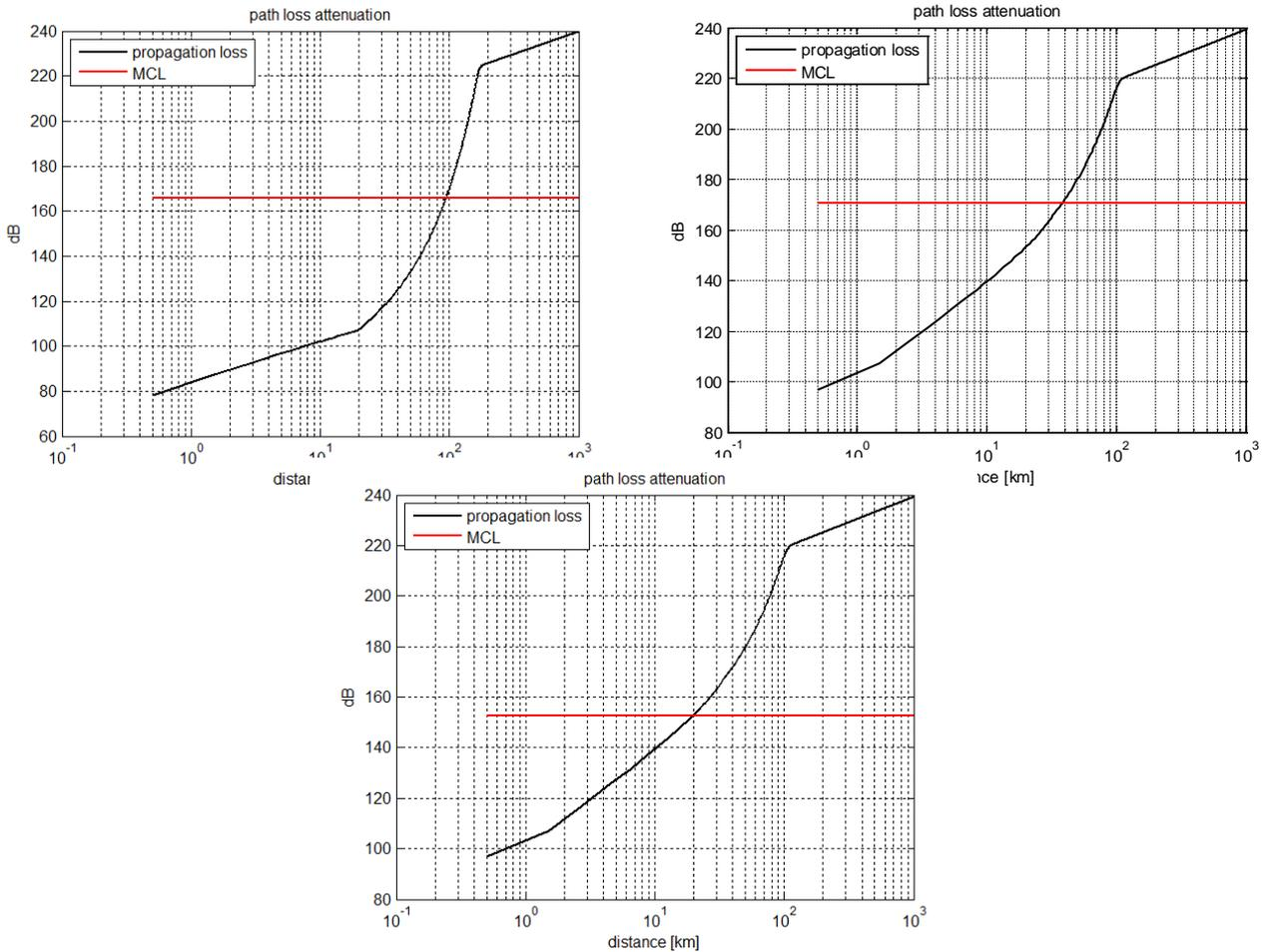
**Figure 28: Path loss attenuation graphs for spurious emission from LTE400 BS (left) fulfilling -36 dBm/100kHz emissions within the RAS frequencies and UE (right) depicting the required separation distances from a radio telescope assuming a flat terrain profile**
