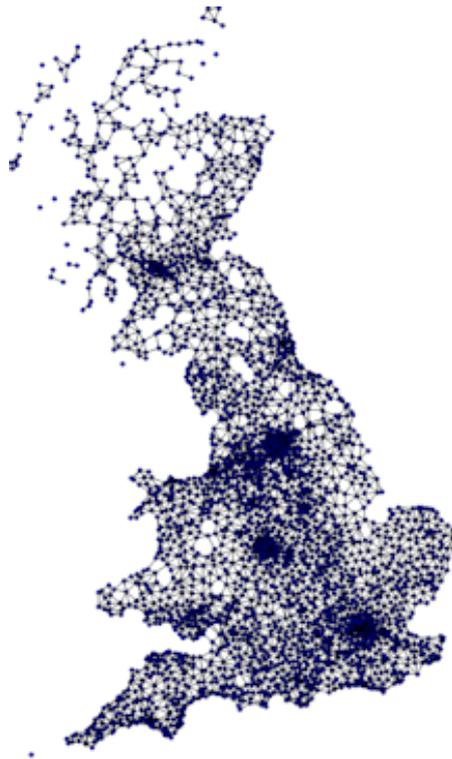
**Figure 42: Calculation of Inter Site Distance using Delaunay triangulation of Tetra site locations in Great Britain**
