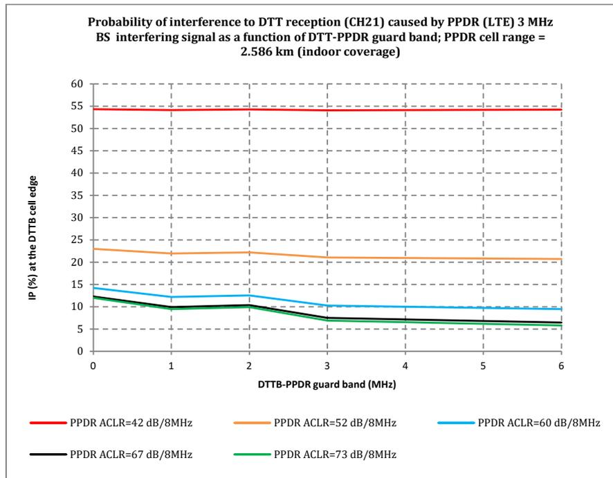
**Figure 13: LTE400 BS (e.i.r.p. 60 dBm/3MHz, cell range 2.568 km) impact on DTT reception at DTT cell edge**
