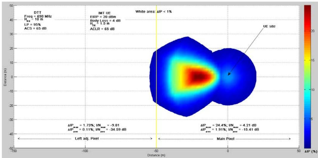
Figure 54: Interference footprint for commercial LTE700 UE impact on DTT
