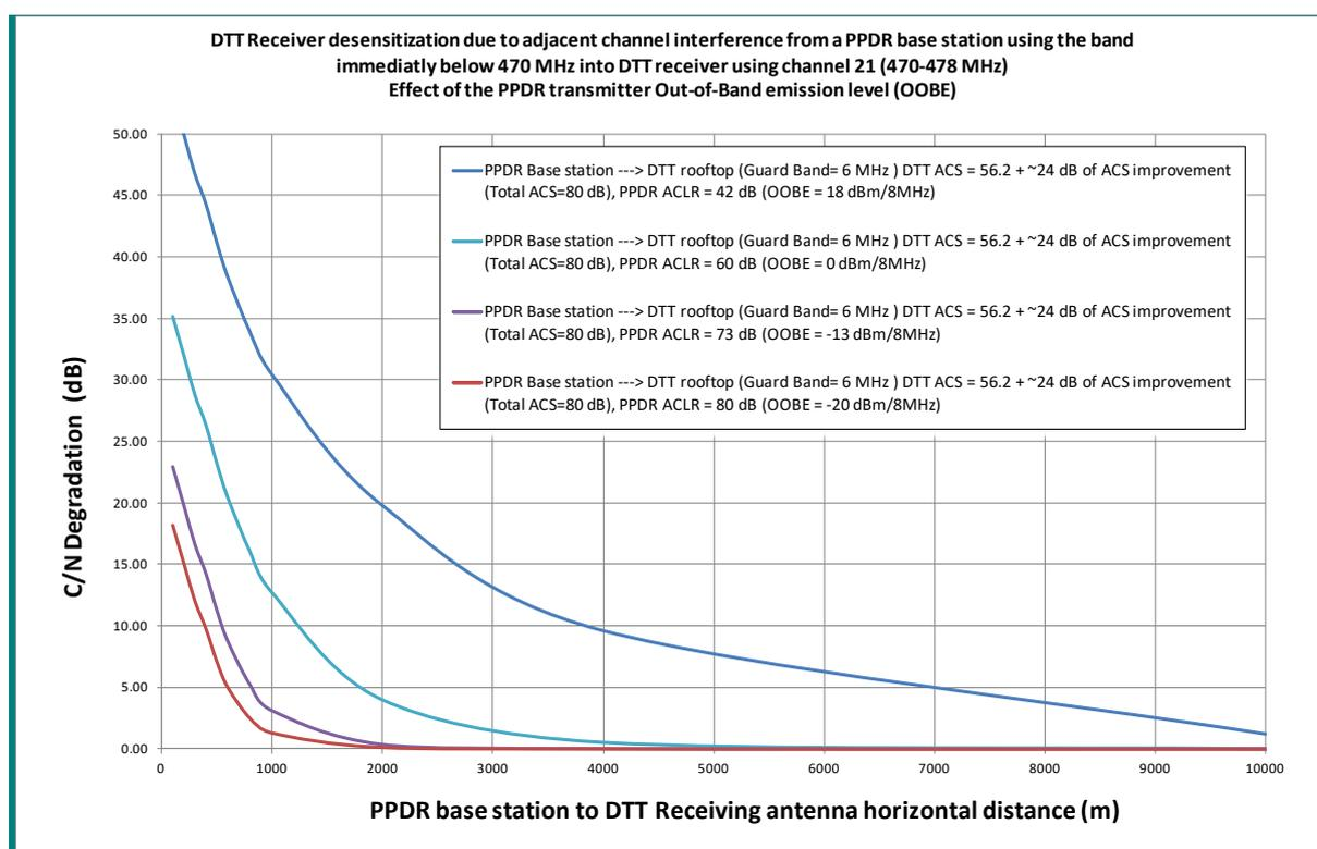
**Figure 18: Effect of the PPDR base station e.i.r.p. Out-of-Band emission level on the risk of interference with the considered criteria**
