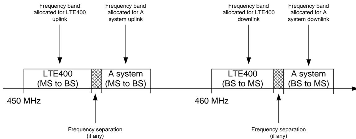
**Figure 1: Illustrative frequency allocation of the 450-470 MHz**
