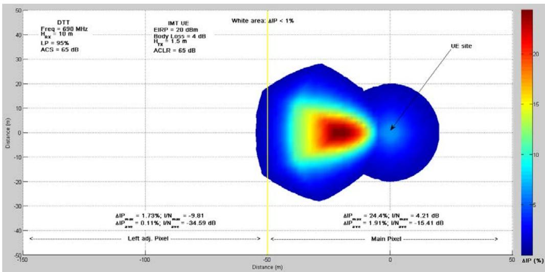
**Figure 20: Reference case: commercial LTE700 UE impact on DTT**
