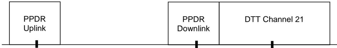
**Figure 53: PPDR (LTE) 400 MHz operating in an adjacent band to DTT channel 21.**
