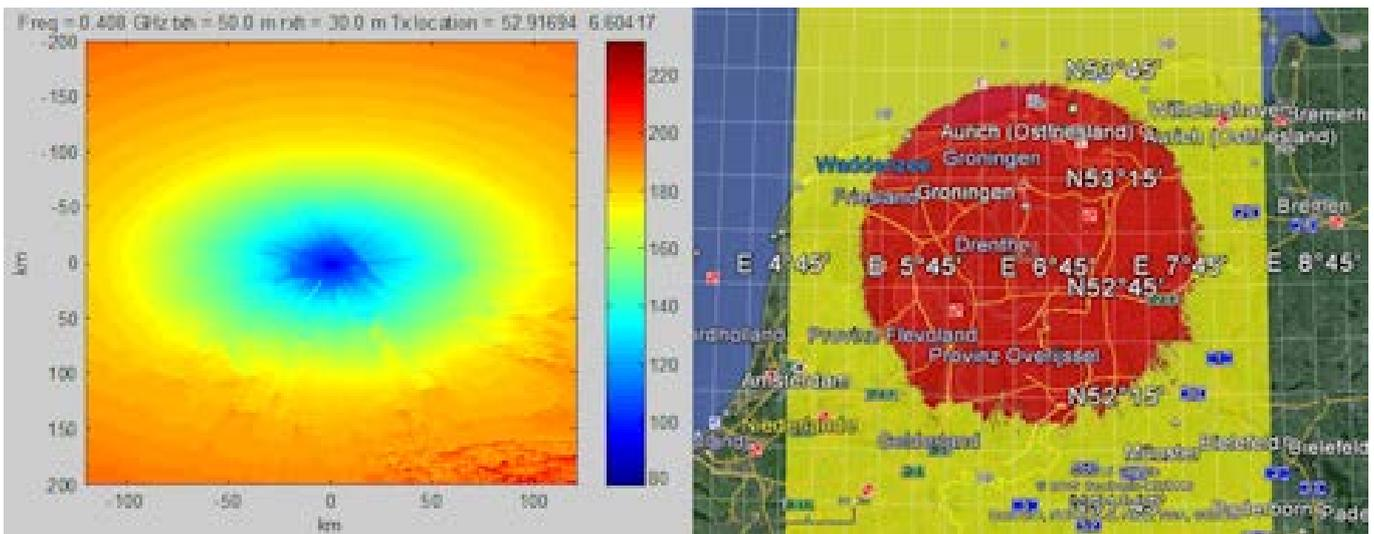
**Figure 32: Attenuation map for Westerbork based on terrain profile analysis for LTE400 base stations (left) and the map for the exclusion zone based on MCL calculations (right)**
