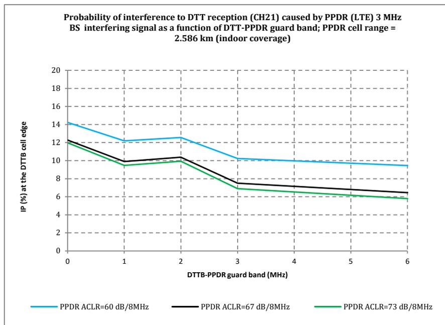
**Figure 14: LTE400 BS (e.i.r.p. 60 dBm/3MHz, cell range 2.568 km) impact on DTT reception at DTT cell edge**
