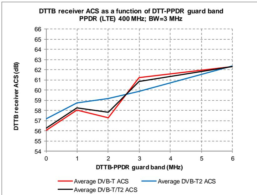
**Figure 41: DTTB ACS values determined by measurements on ten different brand new DTTB receivers**
