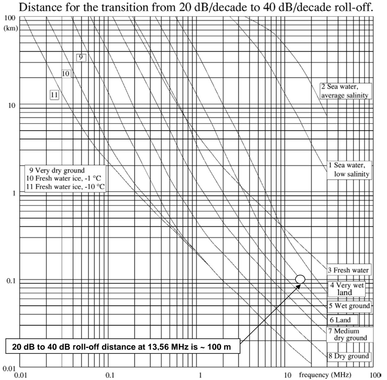
**Figure 30: Roll-off distance determination for 13.56 MHz over wet ground**
