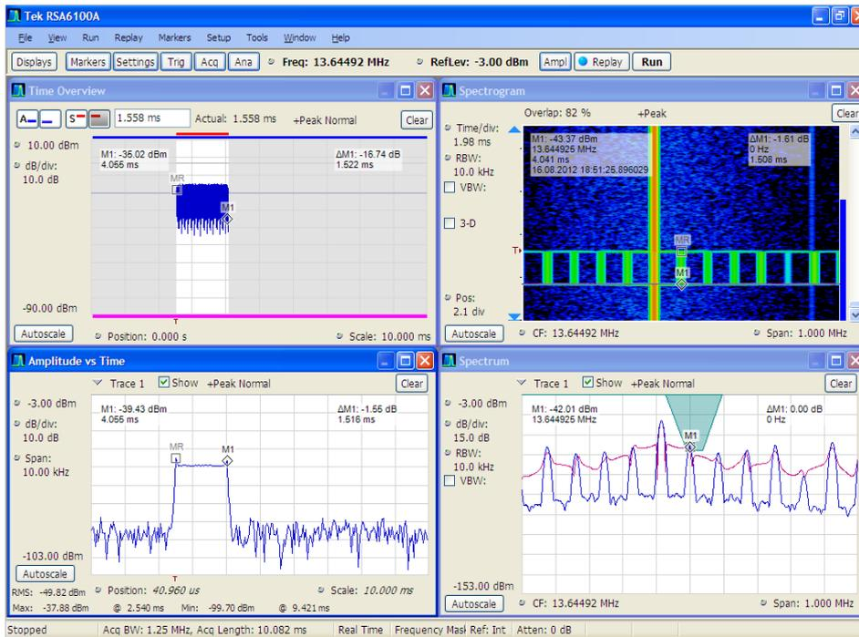
**Figure 17: Time analysis of the Reader 2 signal for a 10 ms time interval**
