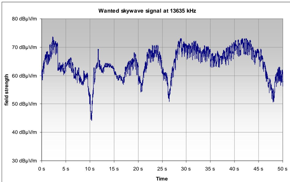
**Figure 29: Field strength vs. time of the wanted broadcast signal on 13.635 MHz**
