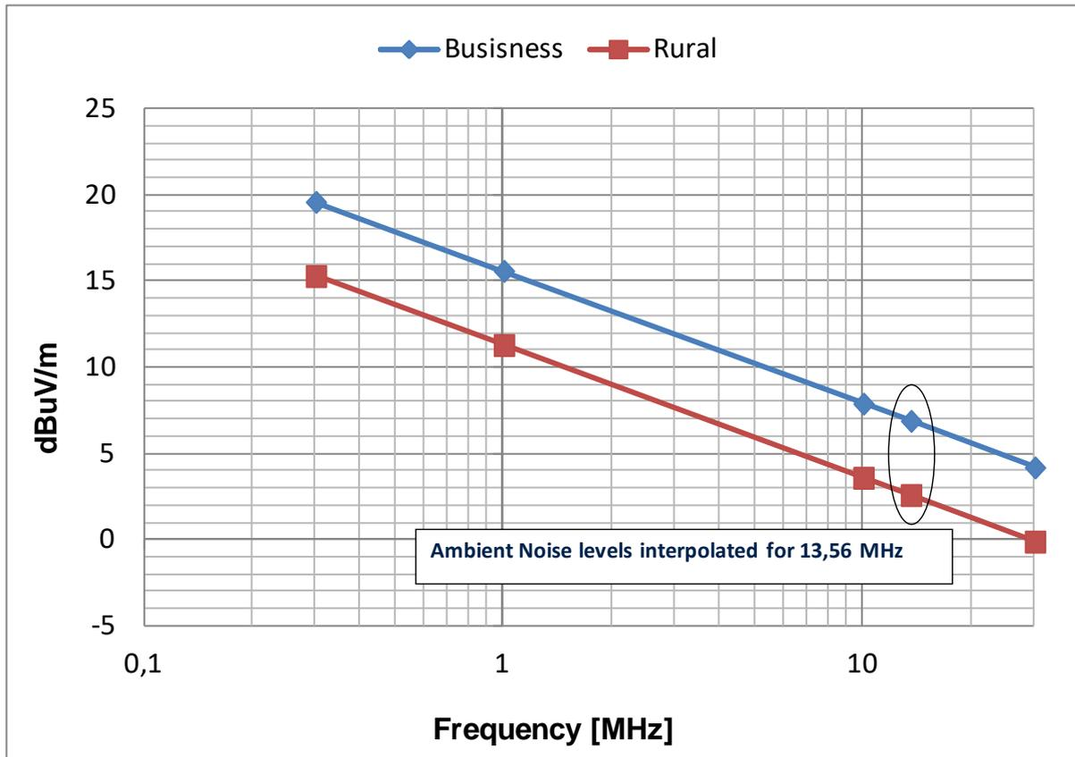
**Figure 31: Slope of Frequency dependent man-made noise level to determine noise levels at 13.56 MHz**
