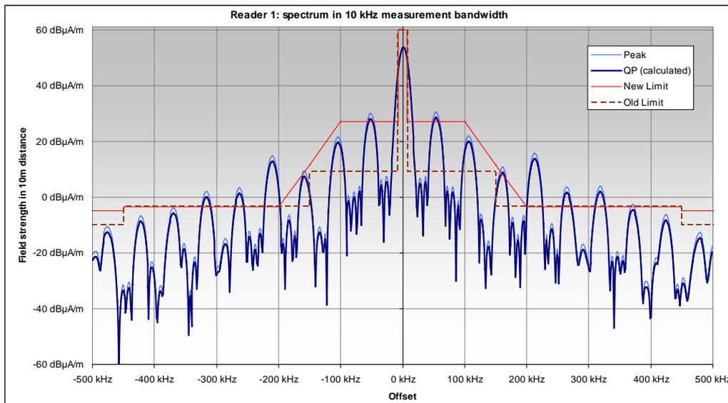
**Figure 11: QP spectrum of Reader 1 and spectrum masks**
