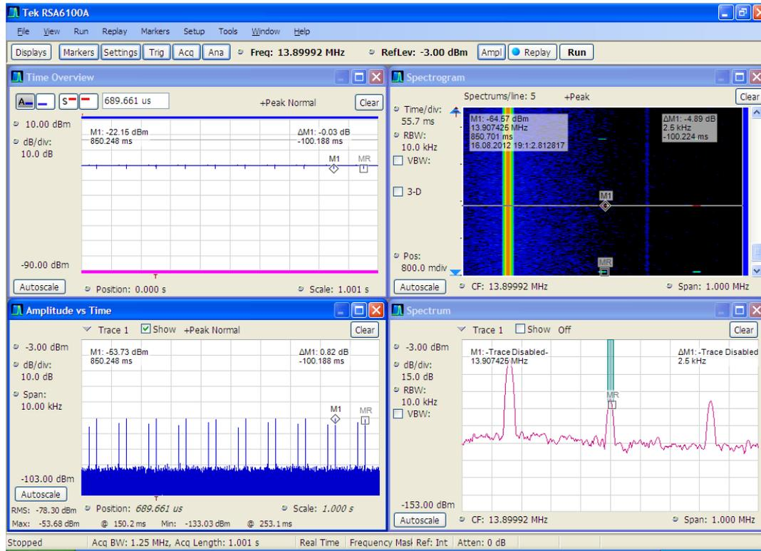
**Figure 20: Time analysis of the Reader 3 signal for a 1 s time interval**
