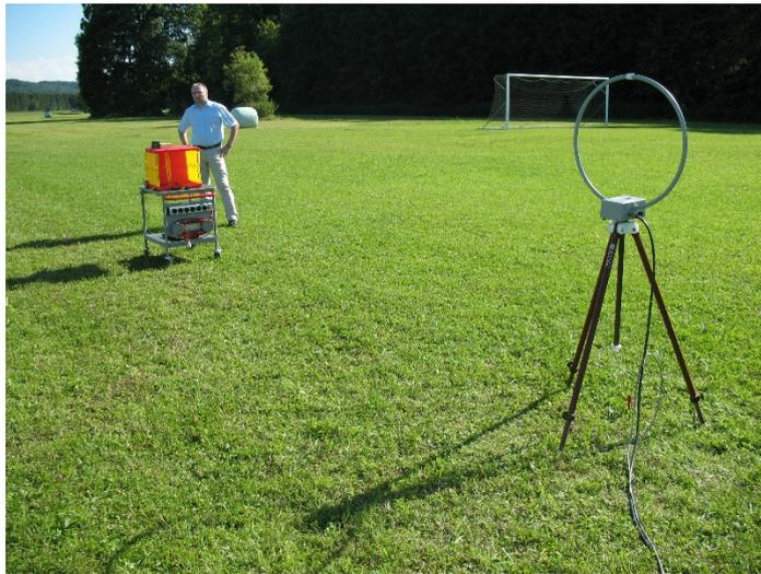
**Figure 21: Magnetic loop measurement antenna**
