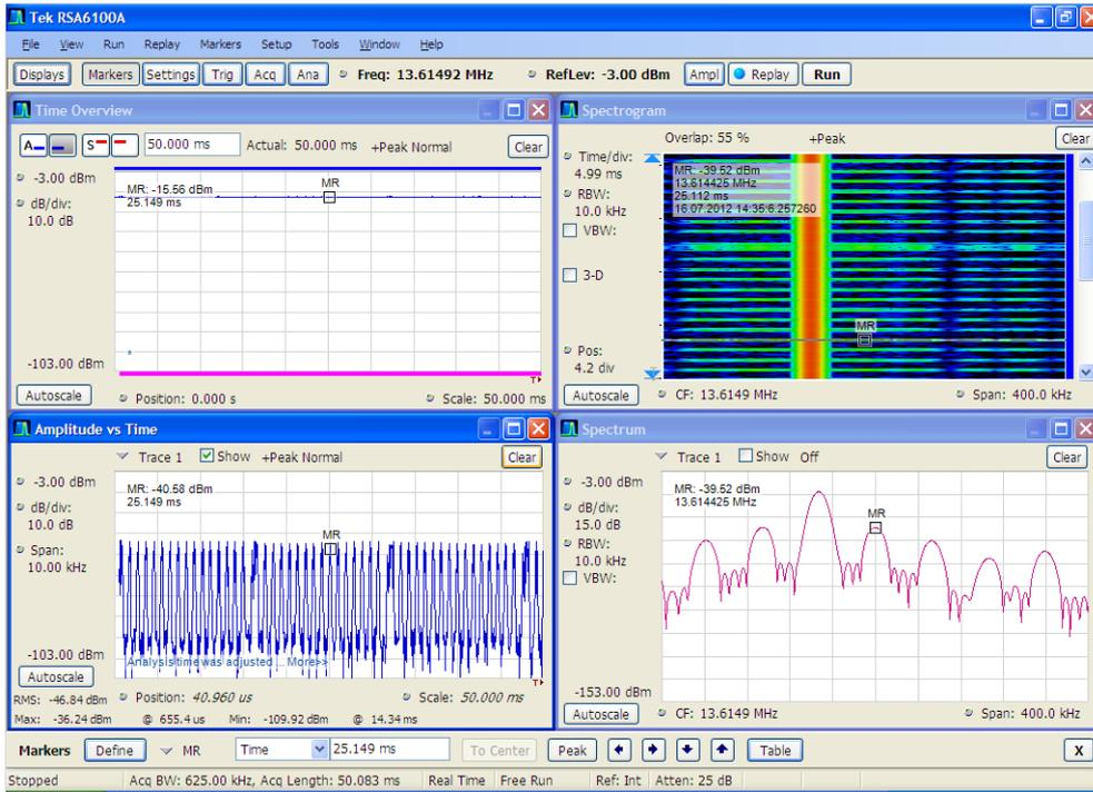
**Figure 16: Time analysis of the Reader 1 signal**
