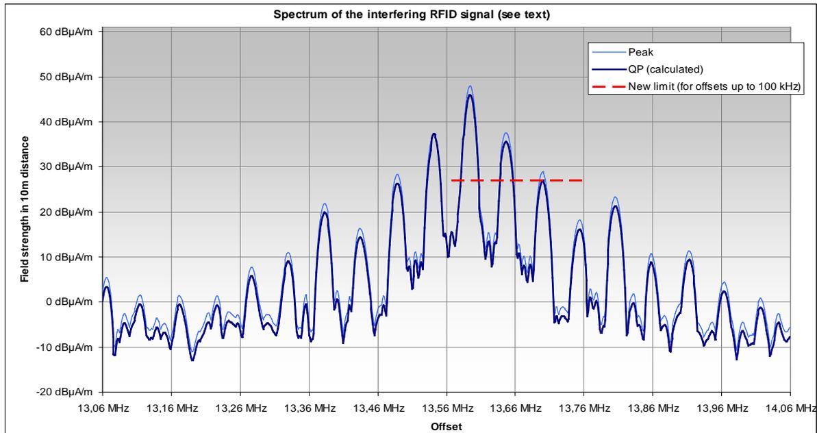
**Figure 26: Interfering RFID signal used for the measurements**
