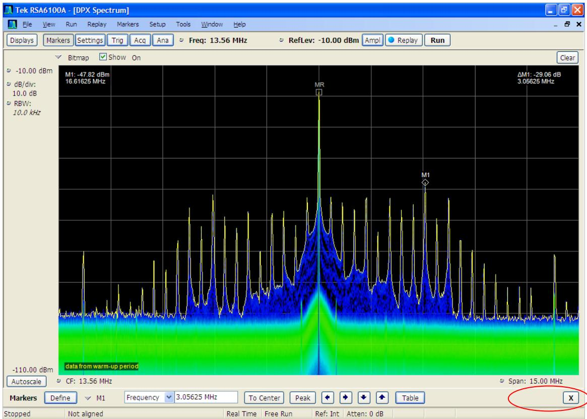
Figure 10: DPX spectrum of Reader 3 (low power, 6.8 MBit/s)
