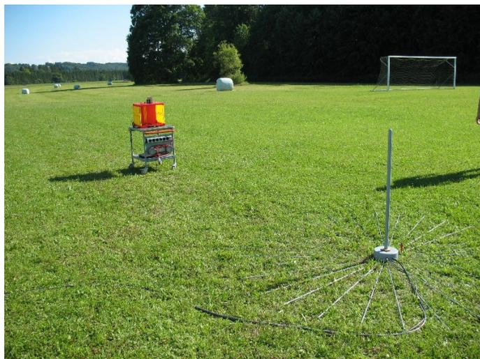
**Figure 22: Electrical monopole measurement antenna**
