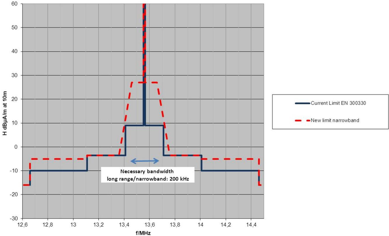
**Figure 4: Long range / narrowband RFID emitter mask**
