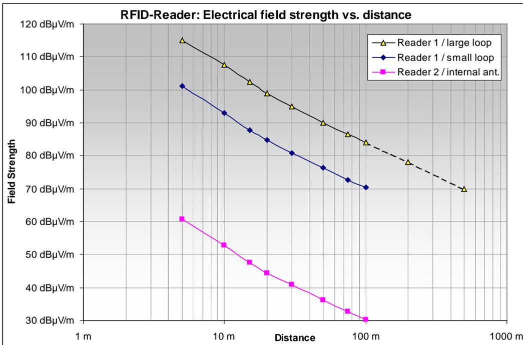
Figure 24: Electrical field strength vs. distance
