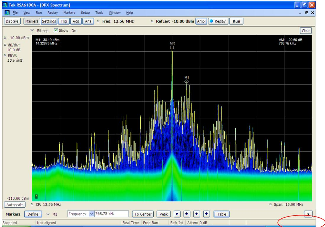
Figure 9: DPX spectrum of Reader 2 (low power, 1.7 MBit/s)
