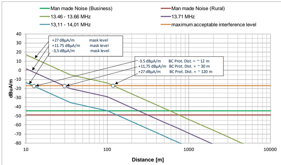
**Figure 33: Magnetic field strength and protection distances for different emission levels of the TX mask (indoor operation)**
