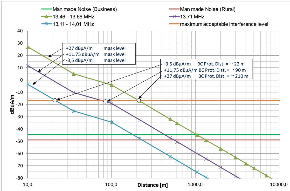
**Figure 32: Magnetic field strength and protection distances for different emission levels of the TX mask (outdoor operation)**
