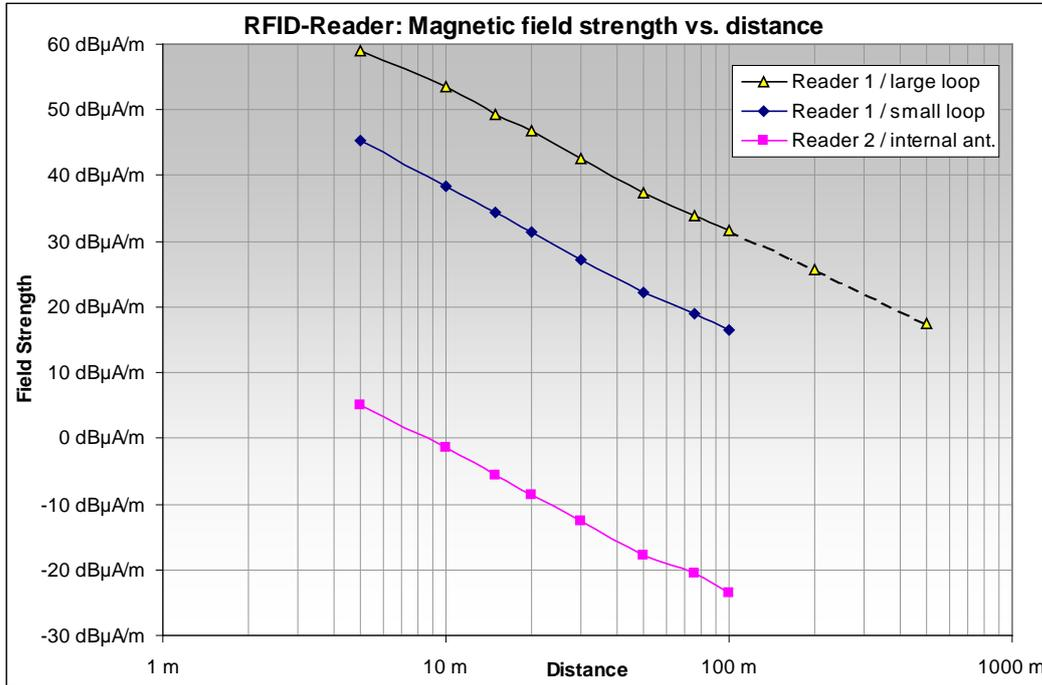
Figure 23: Magnetic field strength vs. distance
