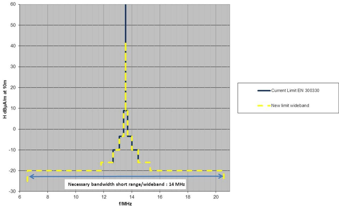
**Figure 3: Short range / wideband RFID emitter mask**
