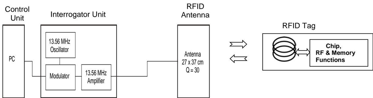
**Figure 1: RFID system**
