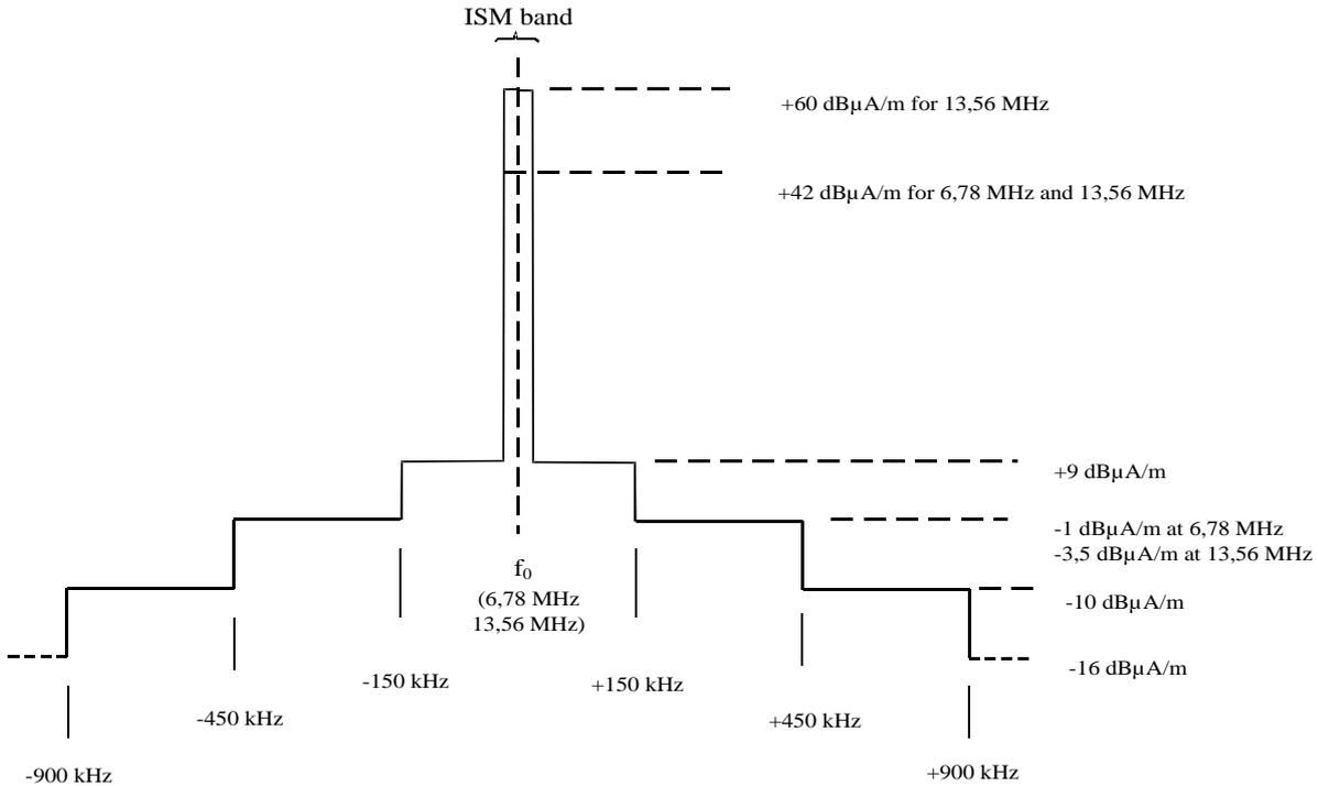
**Figure 2: Present 13.56 MHz RFID emitter mask from EN 300 330**
