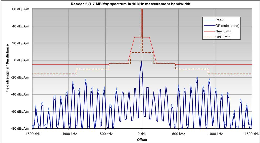
Figure 12: QP spectrum of Reader 2 and spectrum masks close to the carrier
