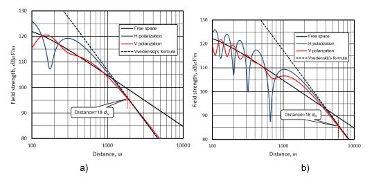
Figure 12: Field strengths vs. distance for different receiving antenna heights (a: 3m, b: 10m)
