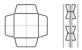
Figure 21: Top and side view of a typical UHF DVB-T/-T2 antenna design on a rectangular mast
