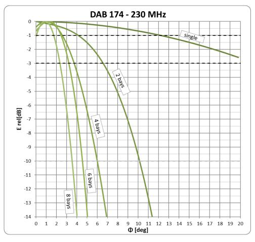
Figure 20: Typical vertical patterns of VHF DAB antennas
