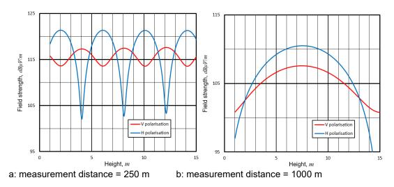
Figure 14: Field strength dependency on height at different measurement distances
