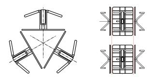
Figure 19: Top and side view of a typical VHF DAB antenna design on a triangular mast
