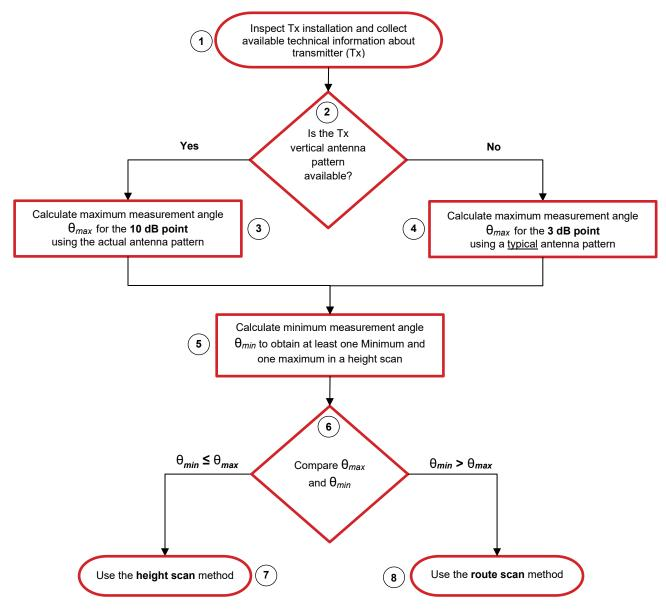
Figure 3: Decision of the applicable measurement method
