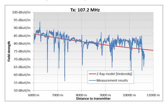
Figure 8: Example evaluation of a route scan
