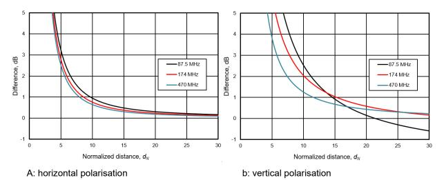
Figure 13: Difference in calculated field strengths between Vvedenskij's formula and exact 2-ray equations
