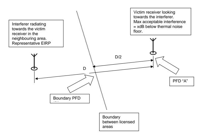
Figure 10: Example of PFD boundary limit
