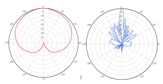
Figure 6: RLAN 17 dBi Sector Antenna – Elevation (blue) and Azimuth (red) Radiation Patterns
