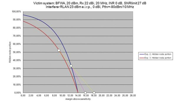
Figure 28: Hidden node probability for BFWA as victim as function of the margin above sensitivity at the BFWA receiver and the propagation condition
