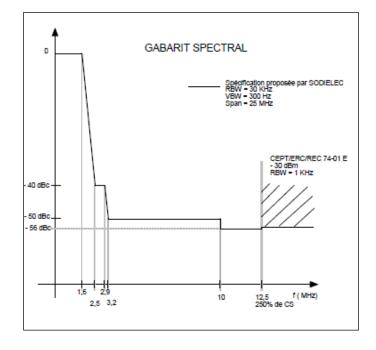
Figure 9: Spectrum emission mask of the public transport automation systems
