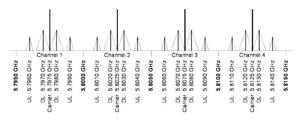
Figure 45: road-tolling systems frequency utilisation for 1.5 MHz sub-carrier frequency, according the ETSI EN 300 674
