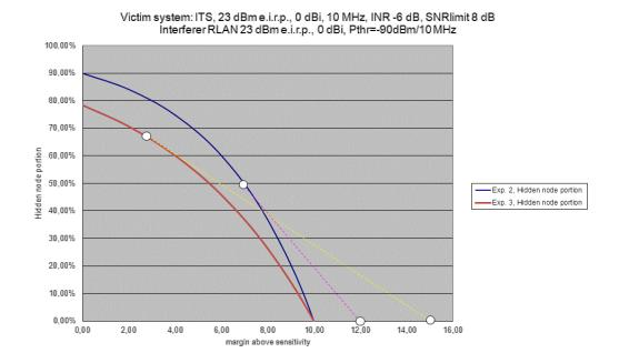
Figure 20: Hidden node probability for ITS as victim as function of the margin above sensitivity at the ITS receiver and the propagation condition
