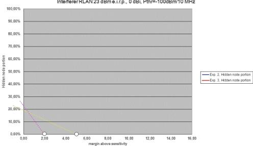
Victim system: ITS, 23 dBm e.i.r.p., 0 dBi, 10 MHz, INR -6 dB, SNRlimit 8 dB Interferer RLAN 23 dBm e.i.r.p., 0 dBi, Pthr=-100dBm/10 MHz
