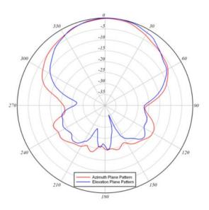
Figure 4: RLAN 6 dBi Directional – Elevation (blue) and Azimuth (red) Radiation Patterns
