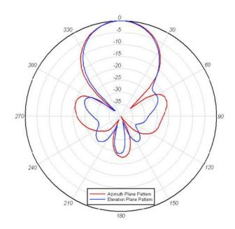
Figure 5: RLAN 12 dBi Directional – Elevation (blue) and Azimuth (red) Radiation Patterns
