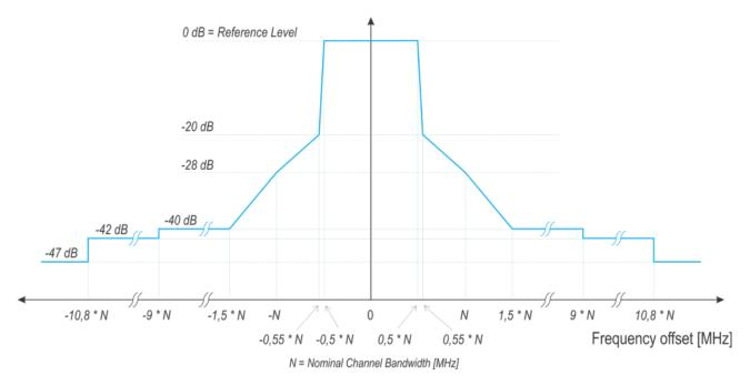
Figure 2: Spectrum mask for RLAN
