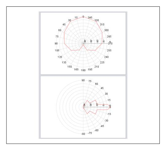
Figure 11: Horizontal and Vertical Pattern of BFWA CS Rx
