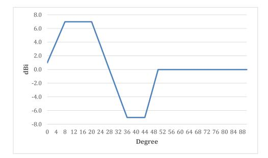
Figure 53: Aircraft Station Antenna Elevation Pattern (ETSI TR 103 108)
