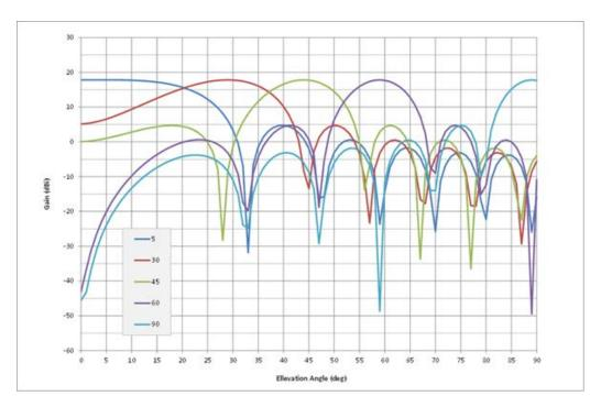
Figure 50: Aircraft Station antenna elevation patterns (ETSI TR 101 599 [24])
