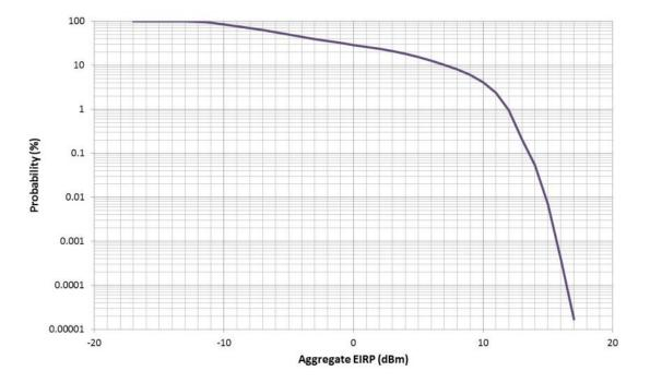
Figure 40: Aggregate e.i.r.p. (in any azimuth direction) produced by a DA2GC GS supporting 12 aircrafts
