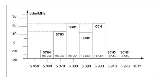
Figure 43: Maximum limit of mean spectral power density for each channel type in ITS-G5A, ITS-G5B, and ITS-G5D
