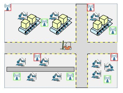
Figure 41: Scenario 1-1: RLAN Access Point in a factory floor
