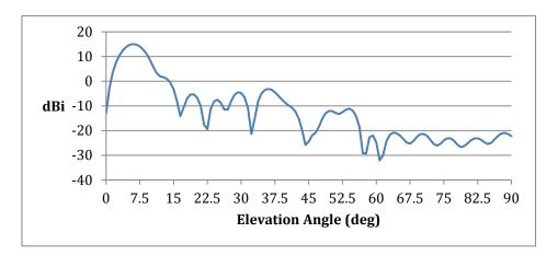
Figure 52: Ground Station Elevation Pattern for Sector Antenna (ETSI TR 103 108)
