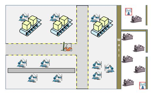
Figure 42: Scenario 1-2: RLAN Access Point and Clients in the adjacent office to WIA
