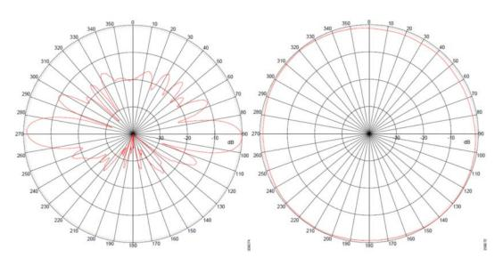
Figure 3: RLAN 6 dBi Omni – Elevation (left) and Azimuth (right) Radiation Patterns
