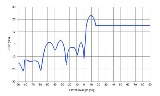
Figure 48: Ground Station antenna elevation pattern (ETSI TR 101 599 [24])
