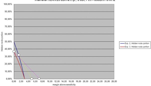
Victim system: BFWA, 14 dBm, Rx 16 dBi, 20 MHz, INR 0 dB, SNRlimit 27 dB Interferer RLAN 23 dBm e.i.r.p., 0 dBi, Pthr=-95dBm/10 MHz
