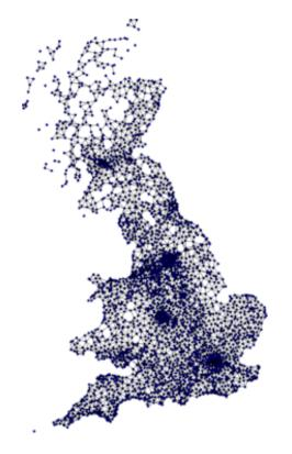
Figure 42: Calculation of Inter Site Distance using Delaunay triangulation of Tetra site locations in Great Britain
