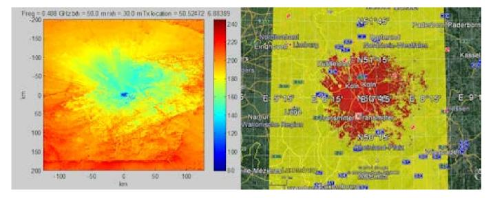
Figure 29: Attenuation map for Effelsberg based on terrain profile analysis for LTE400 base stations (left) and the map for the exclusion zone based on MCL calculations (right)
