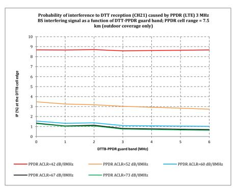
Figure 12: LTE400 BS (e.i.r.p. 60 dBm/3MHz, cell range 7.5 km) impact on DTT reception at DTT cell edge
