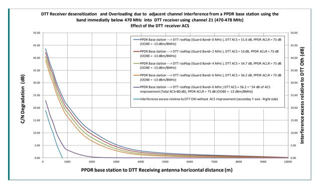
Figure 17: Effect of the DTT receiver ACS on the risk of interference with the considered criteria, OOBE are in terms of e.i.r.p.
