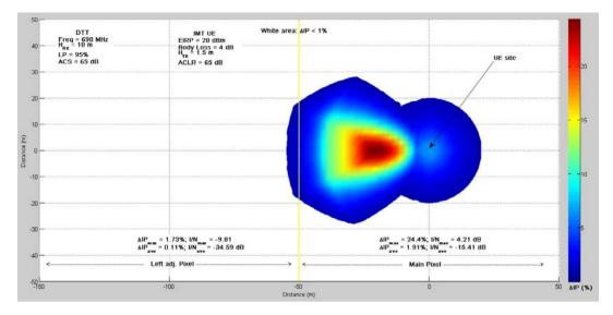
Figure 54: Interference footprint for commercial LTE700 UE impact on DTT
