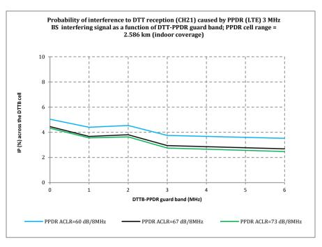
Figure 11: LTE400 BS (e.i.r.p. 60 dBm/3MHz, cell range 2.568 km) impact on DTT reception
