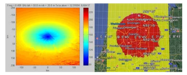
Figure 32: Attenuation map for Westerbork based on terrain profile analysis for LTE400 base stations (left) and the map for the exclusion zone based on MCL calculations (right)
