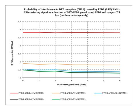
Figure 9: LTE400 BS (e.i.r.p. 60 dBm/3MHz, cell range 7.5 km) impact on DTT reception
