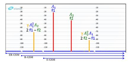
Figure 2: Generation of intermodulation products
