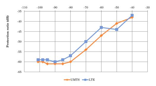
GSM-R at 924,8 MHz – UMTS and LTE at 927,6 MHz
