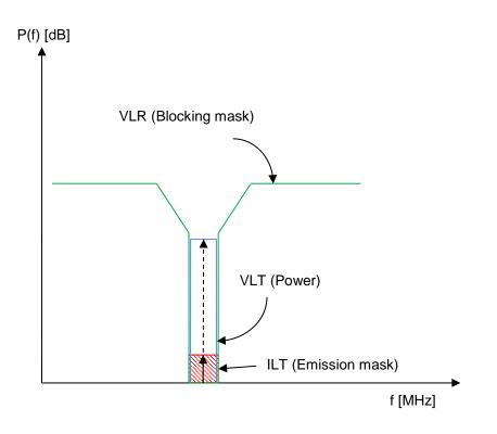
Figure 19: Simplification of coexistence analysis
