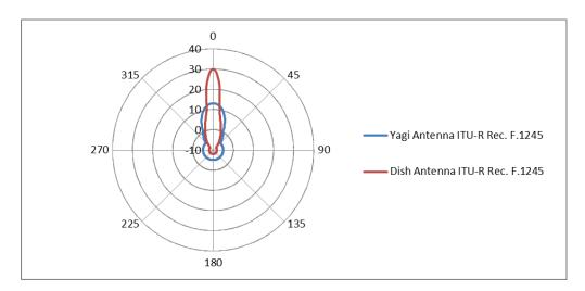
Figure 2: FS antenna patterns derived from ITU-R Rec. F. 1245
