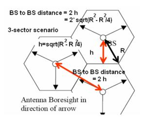
Figure 16: Network layout and cell radius definition
