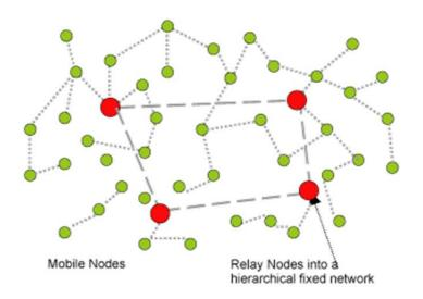
Figure 11: Hybrid Network: Intra-Mesh traffic with Infra-structure support
