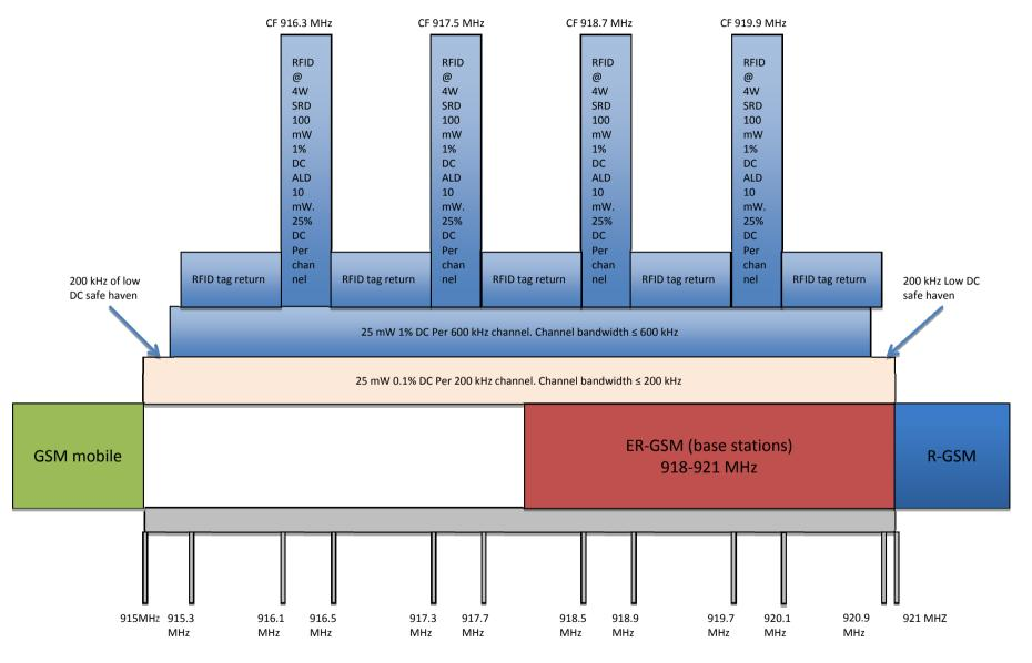
Figure 4: Band plan for 915-921 MHz
