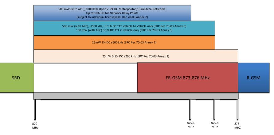
Figure 3: Band plan for 870-876 MHz
